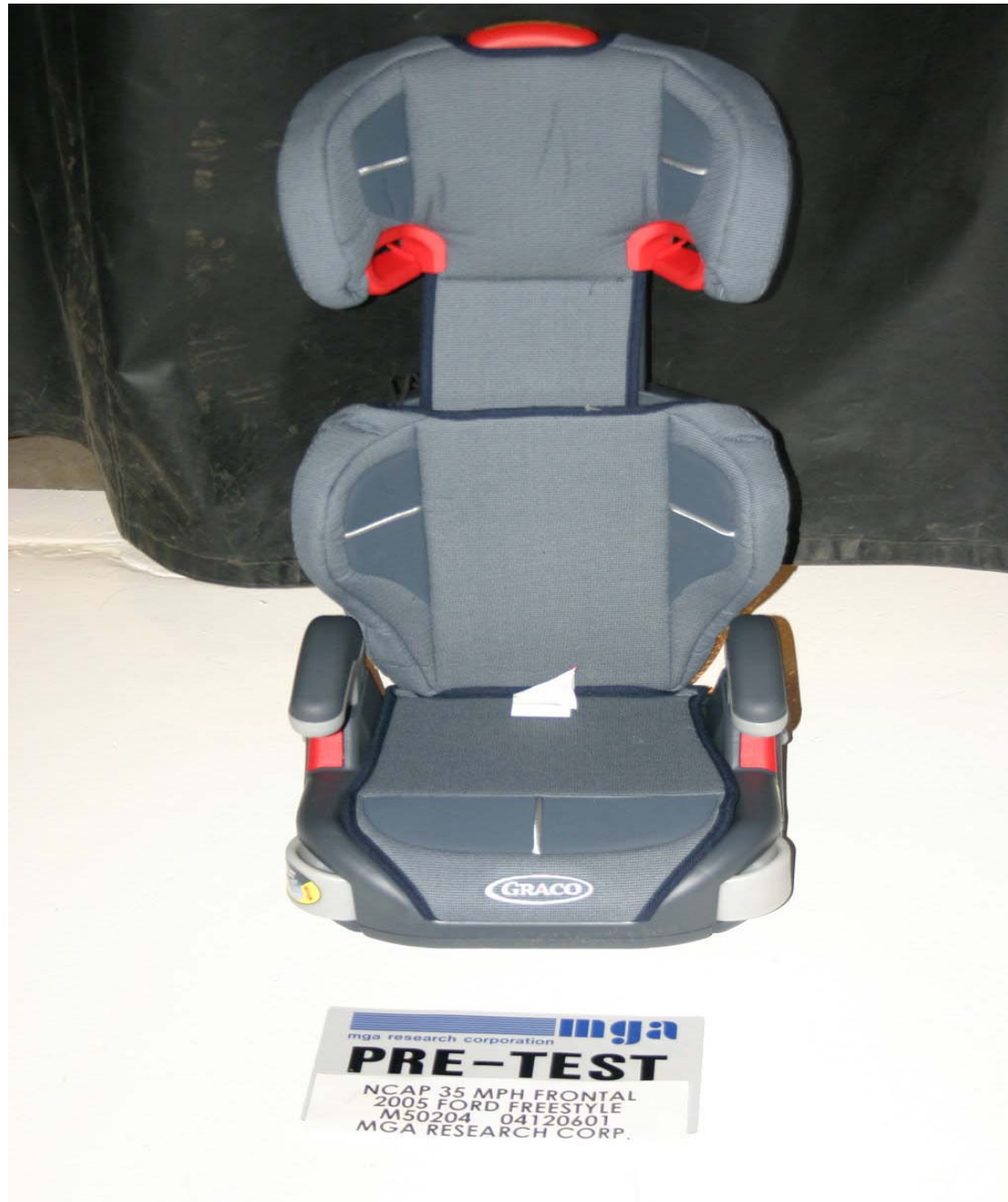
Pre-Test Front View of Position 4 CRS
