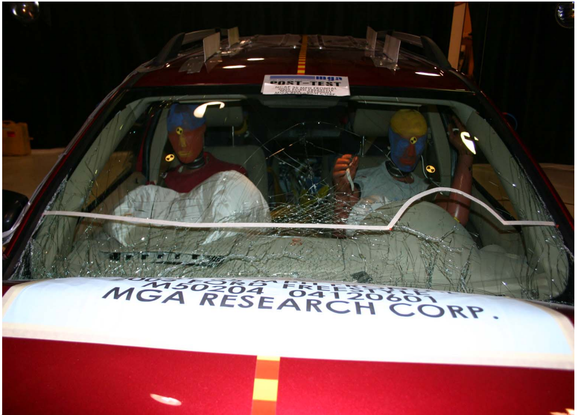
Post-Test Windshield View
