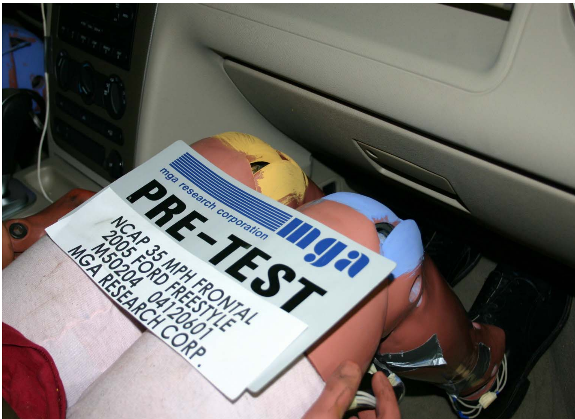
Pre-Test Passenger Side Knee Bolster View
