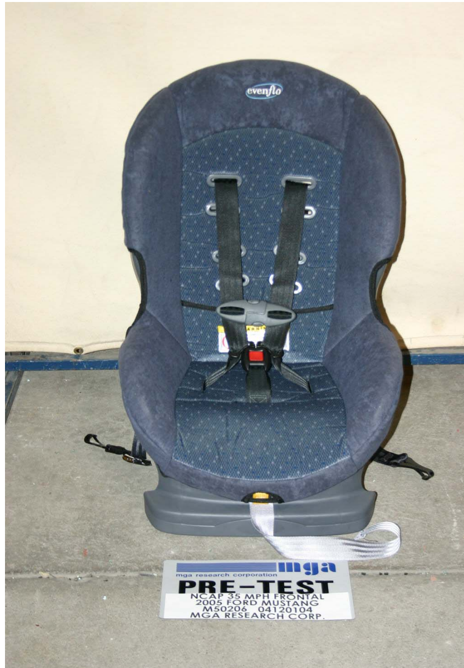
Pre-Test Front View of Position 3 CRS
