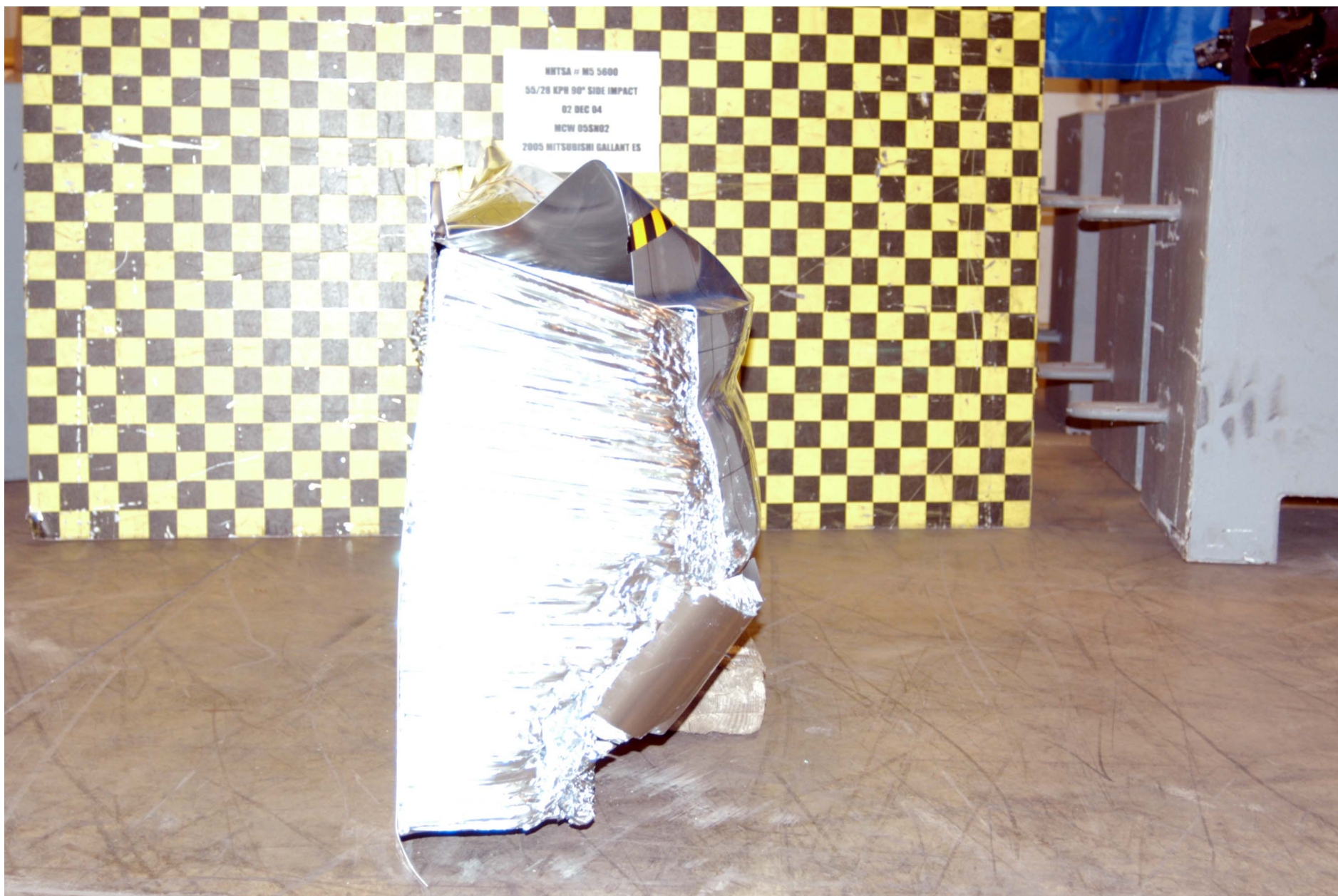
Figure A-52: POST-TEST ALUMINUM BARRIER RIGHT SIDE
