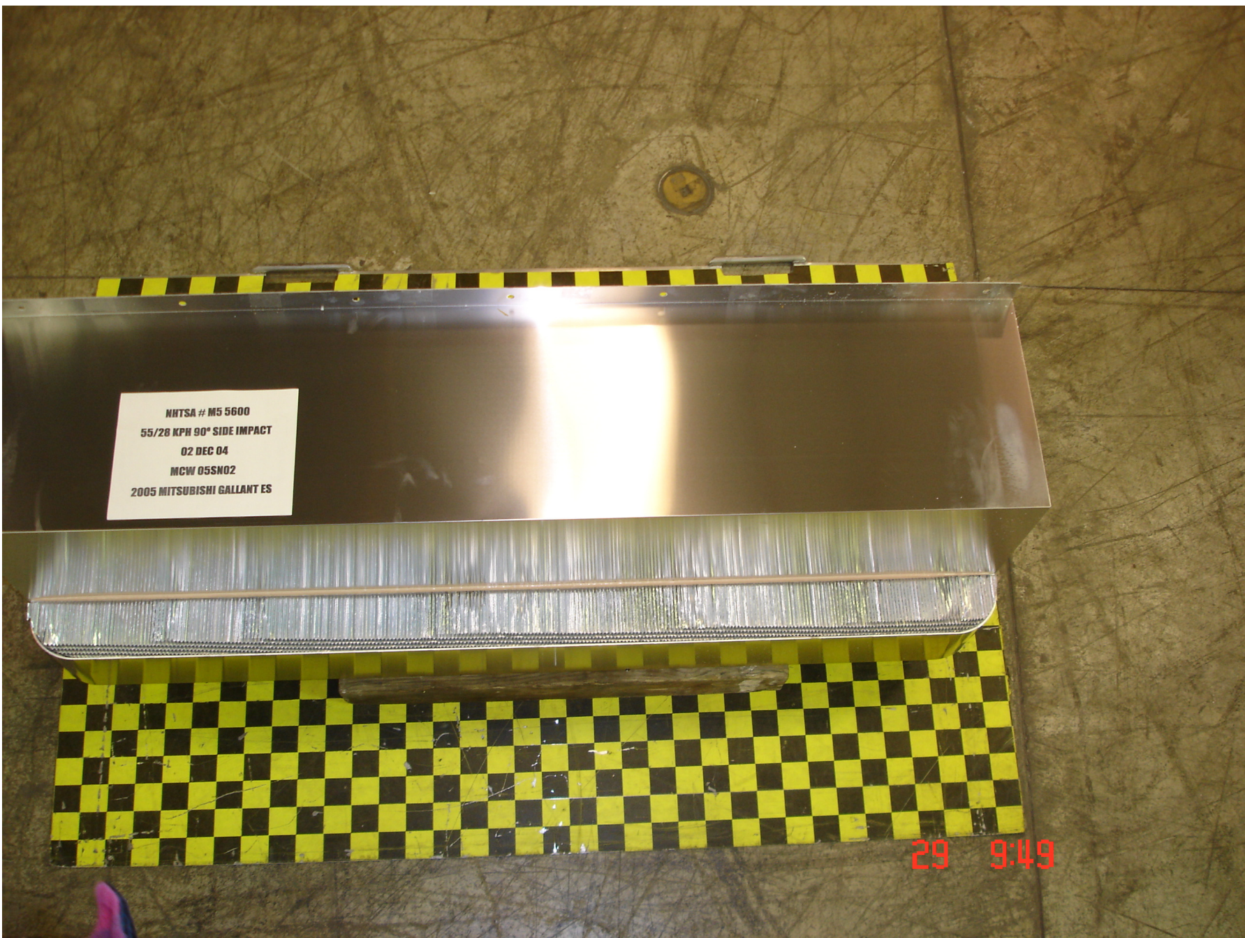
Figure A-53: PRE-TEST ALUMINUM BARRIER TOP
