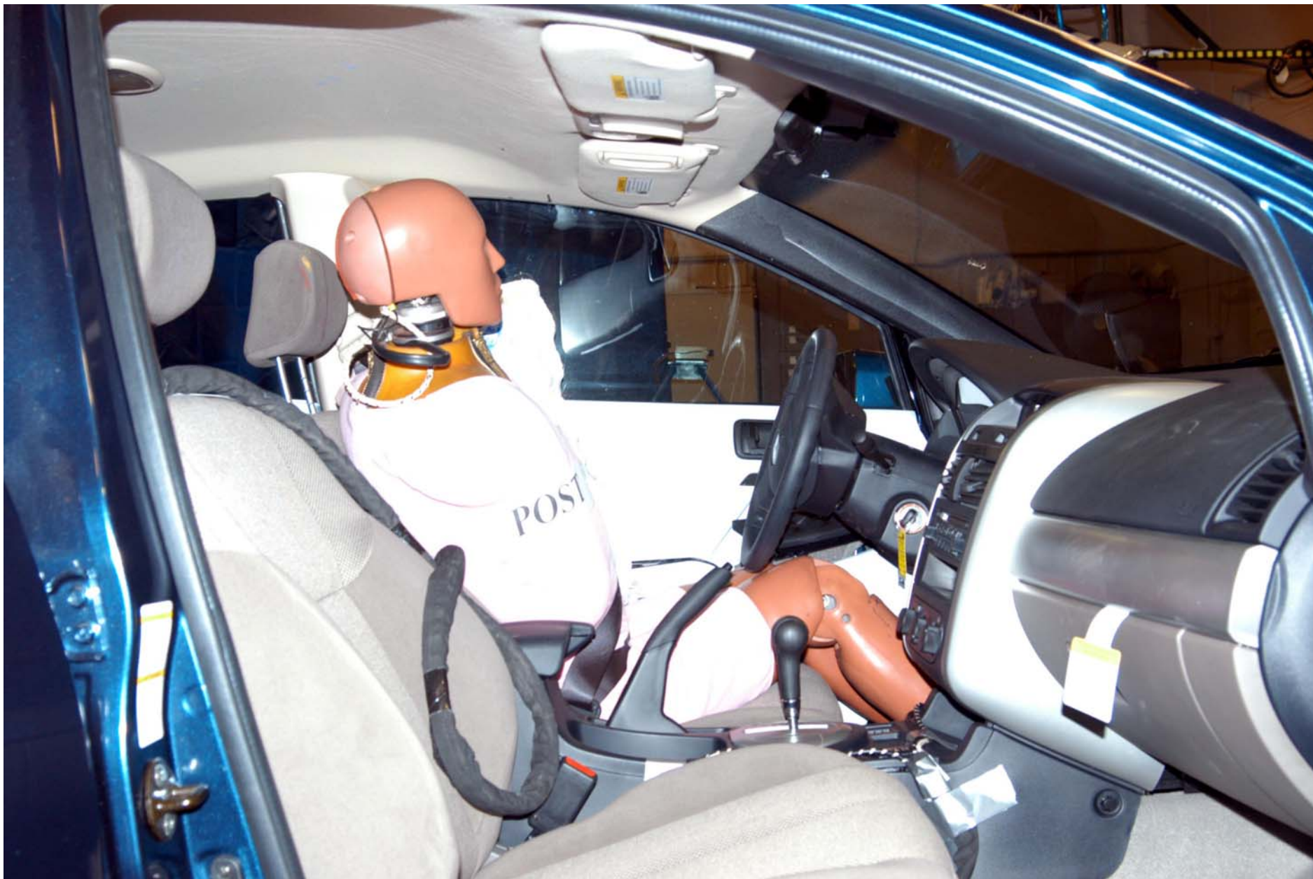
Figure A-18: POST-TEST RIGHT OCCUPANT COMPARTMENT VIEW OF FRONT SID H3
