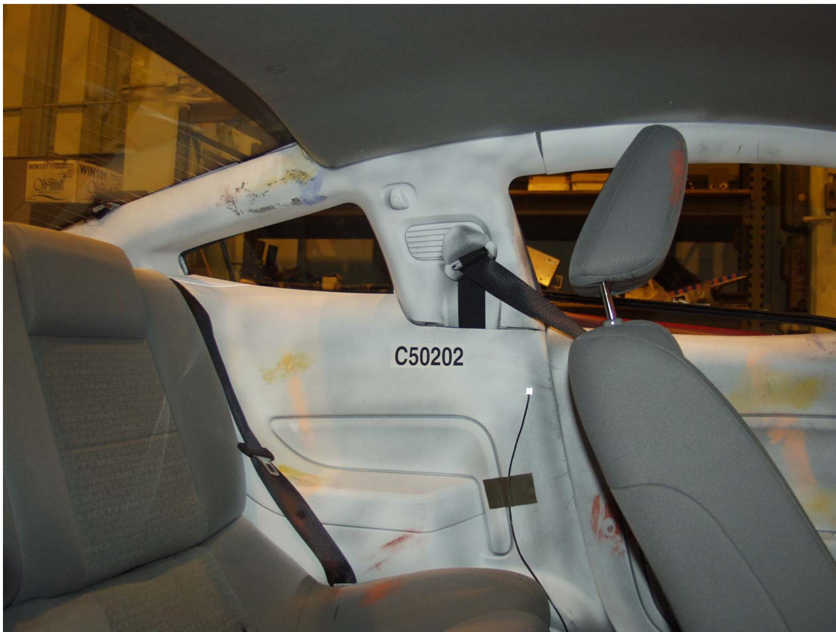
Figure A-36 POST-TEST INTERIOR OF REAR TRIM PANEL SHOWING SID H3 IMPACT LOCATIONS
