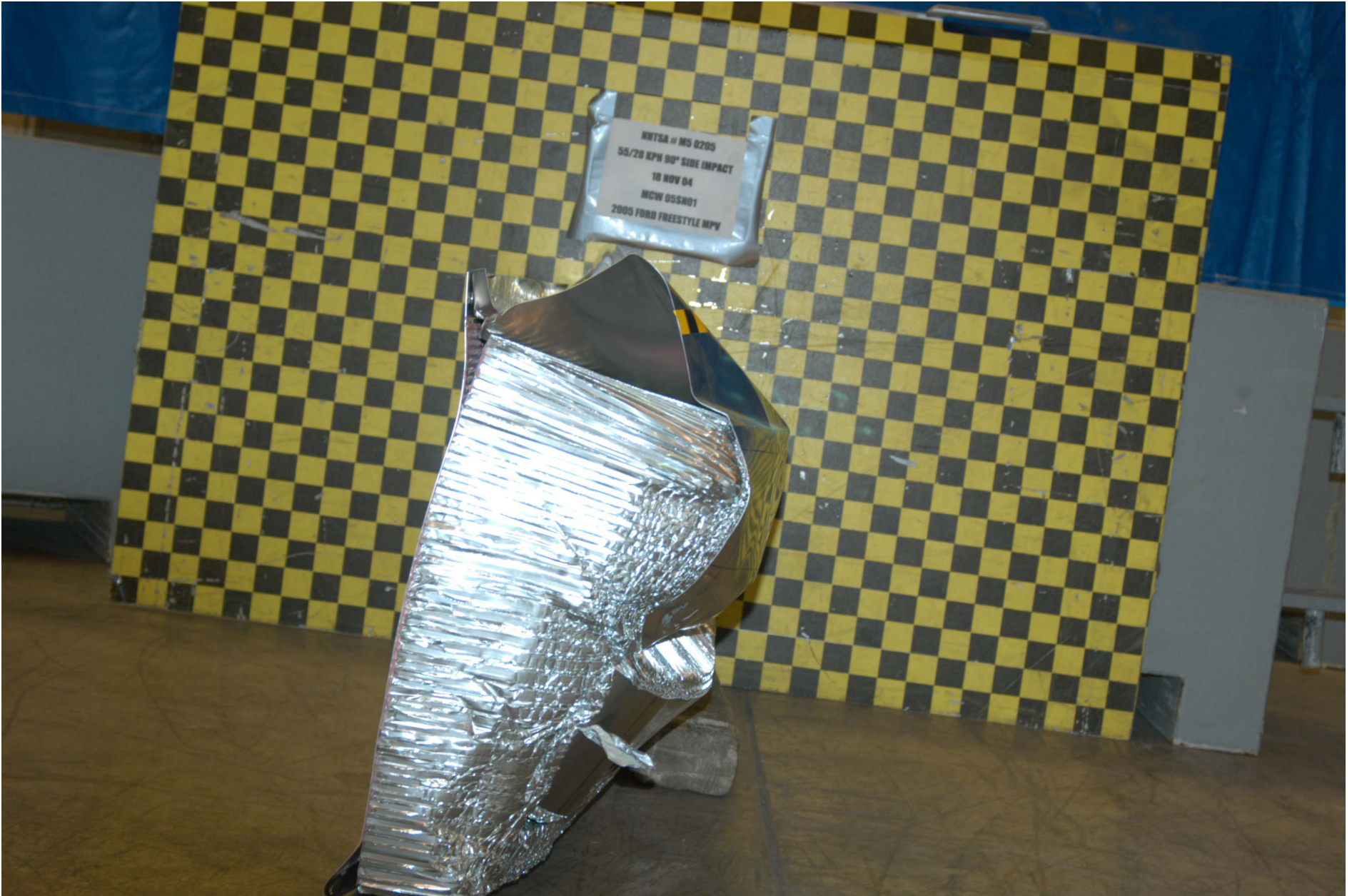
Figure A-52: POST-TEST ALUMINUM BARRIER RIGHT SIDE
