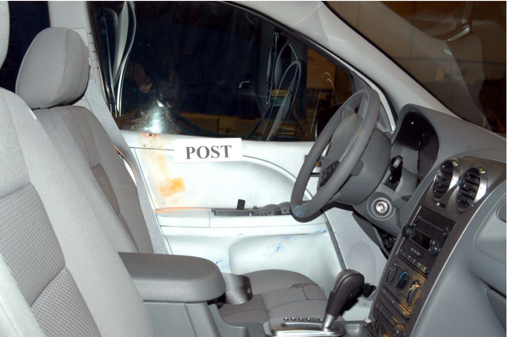
Figure A-26: POST-TEST INTERIOR OF FRONT DOOR SHOWING SID H3 IMPACT LOCATIONS
