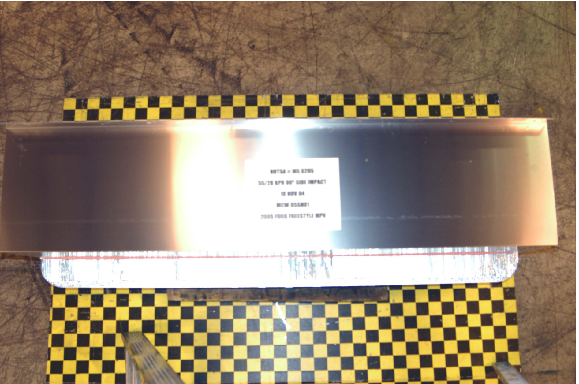
Figure A-53: PRE-TEST ALUMINUM BARRIER TOP
