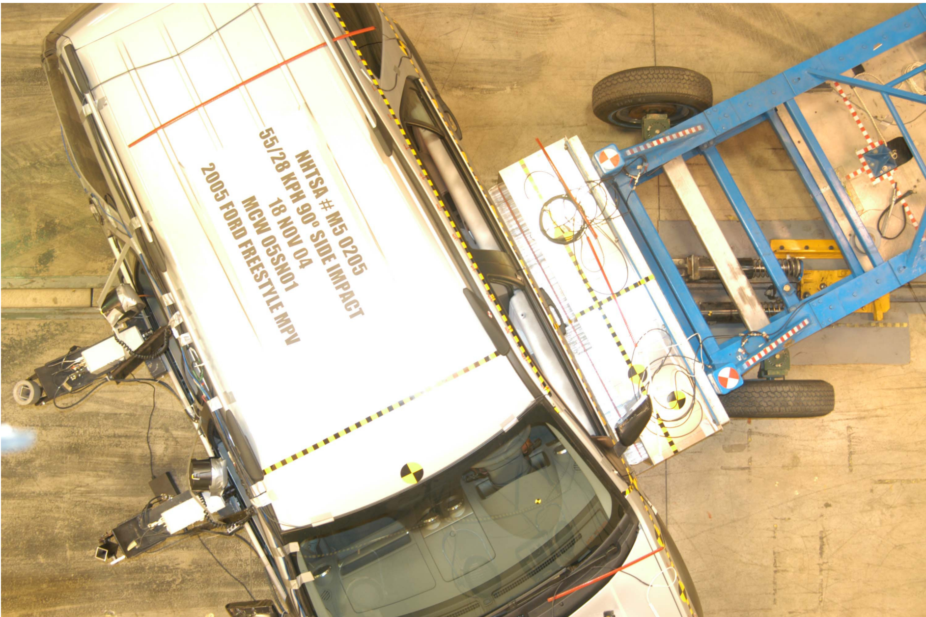
Figure A-35: PRE TEST OVERHEAD VIEW OF MDB IN IMPACT POSITION
