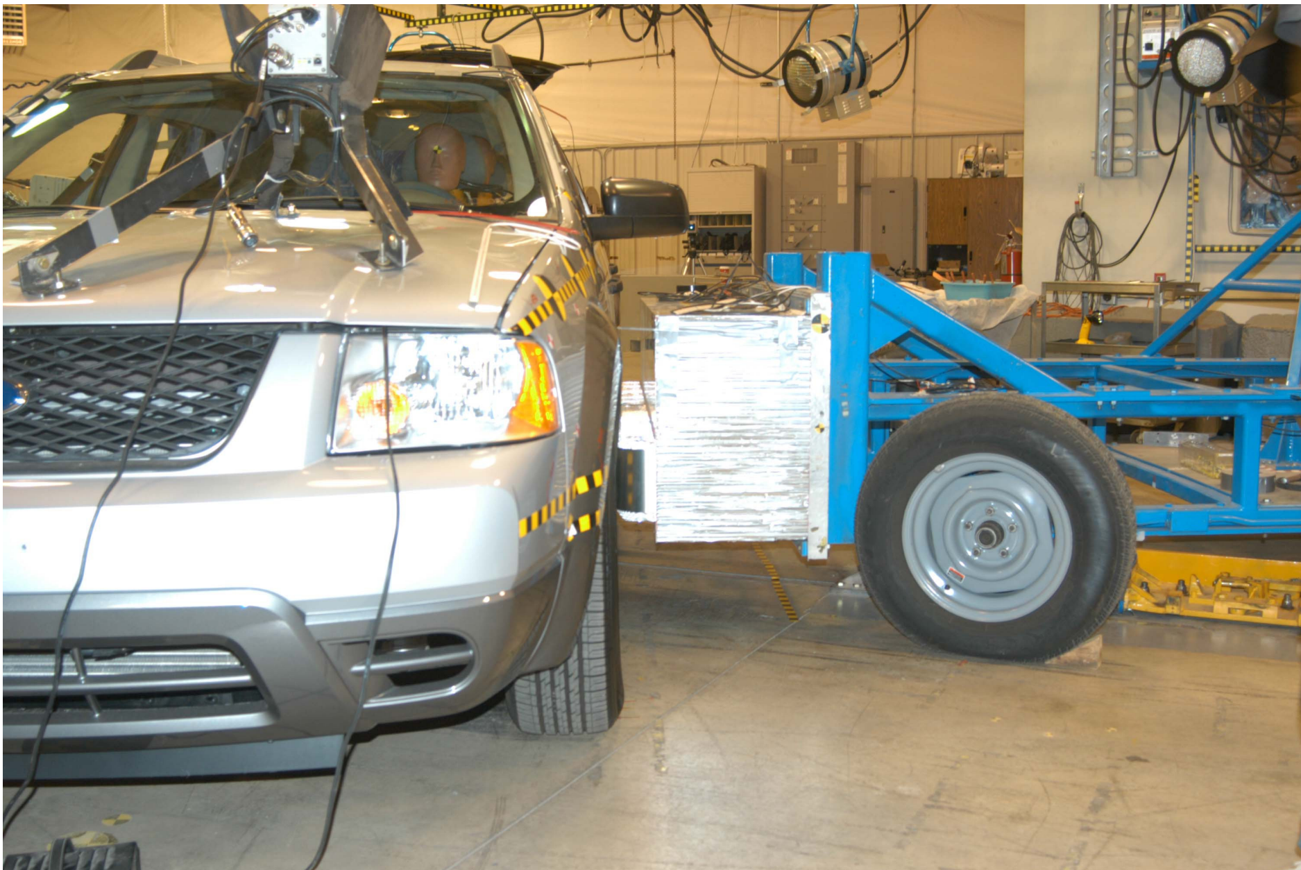
Figure A-31: PRE TEST LEFT SIDE VIEW OF MDB IN IMPACT POSITION
