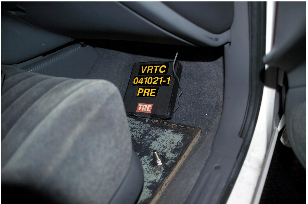
Figure A-50 Pre-Test Vehicle Ballast - View 2
