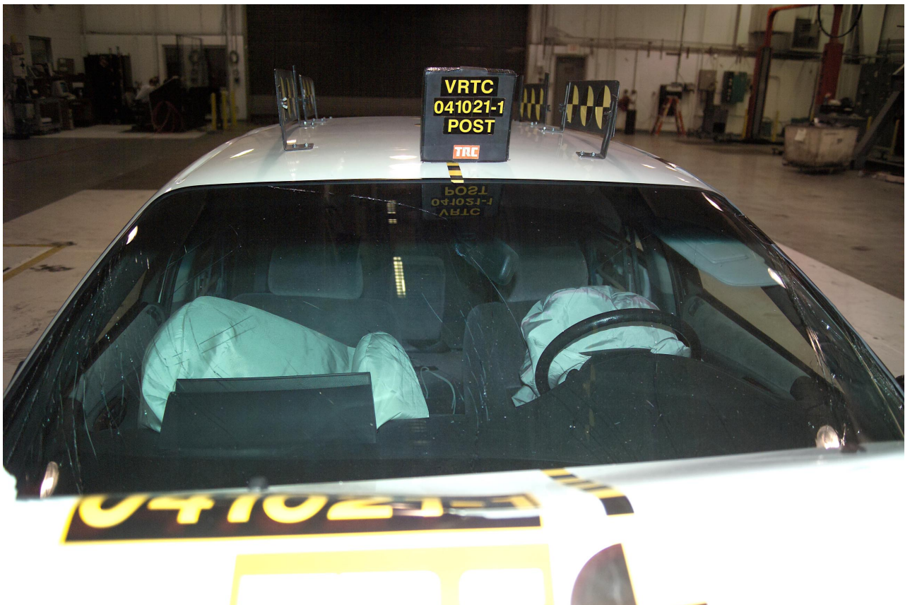
Figure A-31 Post-Test Windshield View
