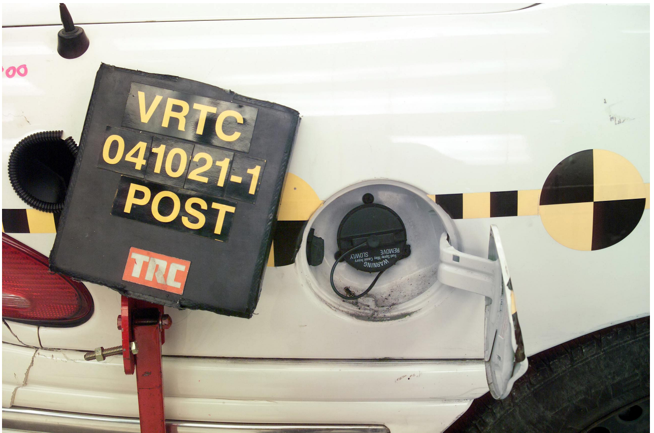
Figure A-28 Post-Test Fuel Filler Cap View
