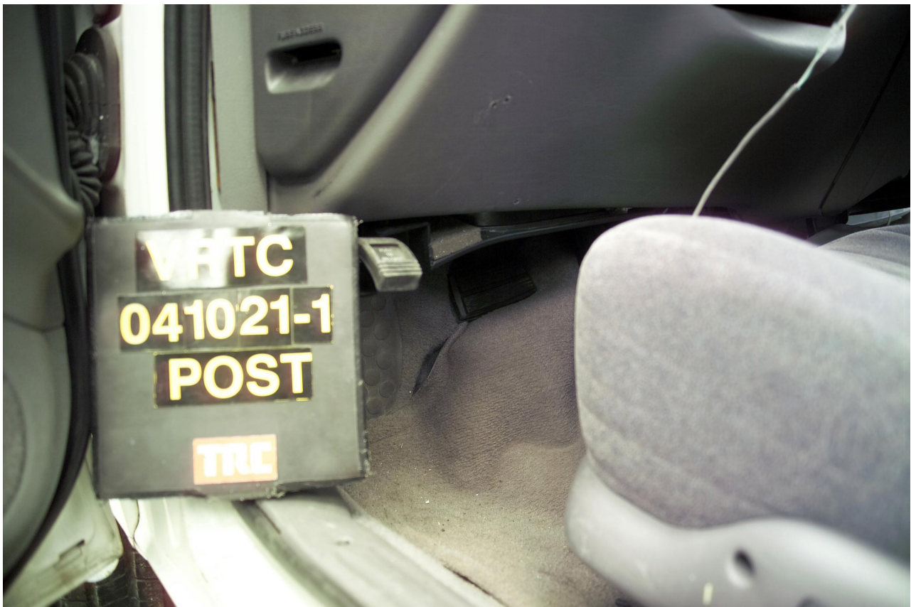
Figure A-34 Post-Test Driver Toe-board Deformation View
