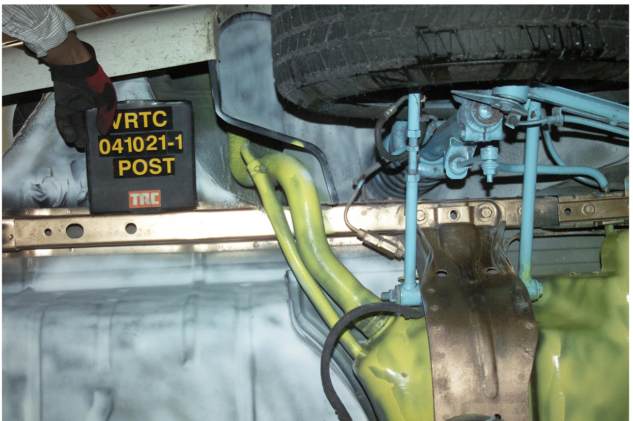
Figure A-26 Post-Test Fuel Filler Neck View
