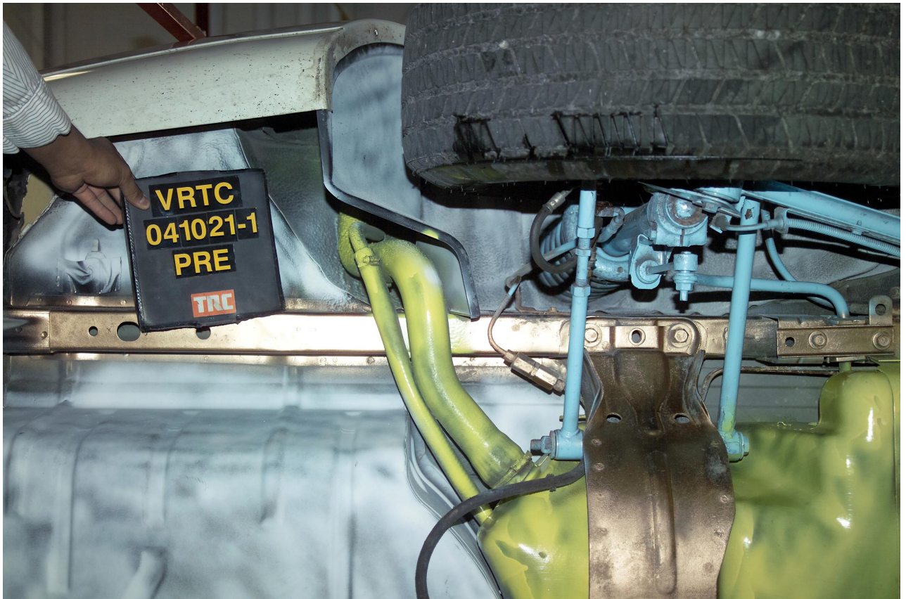
Figure A-25 Pre-Test Fuel Filler Neck View
