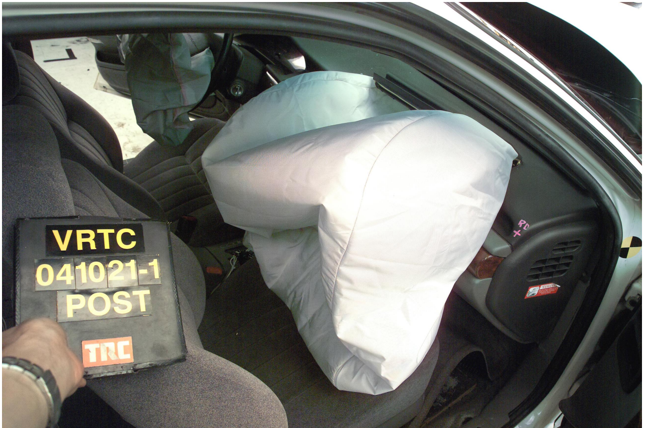
Figure A-35 Post-Test Passenger Airbag View
