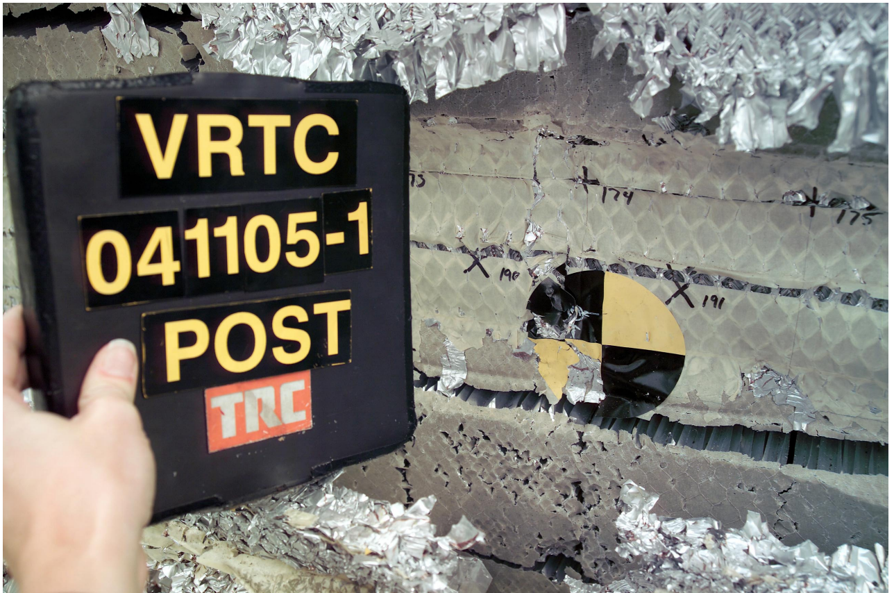
Figure A-46 Post-Test Vehicle Impact Point Deviation View
