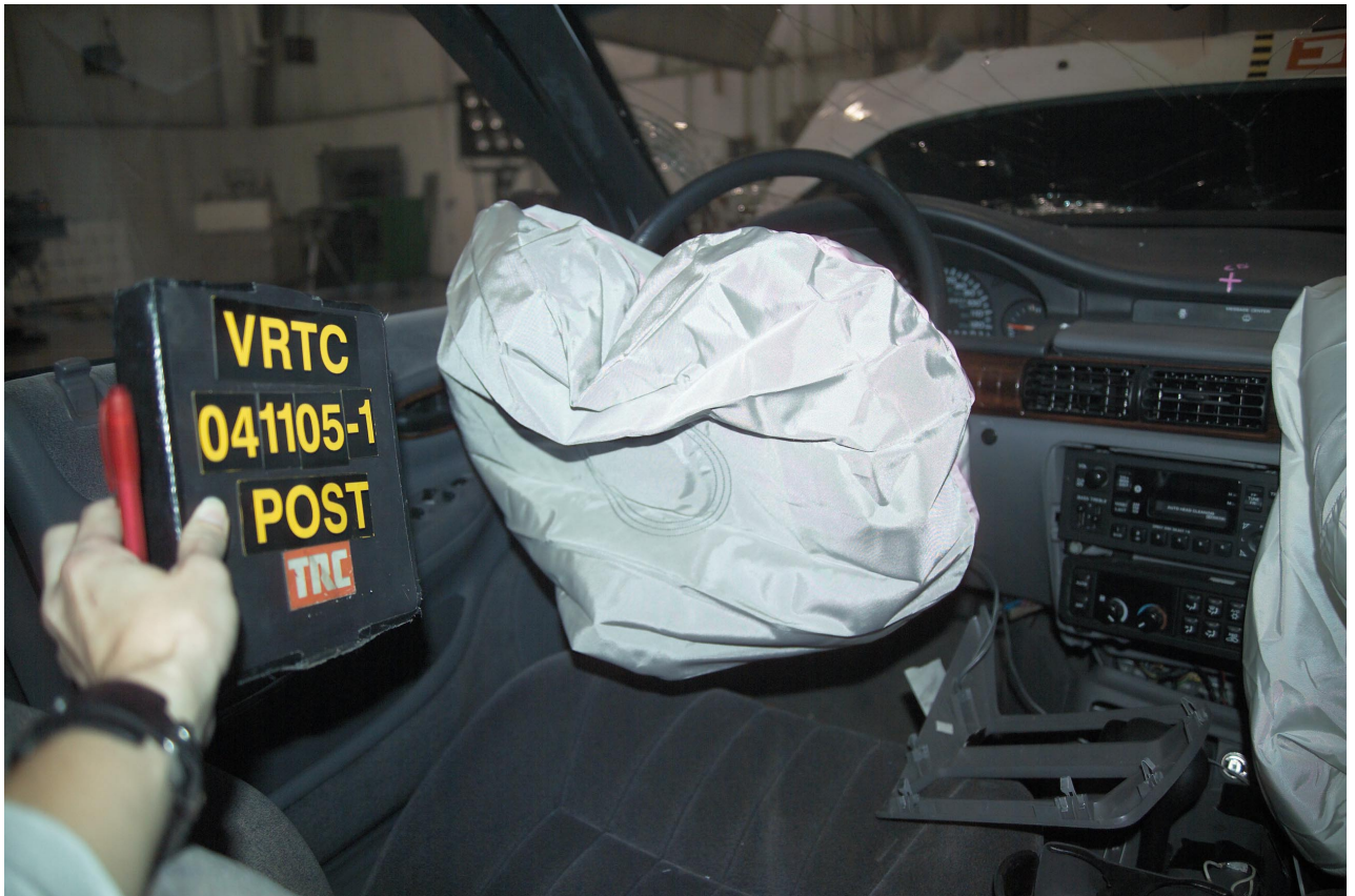
Figure A-33 Post-Test Driver Airbag View
