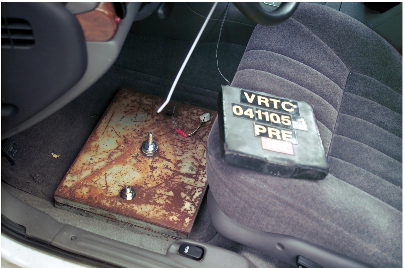
Figure A-47 Pre-Test Vehicle Ballast View
