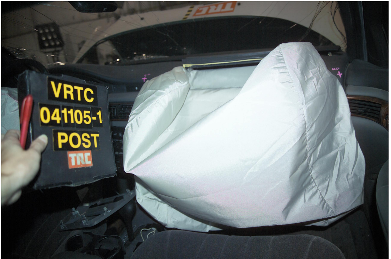
Figure A-35 Post-Test Passenger Airbag View
