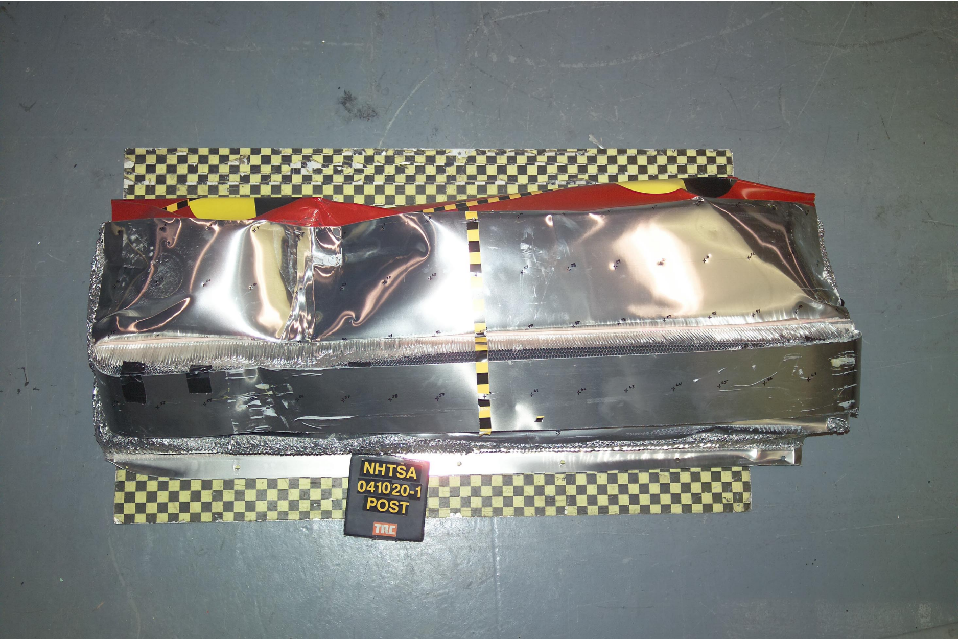
Figure A-10 Post-Test Frontal View of Impactor Face A-14
