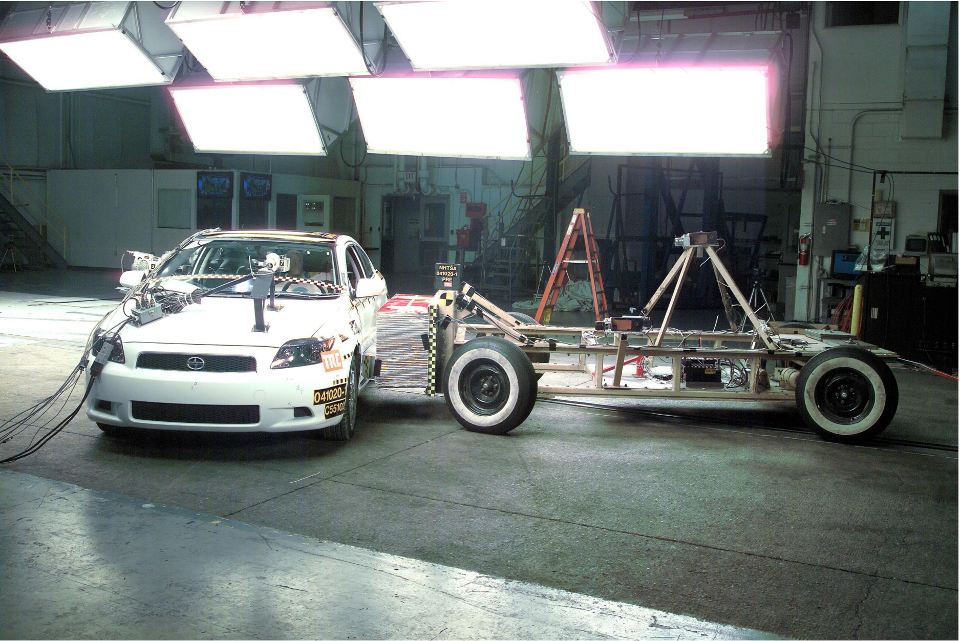
Figure A-45 Pre-Test Left Side View of MDB With Impactor Face in Position A-49
