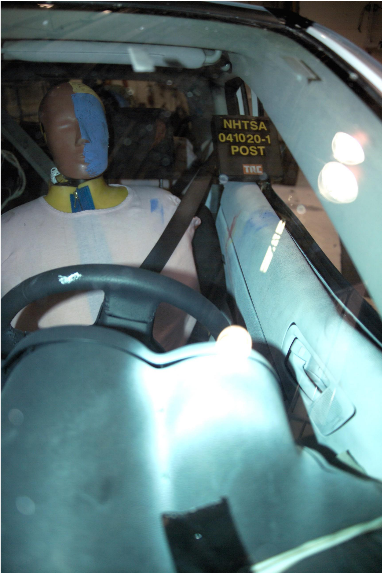
Figure A-30 Post-Test View of Front SID HIII and Door Clearance
