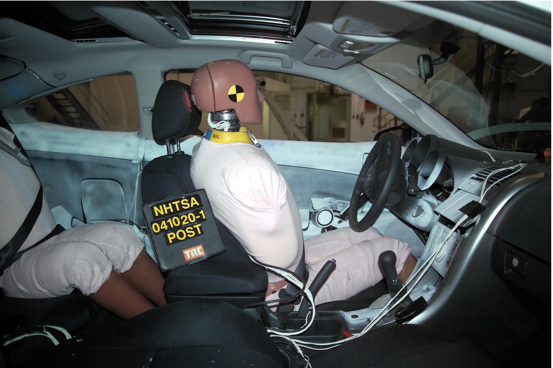
Figure A-22 Post-Test Right Occupant Compartment View of Front SID HIII
