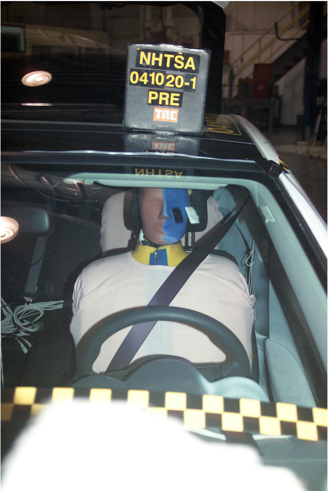
Figure A-29 Pre-Test View of Front SID HIII and Door Clearance
