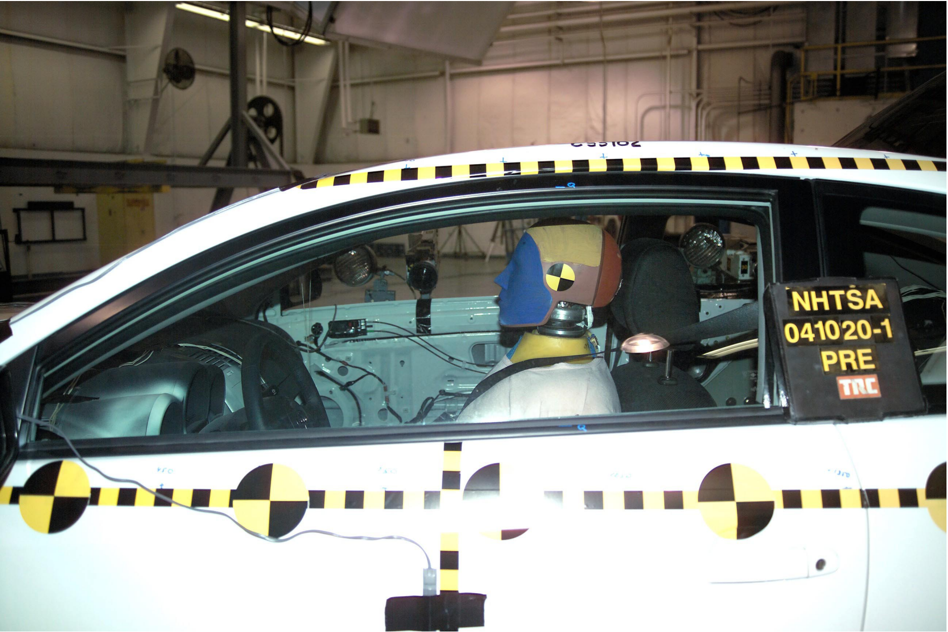
Figure A-25 Pre-Test Left View of Front SID IIII A-29
