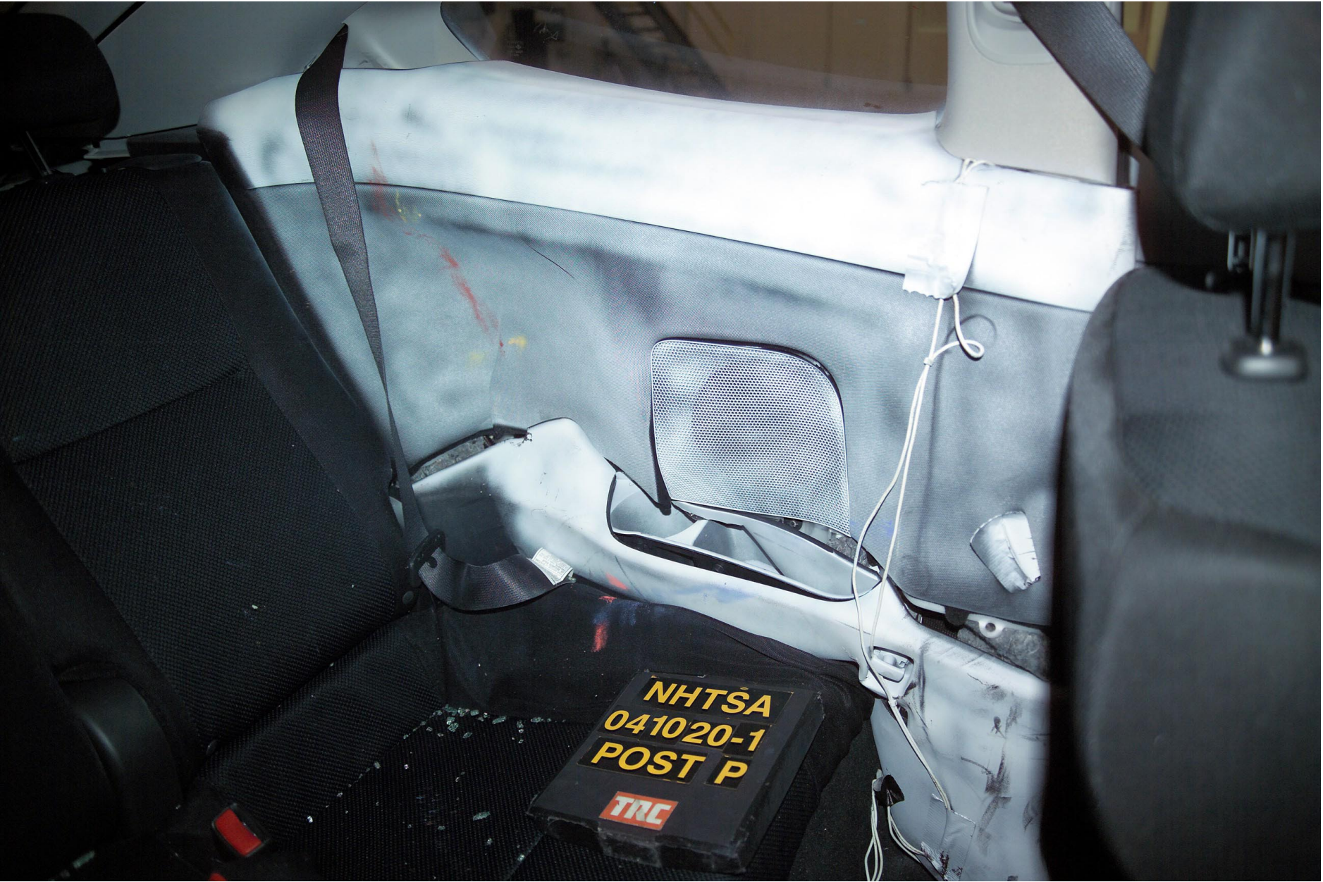
Figure A-40 Post-Test Interior of Rear Panel Showing SID HIII Impact Locations
