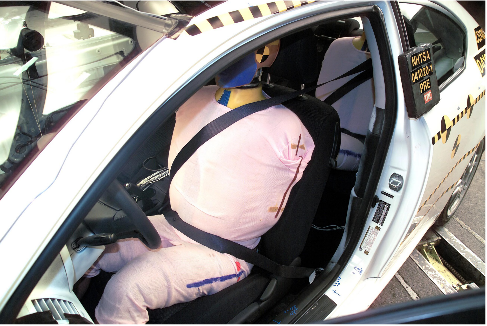
Figure A-27 Pre-Test Left View of Front SID HIII and Belt Position A-31
