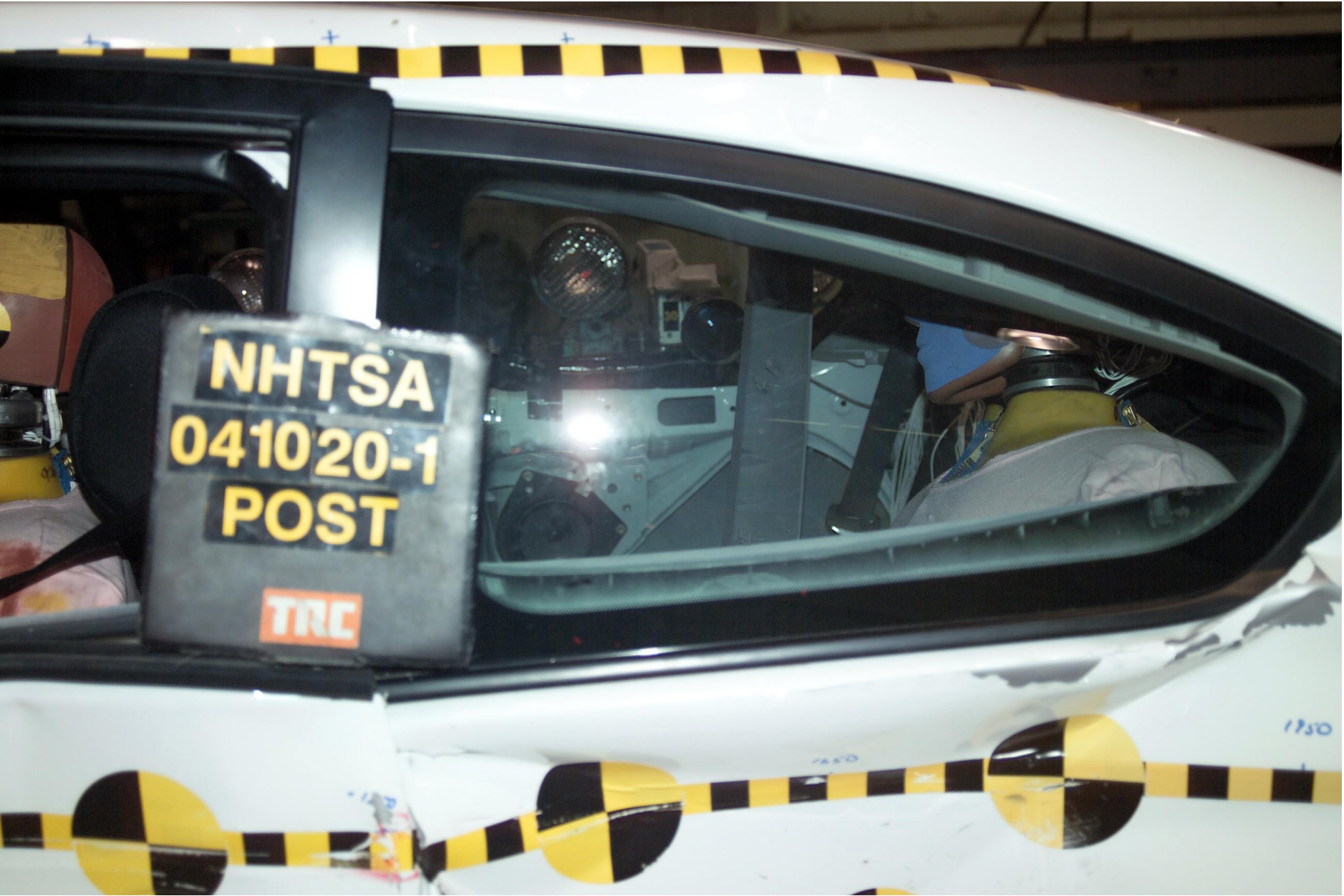
Figure A-32 Post-Test Left View of Rear SID HIII A-36
