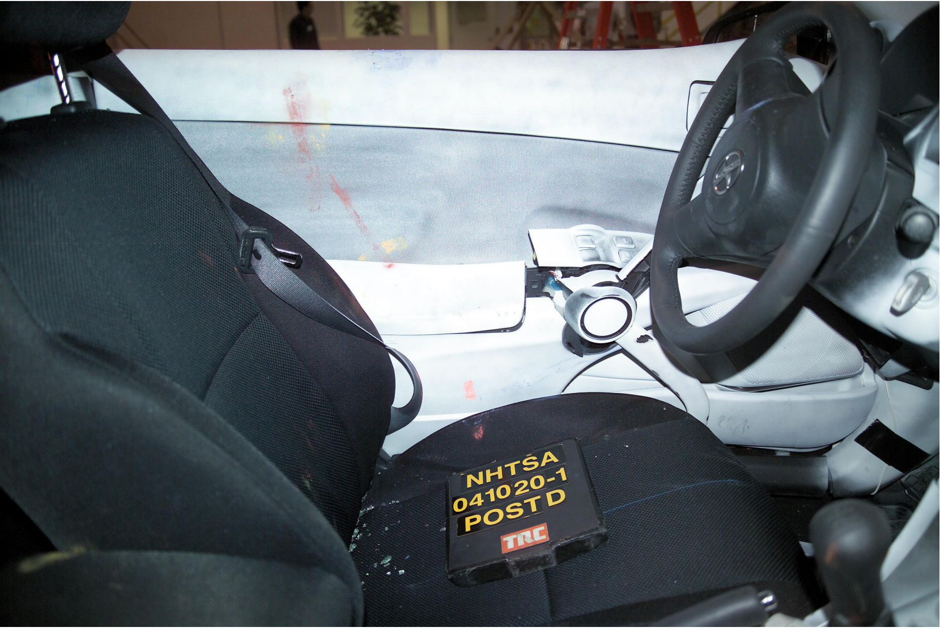
Figure A-36 Post-Test Interior of Front Door Showing SID HIII Impact Locations A-40
