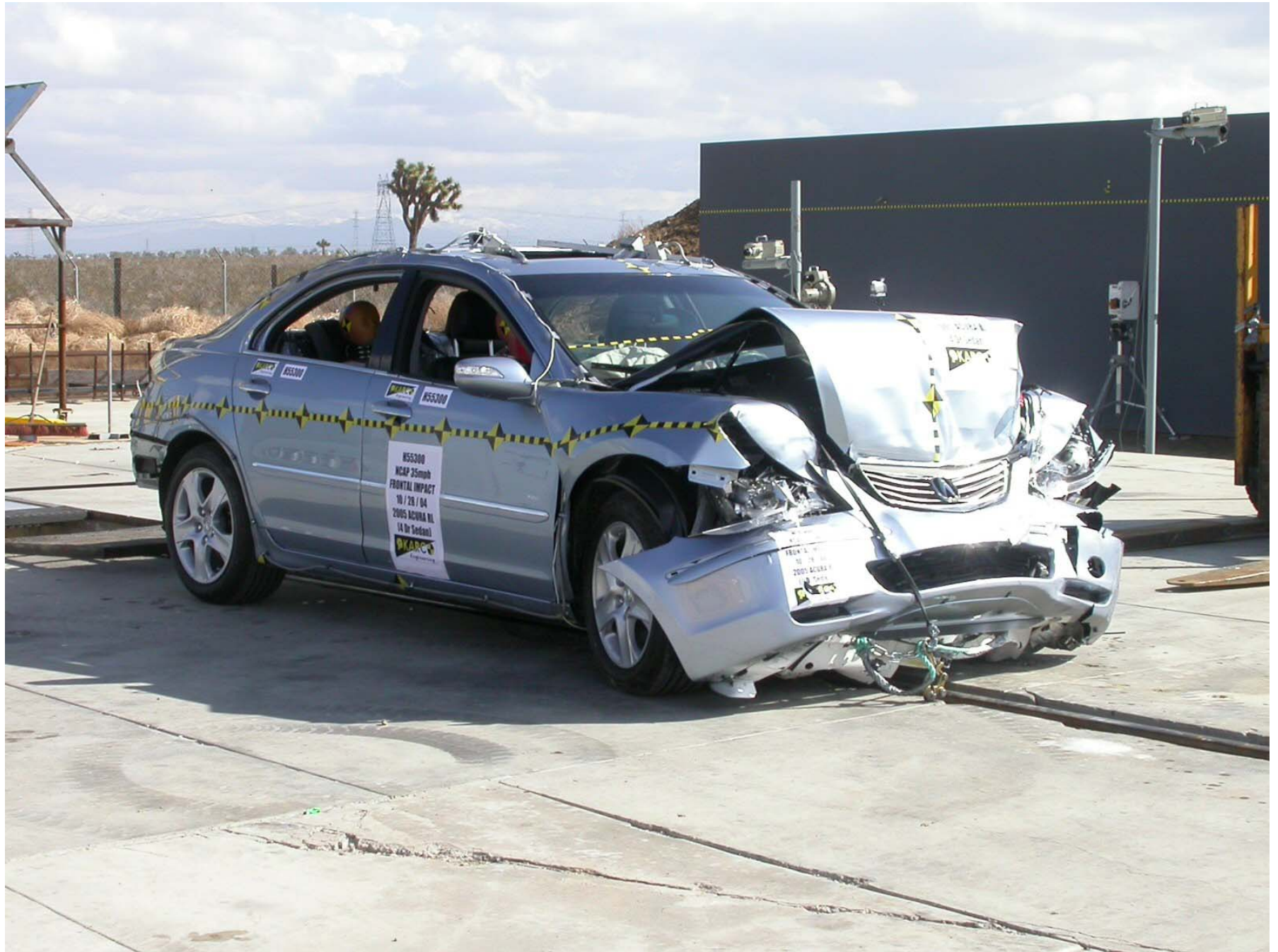
Figure A-14: Post-Test Right Front ¾ View (Vehicle Moved)
