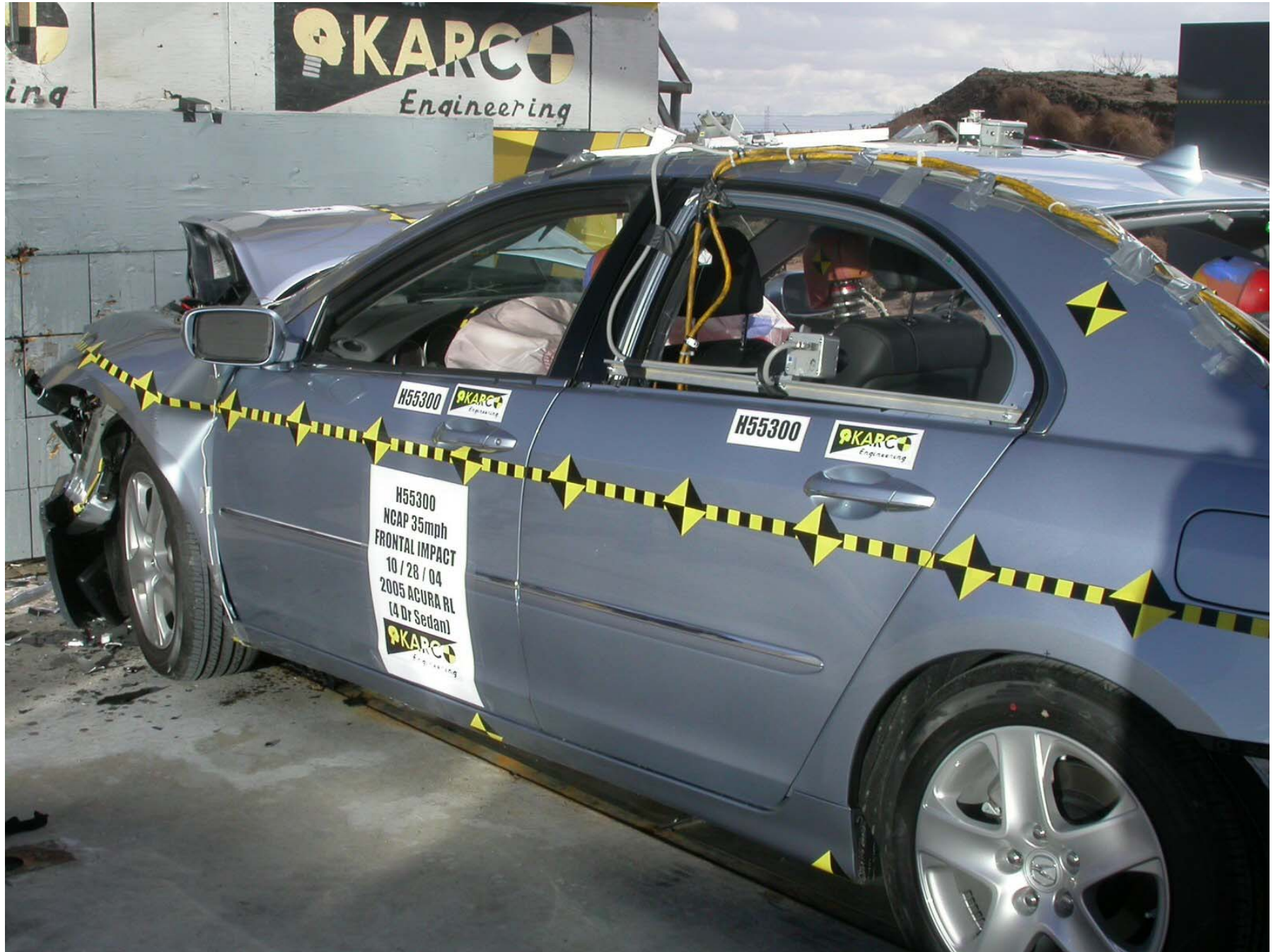
Figure A-17: Left Rear ¾ View of Doors After Impact
