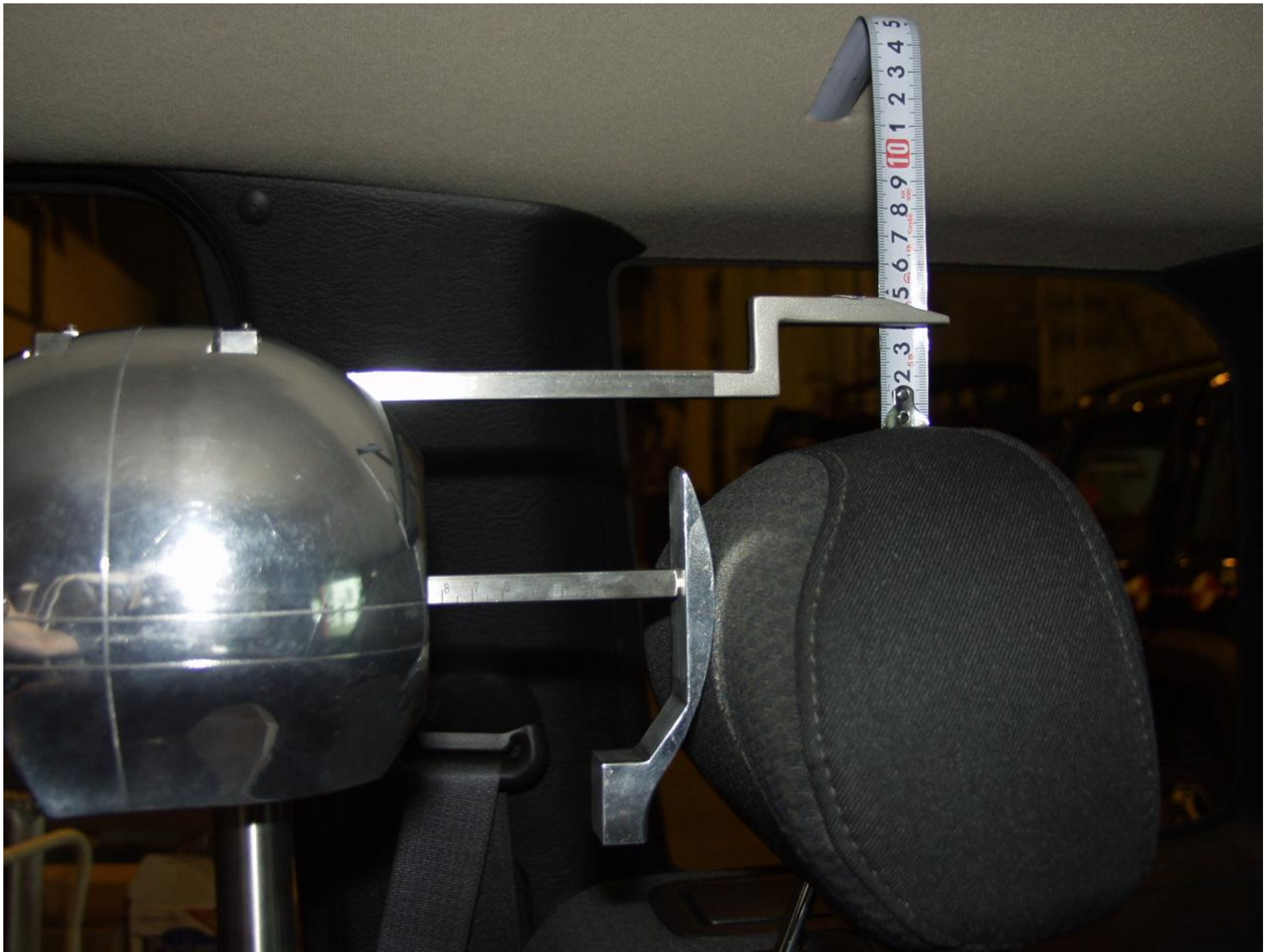
Figure A-2 PASSENGER ICBC BACKSET VIEW
