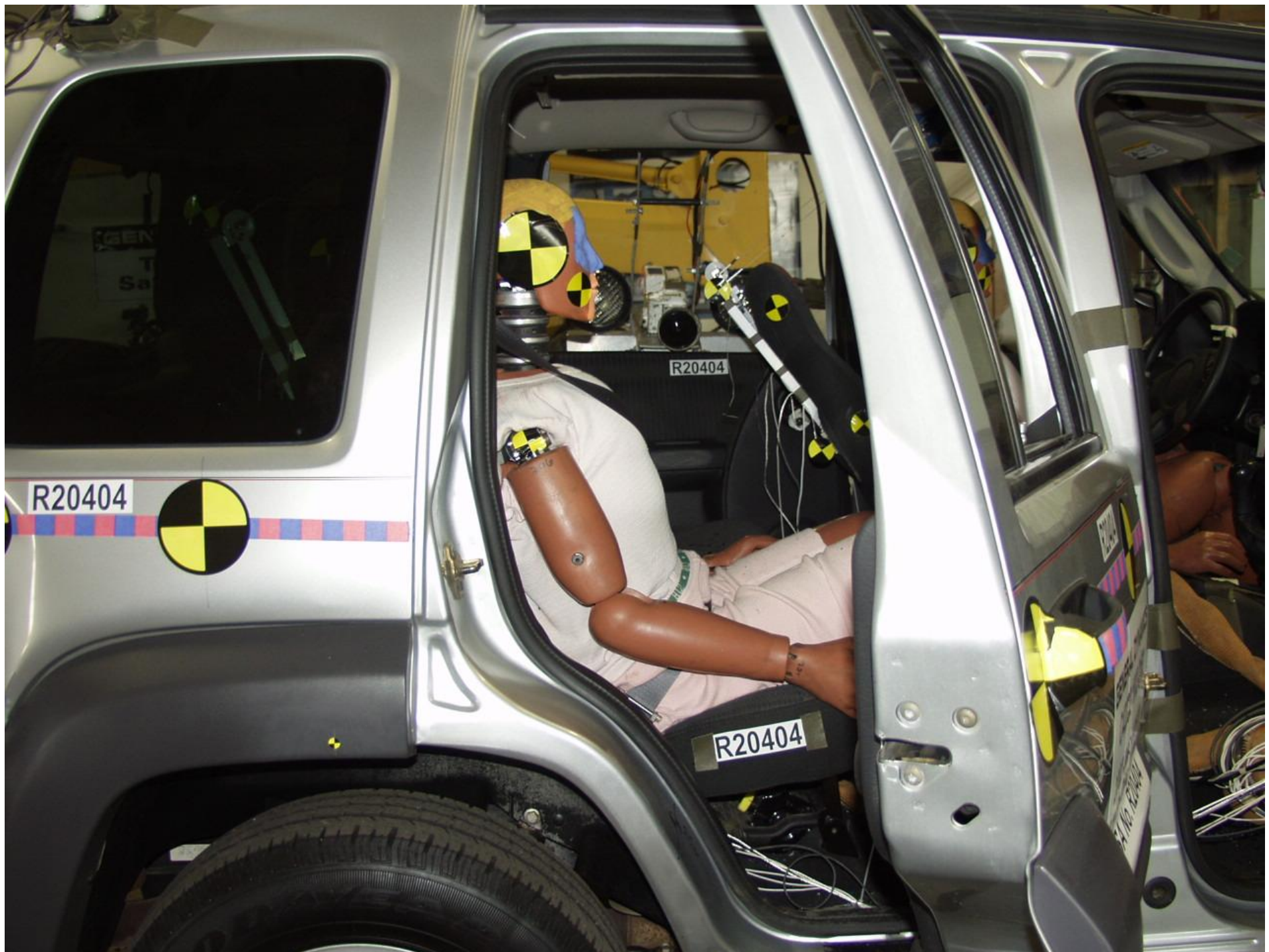
Figure A-22 POST-TEST PASSENGER RIGHT SIDE VIEW
