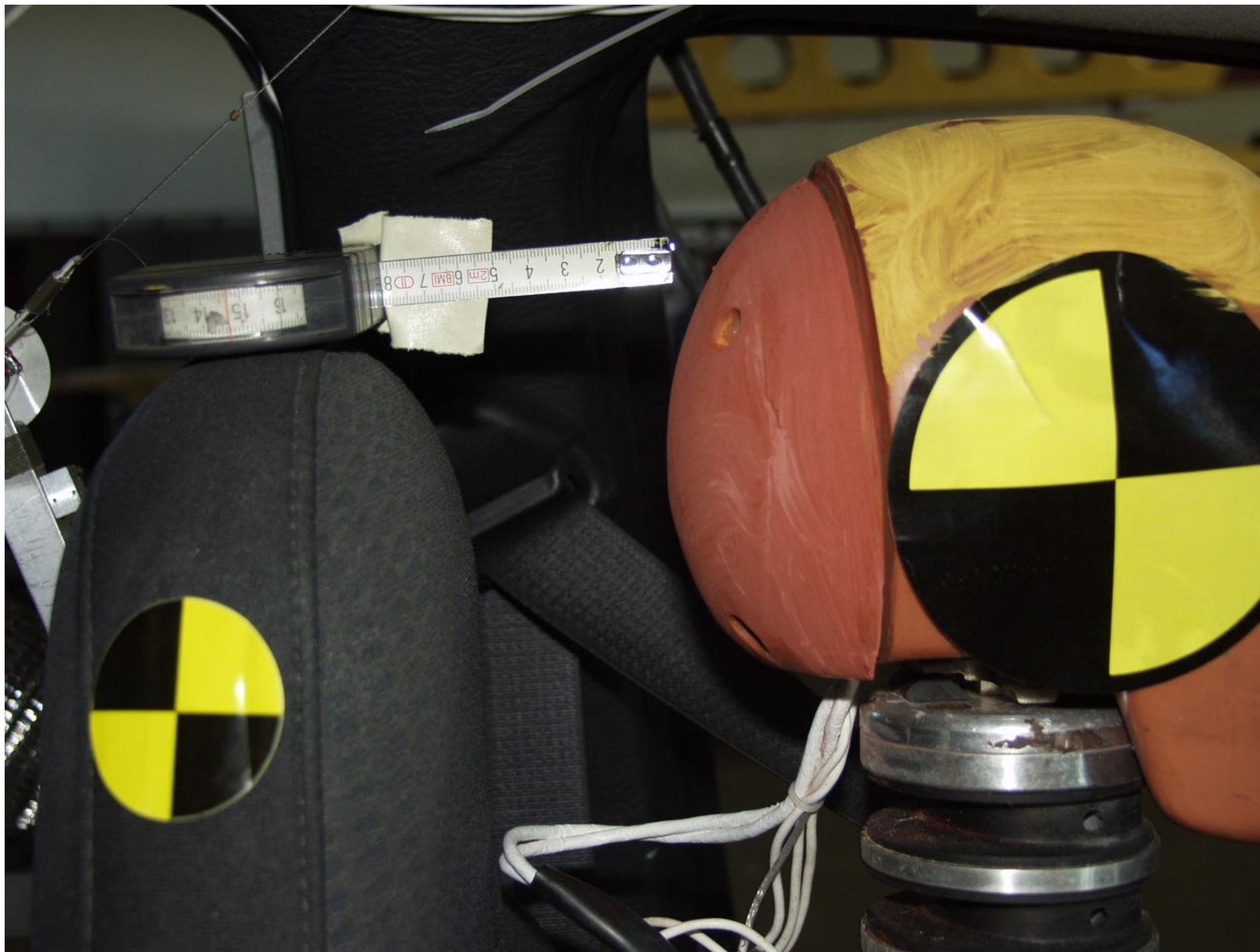
Figure A-3 PRE-TEST DRIVER BACKSET VIEW
