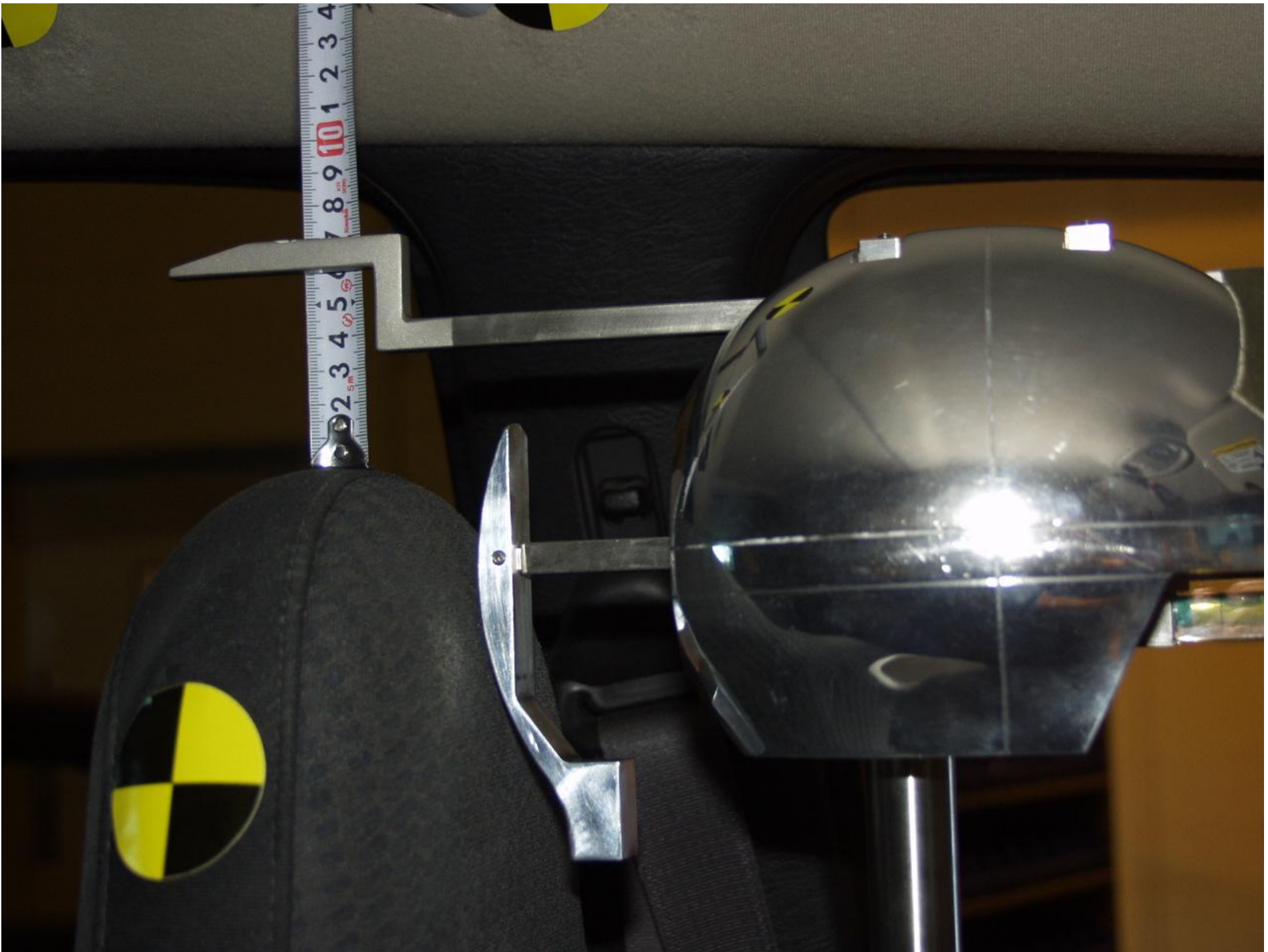
Figure A-1 DRIVER ICBC BACKSET VIEW
