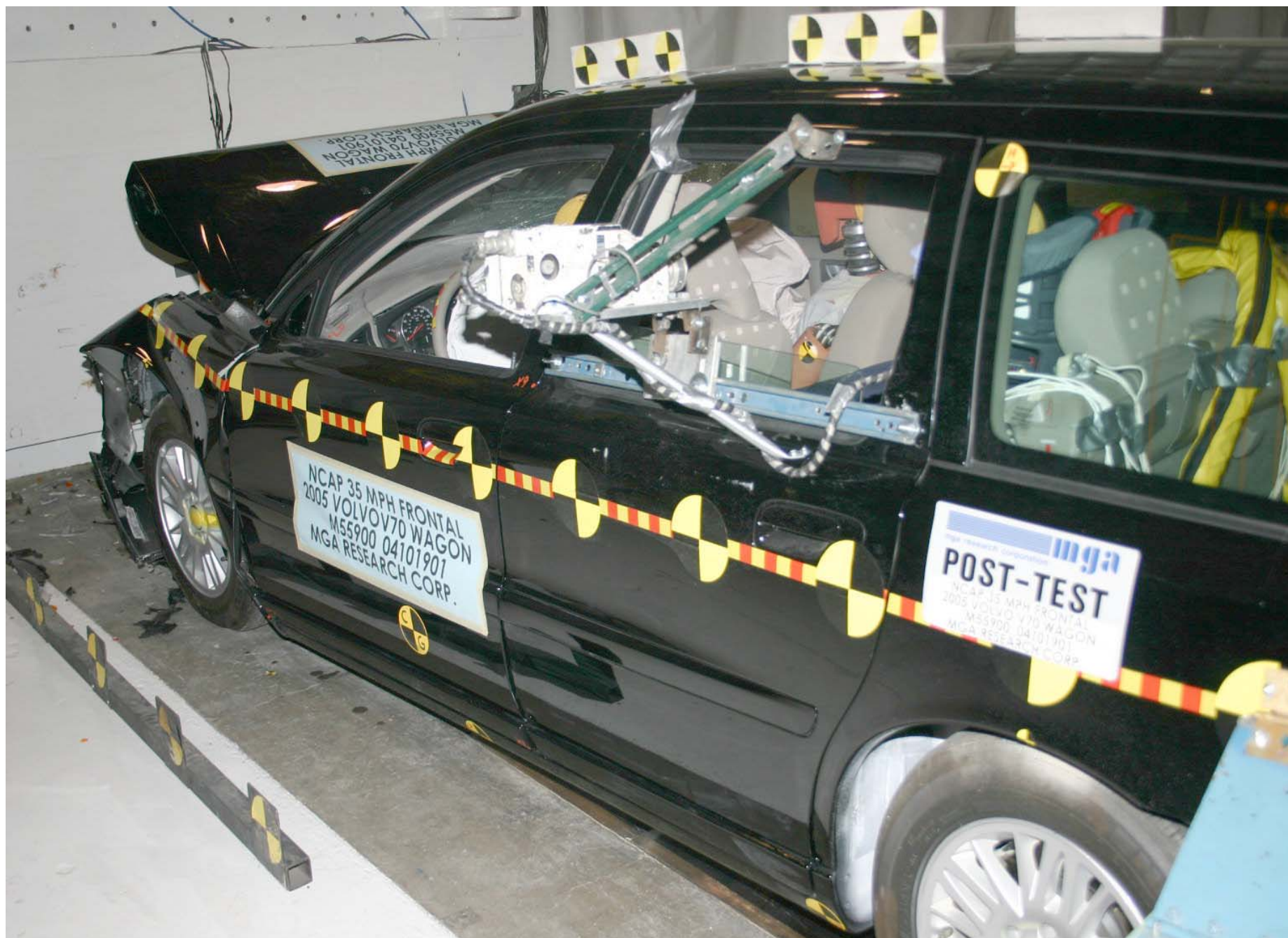
Post-Test Left Side Three-Quarter View of Doors After Impact
