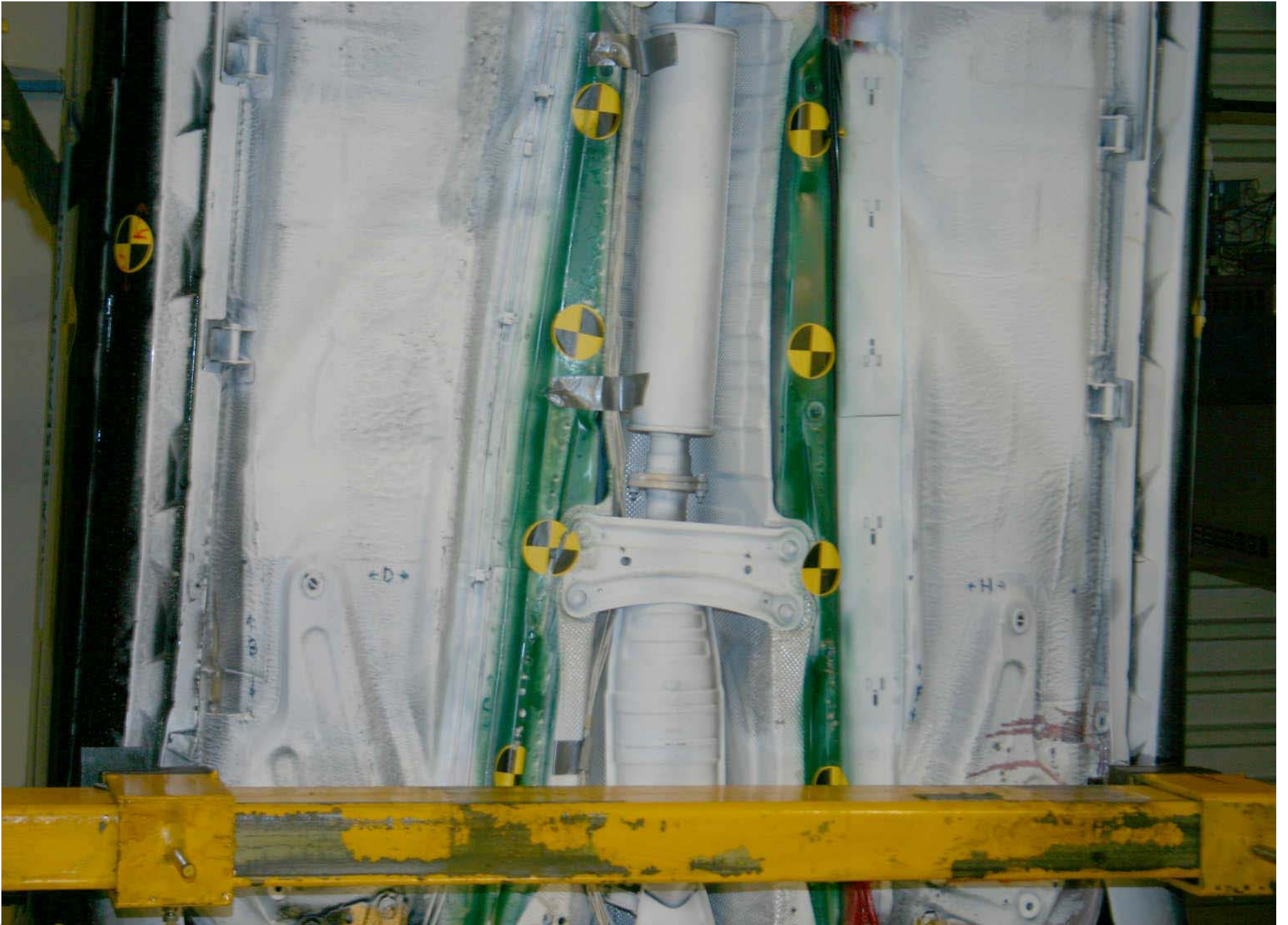
Post-Test Front Mid Underbody
