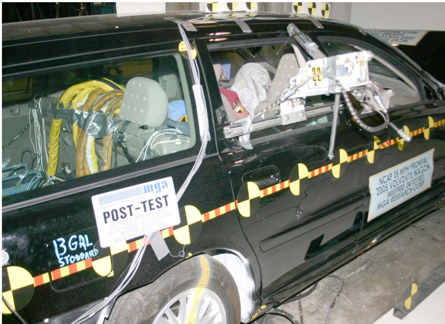
Post-Test Right Side Three-Quarter View of Doors After Impact
