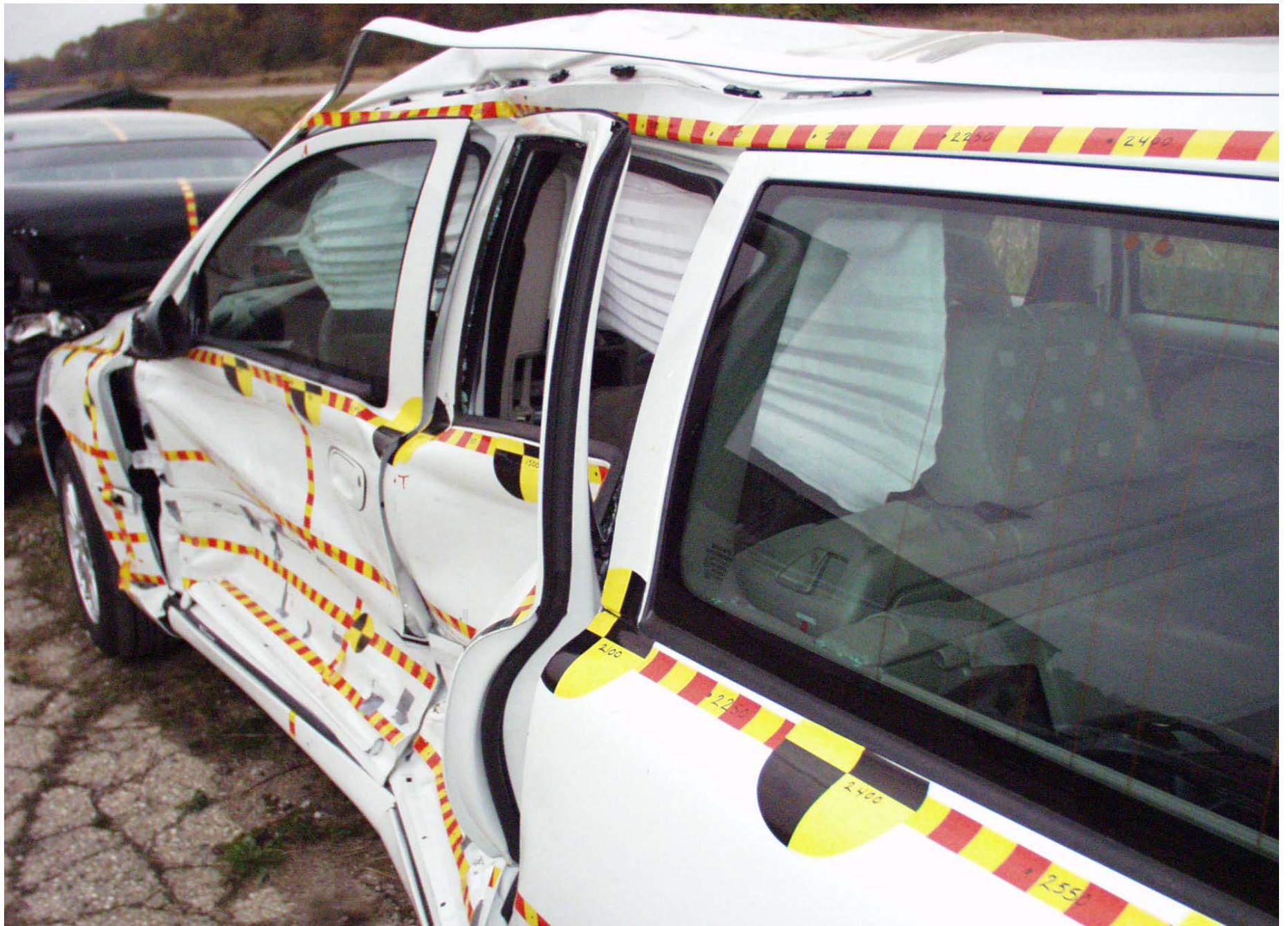
Post-Test Left Rear Door Opening
