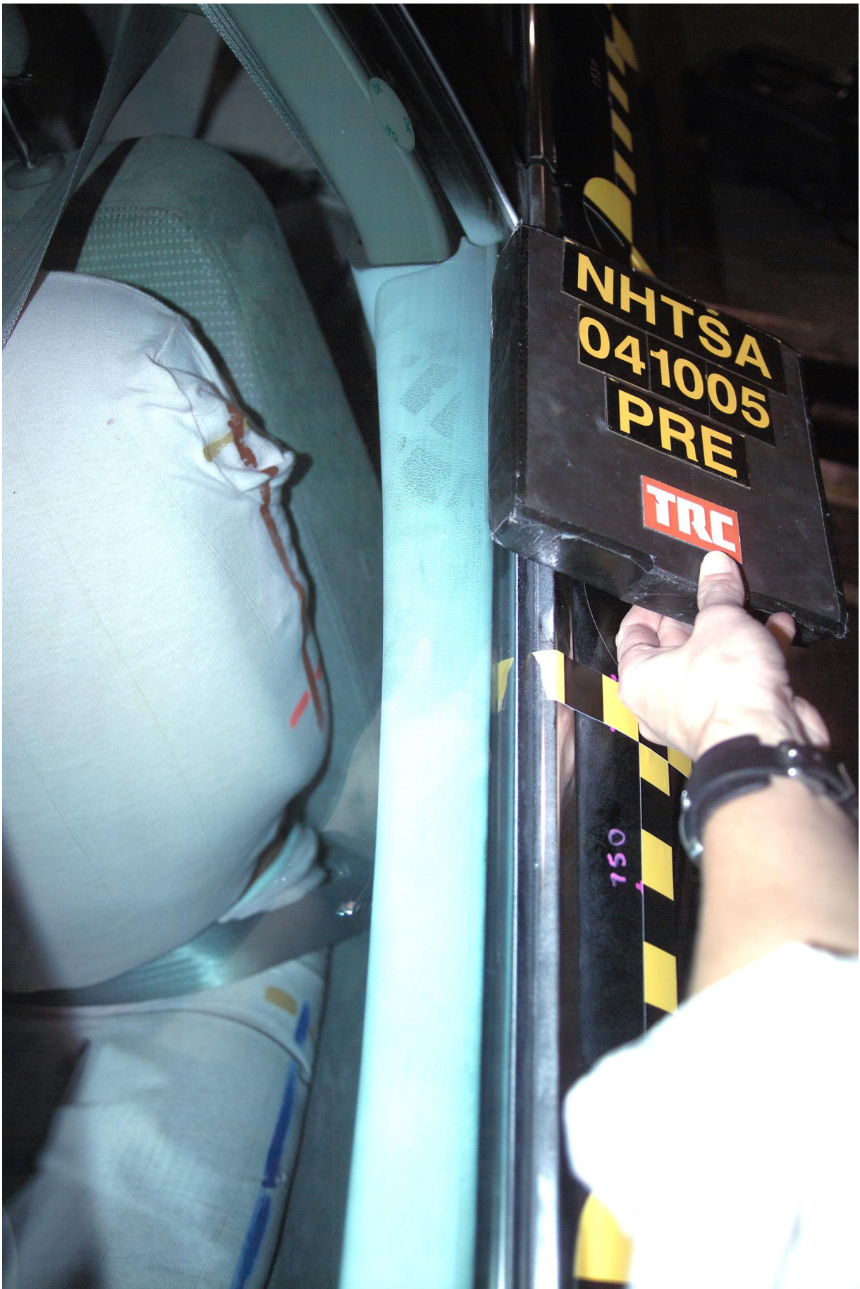
Figure A-28 Pre-Test View of Front SID-HIII and Door Clearance
