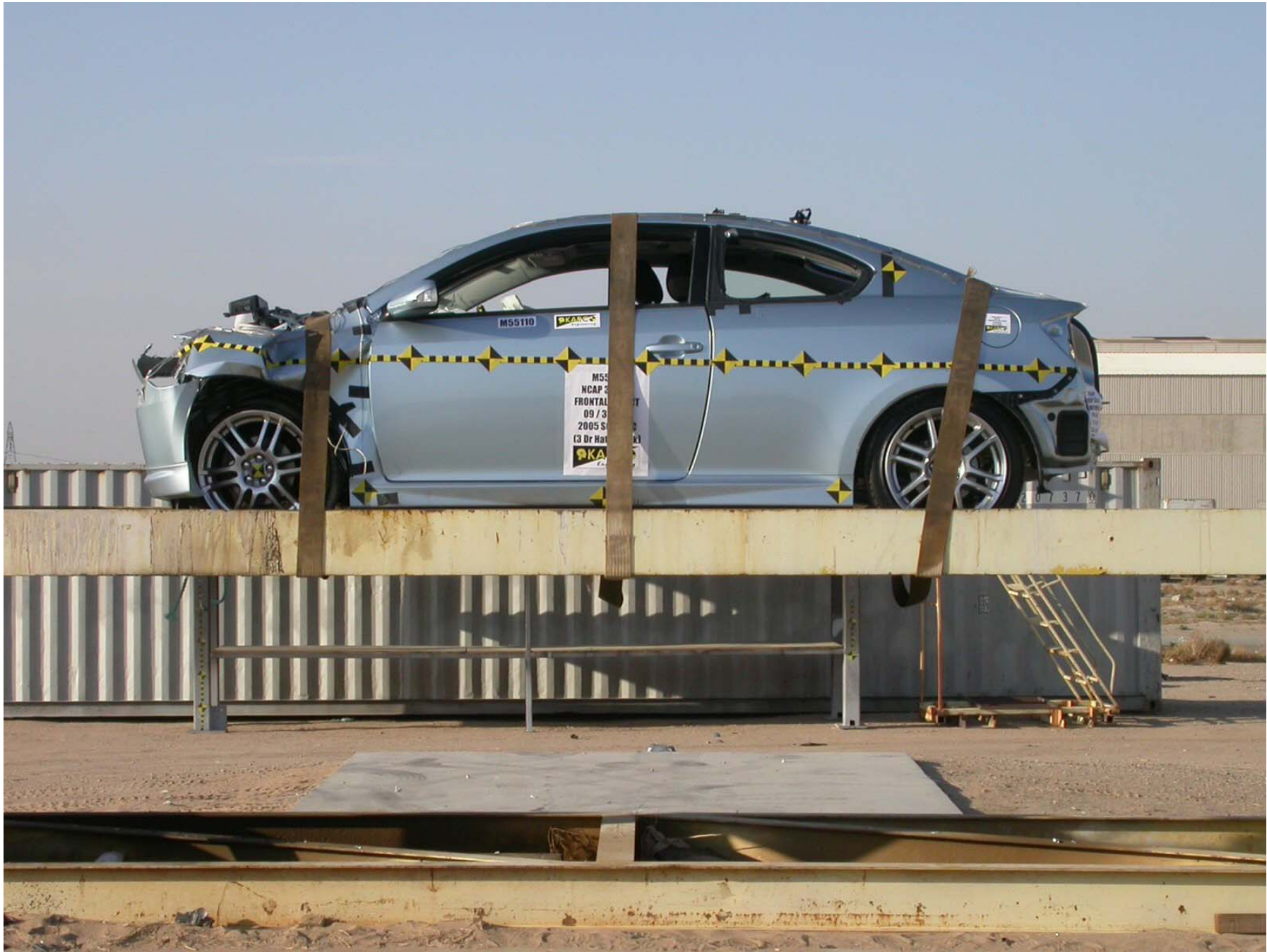
Figure A-58: Vehicle on Rollover Device at 0°
