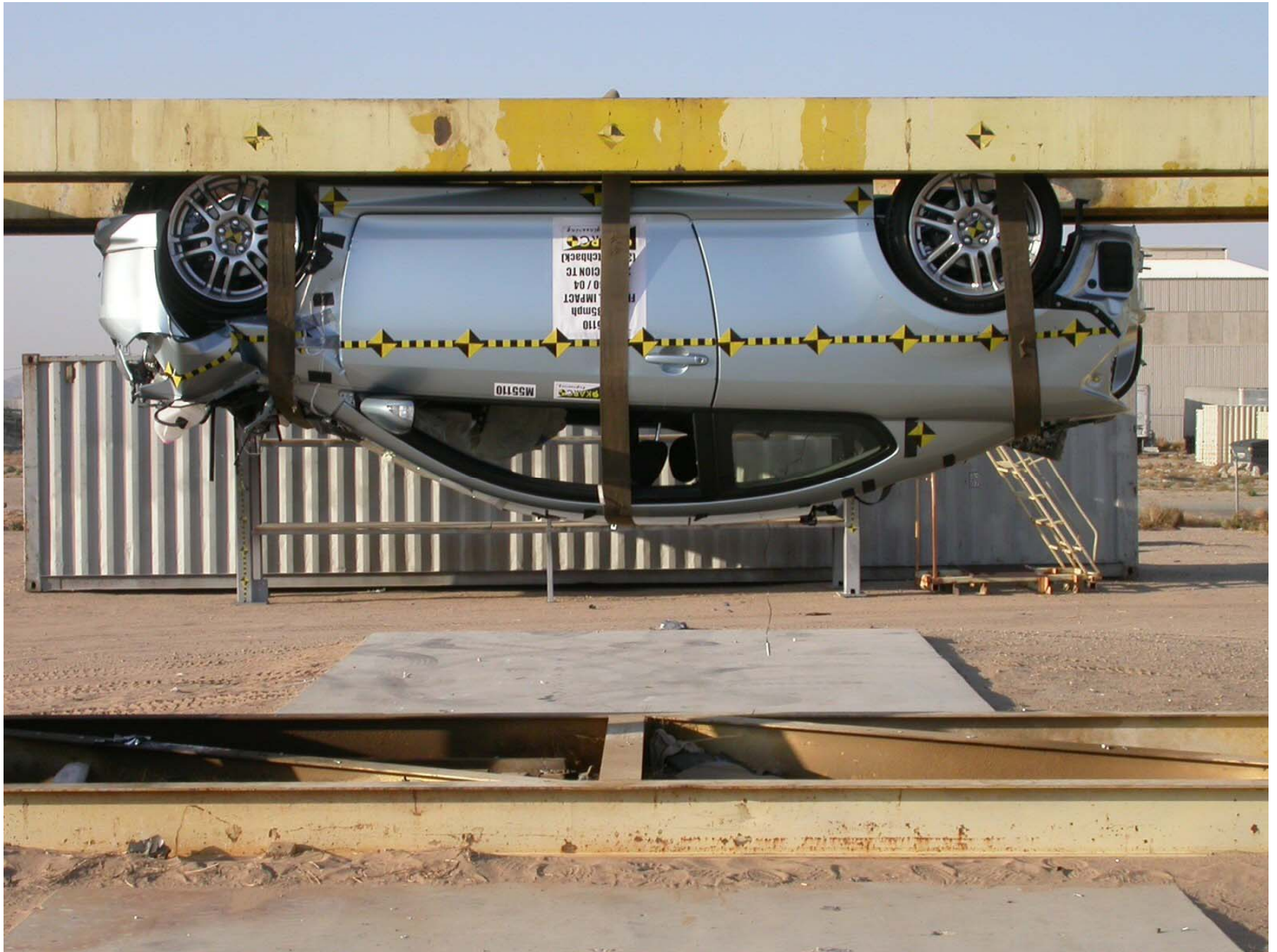
Figure A-60: Vehicle on Rollover Device at 180°
