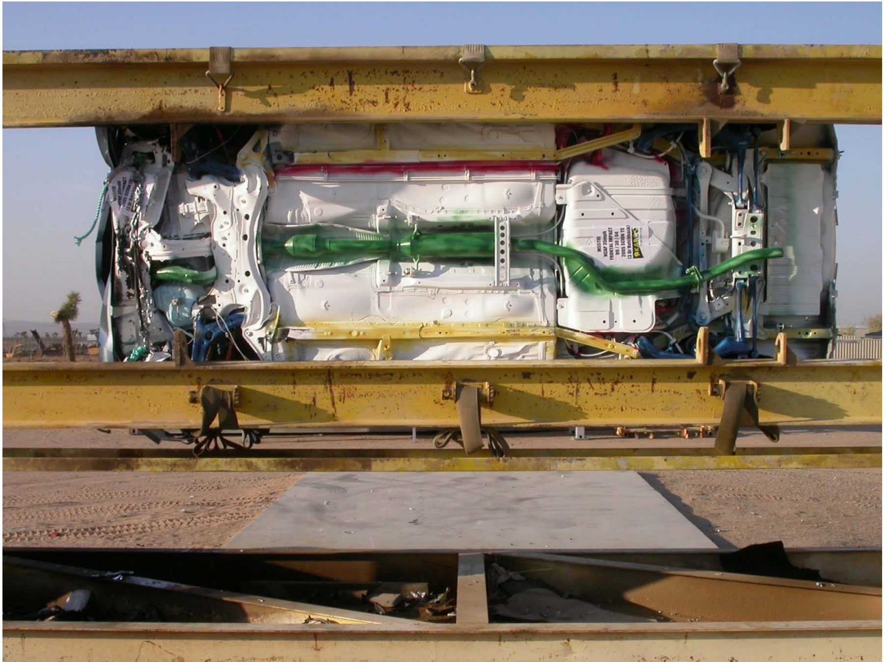
Figure A-61: Vehicle on Rollover Device at 270°
