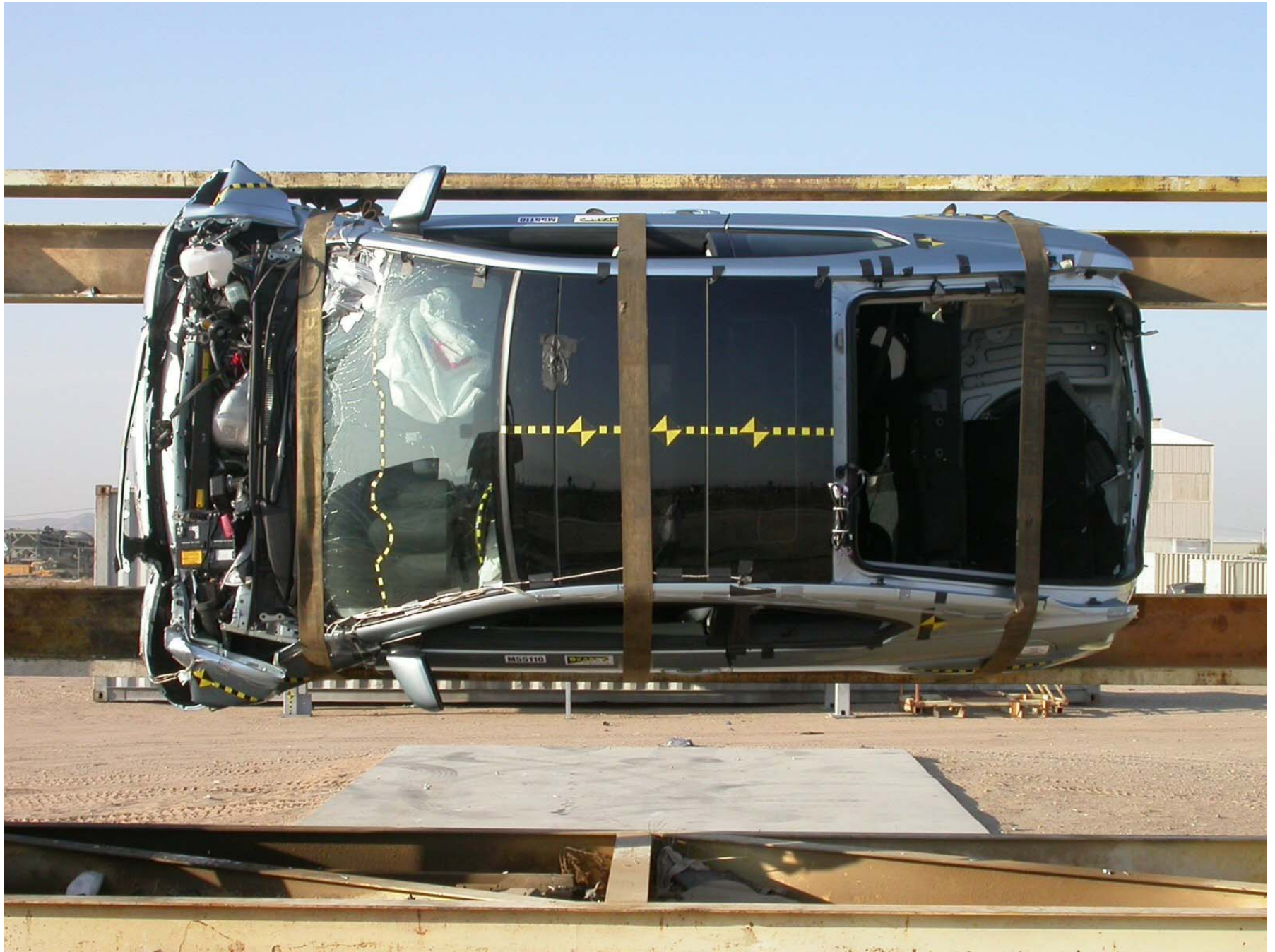
Figure A-59: Vehicle on Rollover Device at 90°
