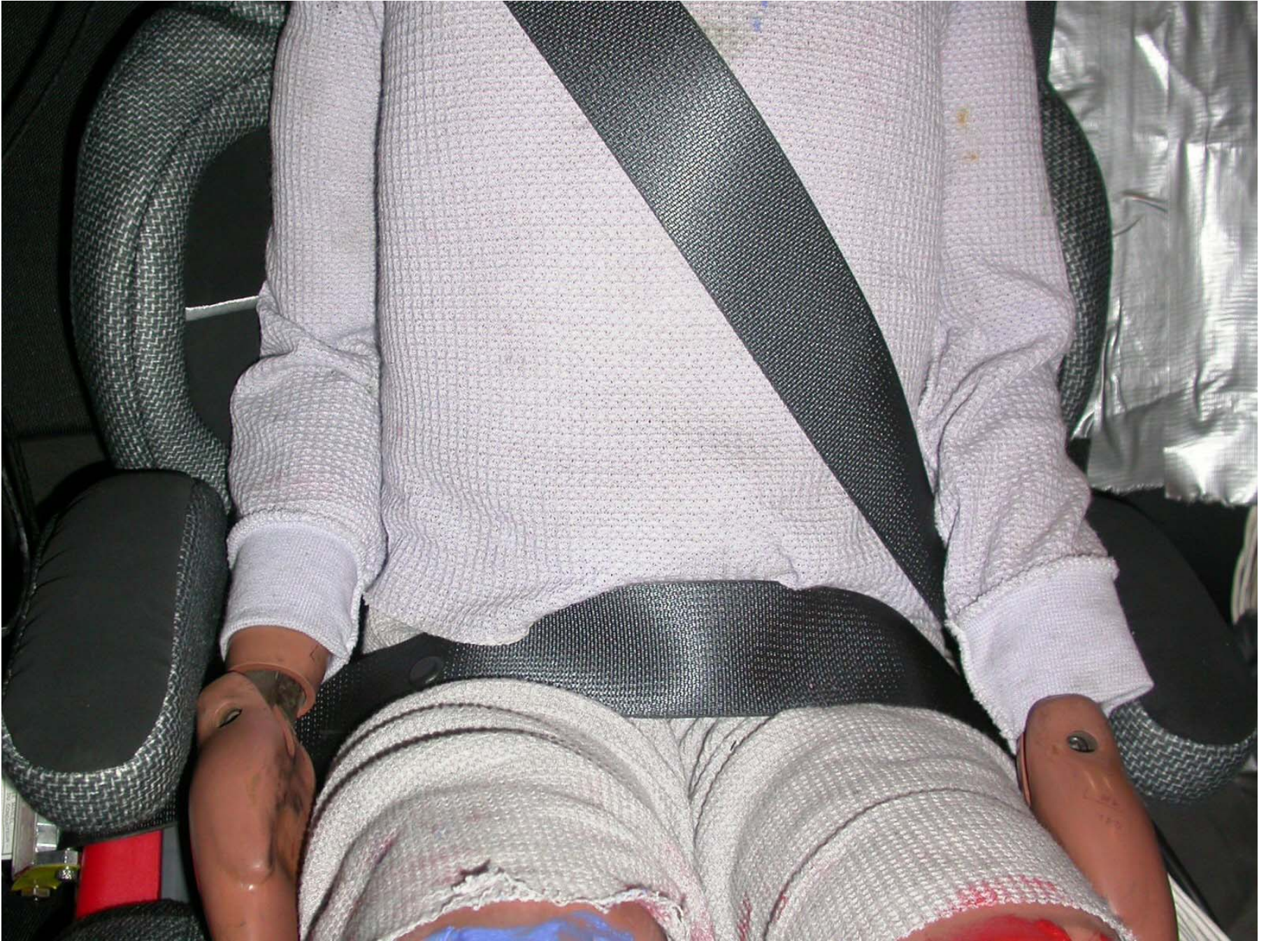
Figure F2-12: Pre-Test Position 3 Front View (Seatbelt Position)
