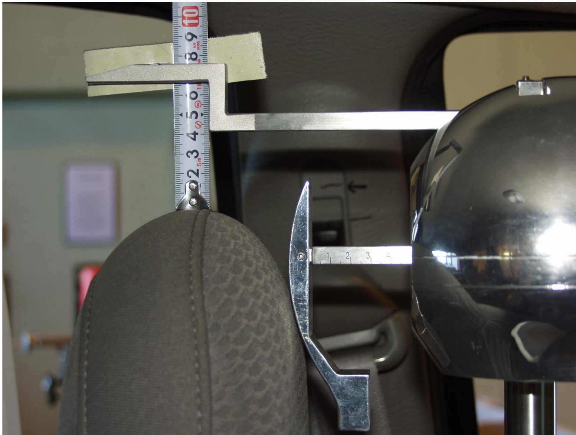
Figure A-1 DRIVER ICBC BACKSET VIEW
