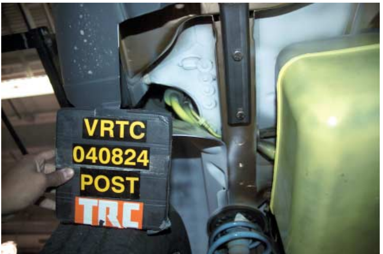
Figure A-29 Post-Test Fuel Filler Neck View
