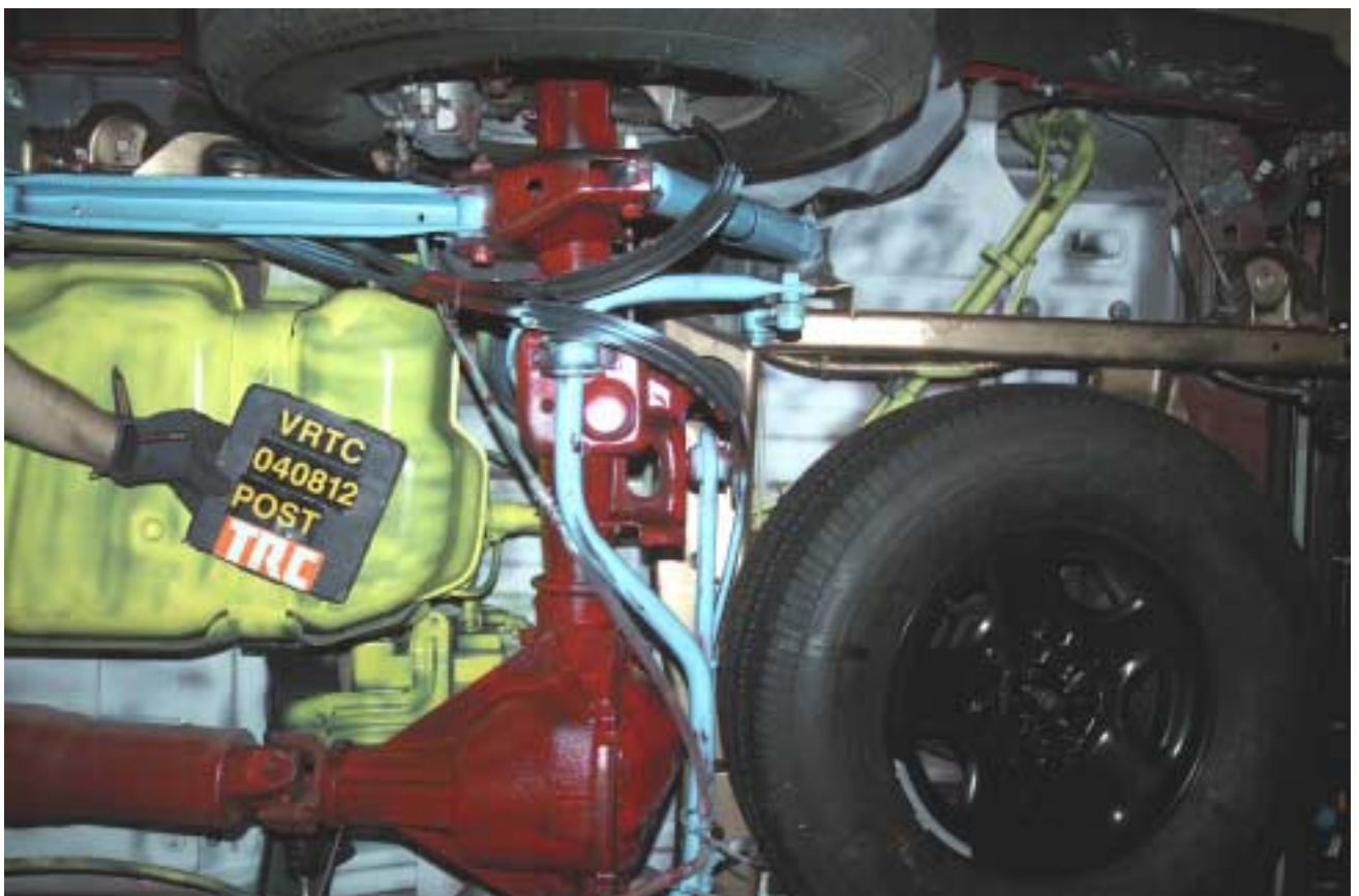
Figure A-27 Post-Test Fuel Filler Neck - View 1
