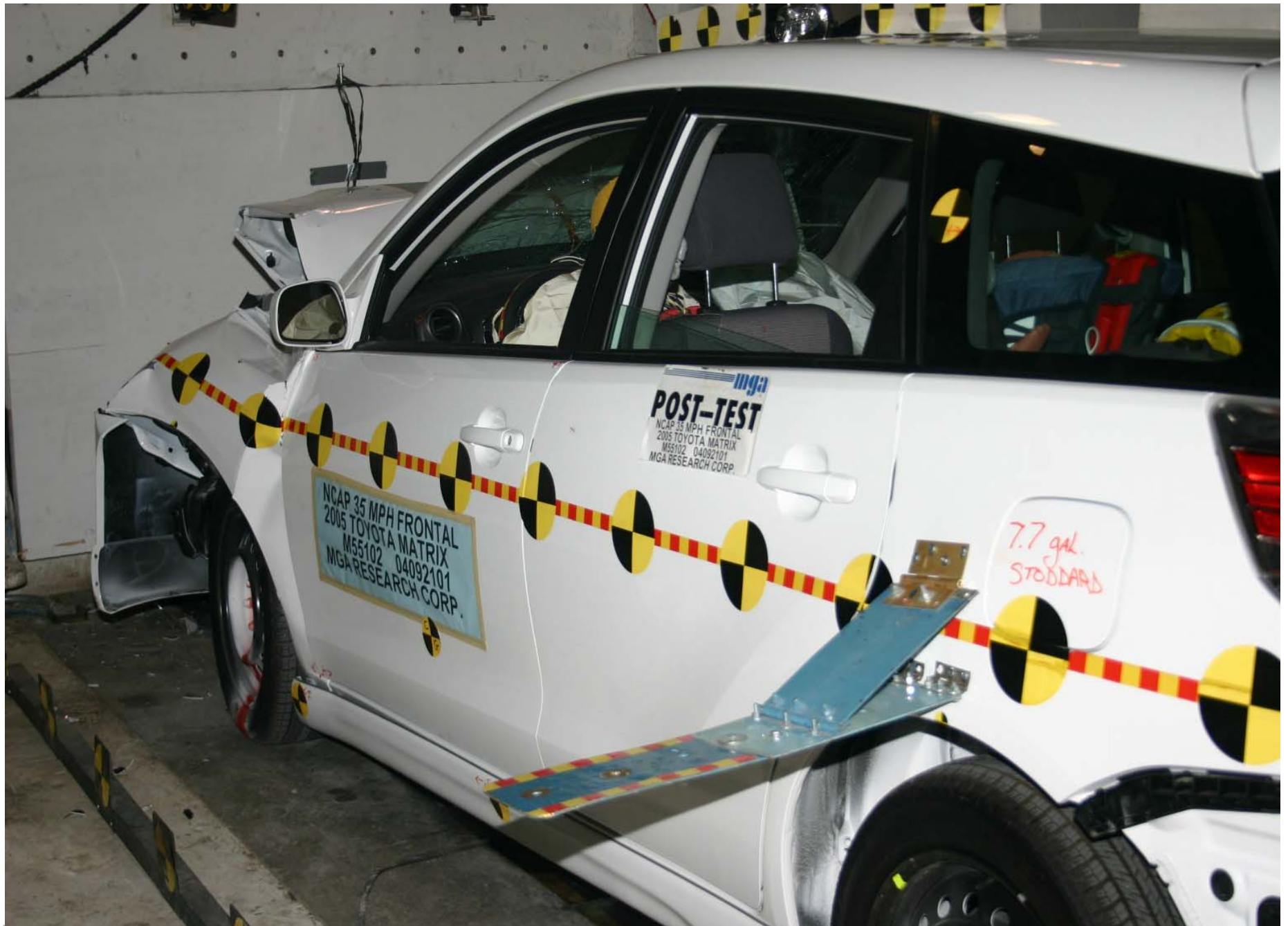
Post-Test Left Side Three-Quarter View of Doors After Impact
