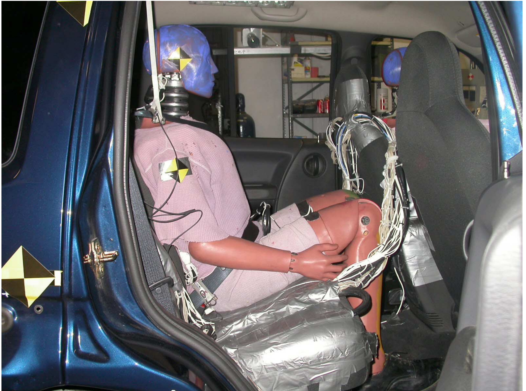
Figure A-98: Pre-Test Center Rear Dummy Door Open (Right Side View)
