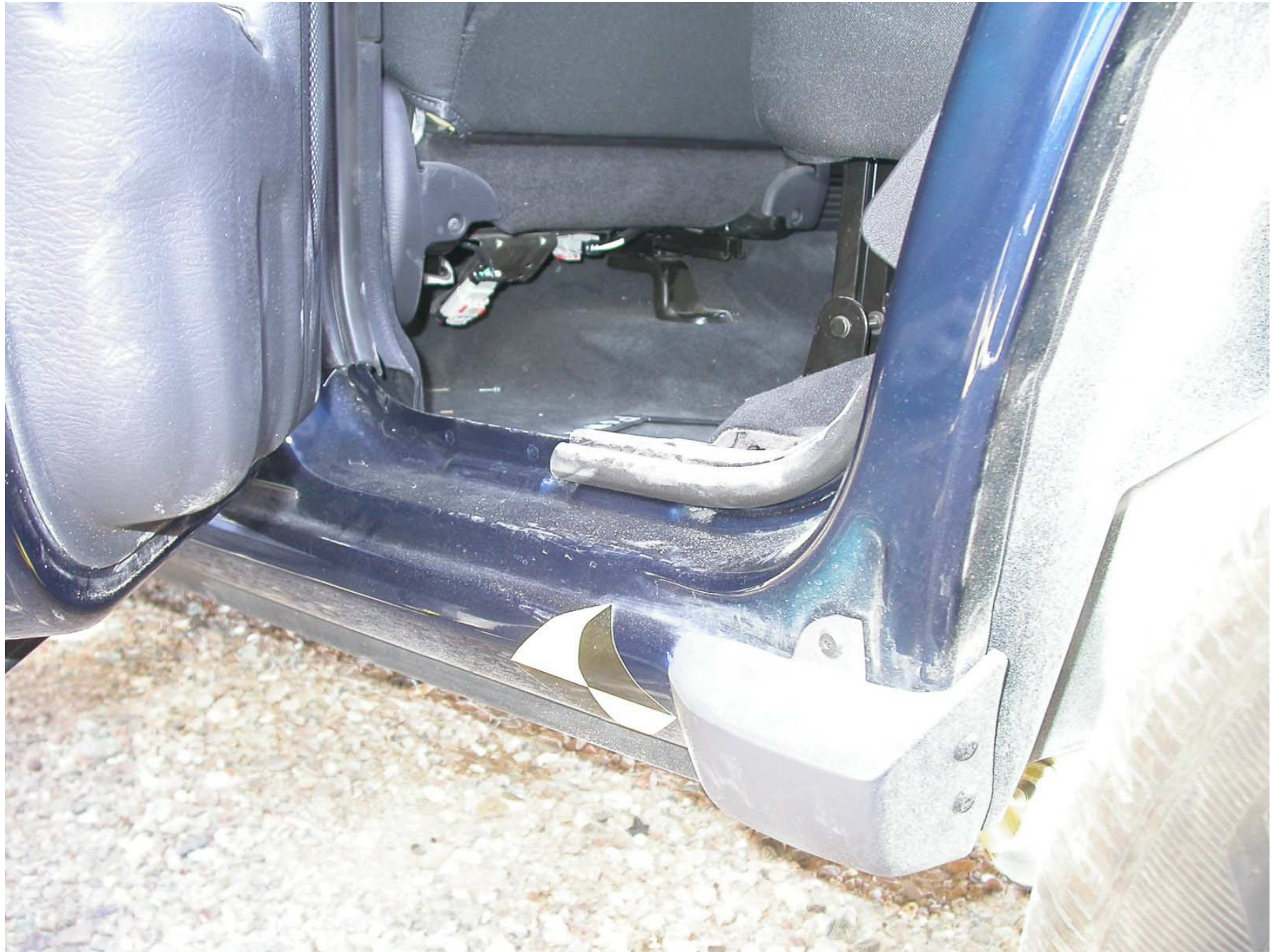
Figure A-22: Post-Test Driver Side Rear Door Sill
