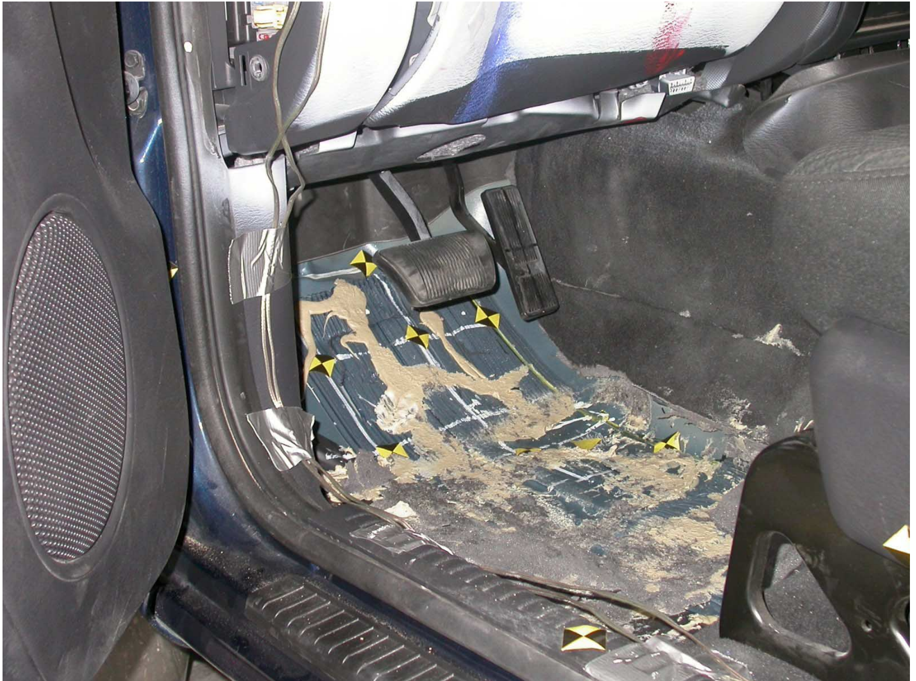
Figure A-69: Post-Test Driver Side Floor Pan
