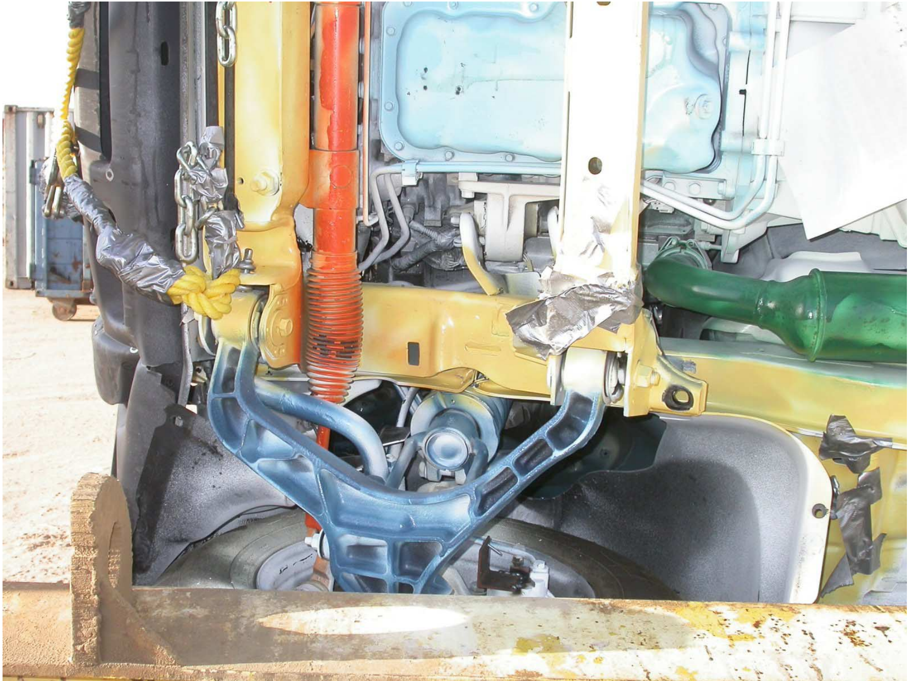
Figure A-53: Right Front Bumper to Rail Attachment (Front of Test Vehicle is to the Left)
