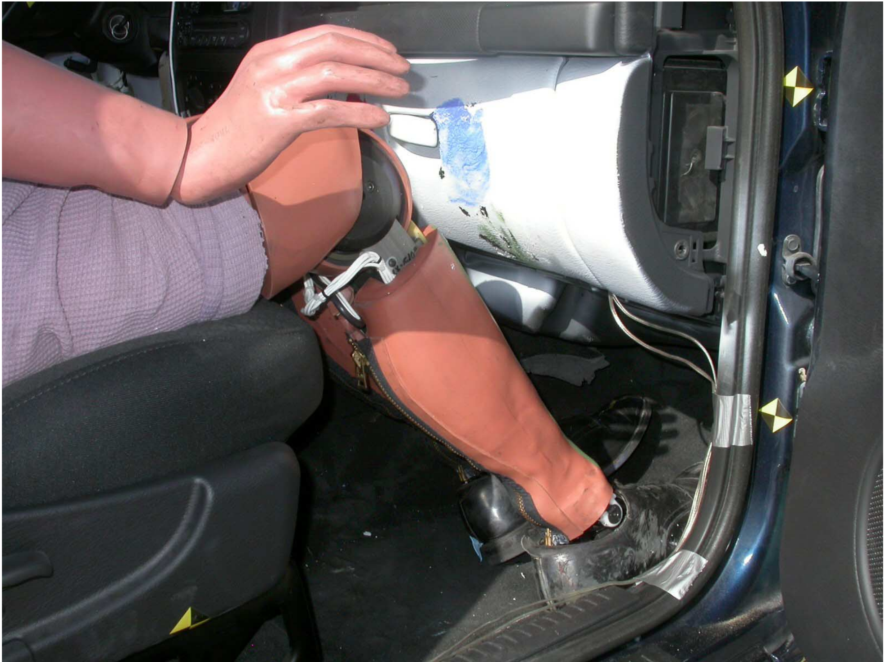
Figure A-82: Post-Test Passenger Dummy Feet
