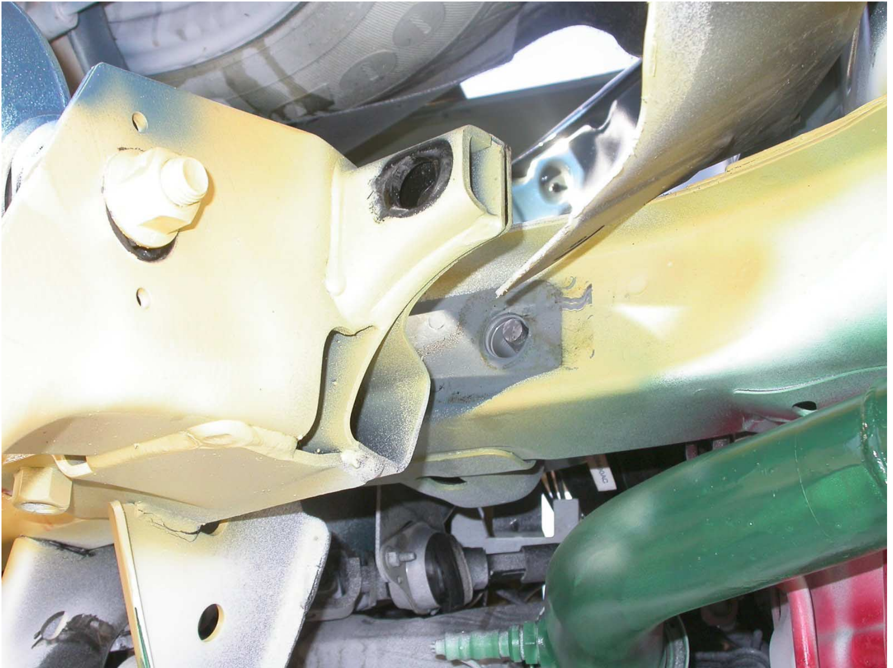
Figure A-47: Post-Test Left Front Sub Frame Mount Damage (Front of Test Vehicle is to the Left)
