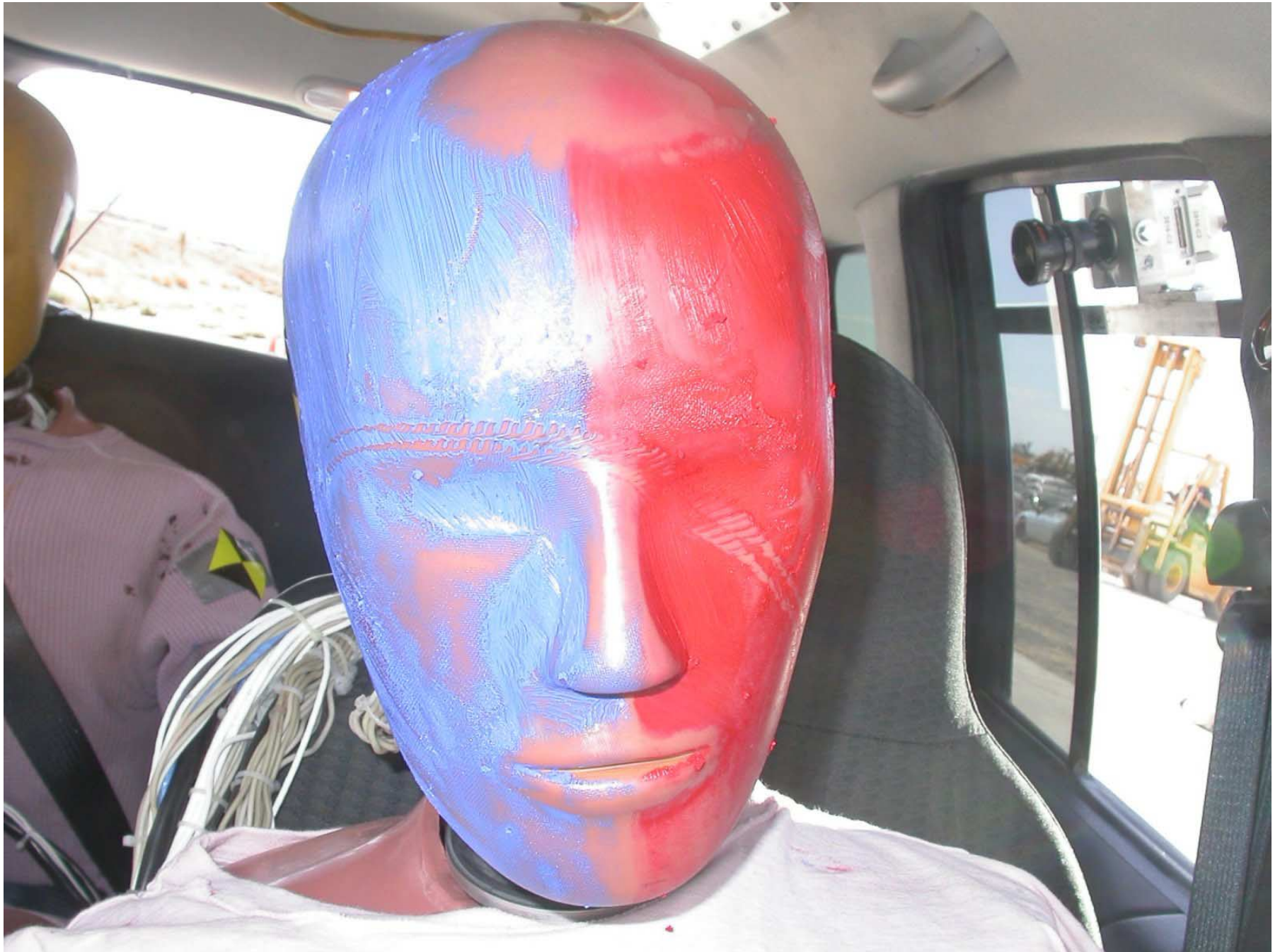
Figure A-72: Post-Test Driver Dummy Head
