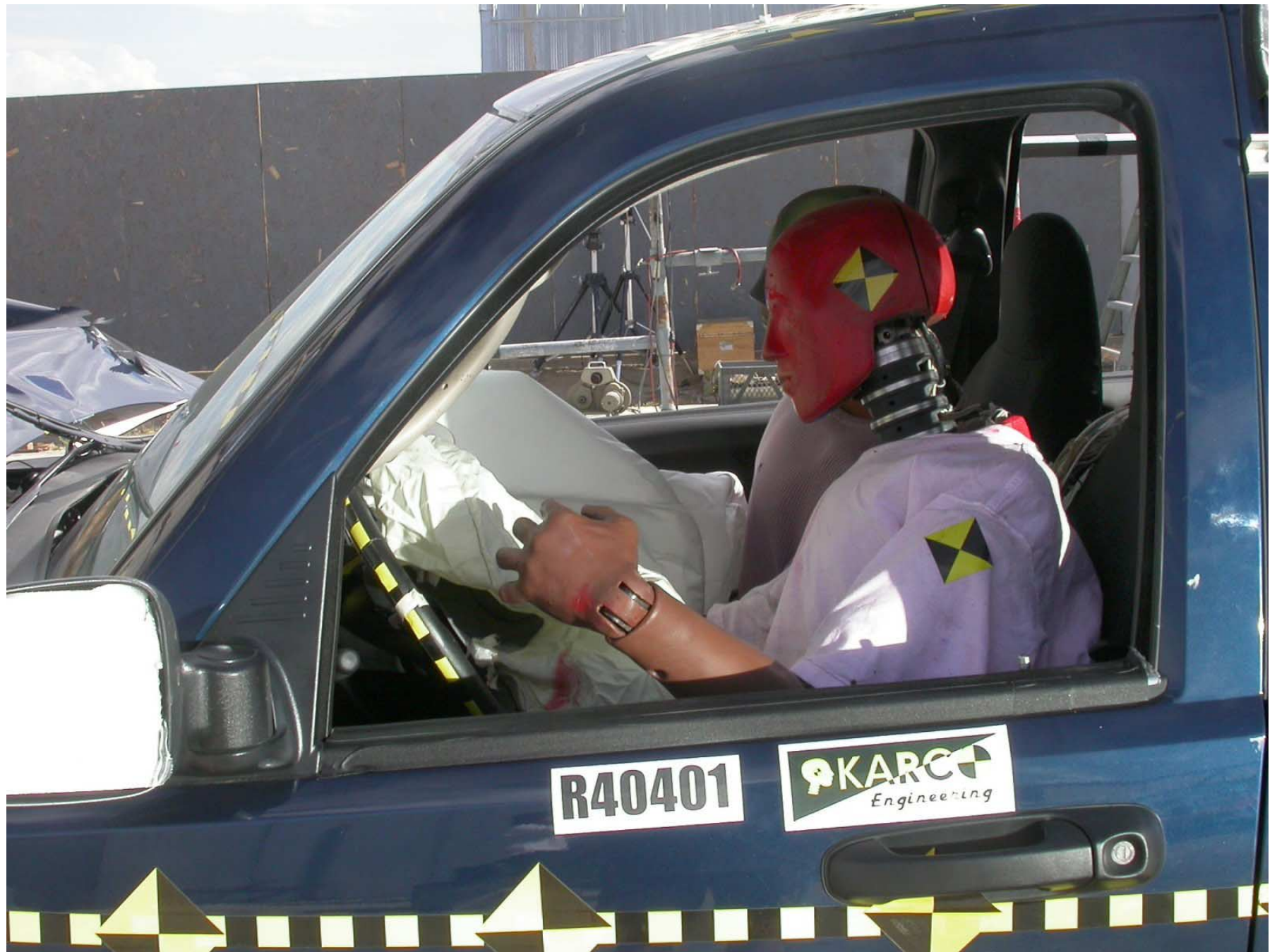
Figure A-59: Post-Test Driver Dummy Through Window
