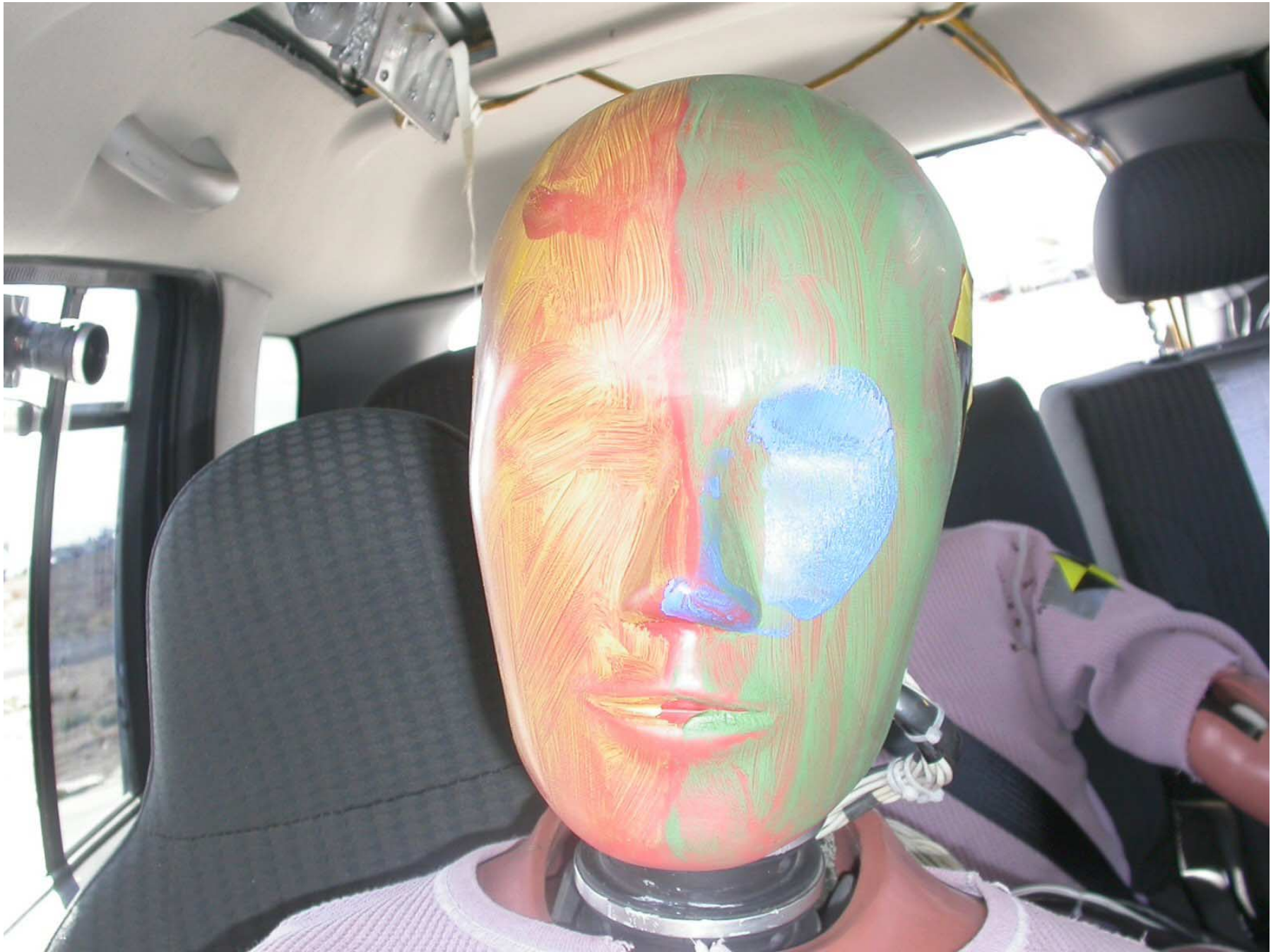
Figure A-89: Post-Test Passenger Dummy Head
