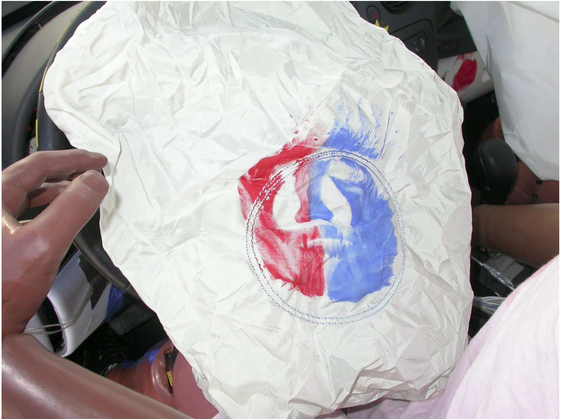
Figure A-73: Post-Test Driver Dummy Contact to Air Bag
