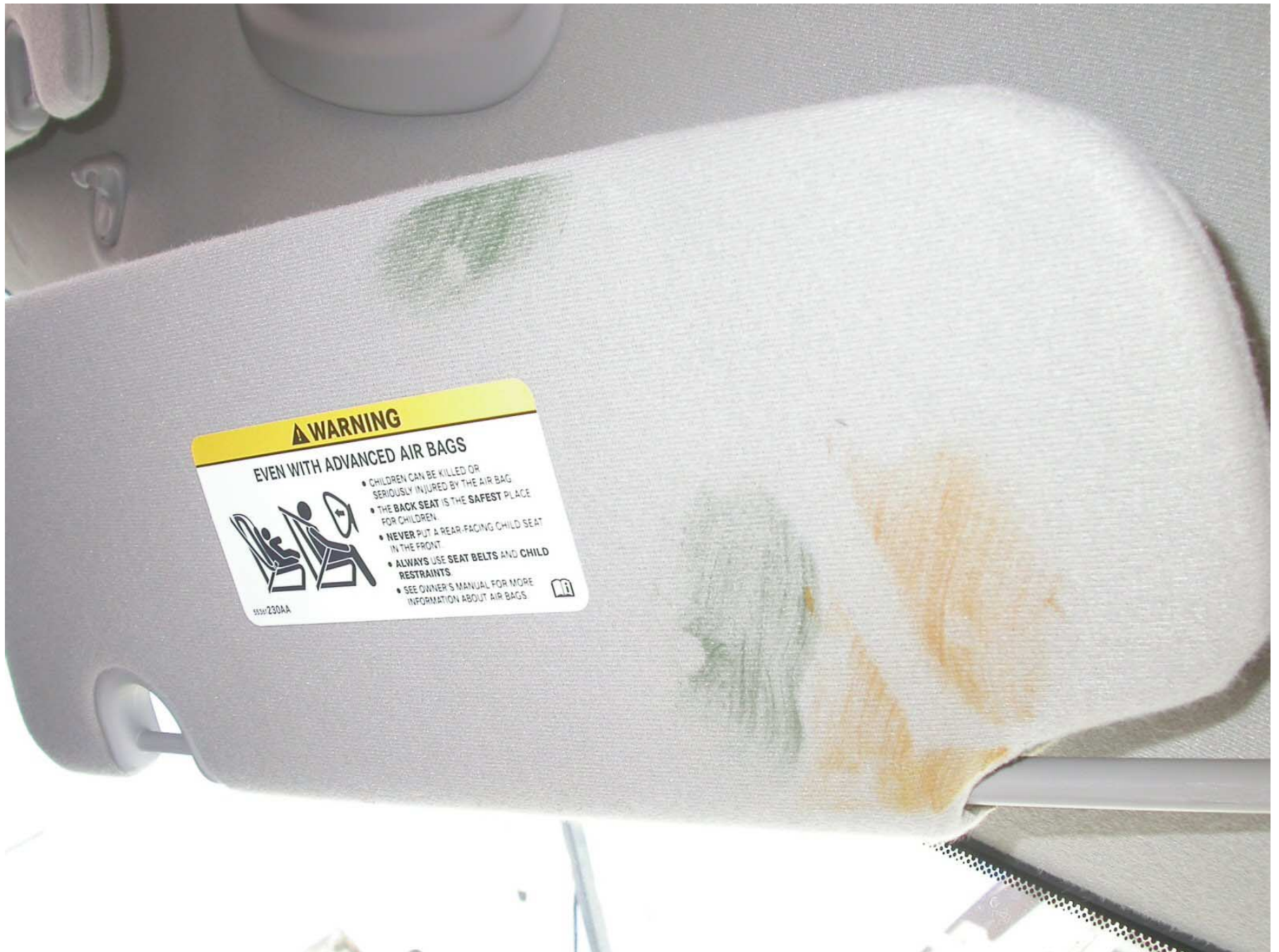
Figure A-91: Post-Test Passenger Dummy Contact With Sun-Visor
