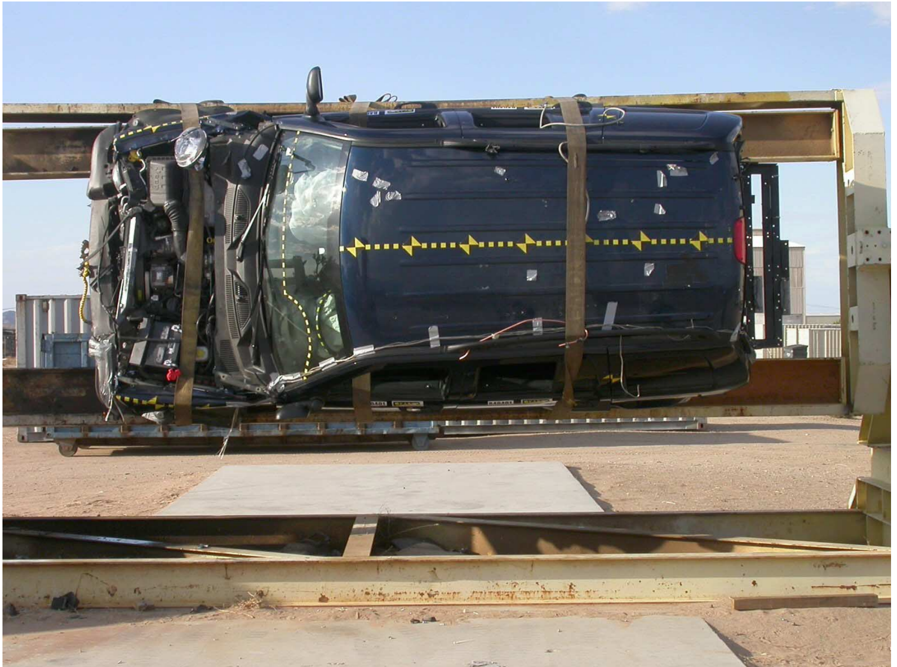
Figure A-106: Vehicle on Rollover Device (90°)
