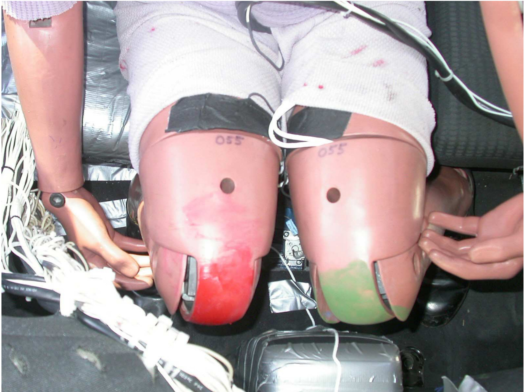
Figure A-103: Post-Test Center Rear Dummy Knees (Overhead View)
