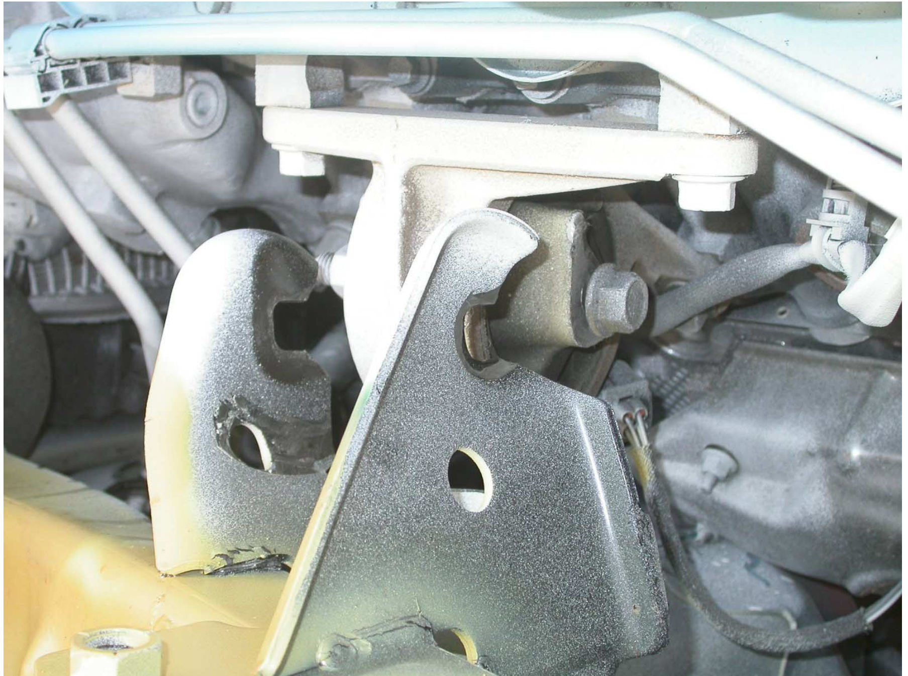
Figure A-55: Post-Test Right Front Right Sub Frame Mount Damage (Front of Test Vehicle is to the Left)
