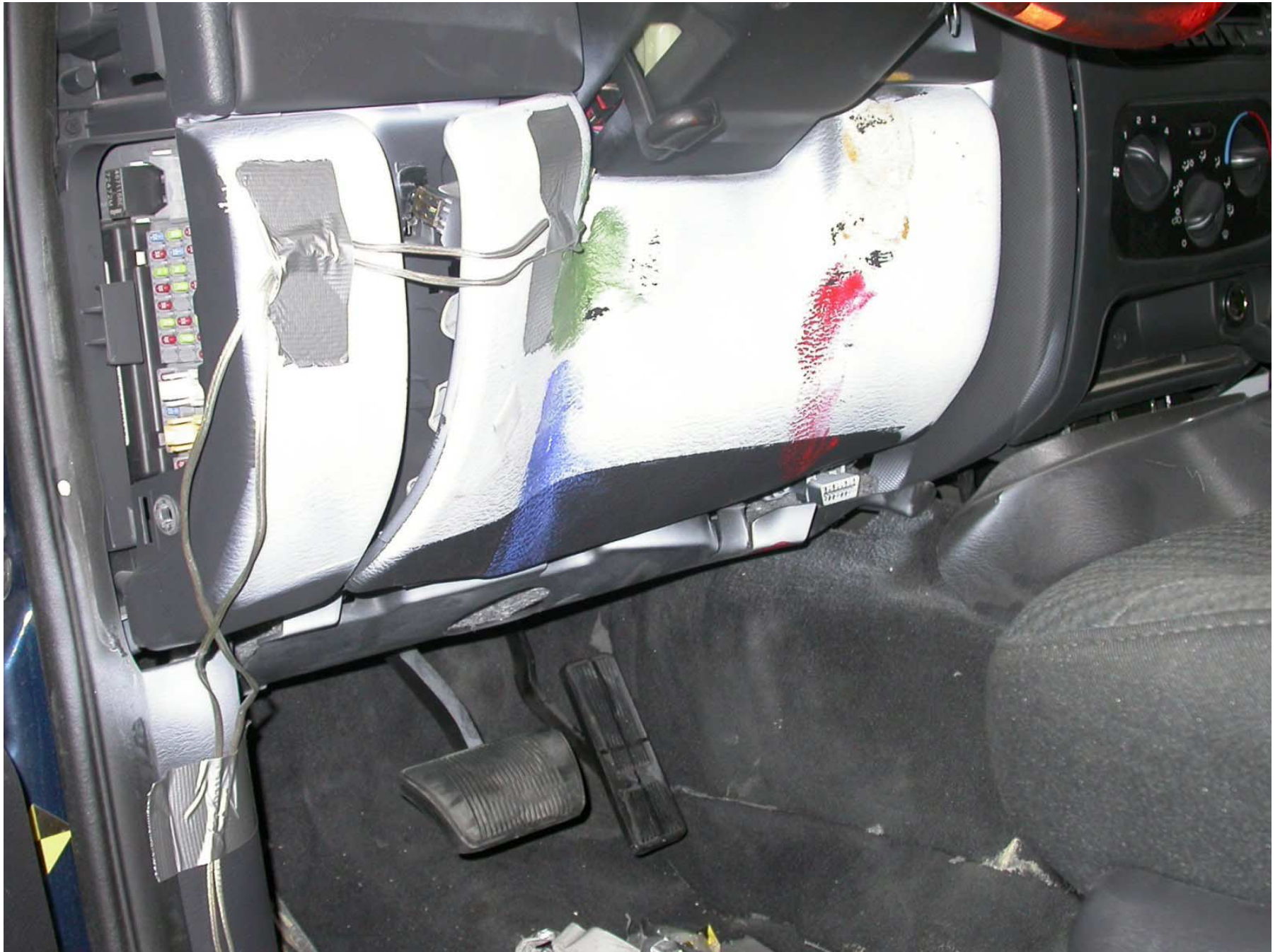
Figure A-67: Post-Test Driver Side Knee Bolster
