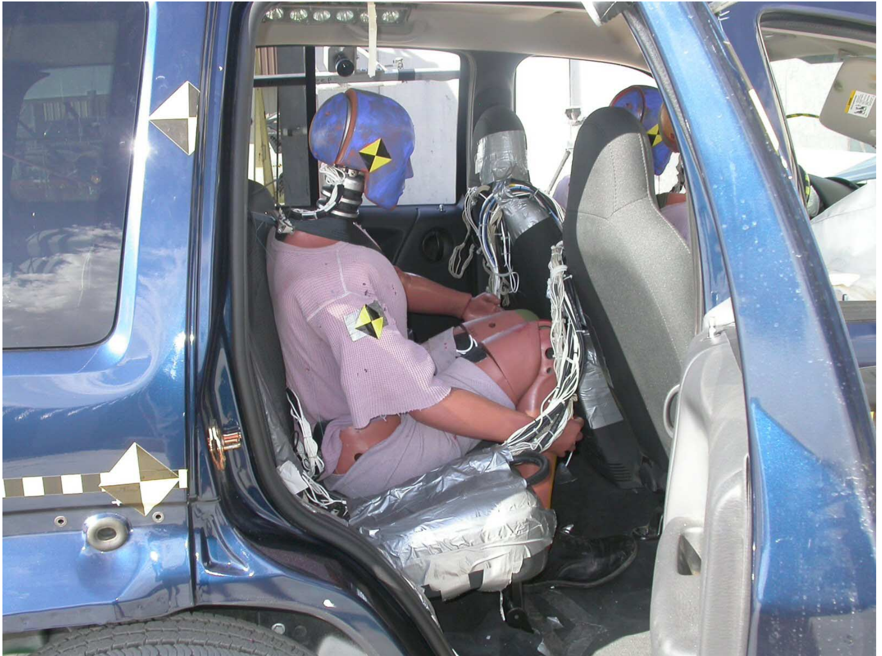
Figure A-99: Post-Test Center Rear Dummy Door Open (Right Side View)
