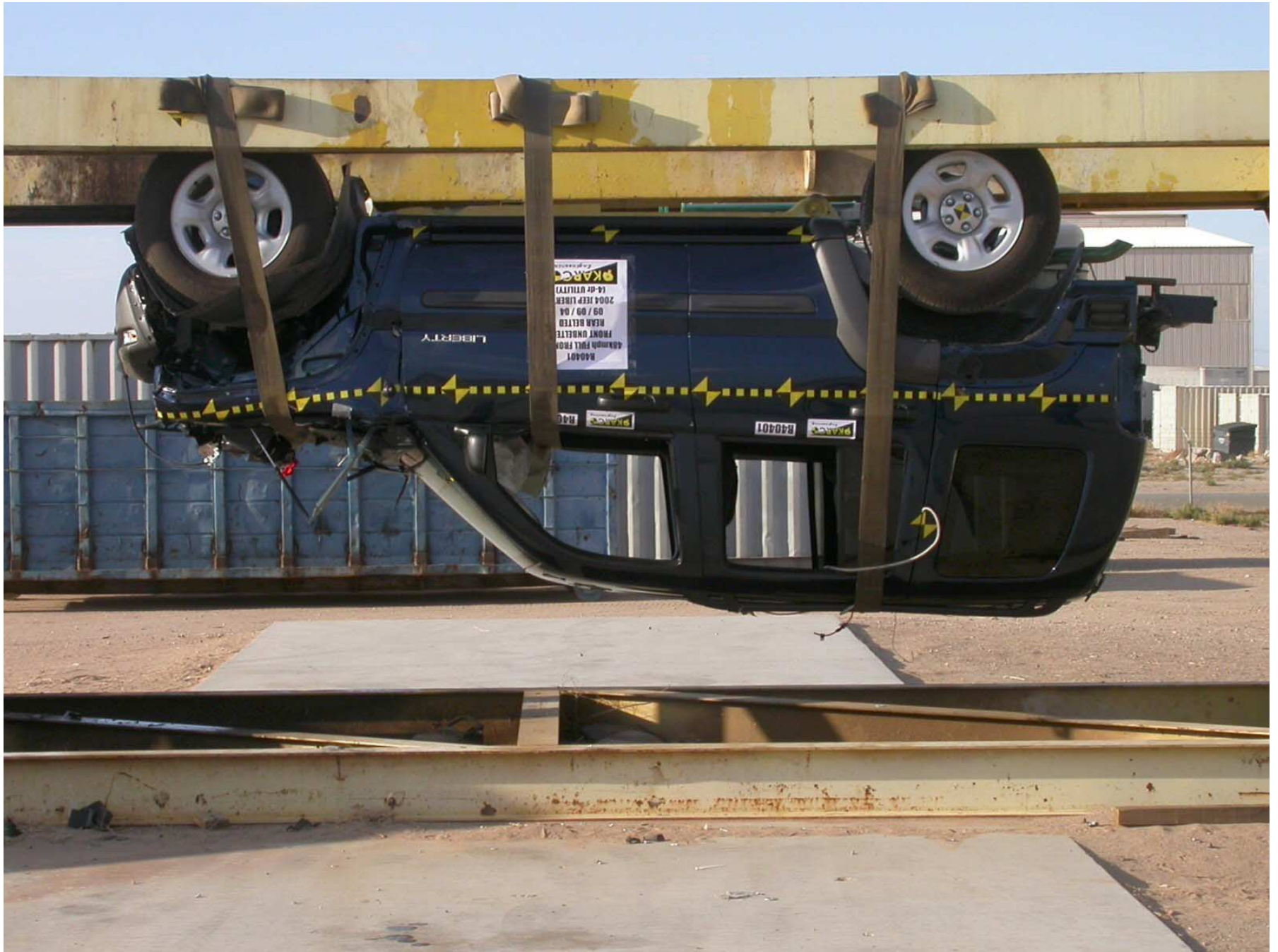
Figure A-107: Vehicle on Rollover Device (180°)
