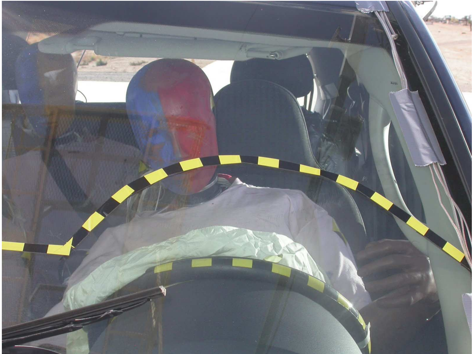
Figure A-57: Post-Test Driver Dummy Front View (Head Position)
