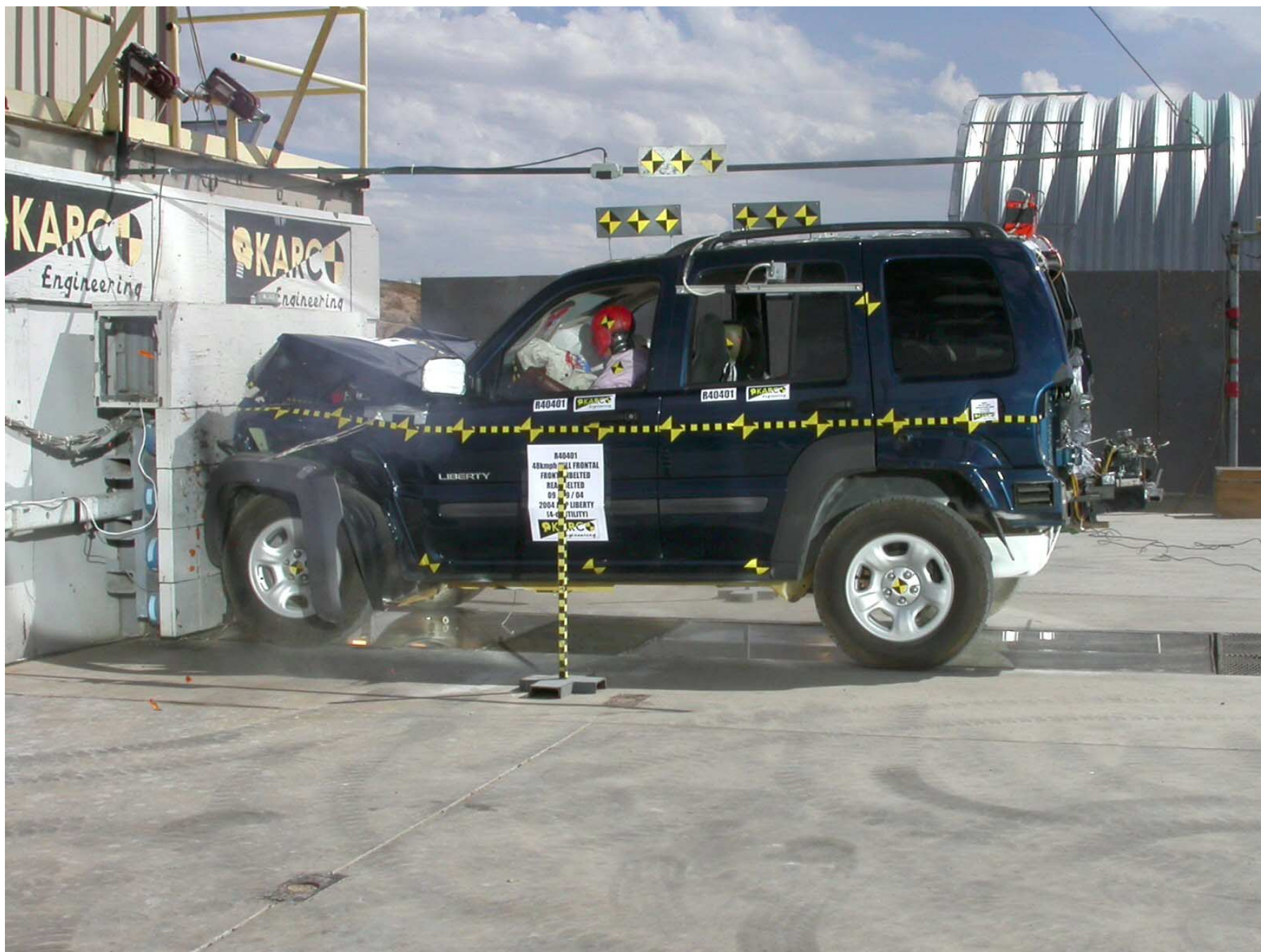
Figure A-109: Vehicle During Impact
