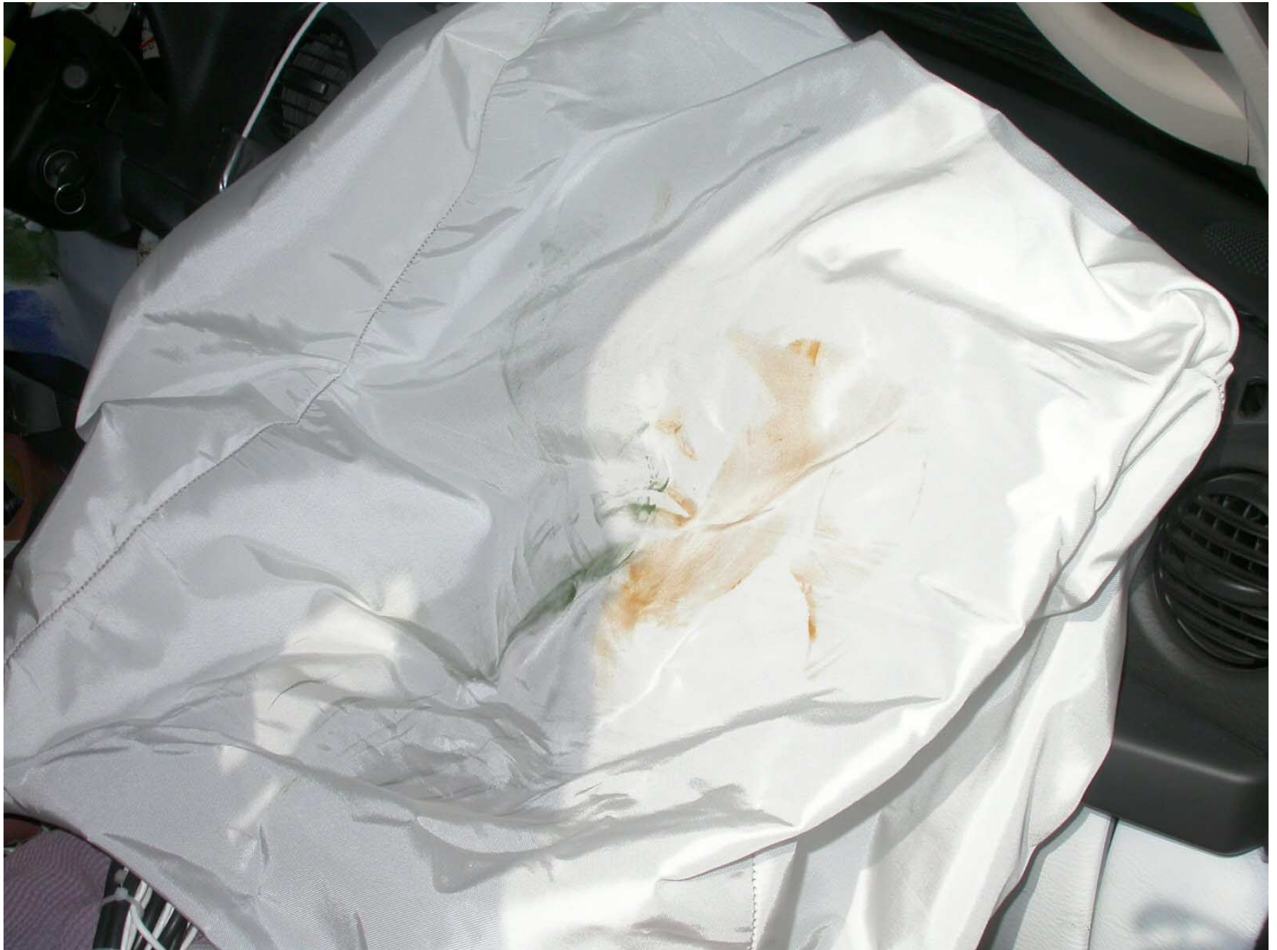
Figure A-90: Post-Test Passenger Dummy Contact to Air Bag
