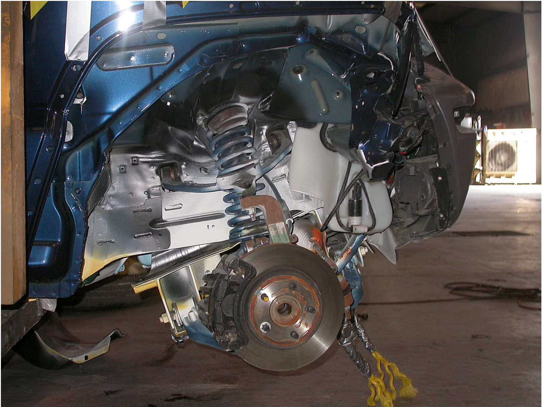
Figure A-50: Post-Test Right Front Wheel Well with Tire and Wheel Removed (Front of Test Vehicle is to the Right)
