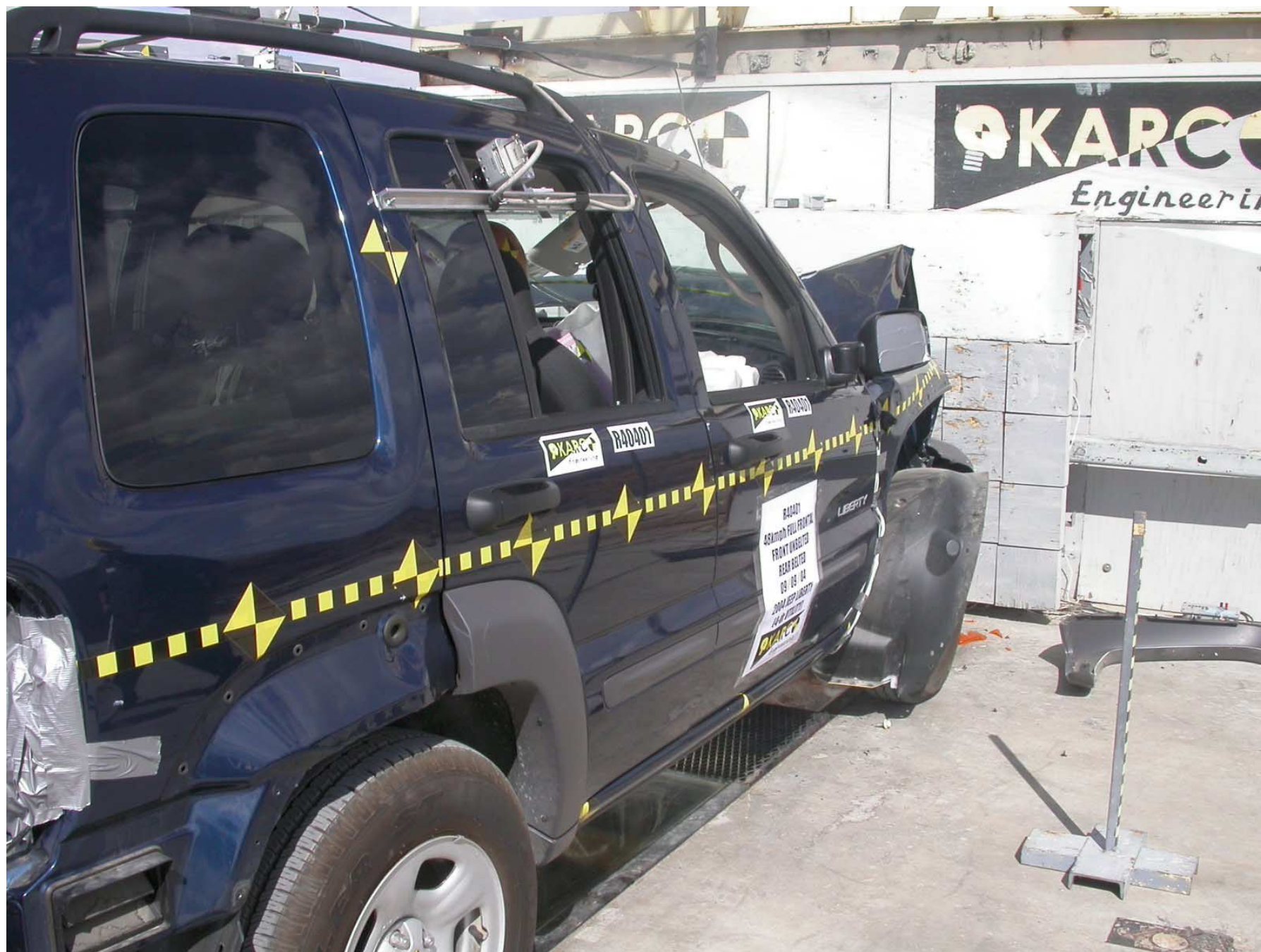
Figure A-23: Post-Test Right Rear \frac{3}{4} View of Doors After Impact
