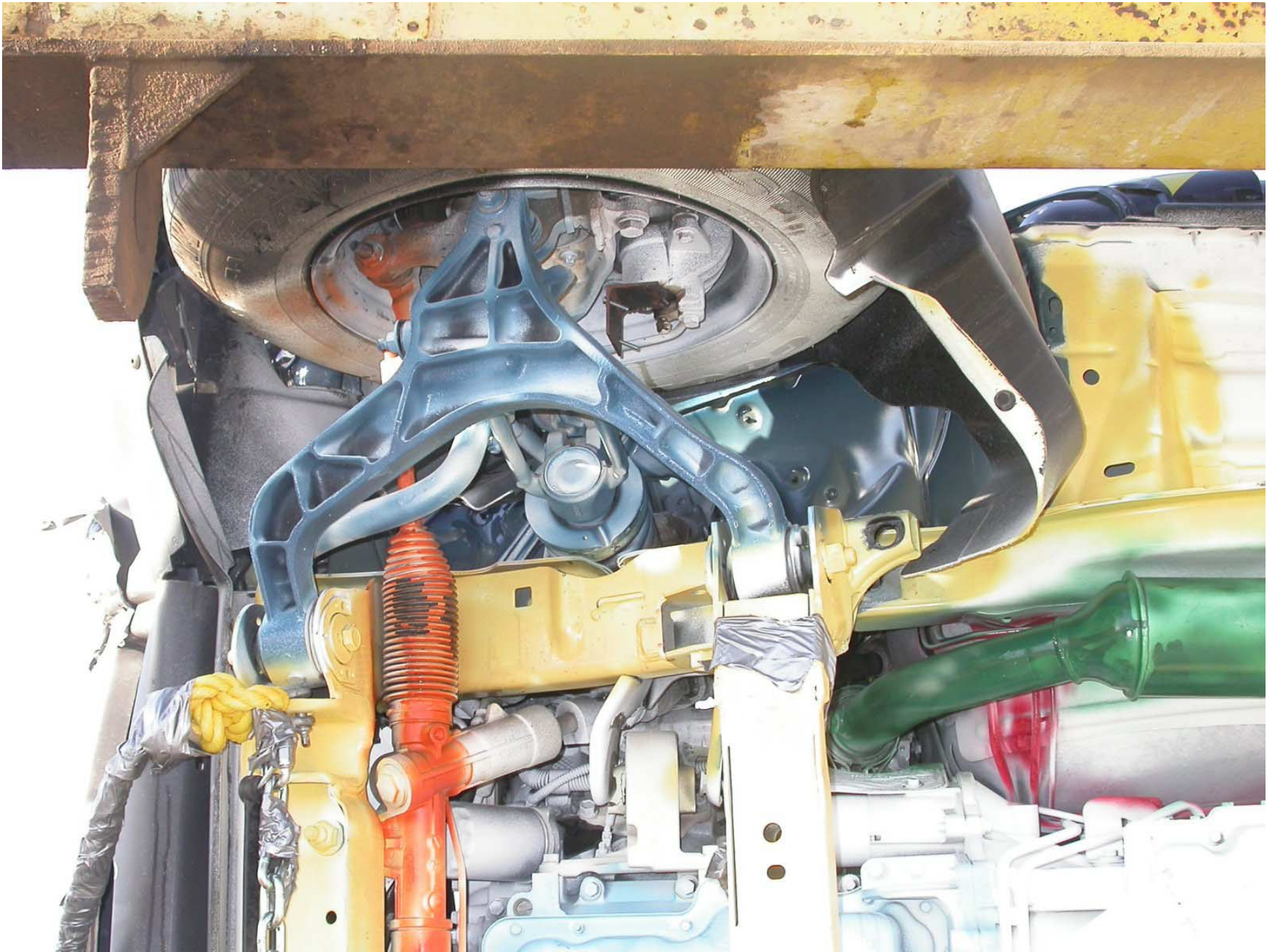
Figure A-46: Post-Test Left Front Bumper to Rail Attachment (Front of Test Vehicle is to the Left)
