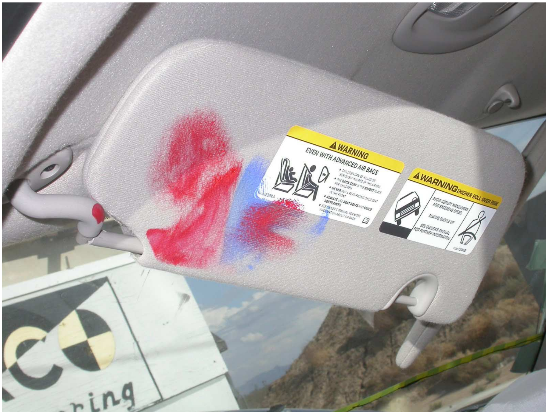
Figure A-74: Post-Test Driver Dummy Contact With Sun-Visor
