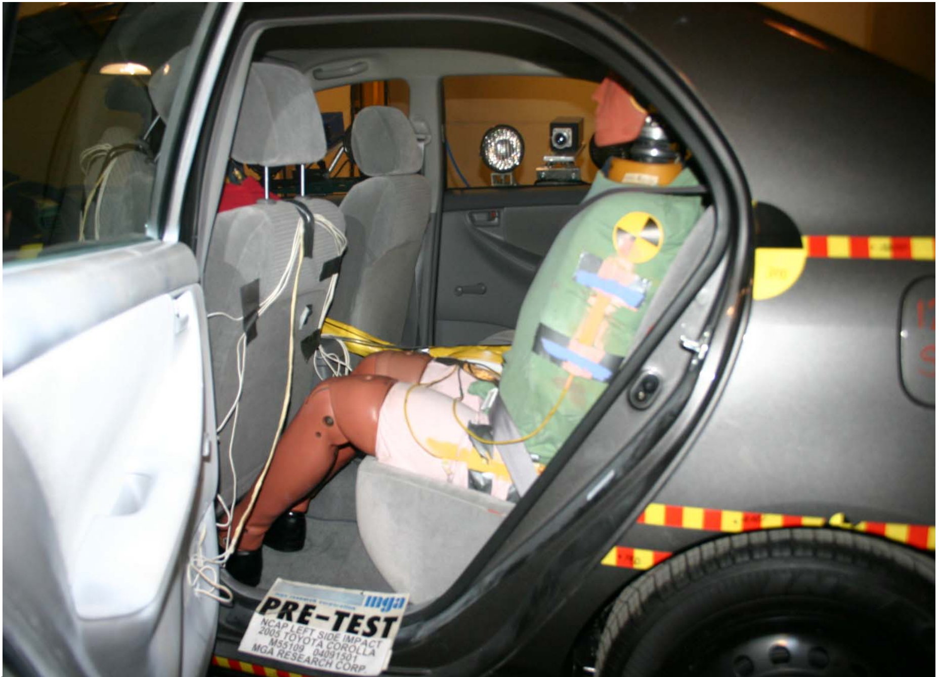
Pre-Test Passenger Dummy Left Side View (Door Open)
