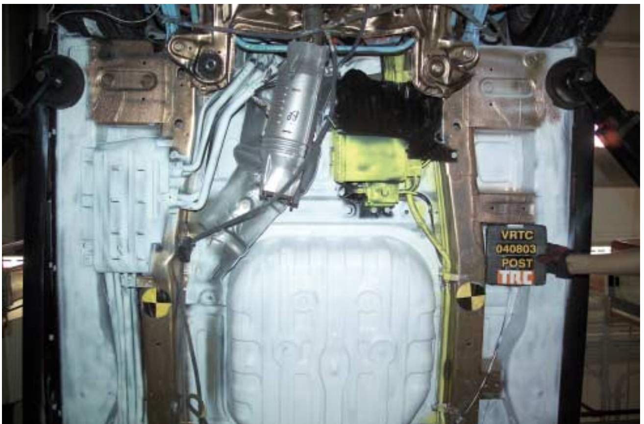
Figure A-17 Post-Test Front Mid Underbody View
