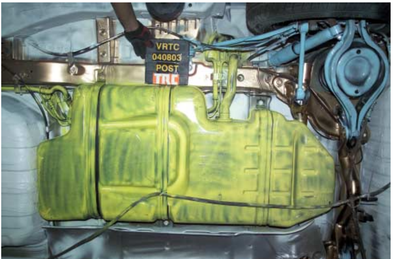
Figure A-25 Post-Test Fuel Tank View
