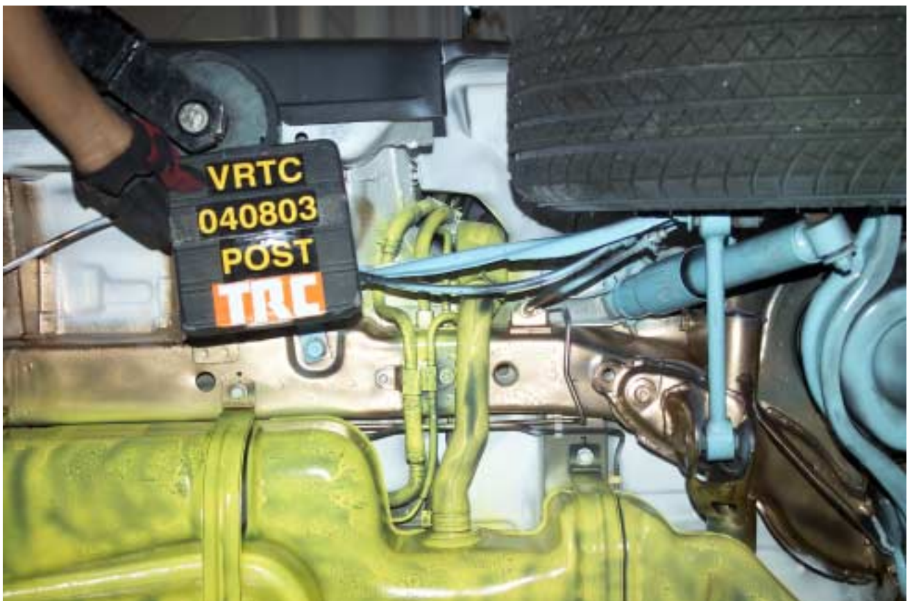
Figure A-27 Post-Test Fuel Filler Neck View
