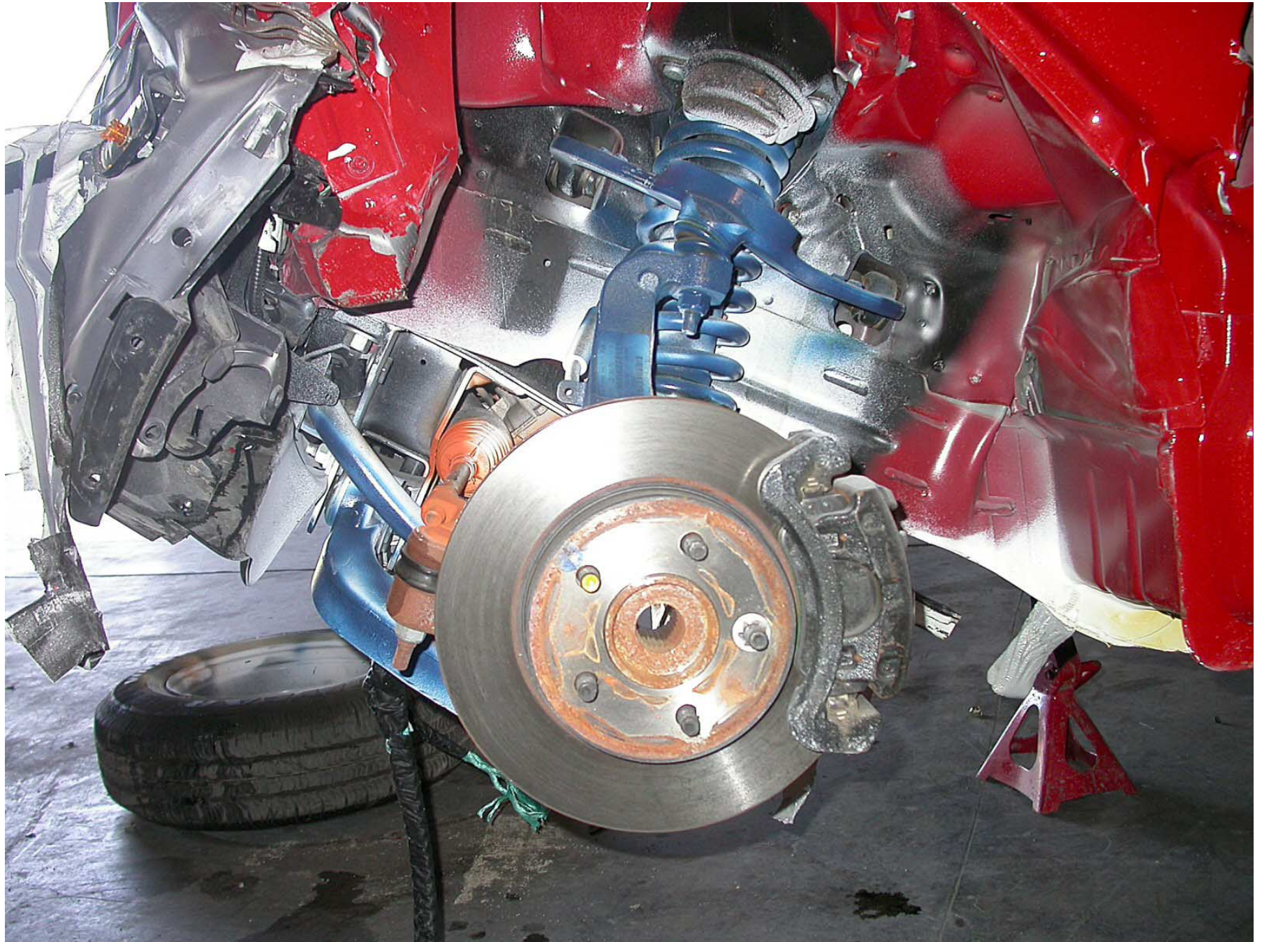
Figure A-43: Post-Test Left Front Wheel Well with Tire and Wheel Removed (Front of Test Vehicle is to the Left)
