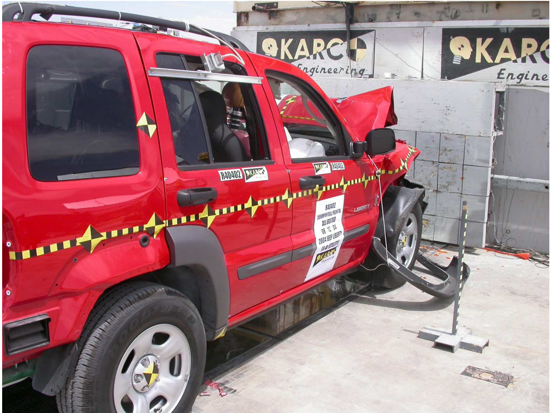
Figure A-23: Post-Test Right Rear ¾ View of Doors After Impact
