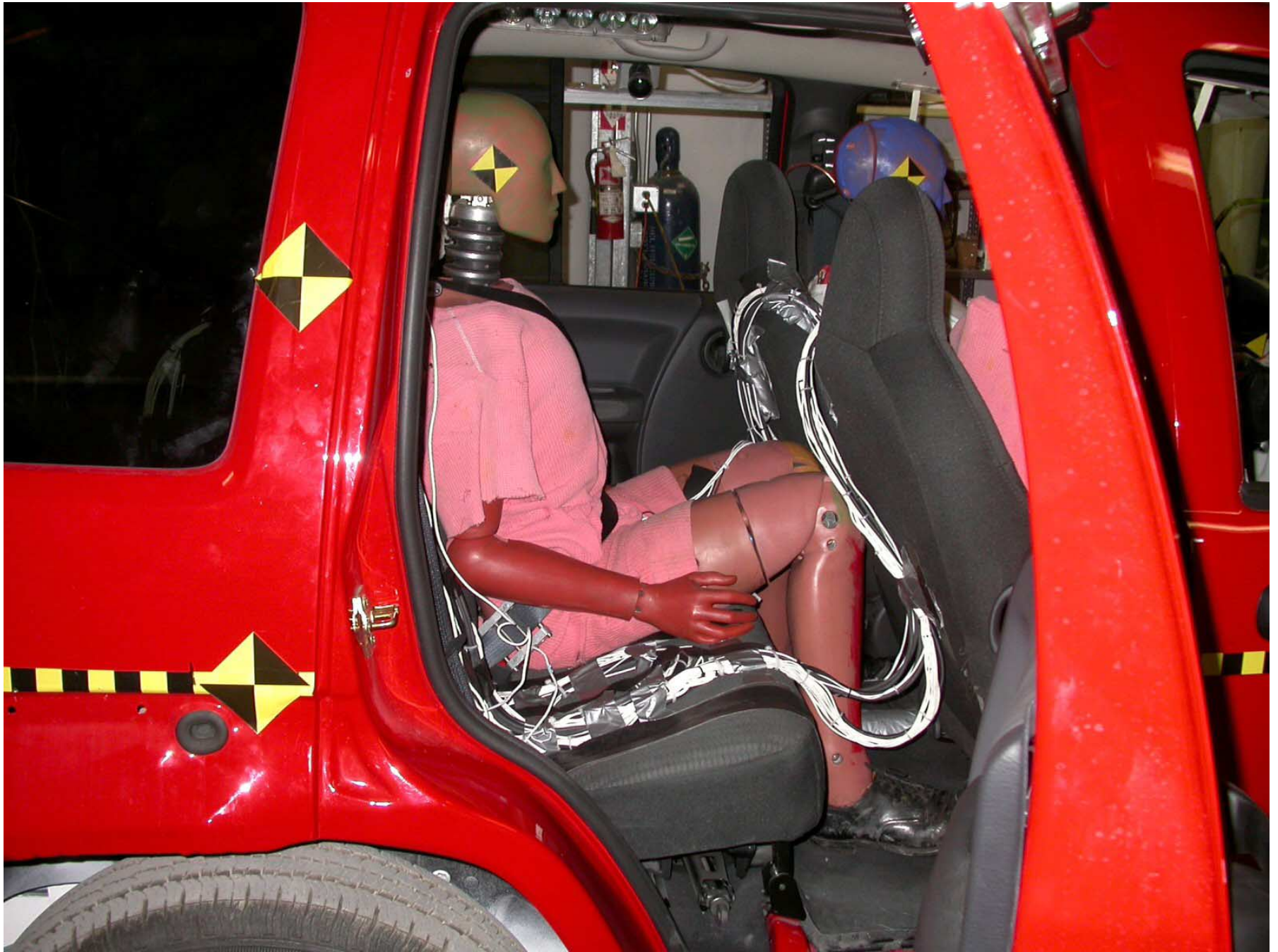
Figure A-97: Pre-Test Center Rear Dummy Door Open (Right Side View)
