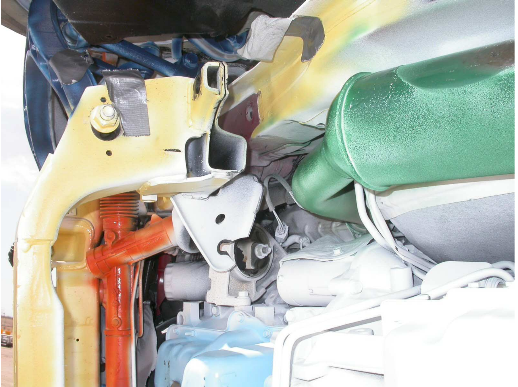
Figure A-47: Post-Test Left Front Sub Frame Mount Damage (Front of Vehicle is to the Left)
