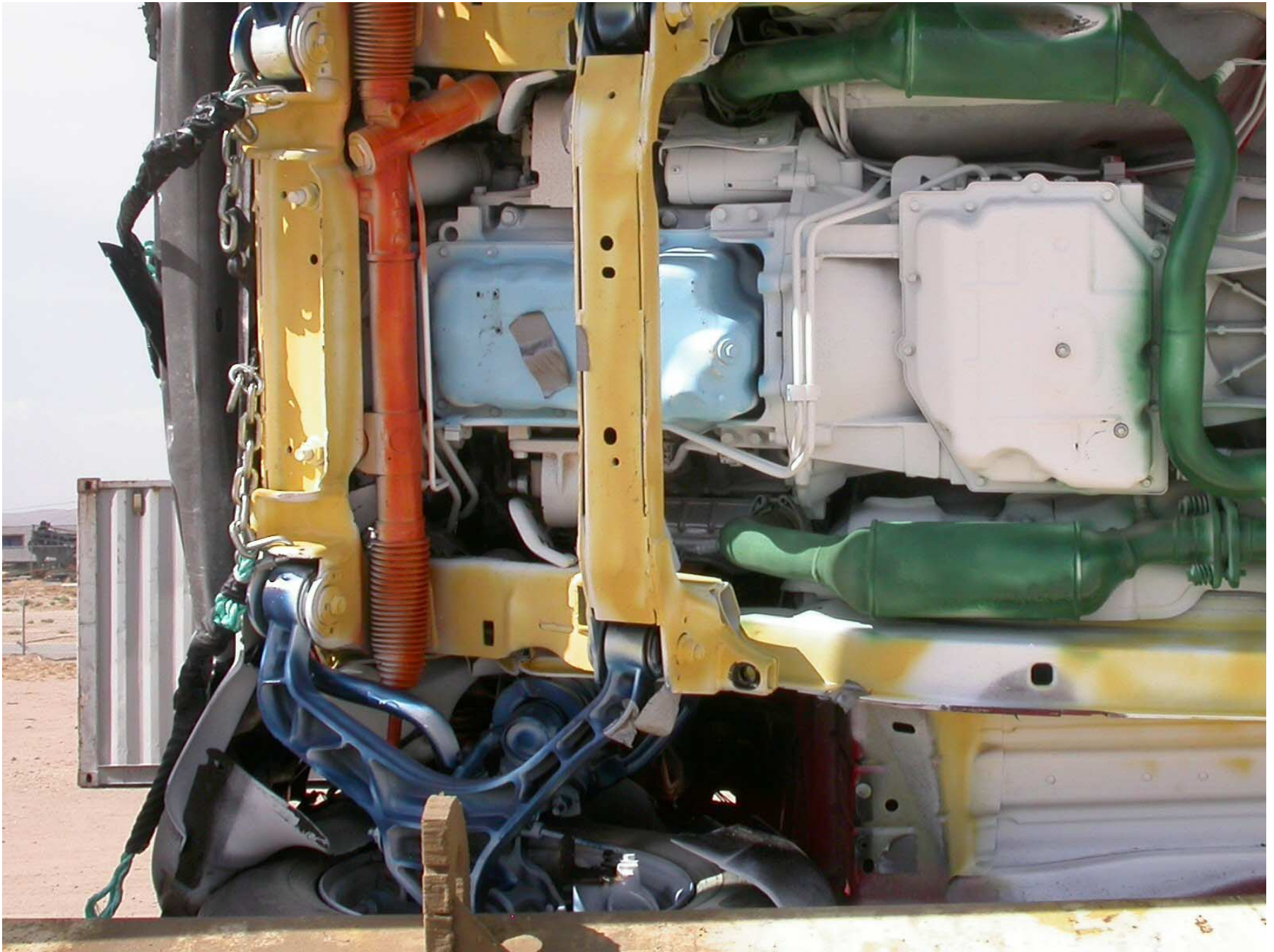
Figure A-52: Right Front Bumper to Rail Attachment (Front of Test Vehicle is to the Left)
