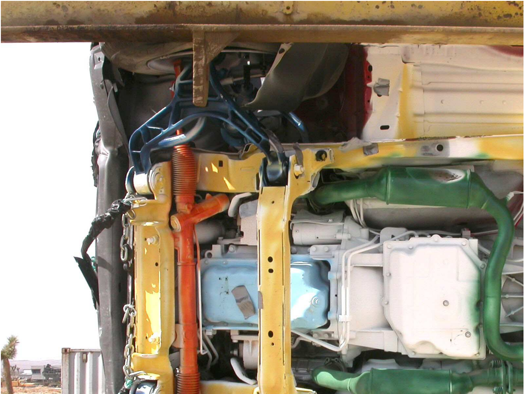
Figure A-46: Post-Test Left Front Bumper to Rail Attachment (Front of Vehicle is to the Left)
