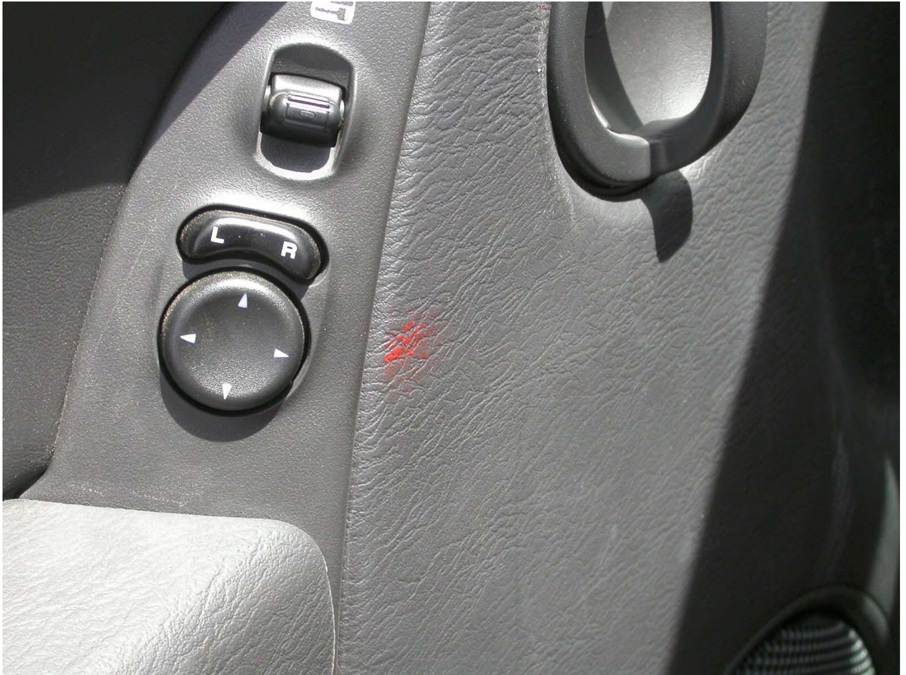
Figure A-73: Post- Test Driver Dummy Contact With Door Panel
