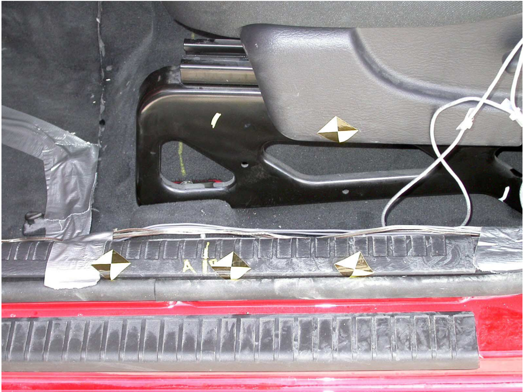
Figure A-69: Post-Test Driver Seat Track
