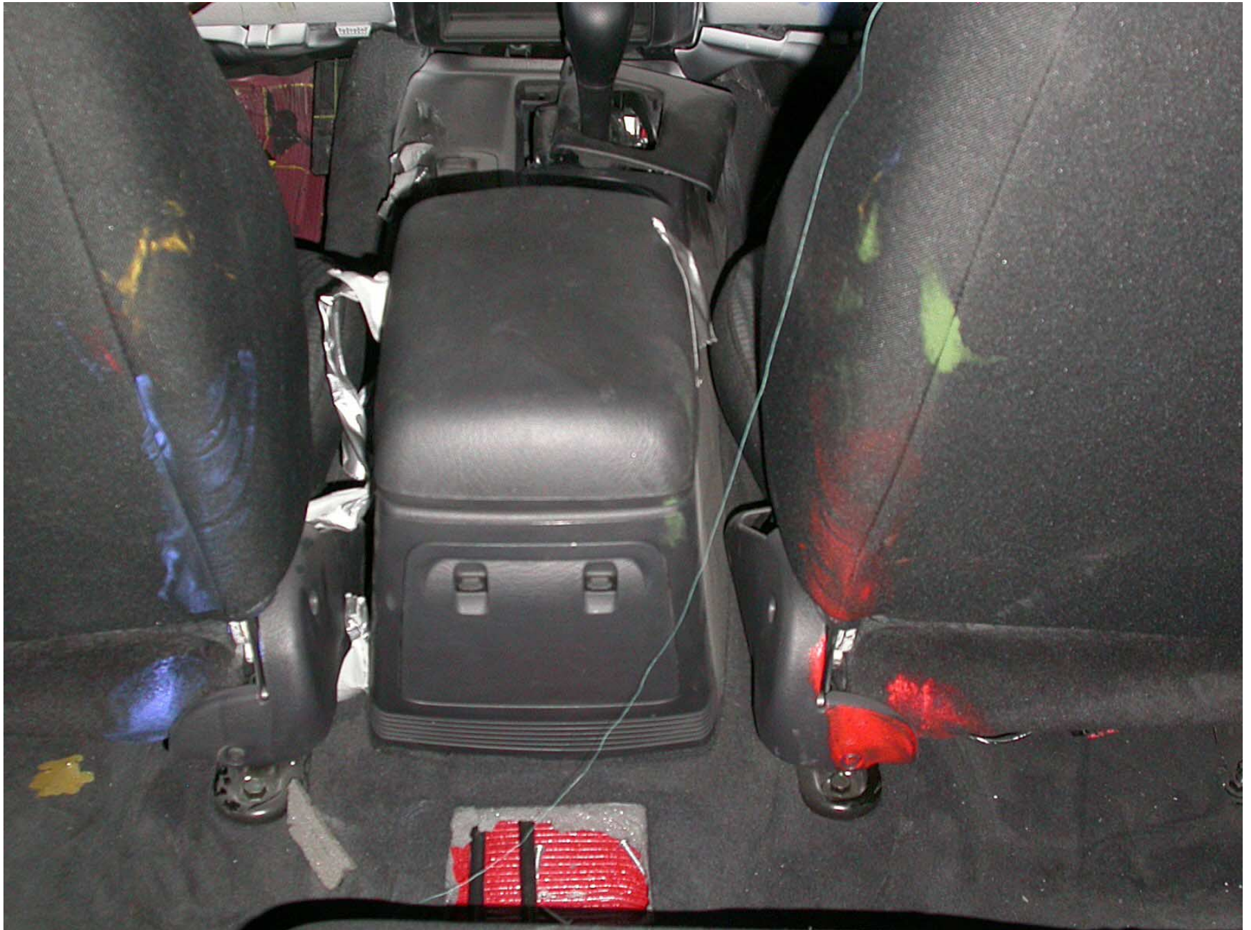
Figure A-104: Post-Test Center Rear Dummy Contact Points
