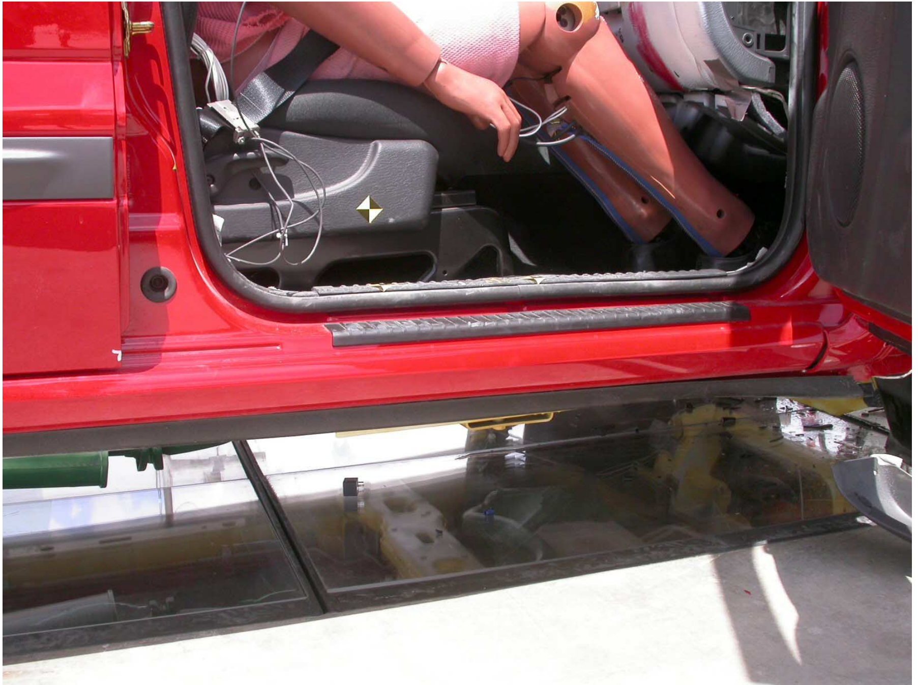
Figure A-28: Post-Test Passenger Side Front Door Sill
