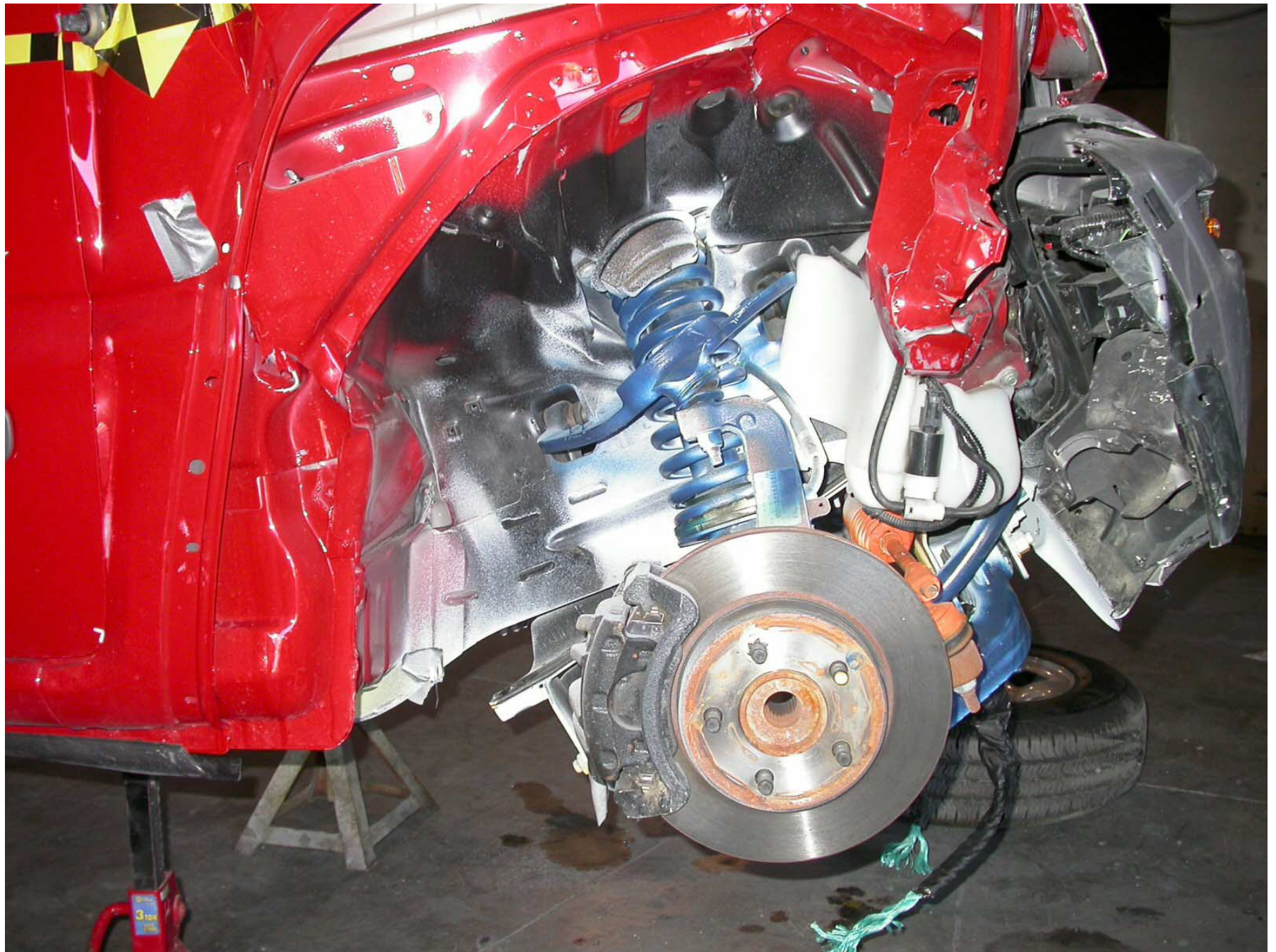
Figure A-49: Post-Test Right Front Wheel Well with Tire and Wheel Removed (Front of Test Vehicle is to the Right)
