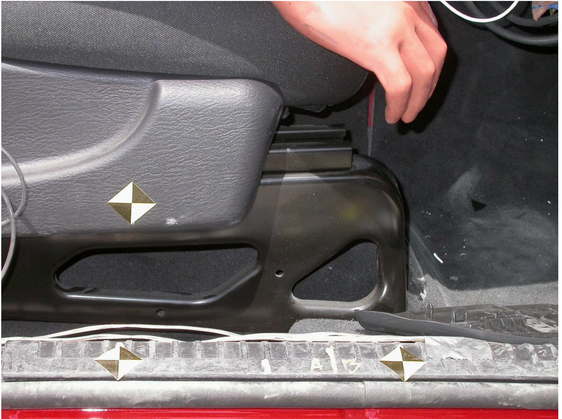
Figure A-87: Post-Test Passenger Seat Track
