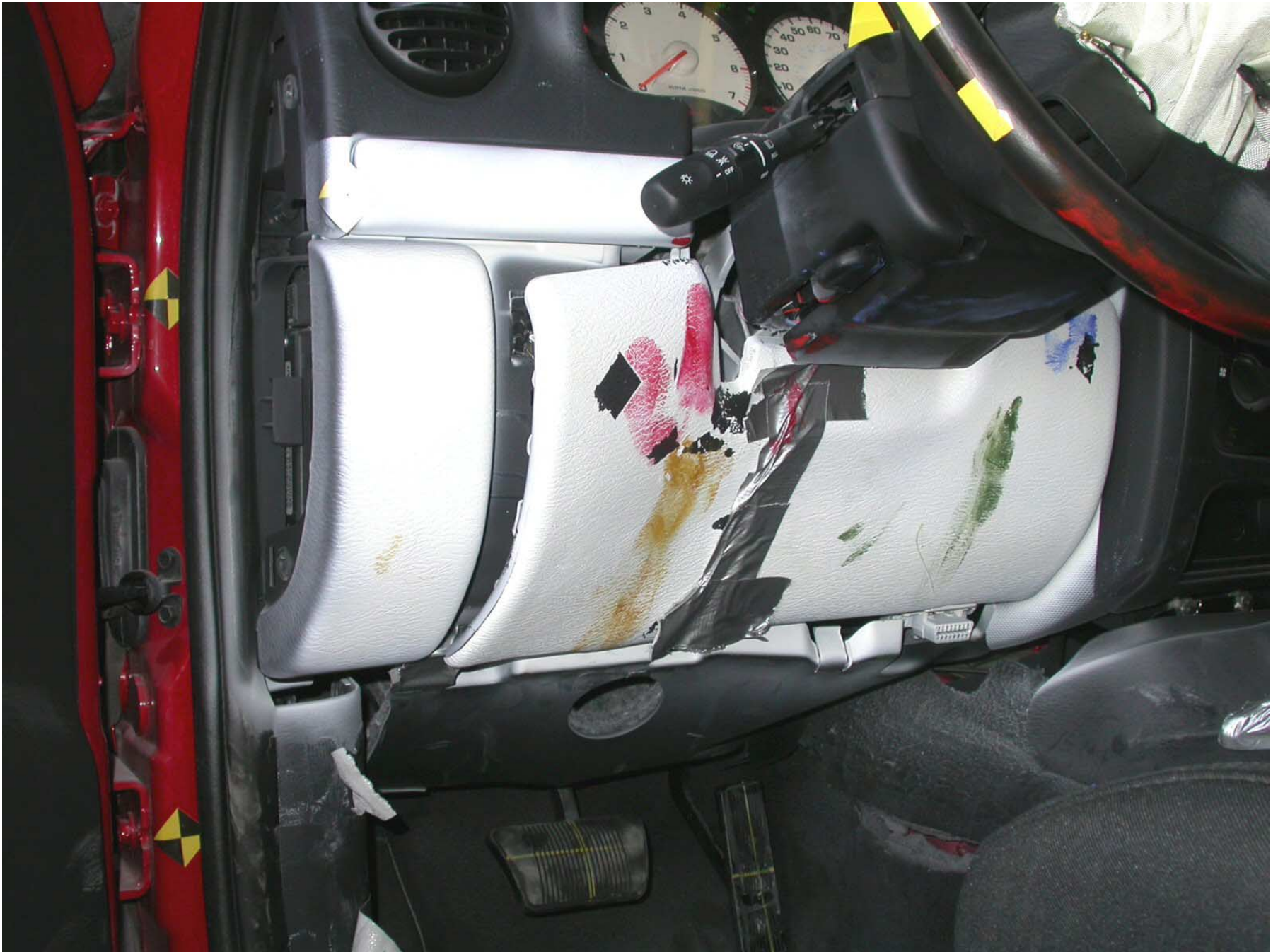
Figure A-65: Post-Test Driver Side Knee Bolster
