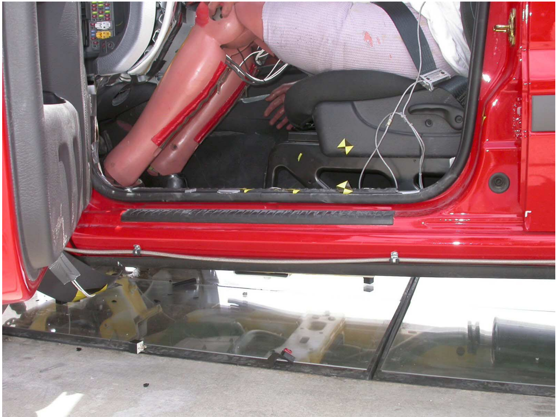
Figure A-21: Post-Test Driver Side Front Door Sill
