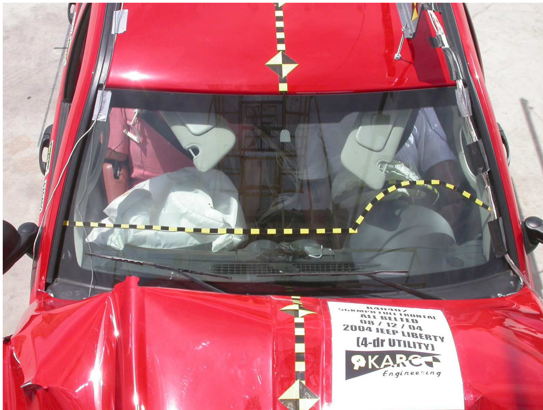
Figure A-31: Post-Test Windshield View
