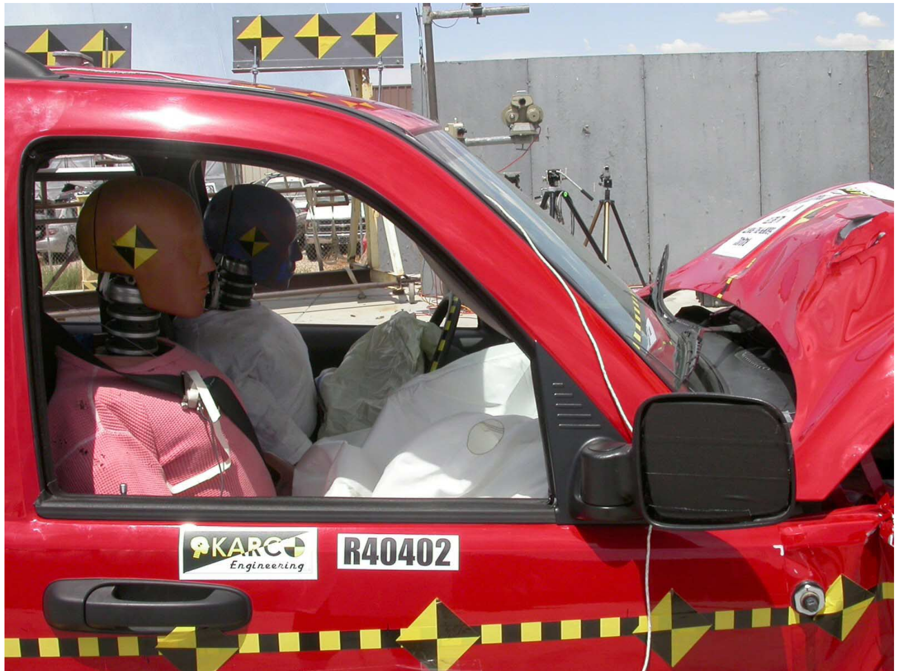
Figure A-24: Post-Test Passenger Side A Pillar
