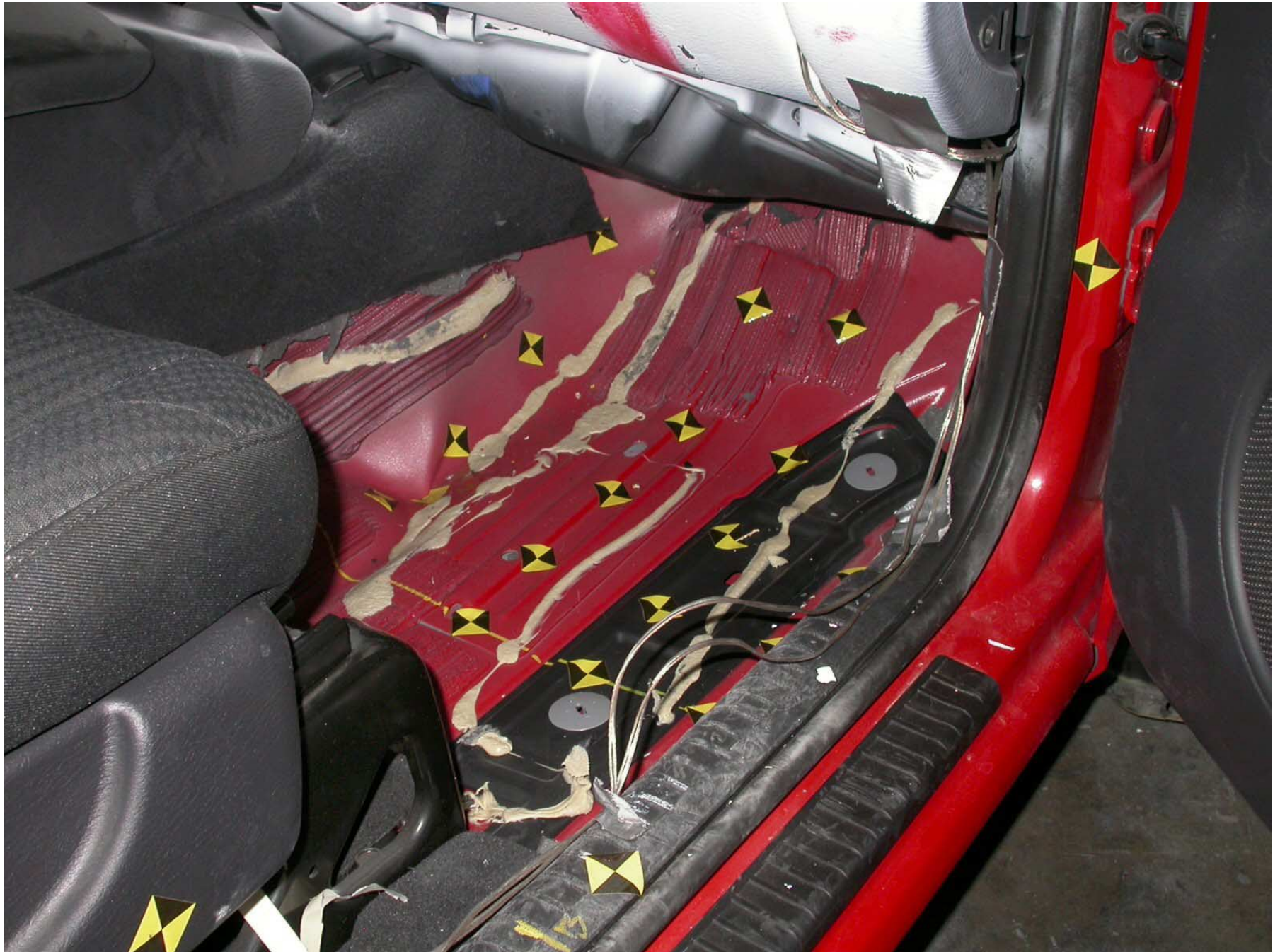
Figure A-85: Post-Test Passenger Side Floor Pan
