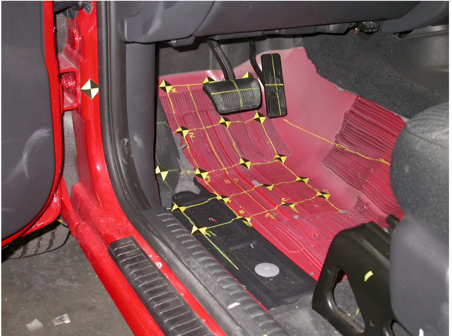
Figure A-66: Pre-Test Driver Side Floor Pan
