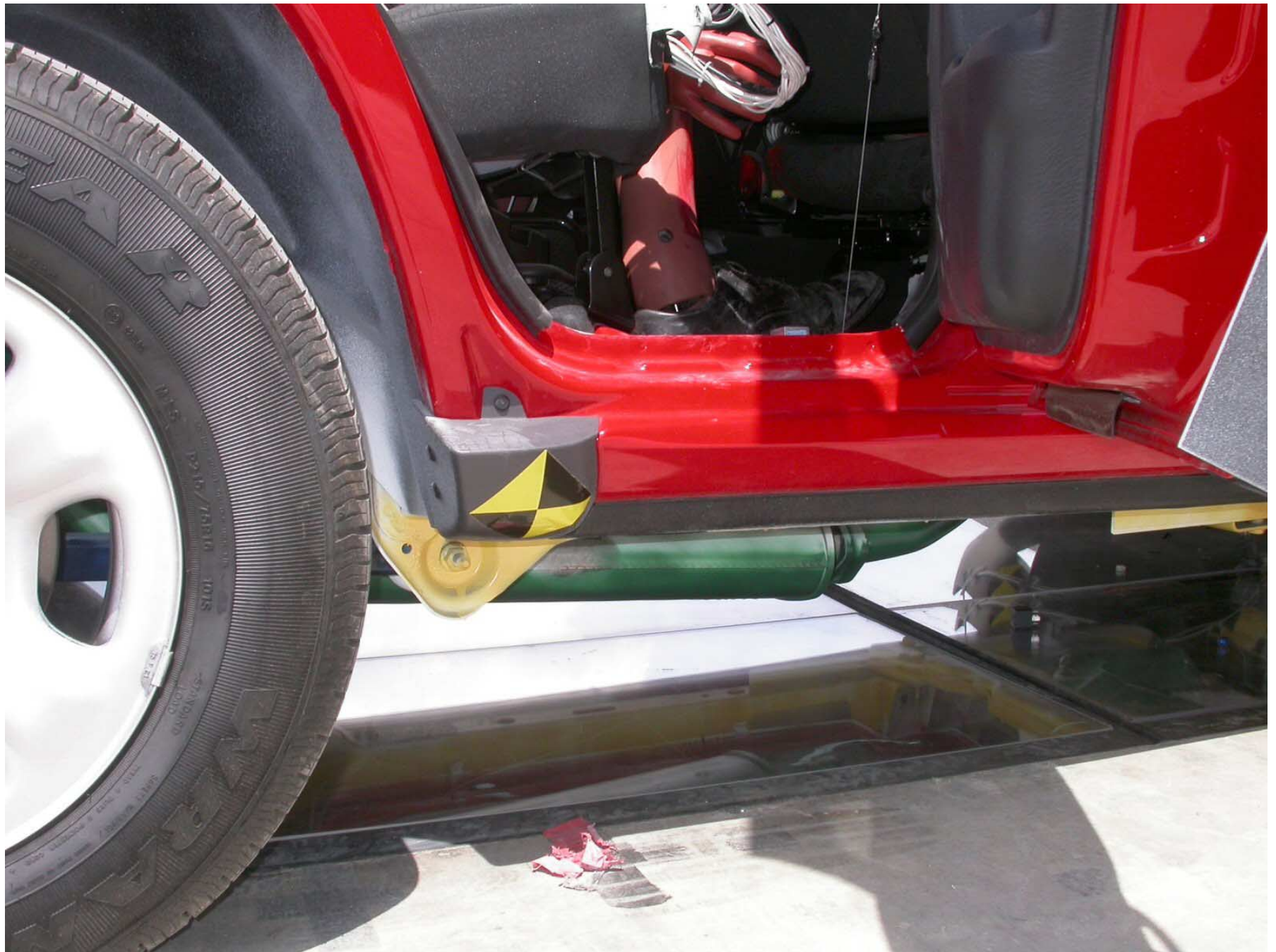
Figure A-29: Post-Test Passenger Side Rear Door Sill
