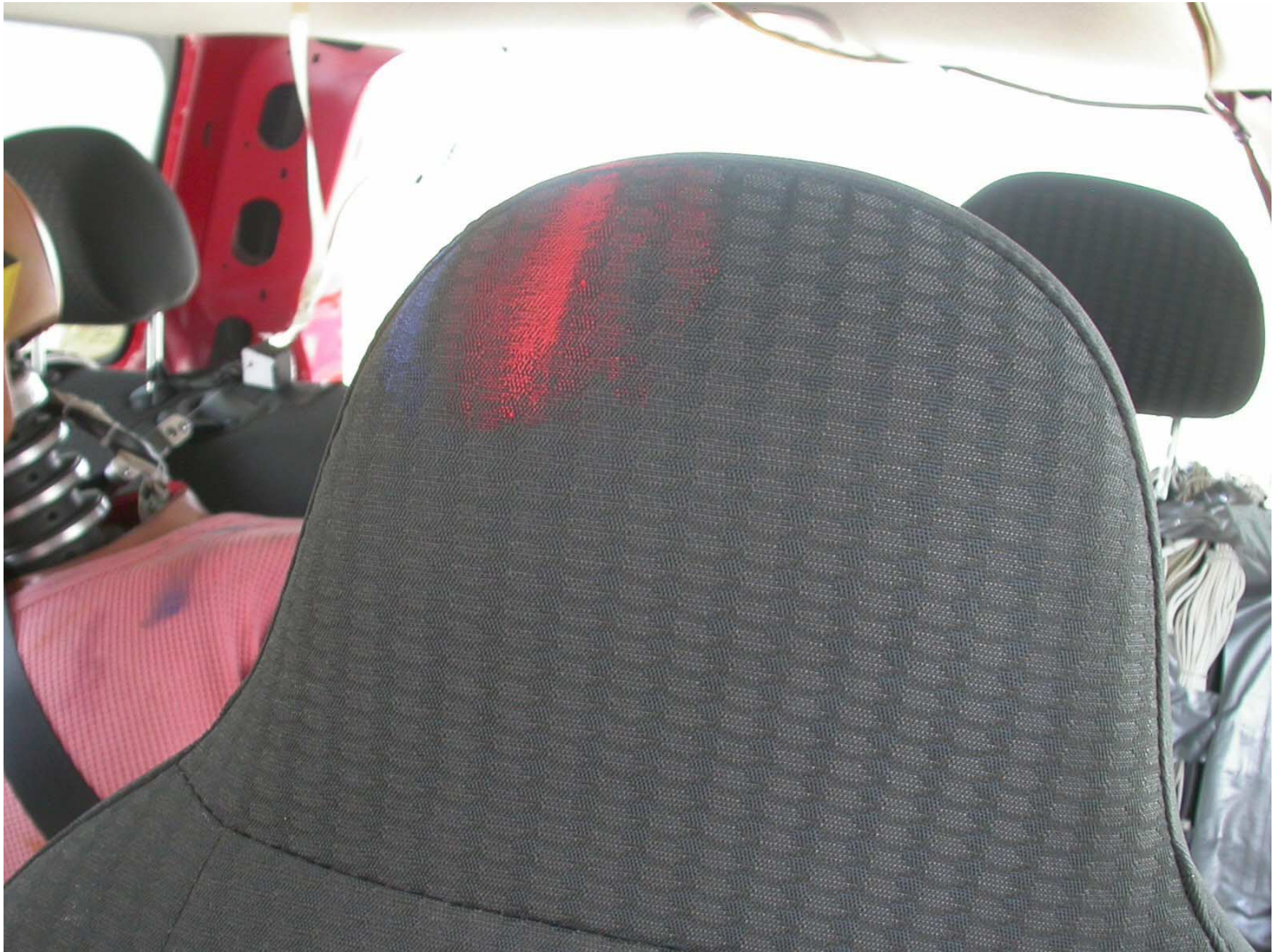
Figure A-72: Post-Test Driver Dummy Contact With Seat Head Rest
