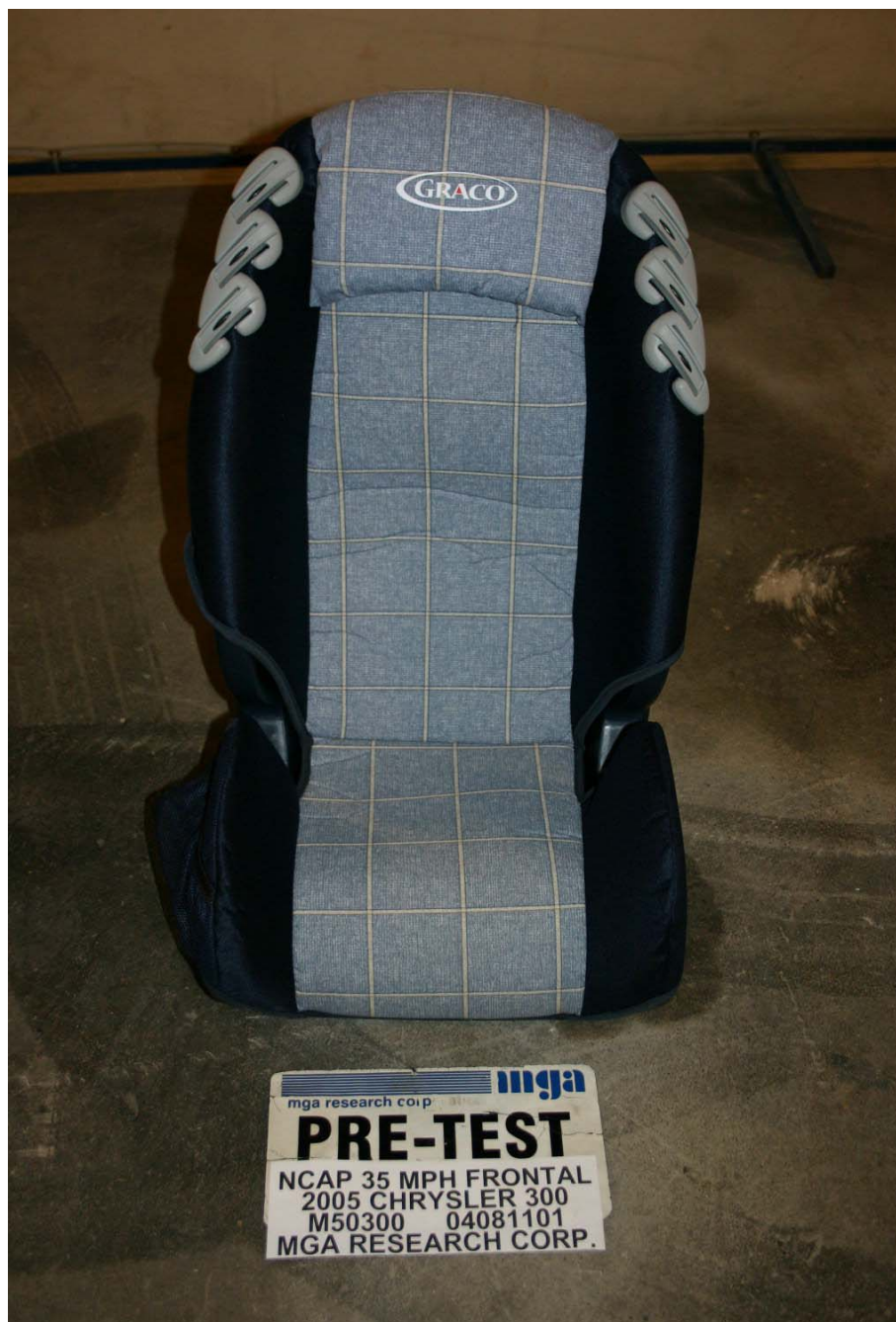
Pre-Test Front View of Position 4 CRS
