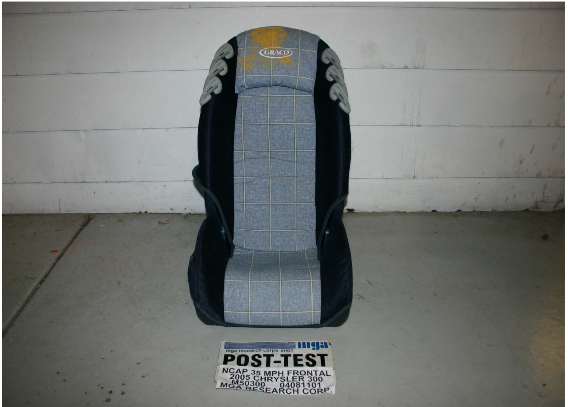
Post-Test Front View of Position 4 CRS
