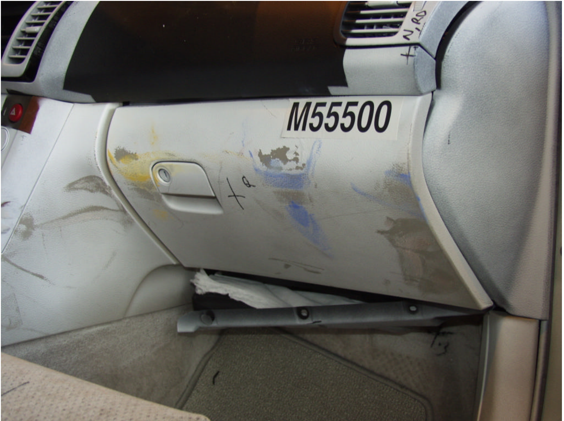
Figure A-53 POST-TEST PASSENGER KNEE BOLSTER VIEW
