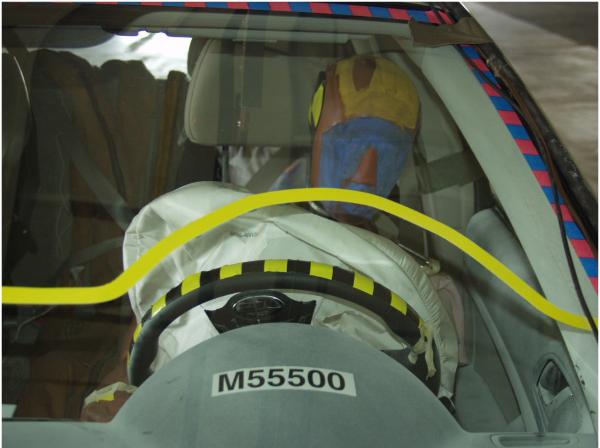
Figure A-31 POST-TEST DRIVER HEAD LOCATION
