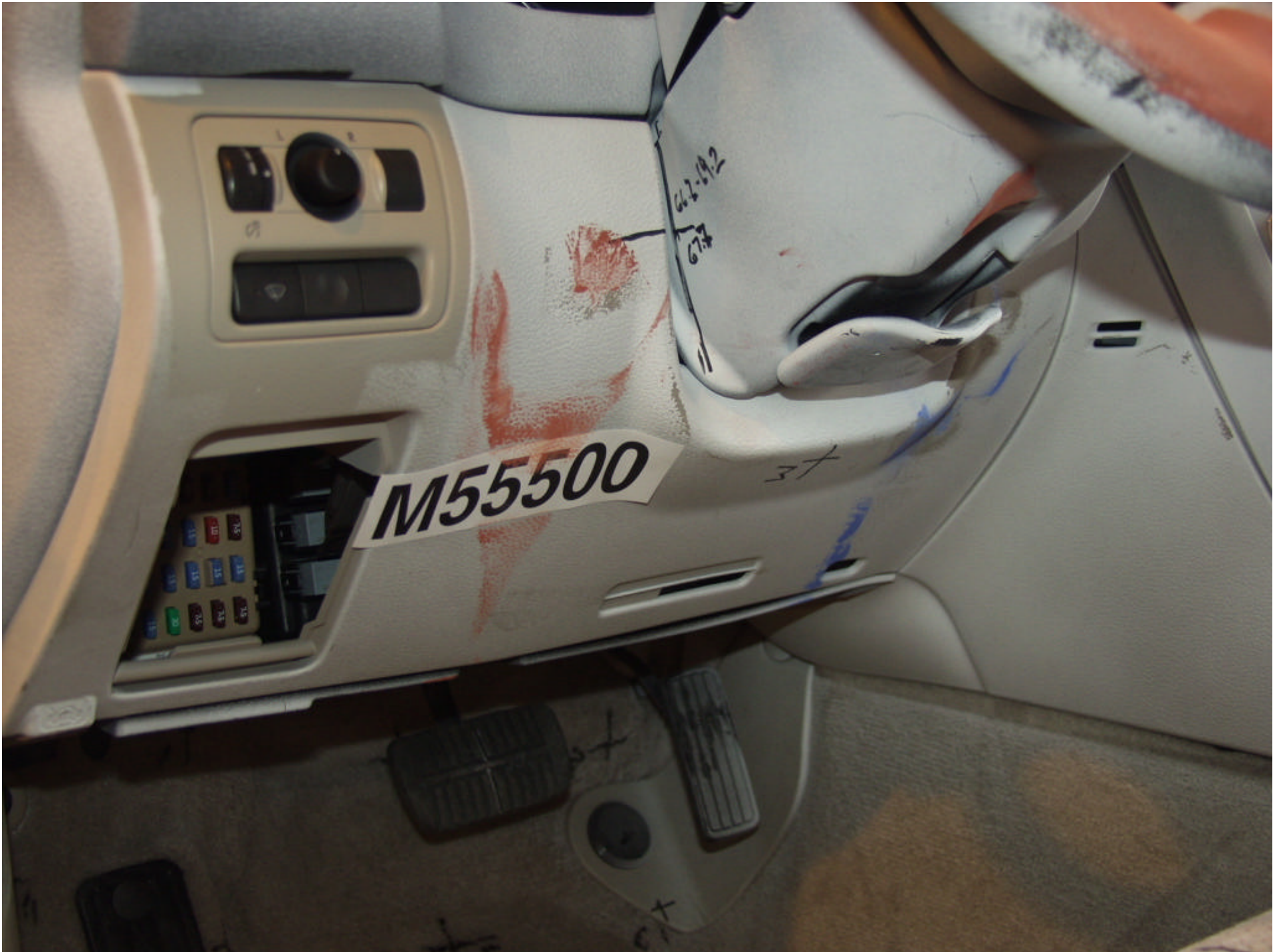
Figure A-39 POST-TEST DRIVER KNEE BOLSTER VIEW
