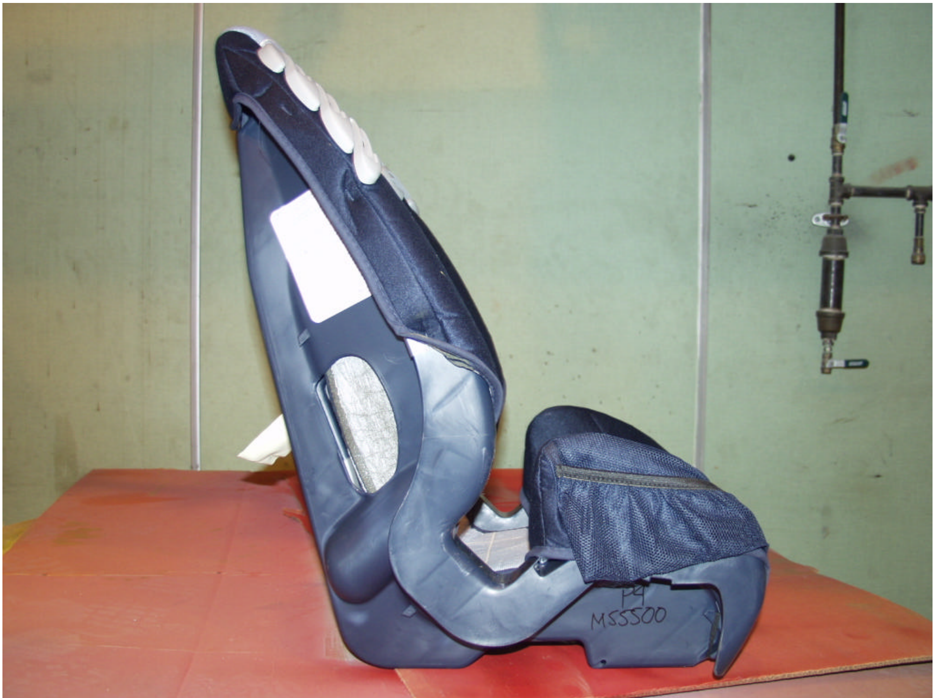
Figure 3-18 POST-TEST RIGHT SIDE VIEW OF POSITION 4 CRS
