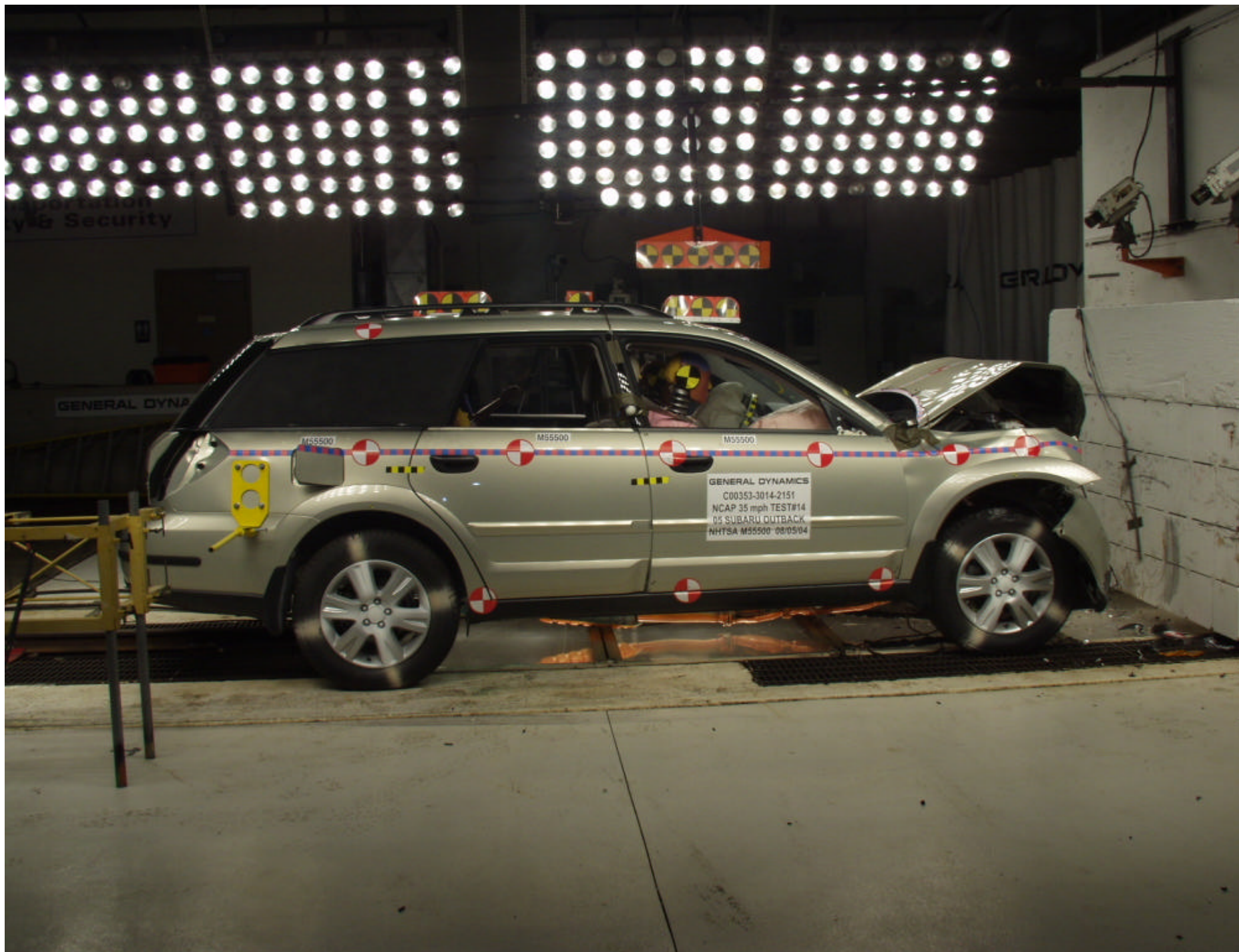
Figure A-11 POST-TEST RIGHT SIDE VIEW
