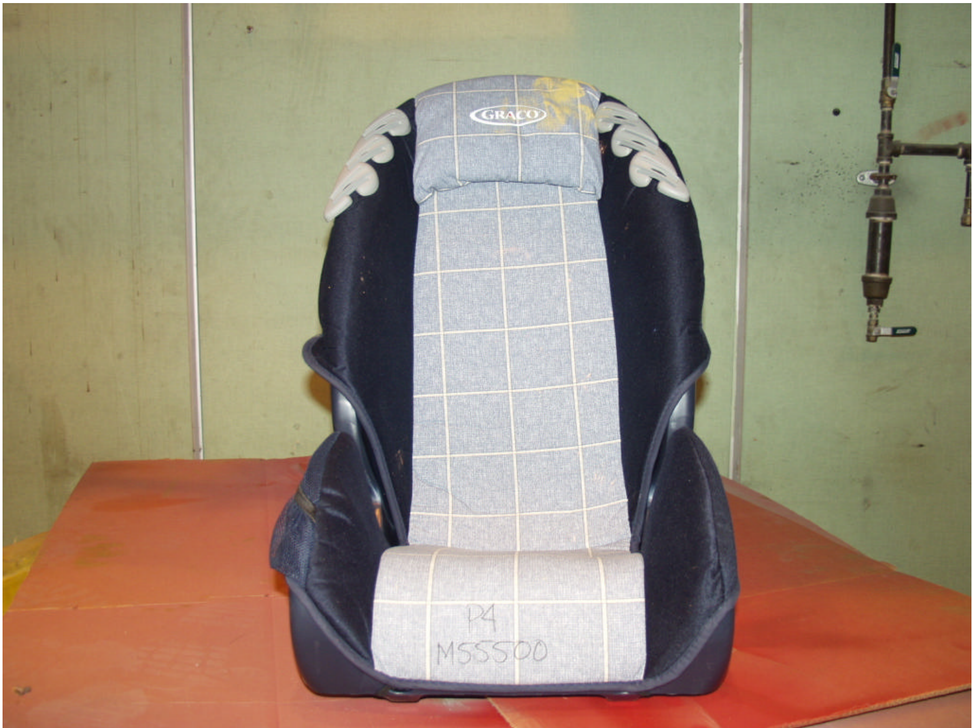
Figure 3-12 POST-TEST FRONTAL VIEW OF POSITION 4 CRS
