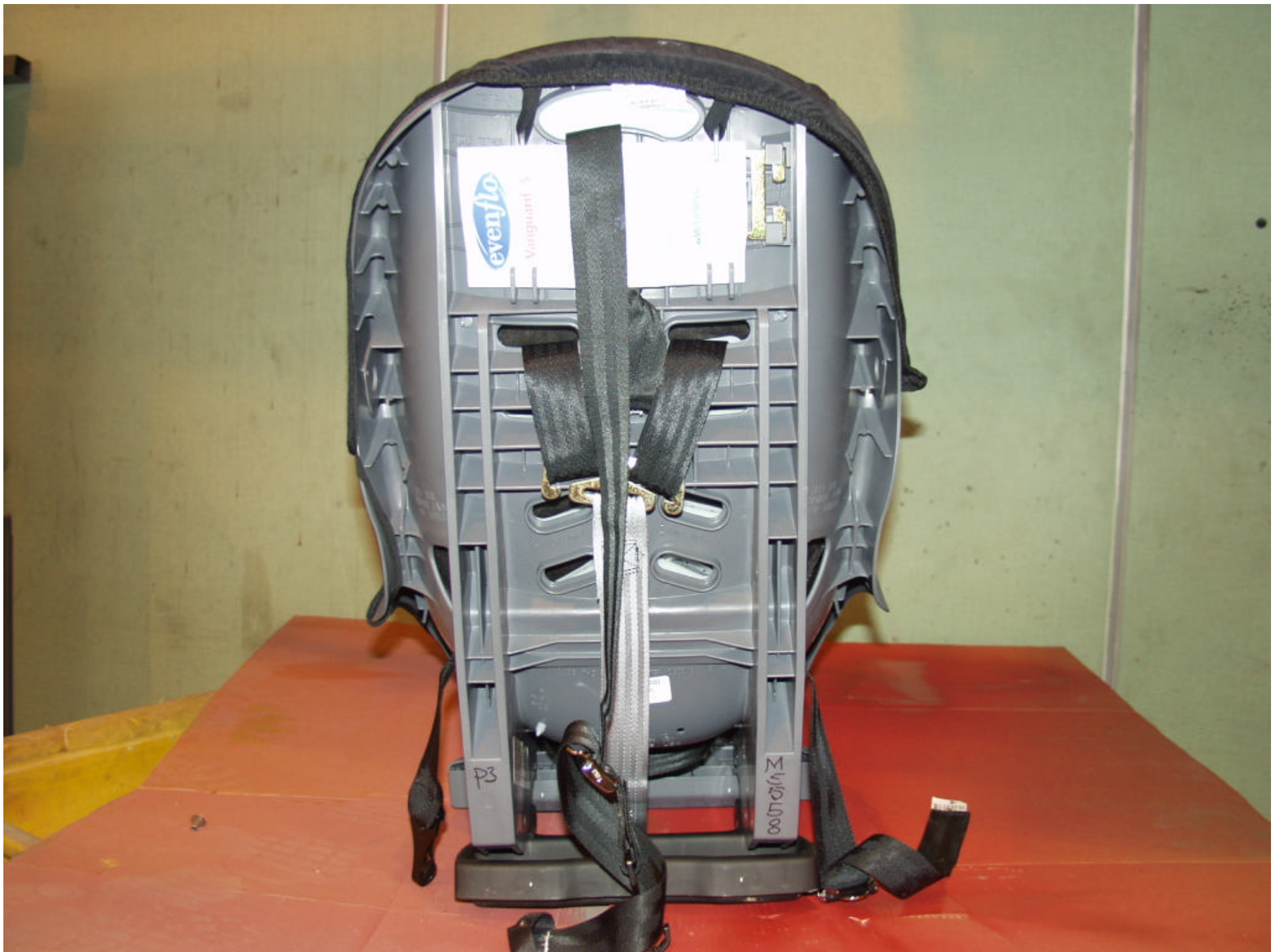
Figure 3-5 POST-TEST REAR VIEW OF POSITION 3 CRS
