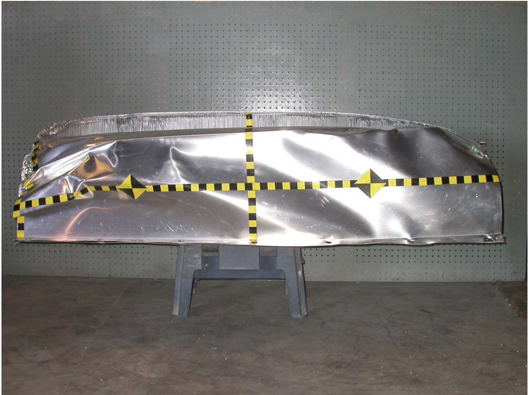
Figure A-53: Top View of Deformable Barrier, Post-Test
