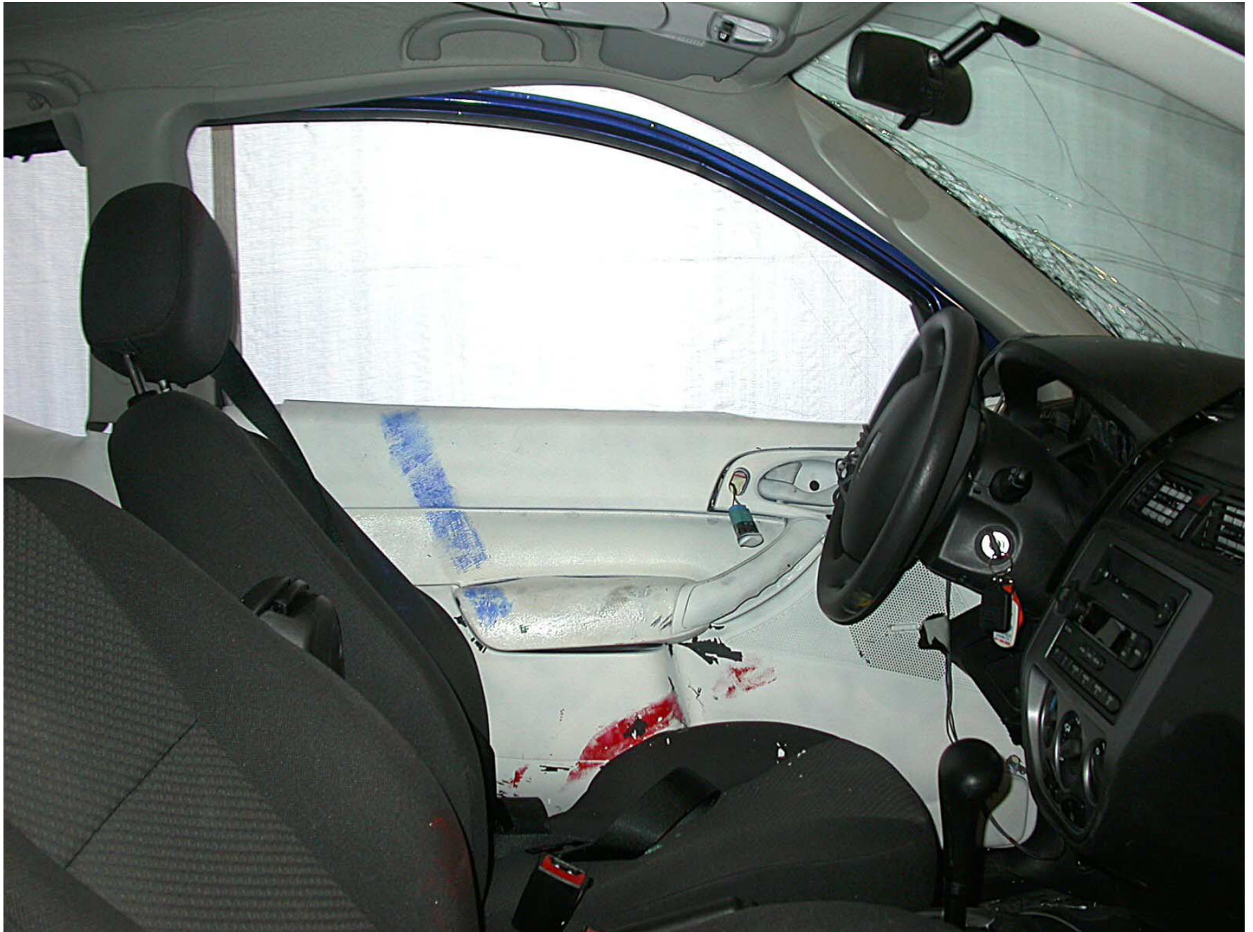
Figure A-41: Driver Dummy Contact Points Inside View, Post-Test (Vehicle Moved)
