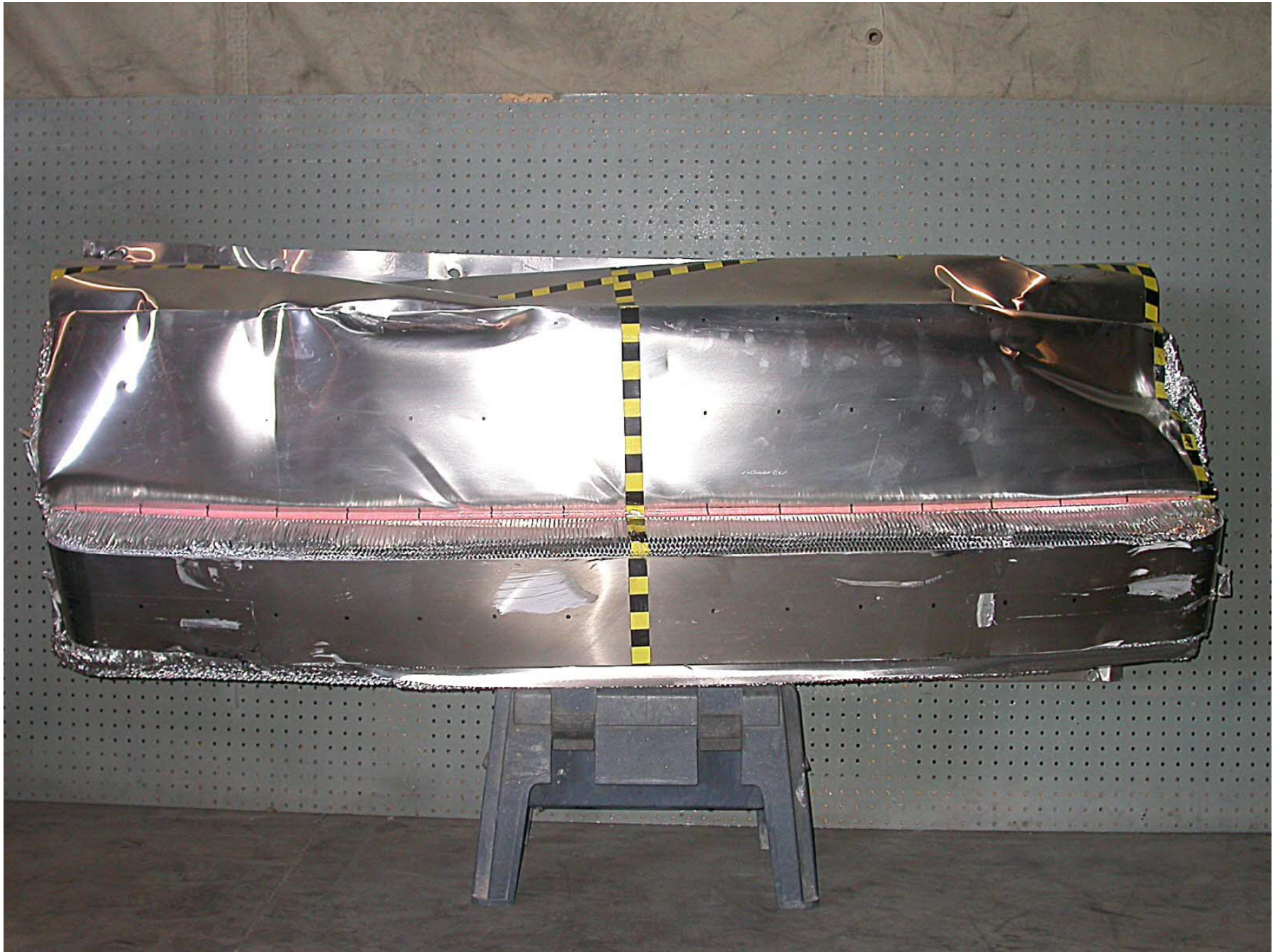
Figure A-51: Front View of Deformable Barrier, Post-Test
