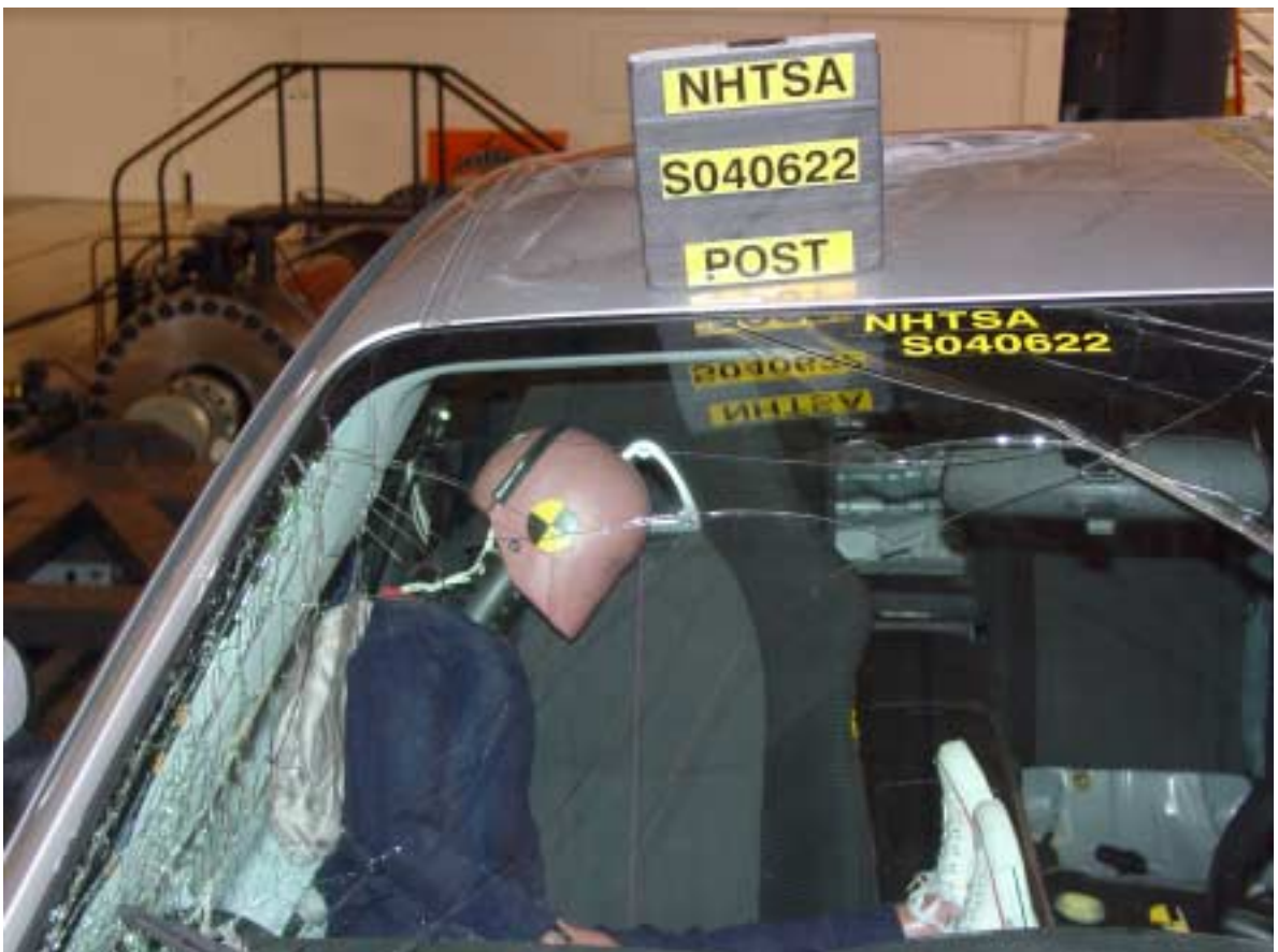
Figure A-8 Post-Test Front View of Dummy
