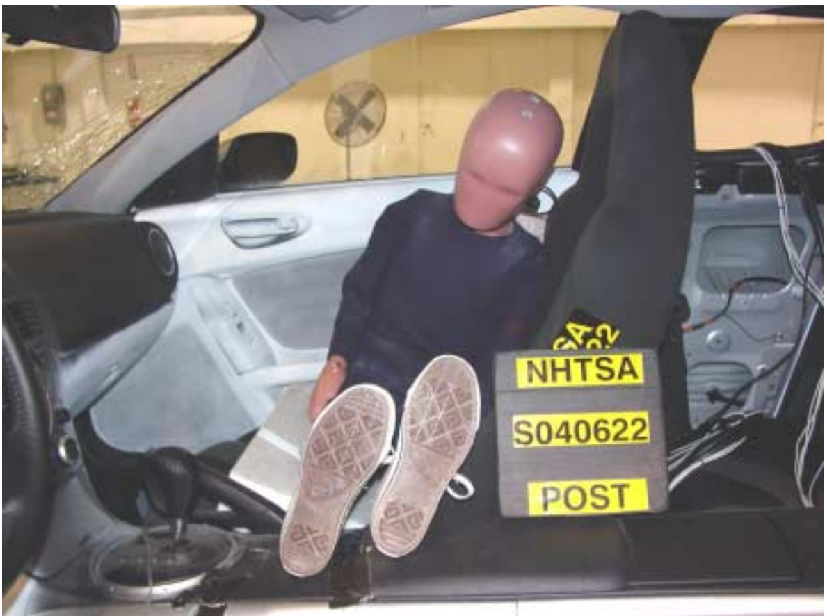
Figure A-6 Post-Test Left Side View of Dummy
