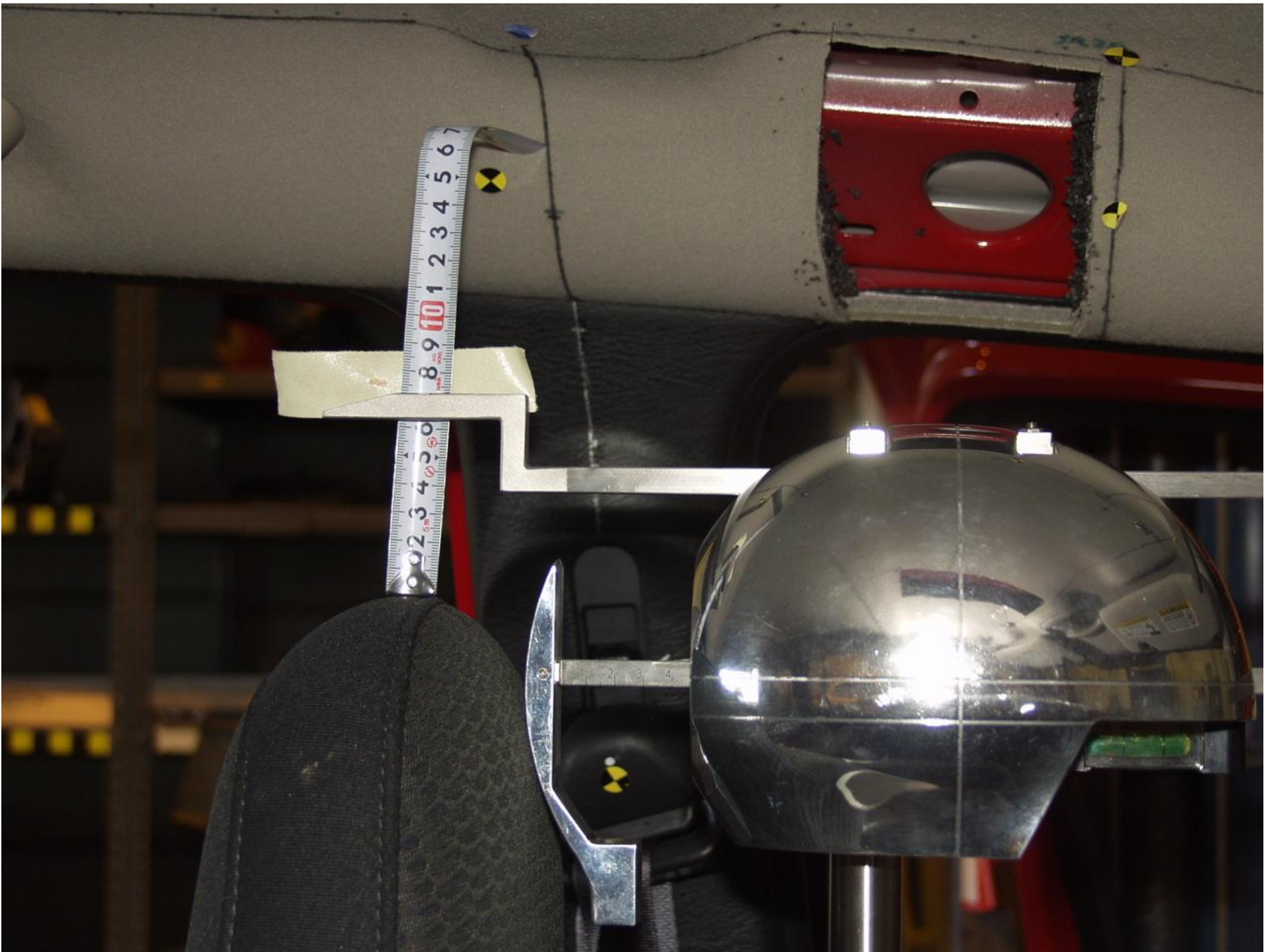
Figure A-1 DRIVER ICBC BACKSET VIEW
