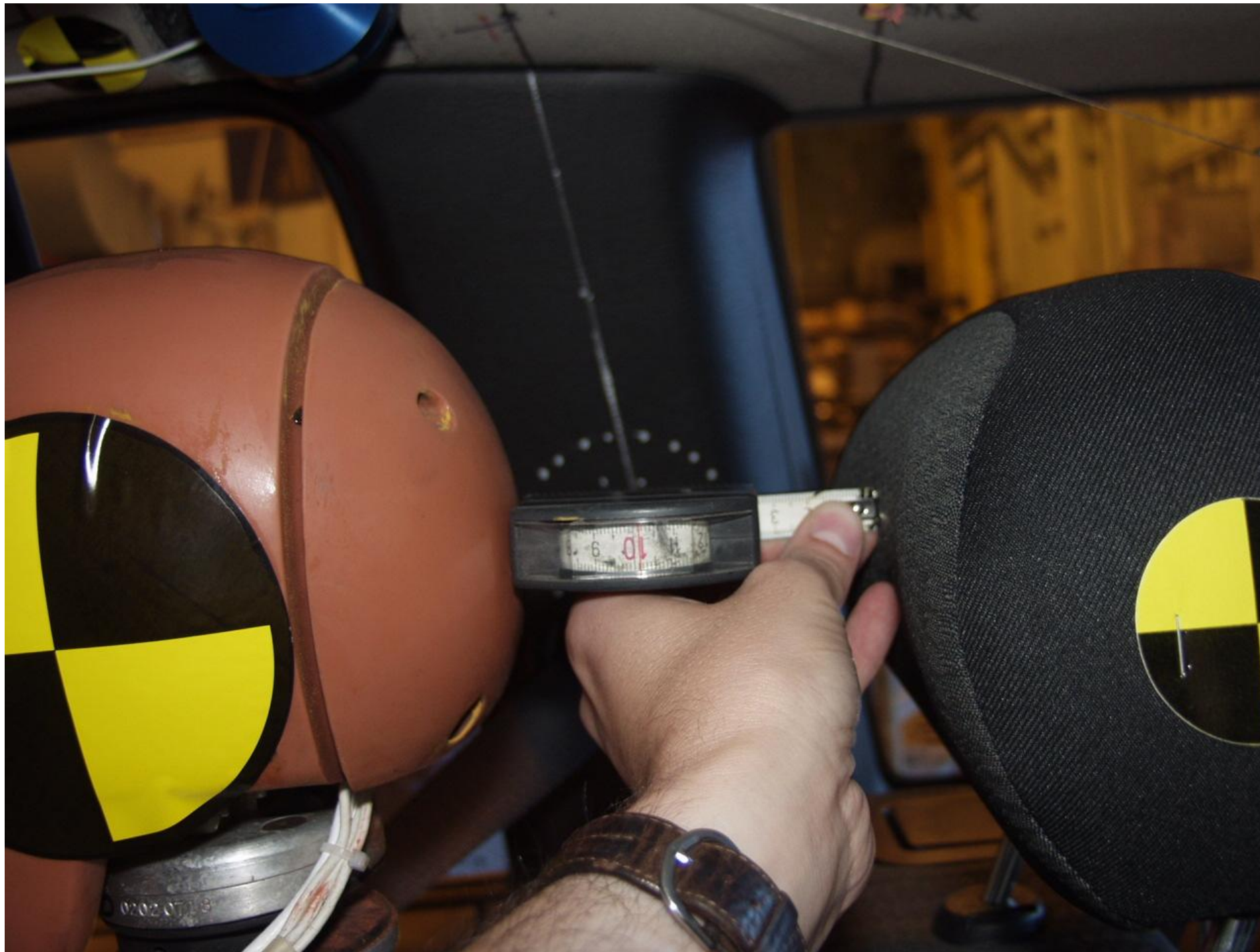
Figure A-4 PRE-TEST PASSENGER BACKSET VIEW
