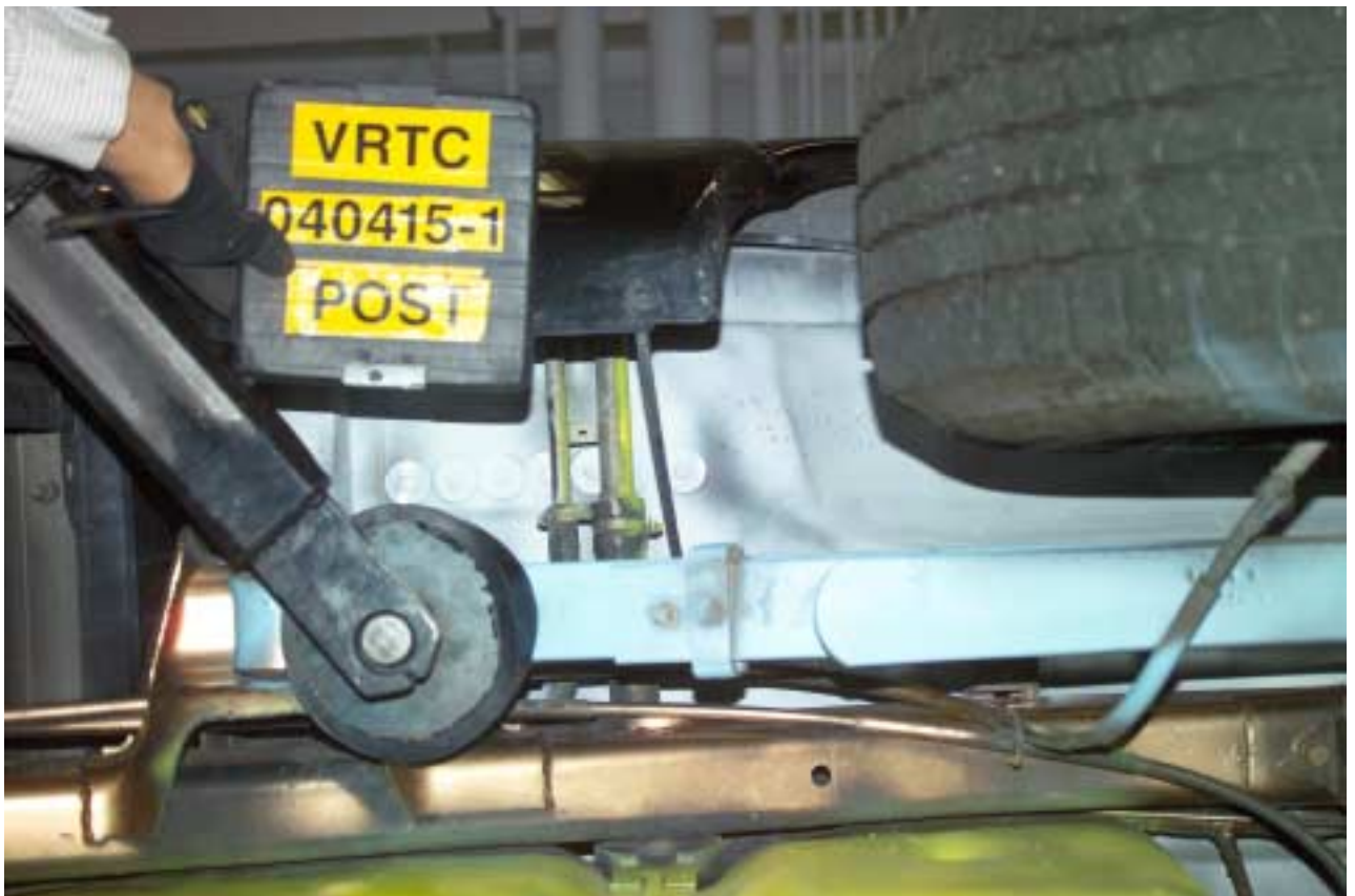
Figure A-25 Post-Test Fuel Filler Neck View
