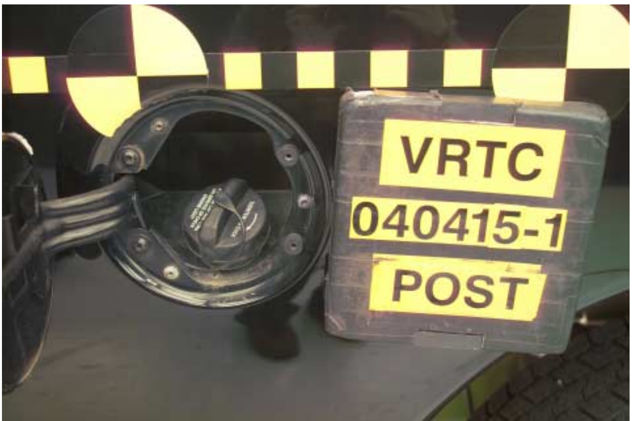
Figure A-27 Post-Test Fuel Filler Cap View
