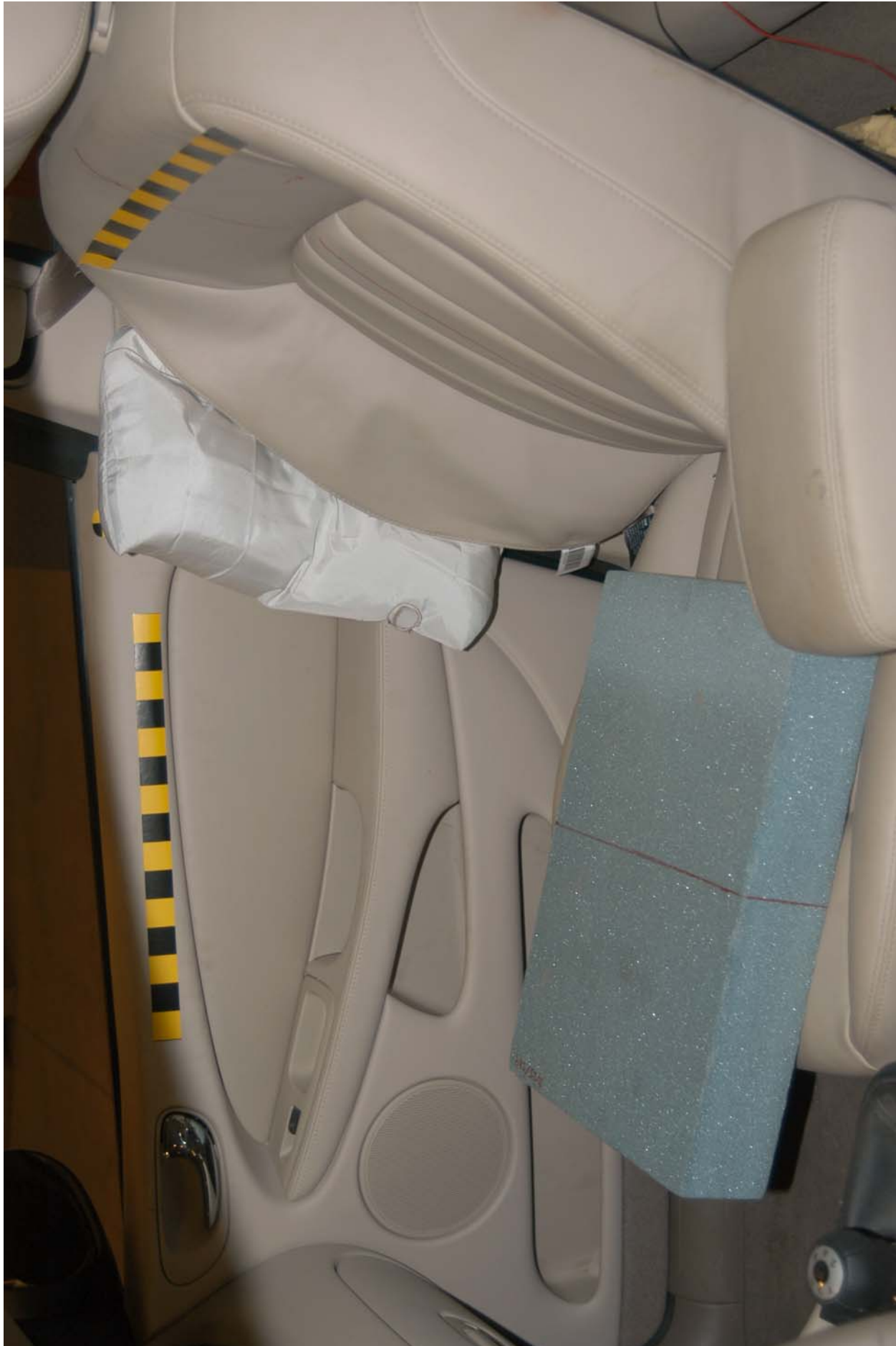
Figure A-10: POST-TEST (25 MARCH 2004) LEFT OVERALL VIEW OF AIRBAG AND BOOSTER BLOCK
