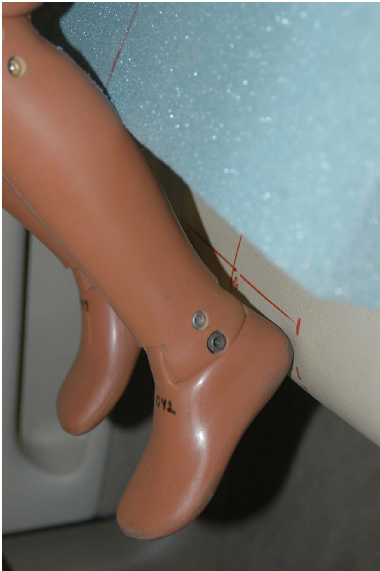
Figure A-9: PRE-TEST (25 MARCH 2004) VIEW OF HYBRID III 3-YEAR-OLD FEET PLACEMENT
