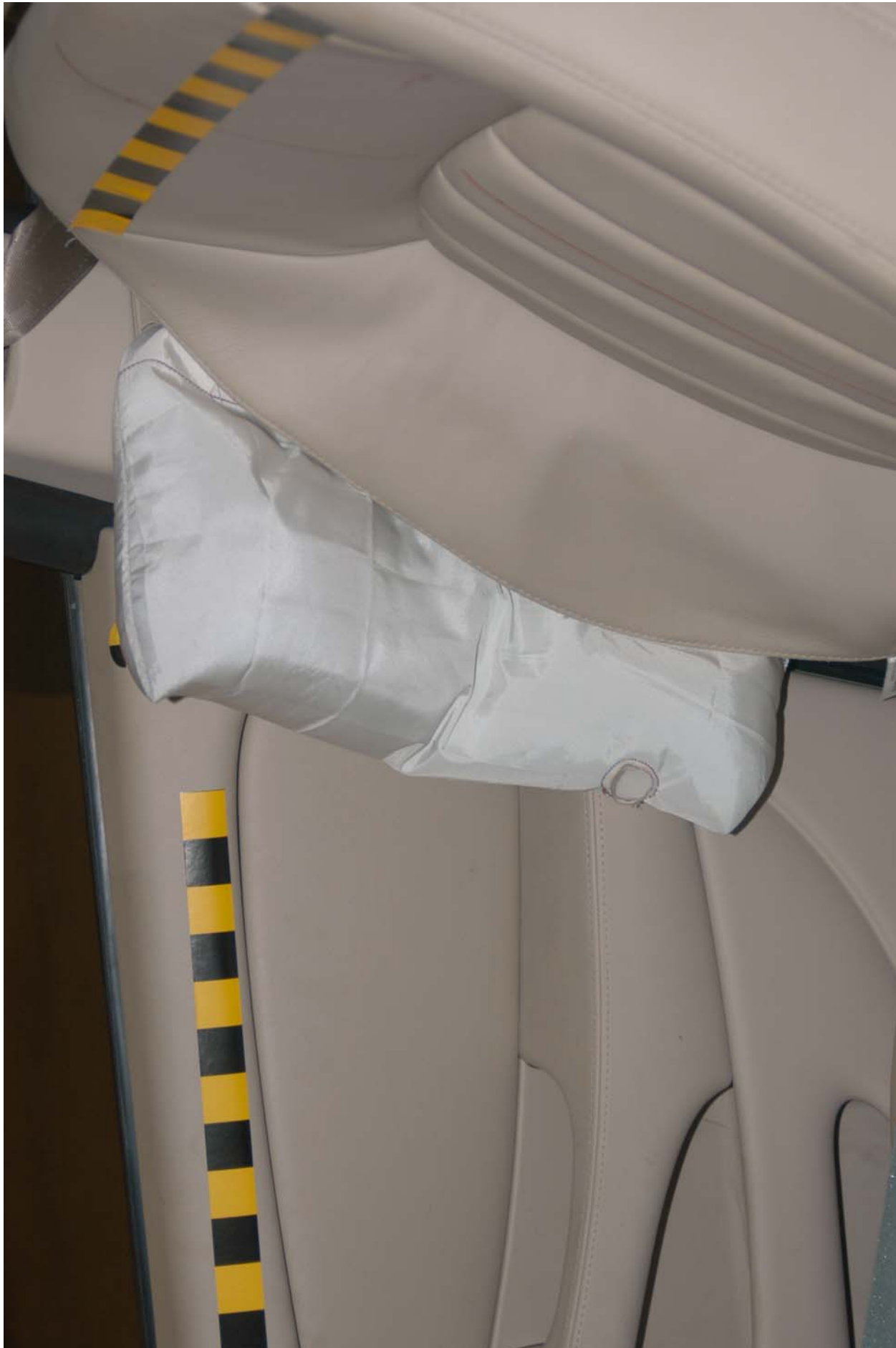
Figure A-11: POST-TEST (25 MARCH 2004) LEFT VIEW OF AIRBAG
