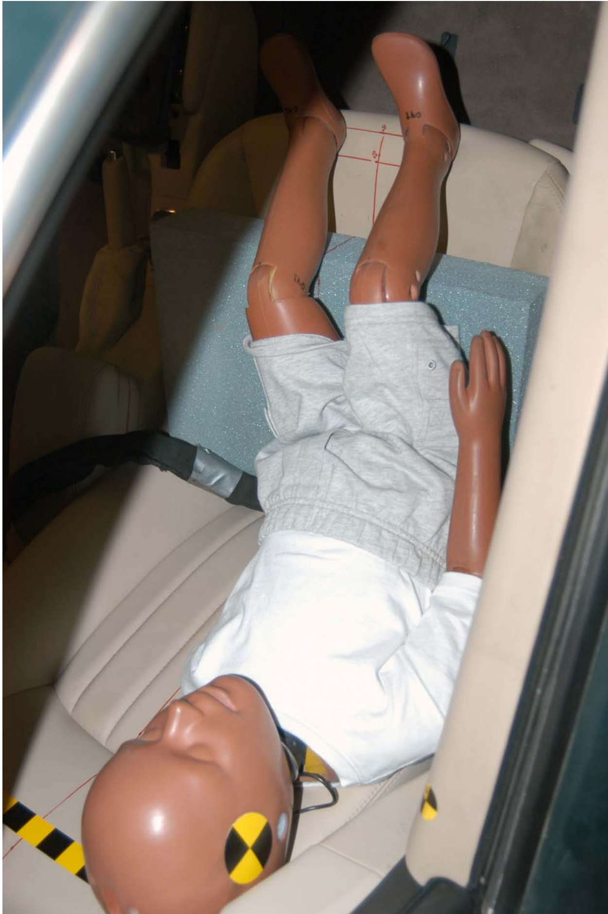
Figure A-3: PRE-TEST (25 MARCH 2004) RIGHT OCCUPANT COMPARTMENT VIEW OF HYBRID III 3-YEAR-OLD
