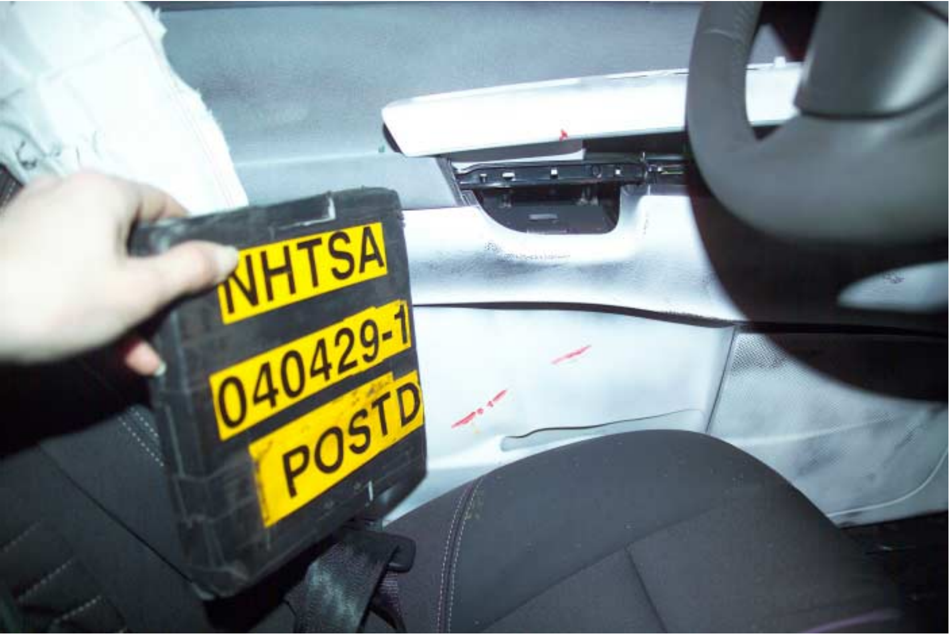
Figure A-35 Post-Test Front SID HIII Contact - View 2 A-38
