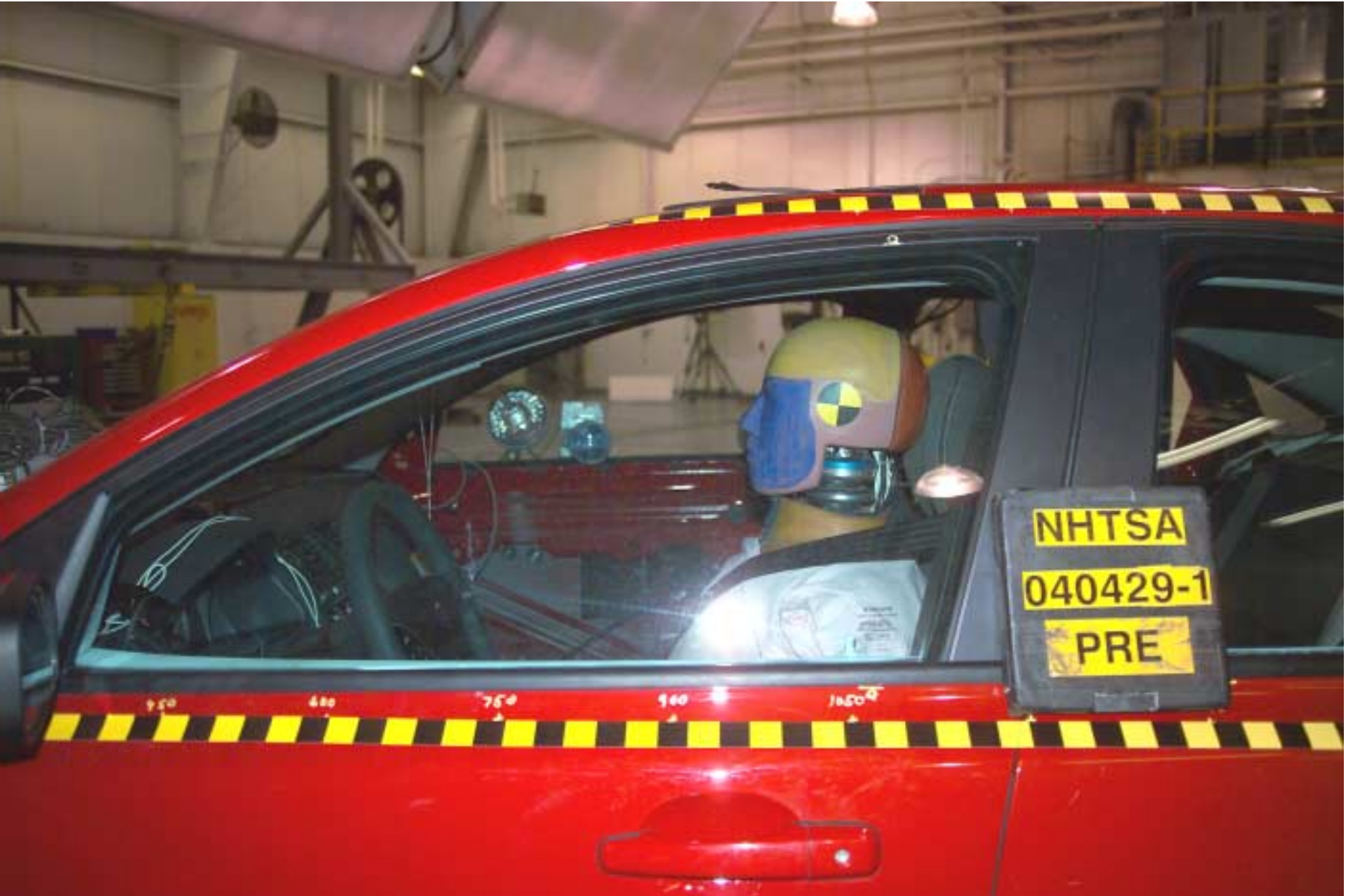
Figure A-22 Pre-Test Left View of Front SID HIII
