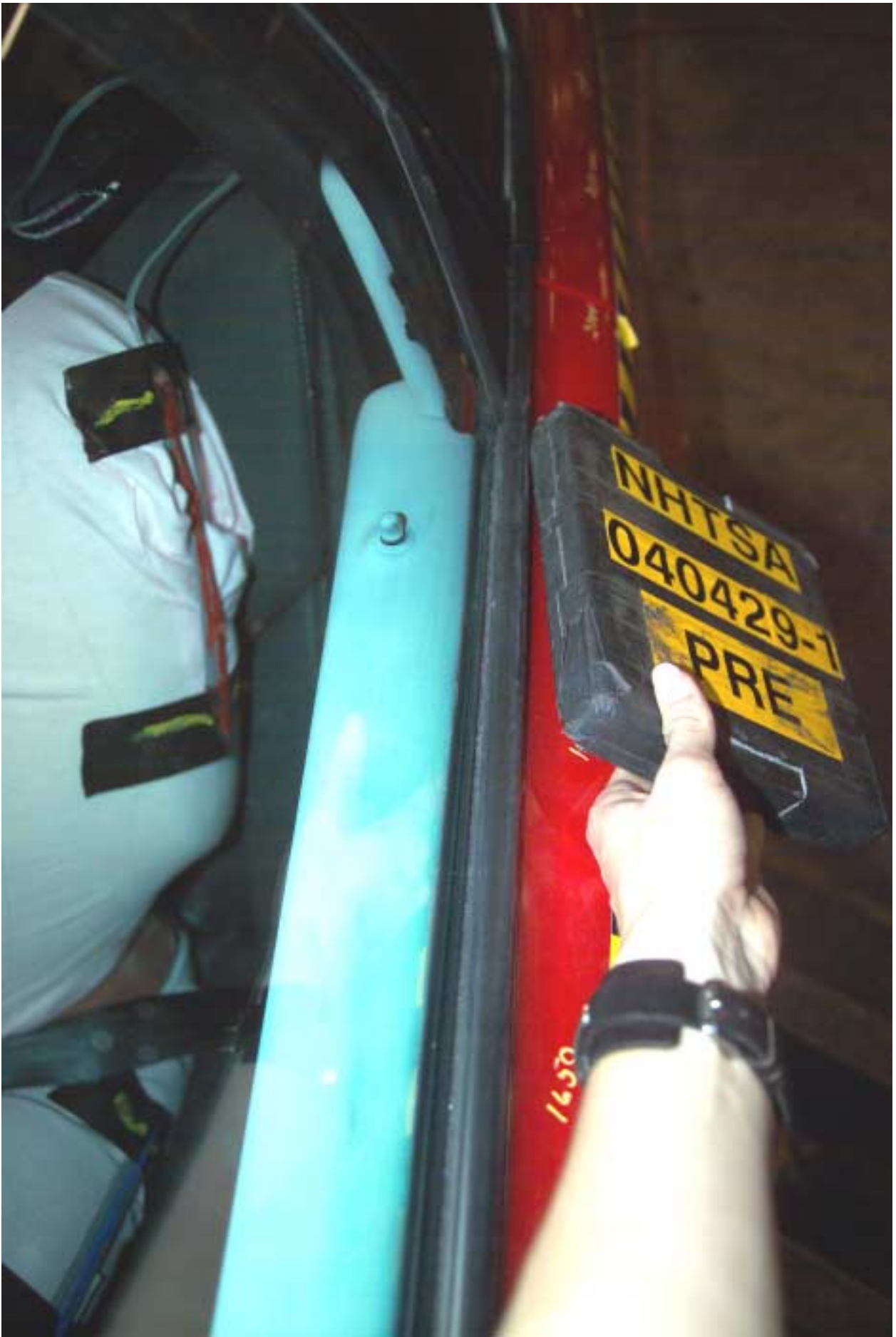
Figure A-30 Pre-Test View of Rear SID HIII and Door Clearance
