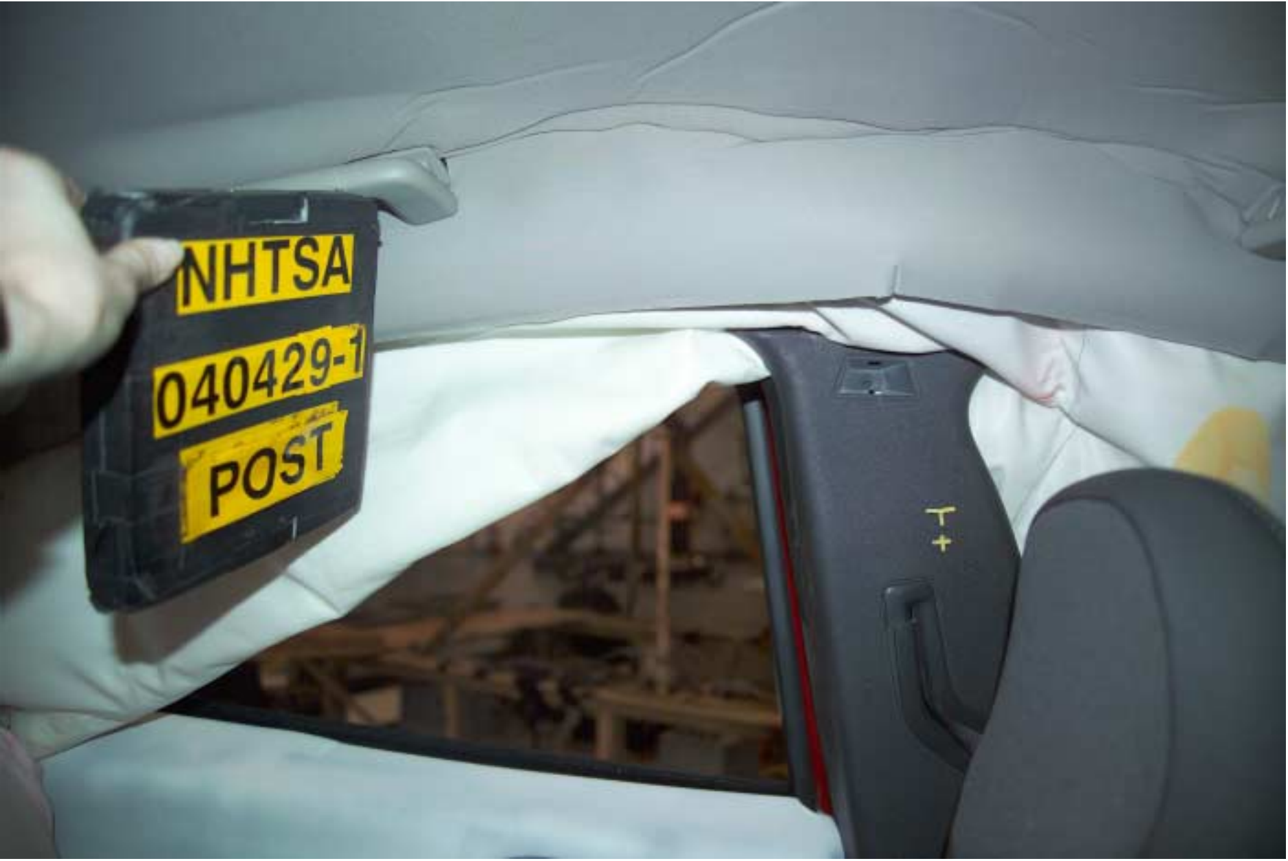
Figure A-55 Post-Test Side Curtain Airbag Deployment - View 1 A-58
