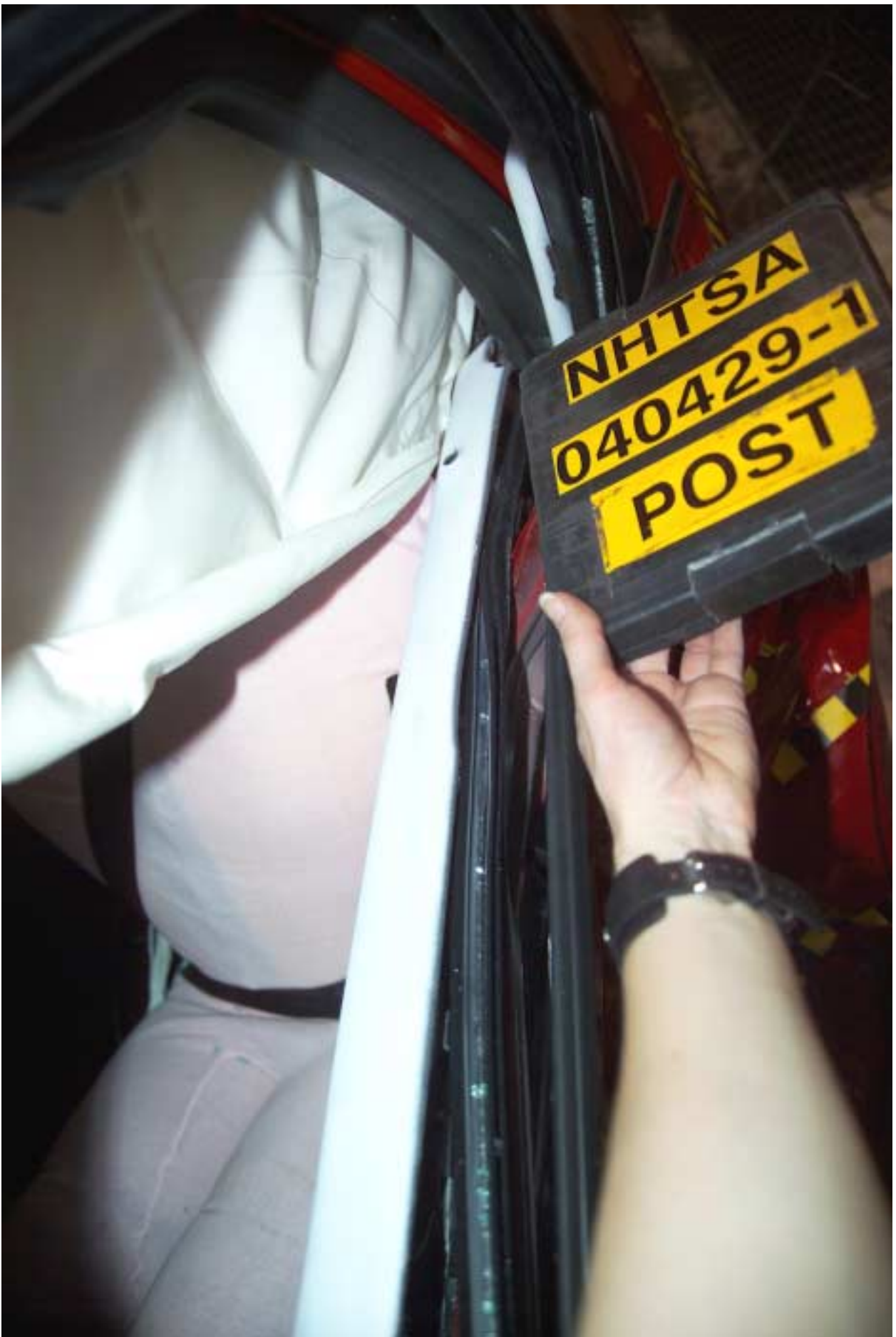
Figure A-31 Post-Test View of Rear SID HIII and Door Clearance
