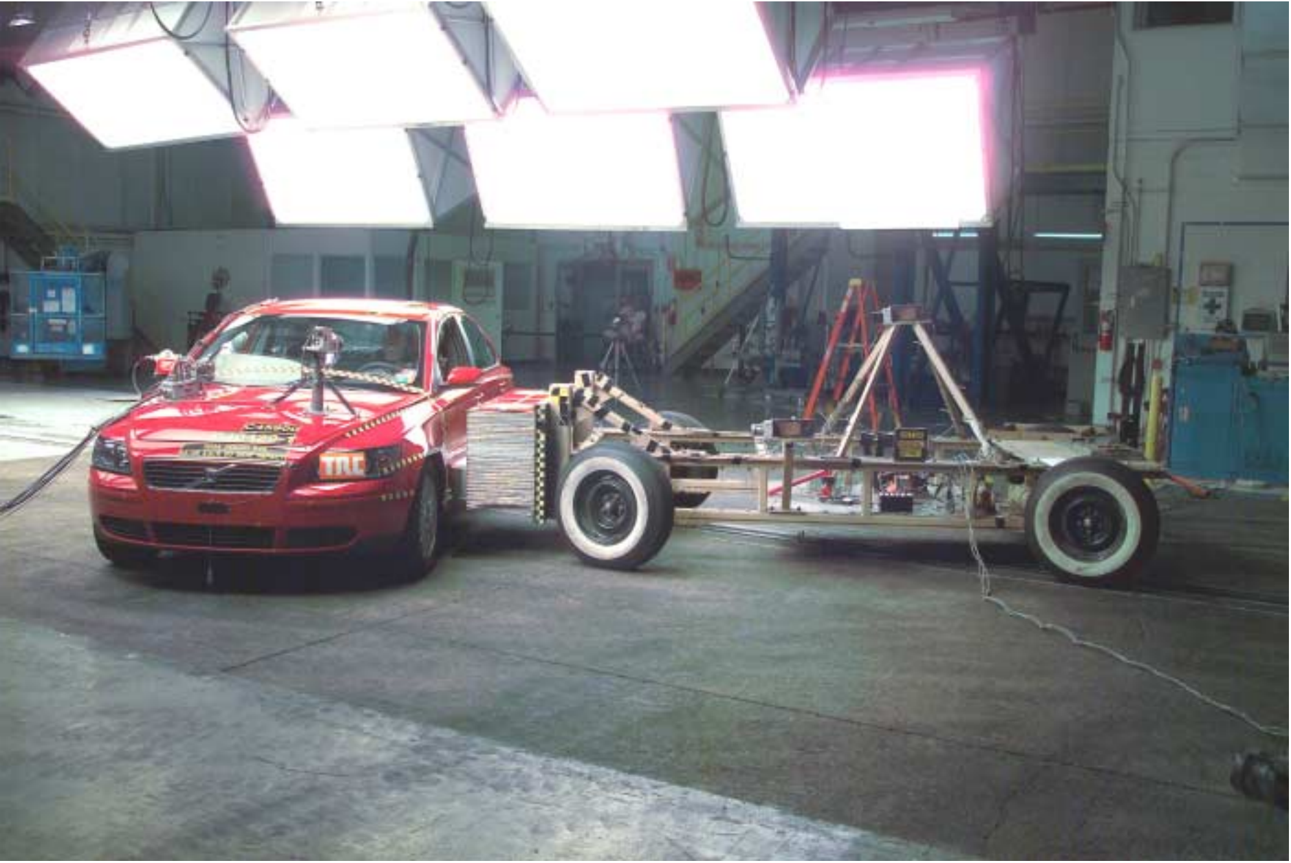
Figure A-41 Pre-Test Left Side View of MDB With Impactor Face in Position A-44
