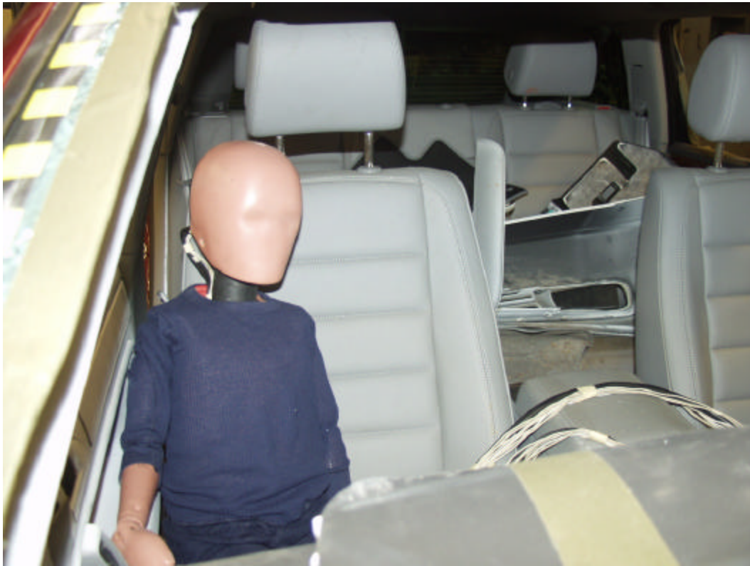
Figure A-5: Pre-Test Frontal View of Dummy
