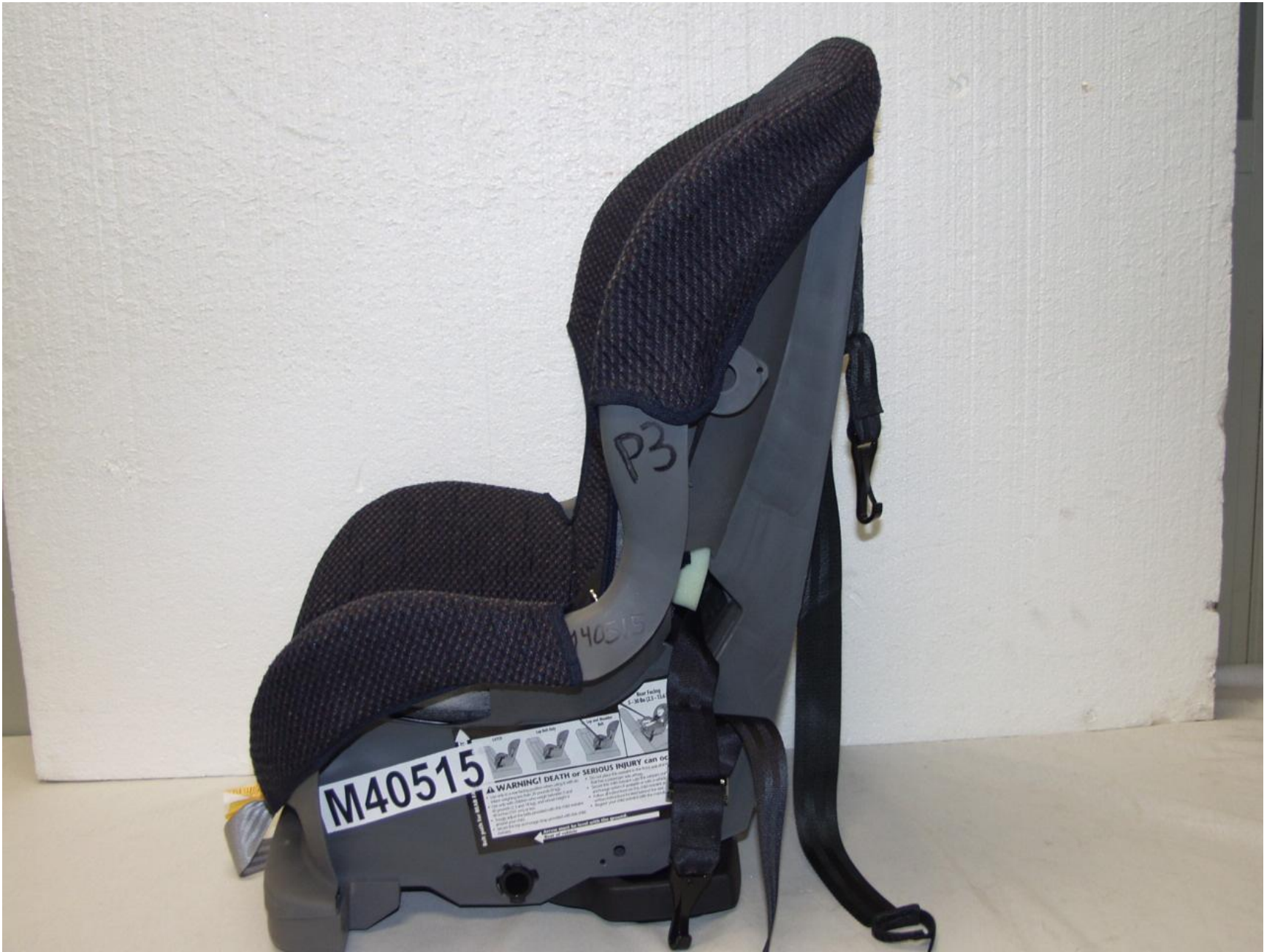
Figure 3-7: POST-TEST LEFT SIDE VIEW OF POSITION 3 CRS
