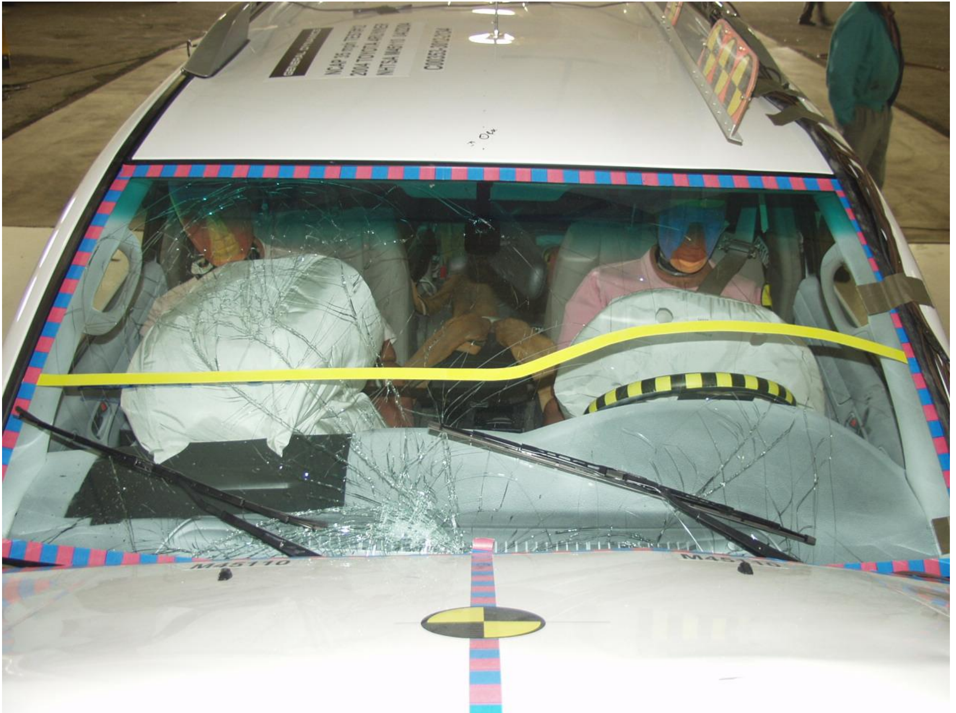
Figure A-19 POST-TEST WINDSHIELDVIEW
