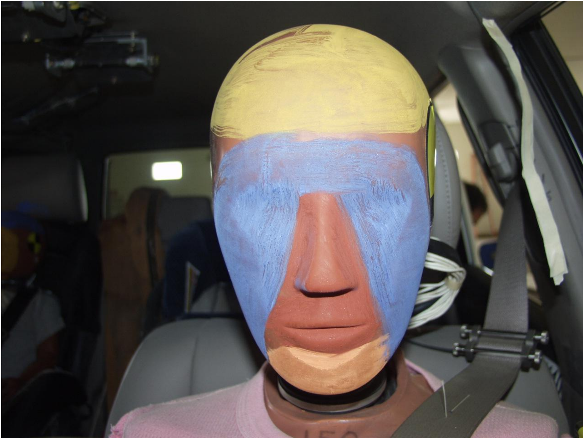
Figure A-42 POST-TEST DRIVER HEAD VIEW
