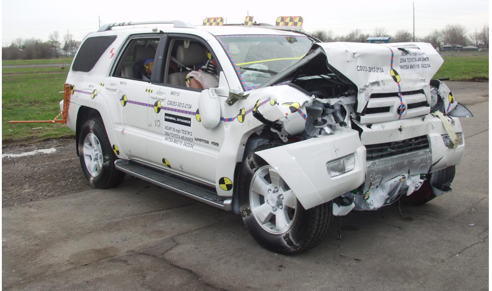
Figure A-13 POST-TEST RIGHT FRONT THREE-QUARTER VIEW
