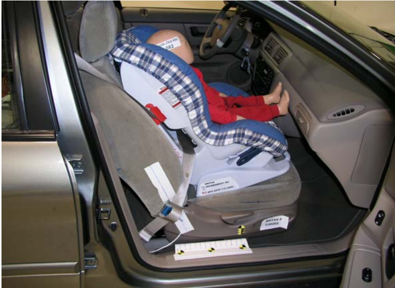
Britax Roundabout Fwd Facing With Belt Forward No Blanket
