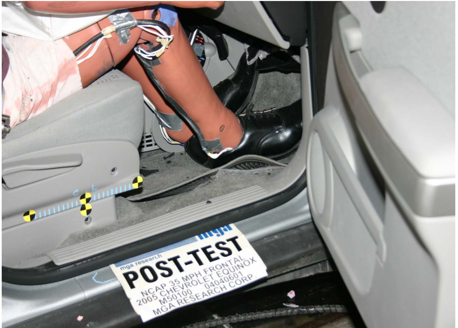
Post-Test Passenger Dummy Feet Position
