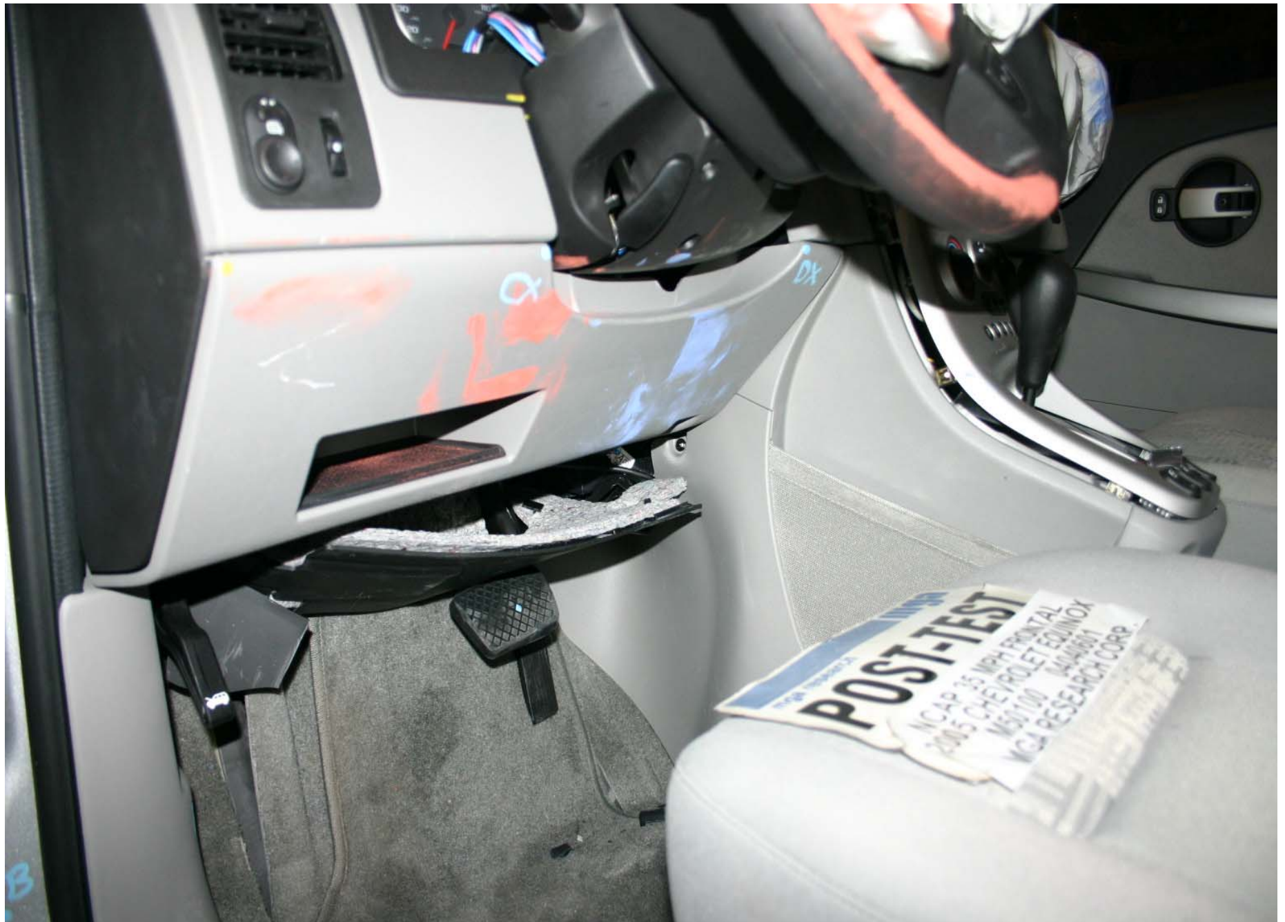
Post-Test Driver Dummy Knee Contact
