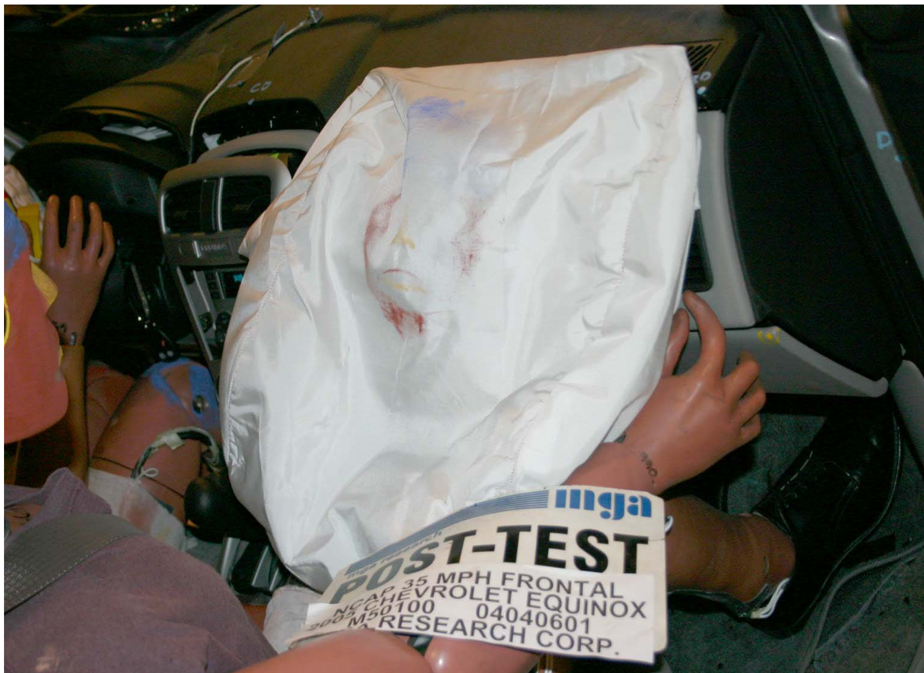
Post-Test Passenger Dummy Airbag Contact
