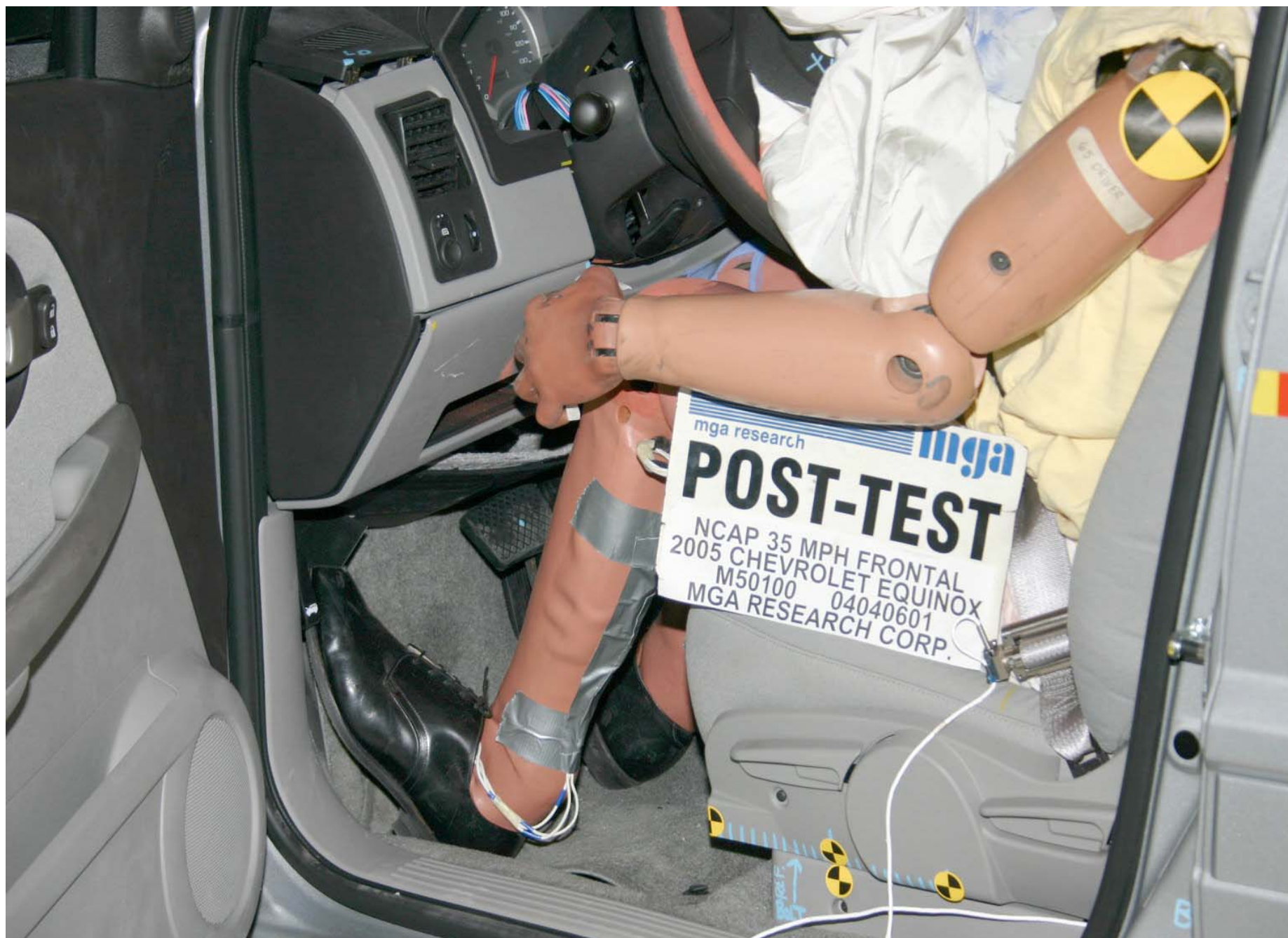
Post-Test Driver Side Knee Bolster View
