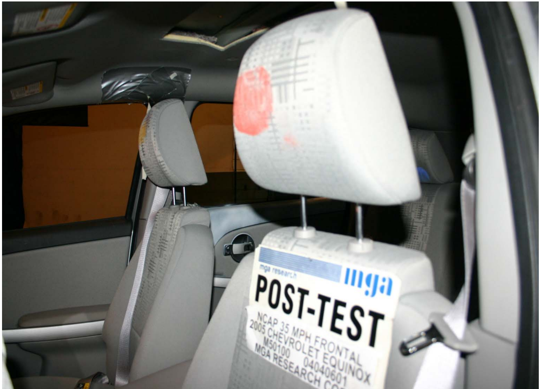
Post-Test Driver Dummy Head Contact
