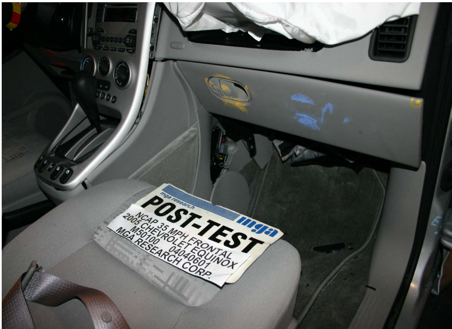
Post-Test Passenger Dummy Knee Contact
