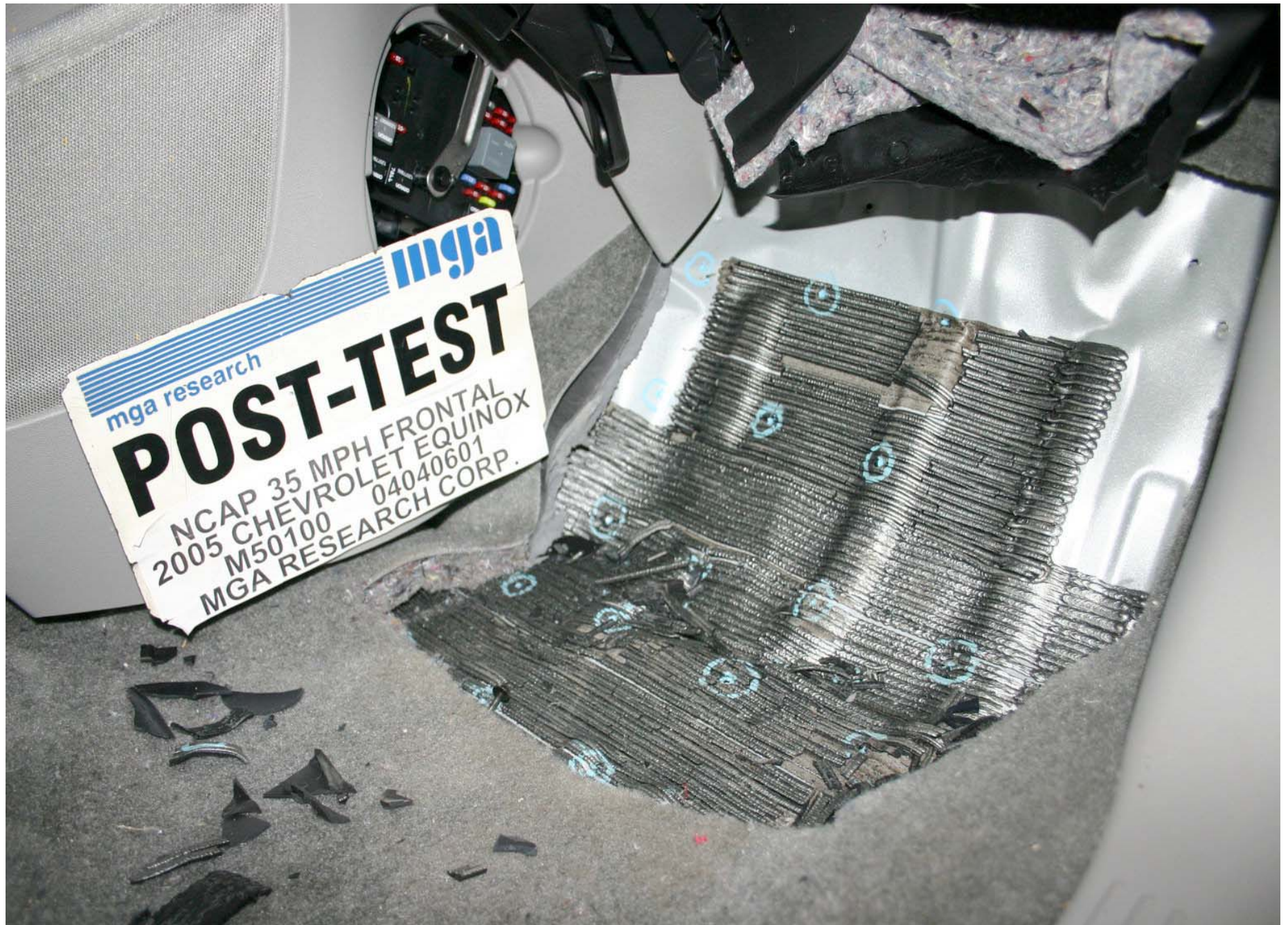
Post-Test Passenger Side Floor Pan View
