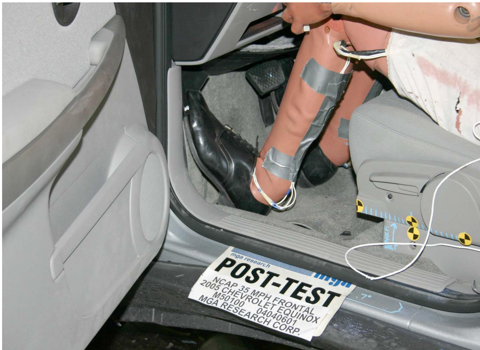
Post-Test Driver Dummy Feet Position
