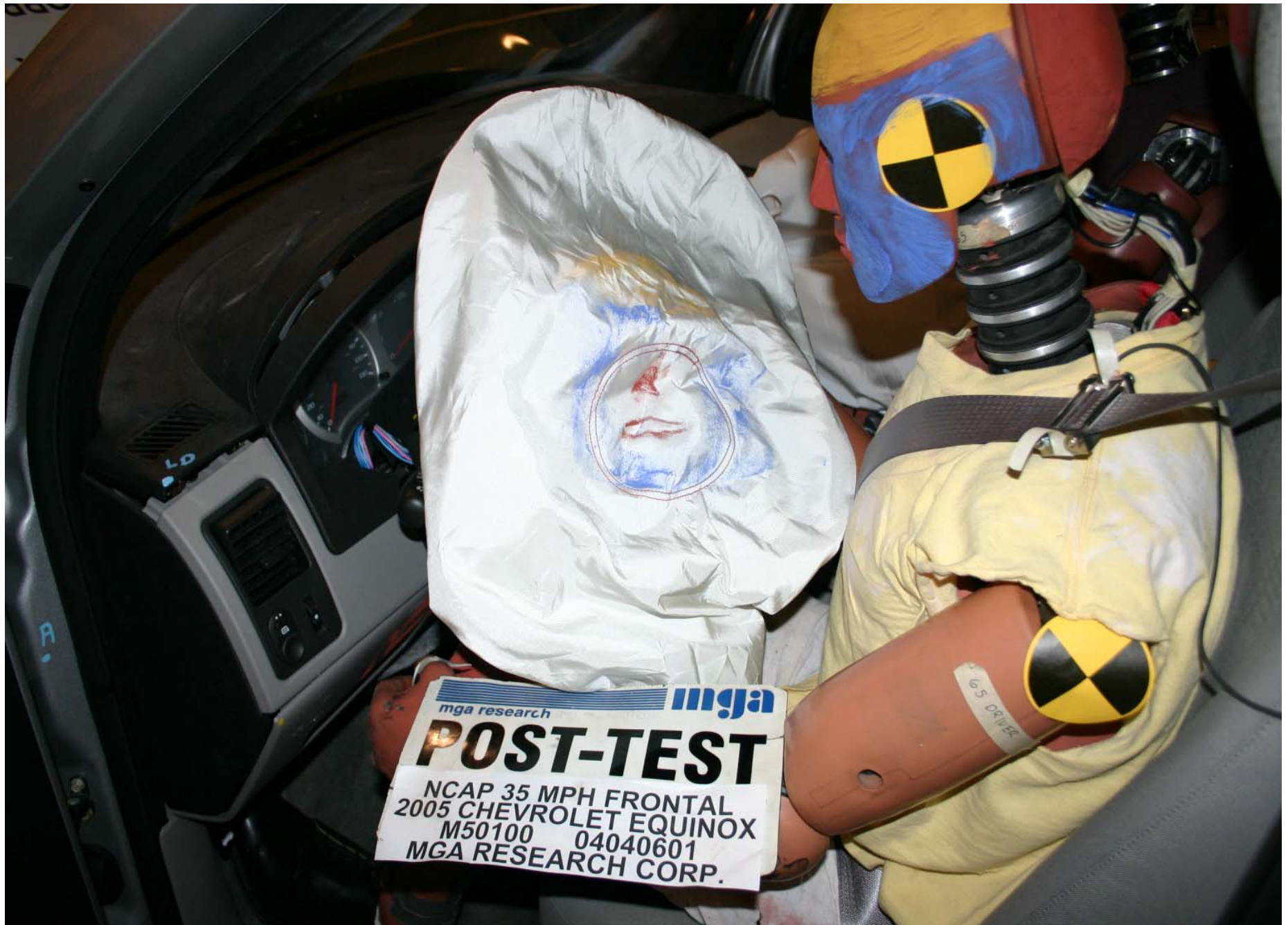
Post-Test Driver Dummy Airbag Contact
