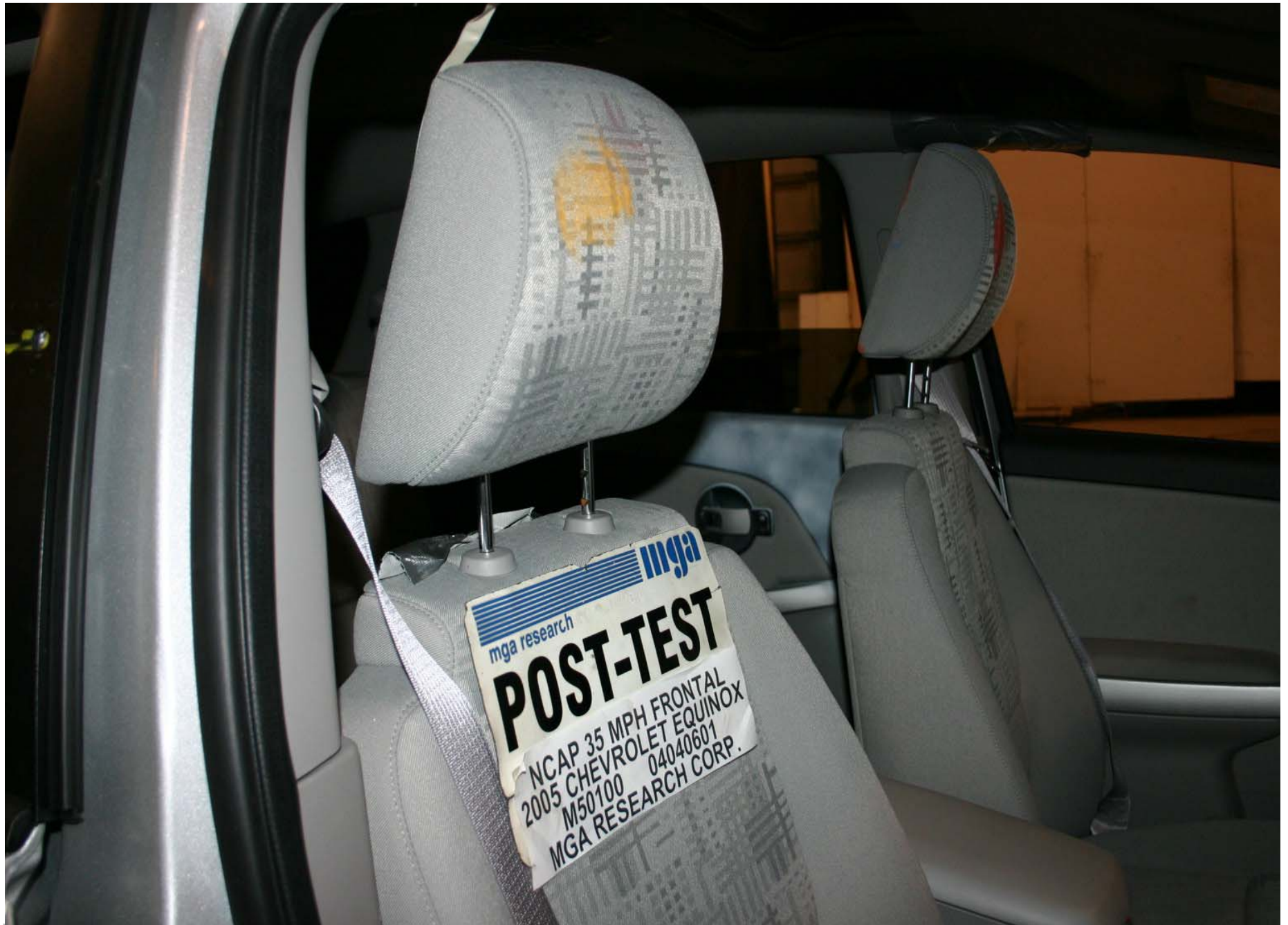
Post-Test Passenger Dummy Head Contact
