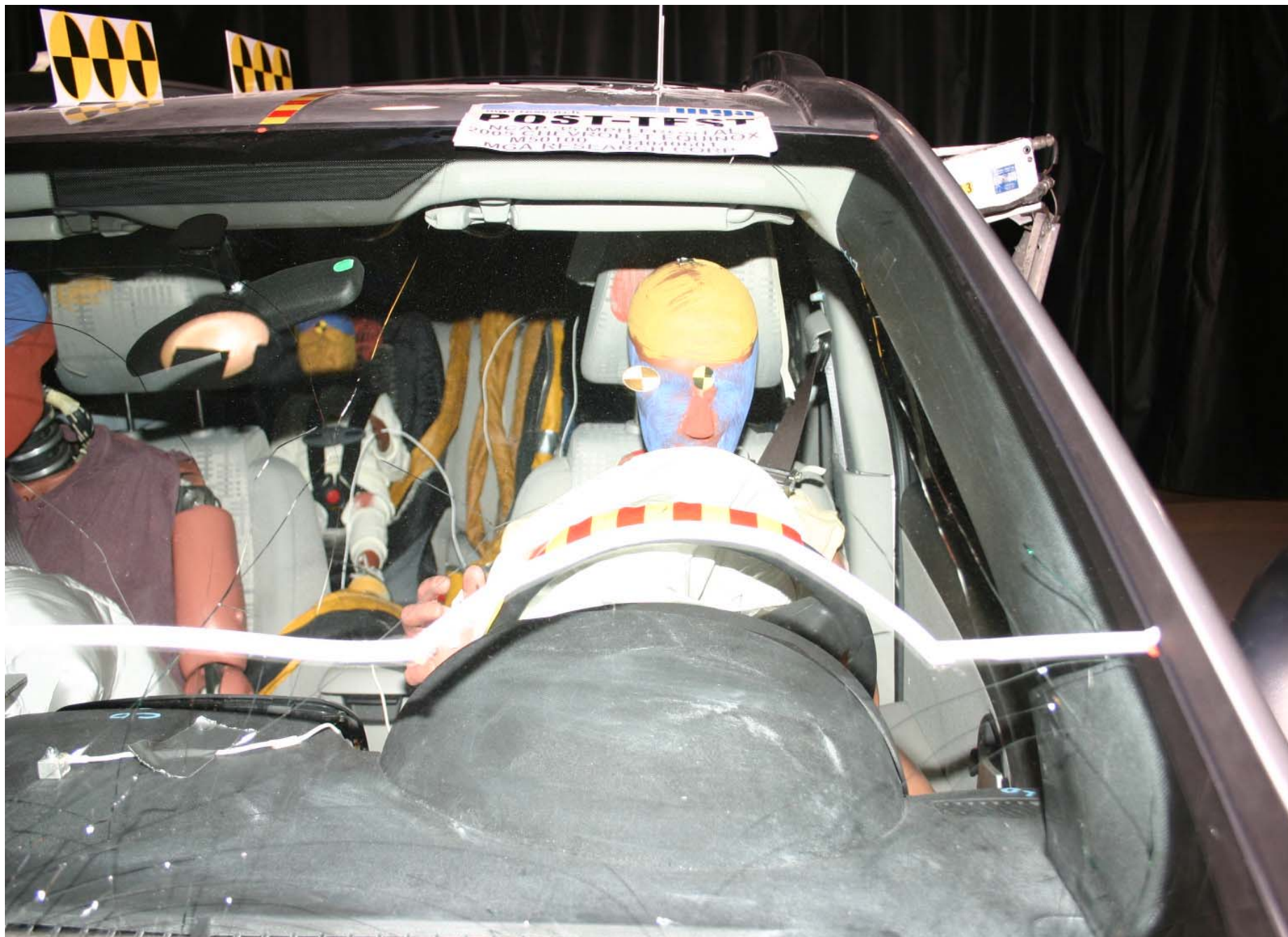
Post-Test Driver Dummy Front View (head position)
