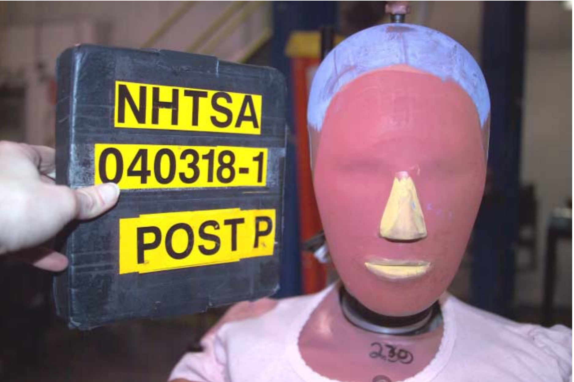
Figure A-49 Post-Test Passenger Dummy Head Contact - View 1 7-53
