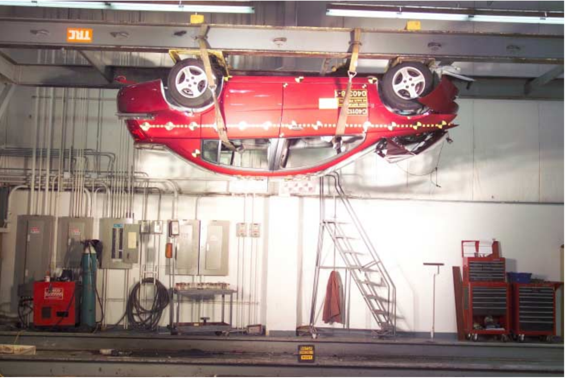
Figure A-56 Post-Test Vehicle on Static Rollover Device - 180° View 7-60
