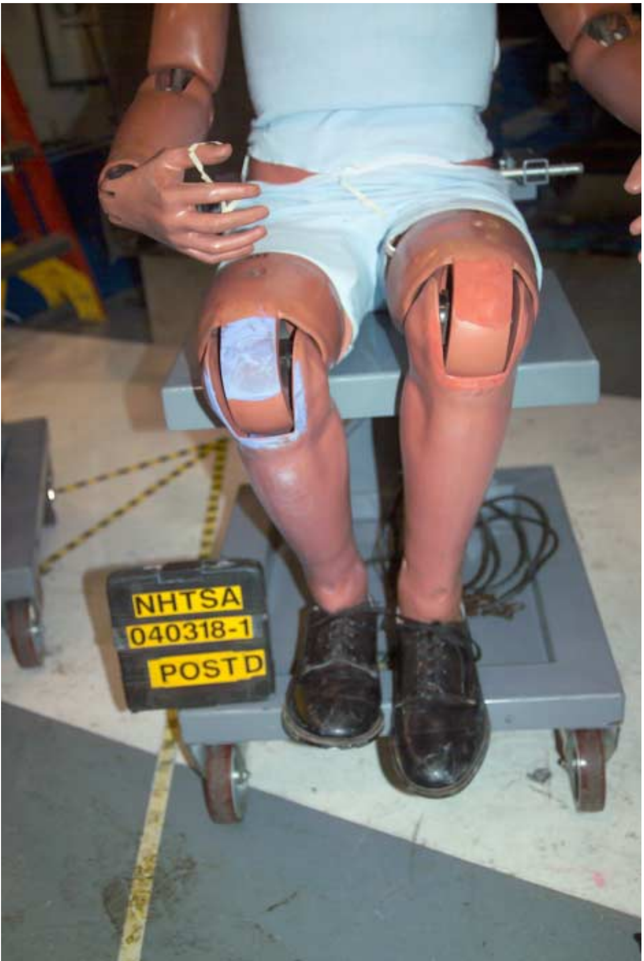
Figure A-46 Post-Test Driver Dummy Knee Contact - View 1
