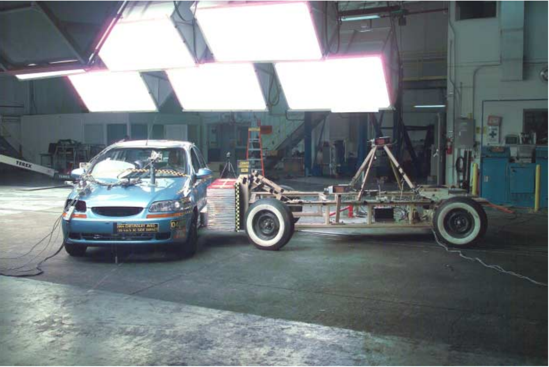
Figure A-39 Pre-Test Left Side View of MDB With Impactor Face in Position A-42
