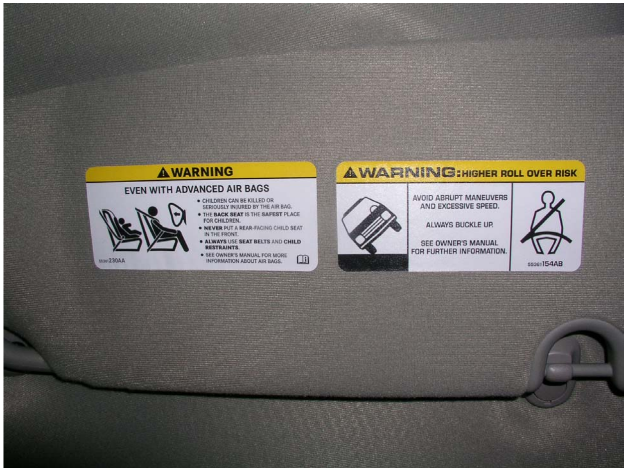
2004 Dodge Durango MPV S.4.5.1 Air Bag Labeling Failure (Data Sheet 5 – 3.6.3)
