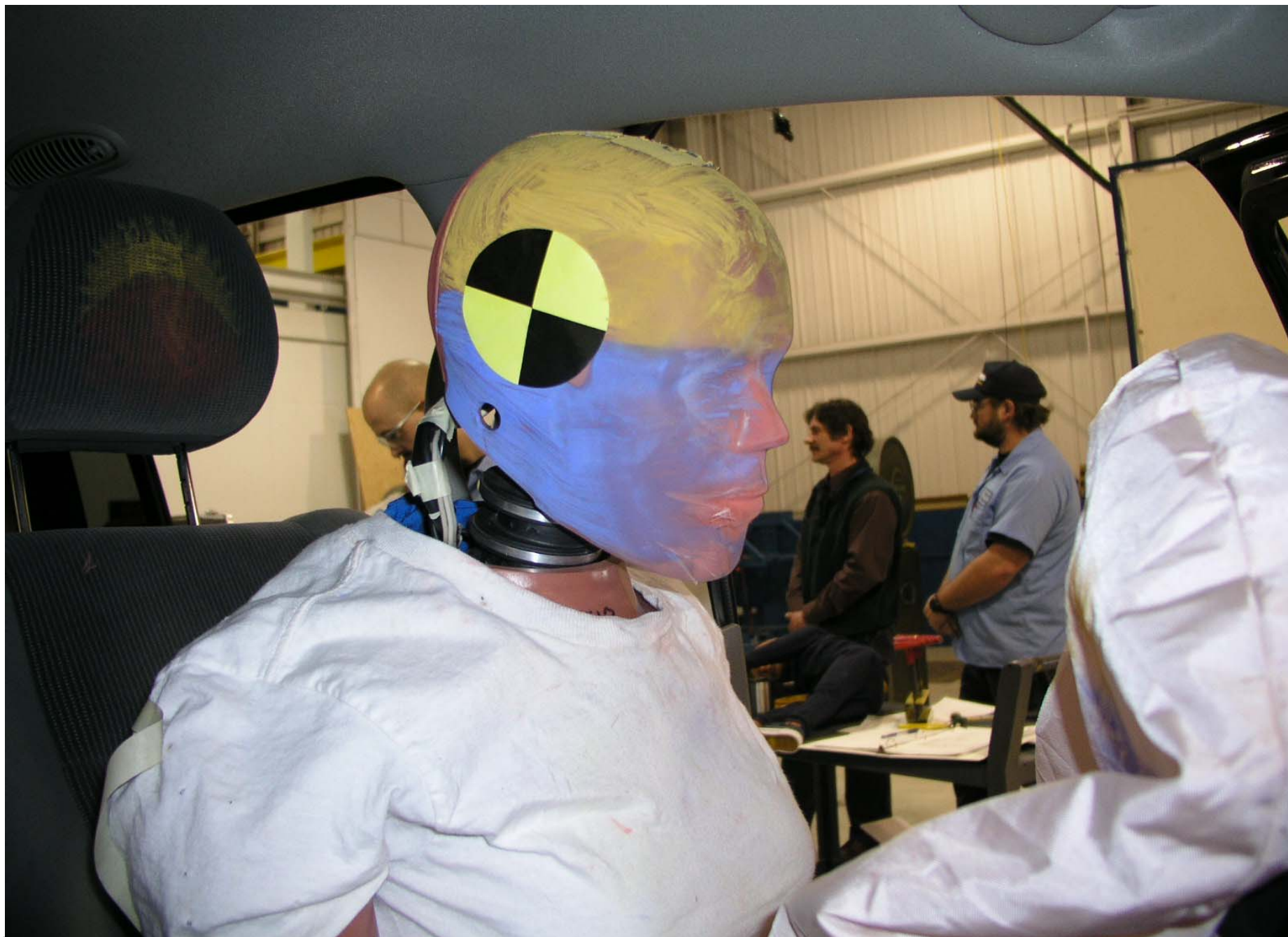
Post-Test 5th Fem. P1 Driver Dummy Right Side Head Contact View
