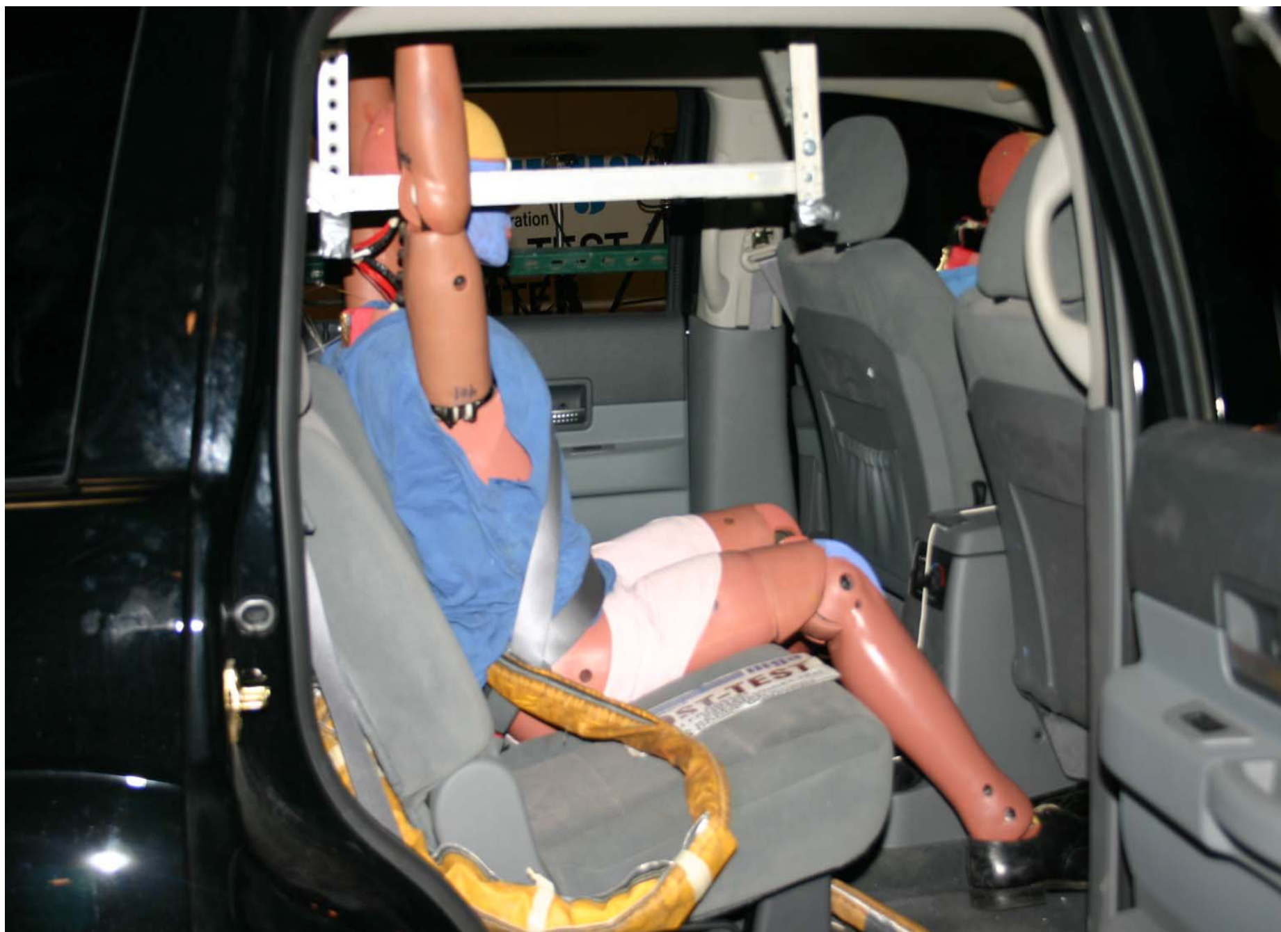
Post-Test CRP Dummy Position Right Side View (Door Open)
