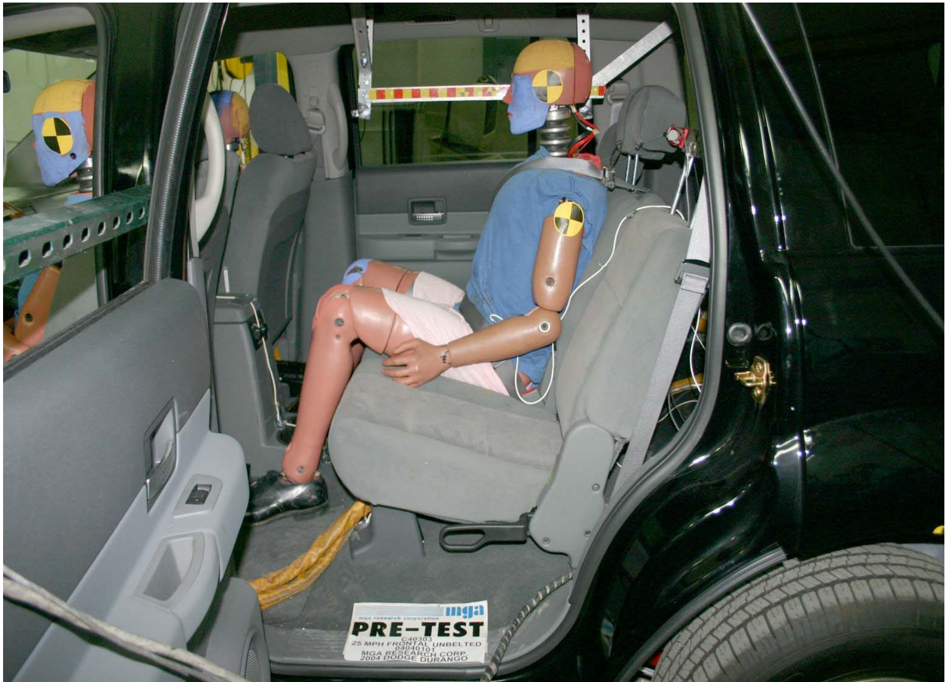
Pre-Test CRP Dummy Position Left Side View (Door Open)
