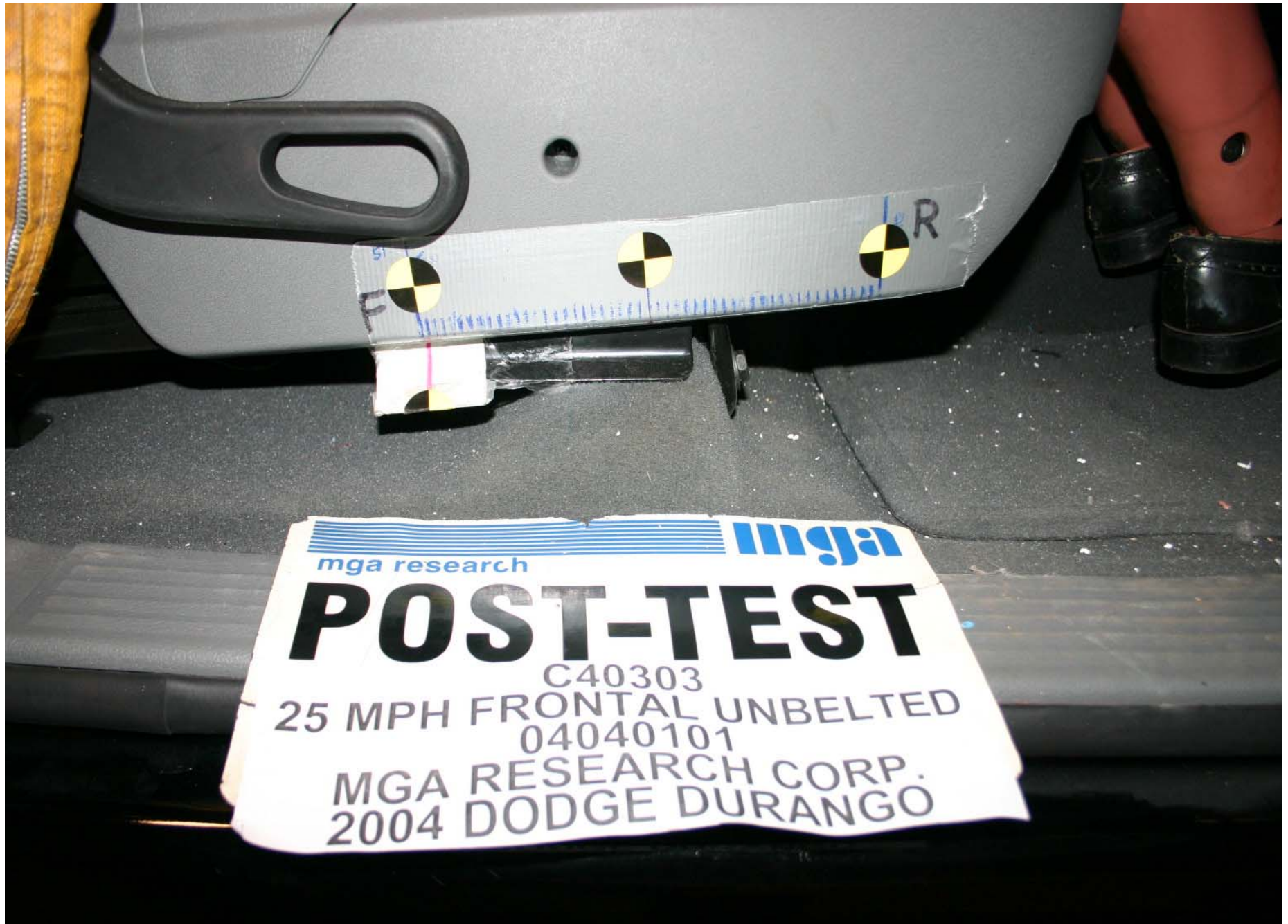
Post-Test Passenger Dummy Seat Position
