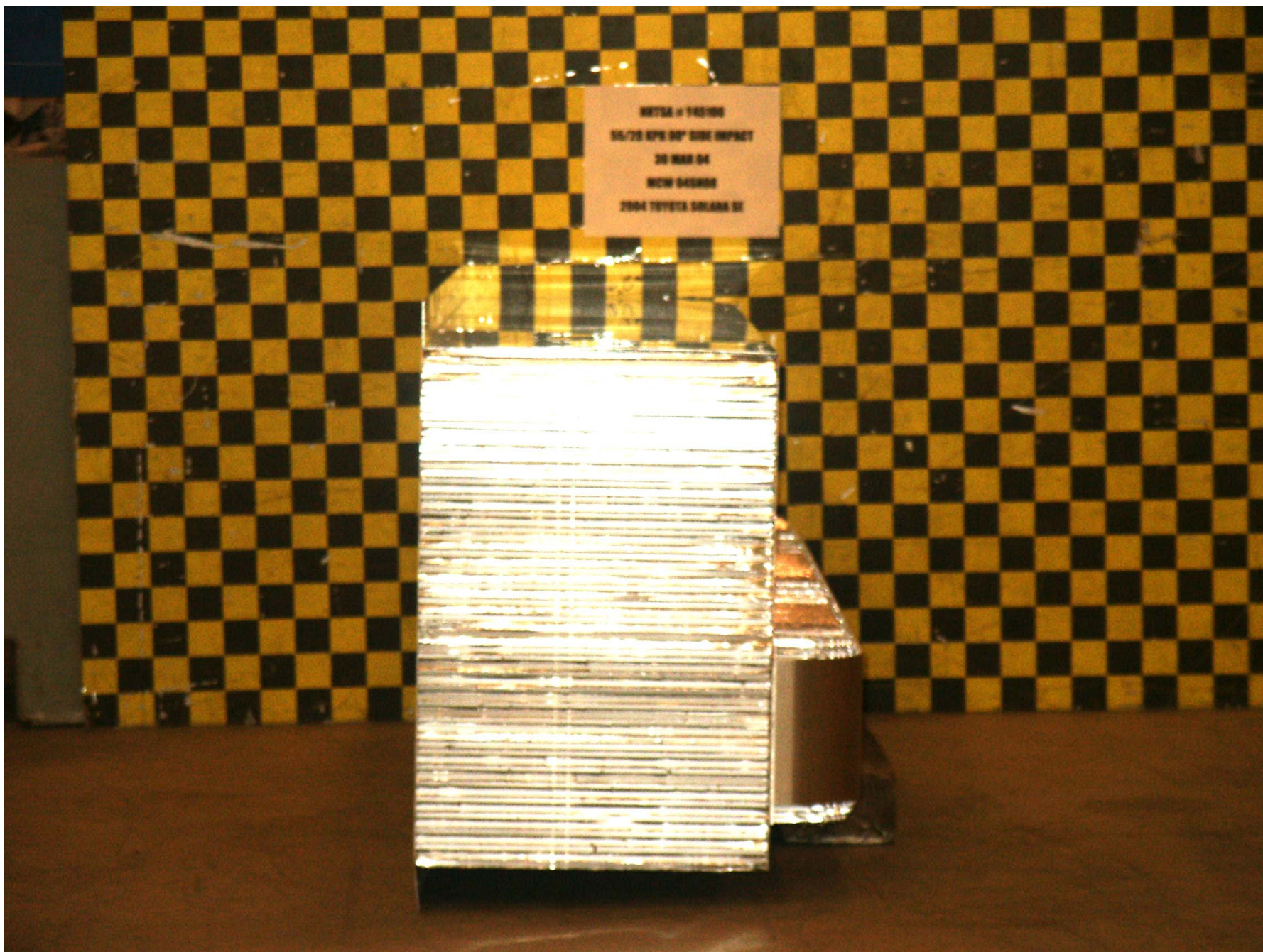
Figure A-51: PRE-TEST ALUMINUM BARRIER RIGHT SIDE
