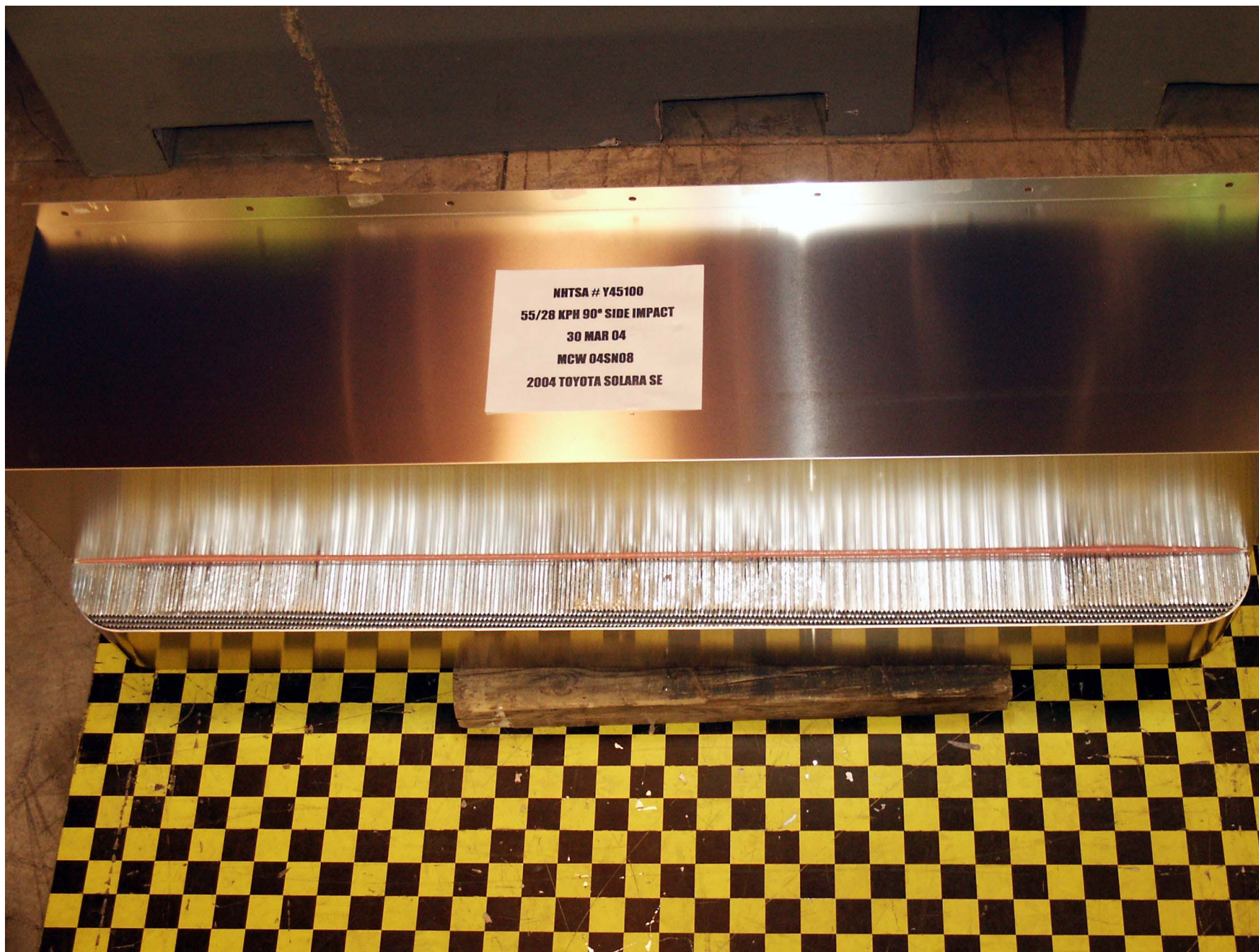
Figure A-53: PRE-TEST ALUMINUM BARRIER TOP
