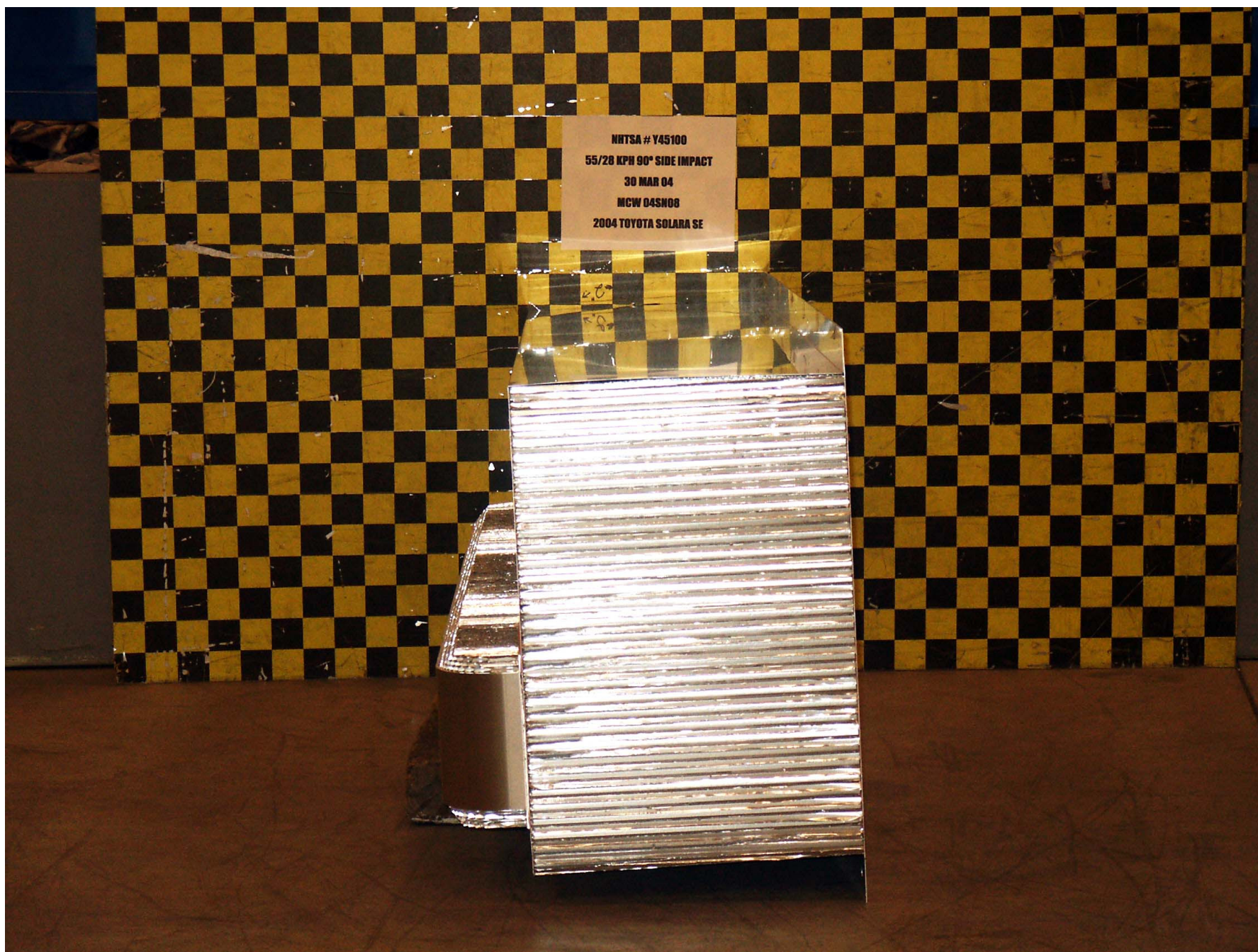
Figure A-49: PRE-TEST ALUMINUM BARRIER LEFT SIDE
