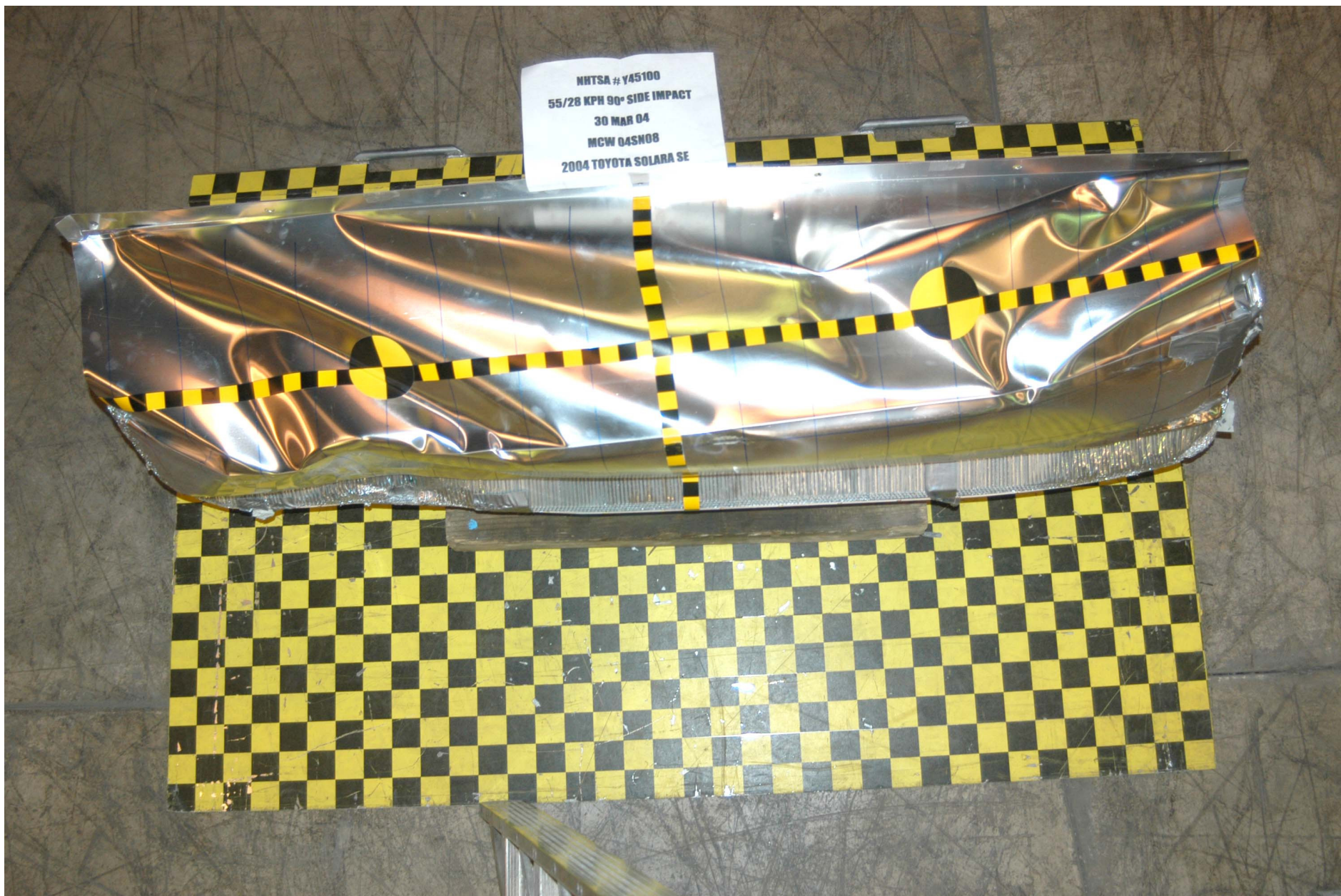
Figure A-54: POST-TEST ALUMINUM BARRIER TOP
