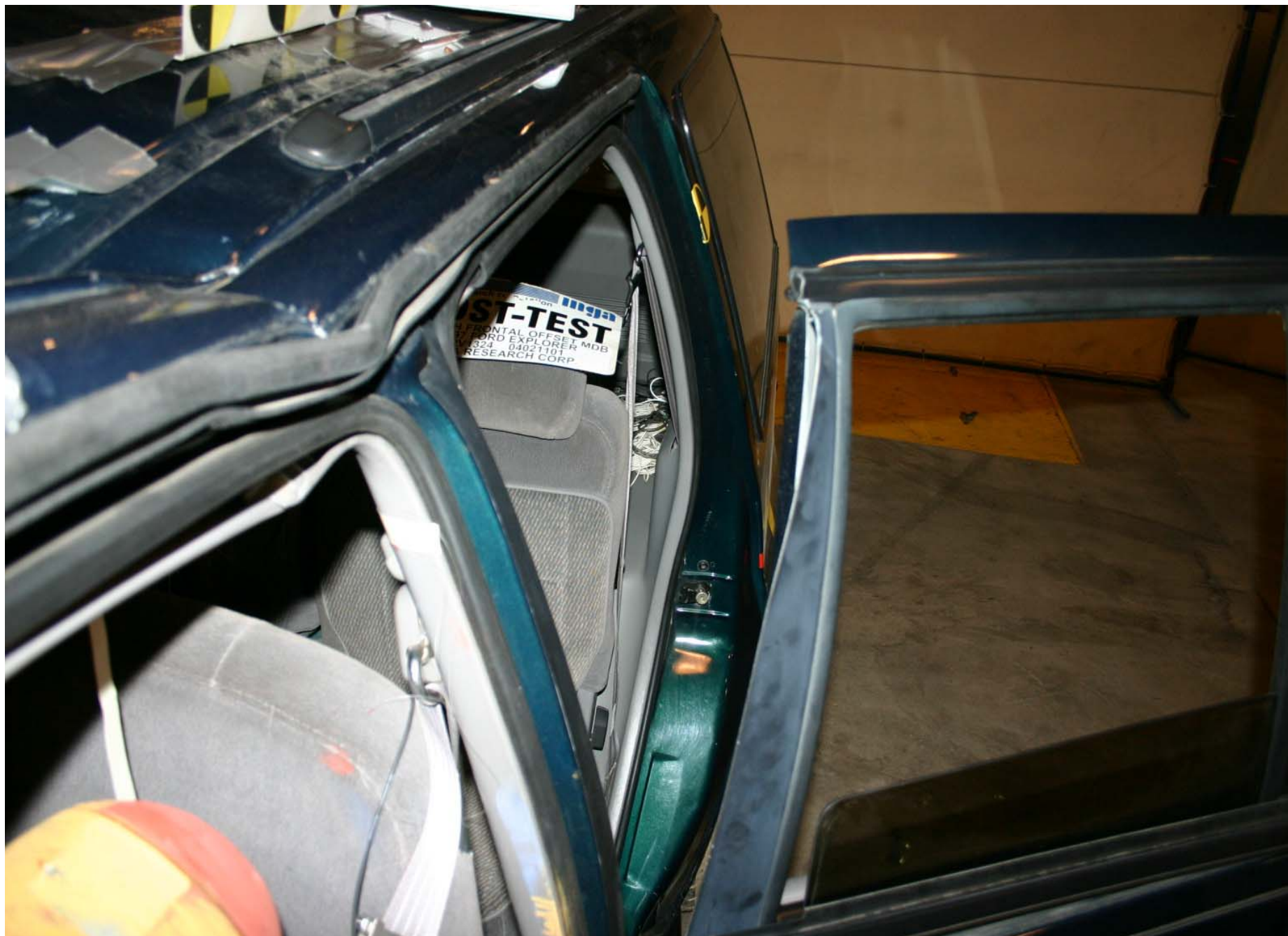
Post-Test Driver Dummy Head Contact
