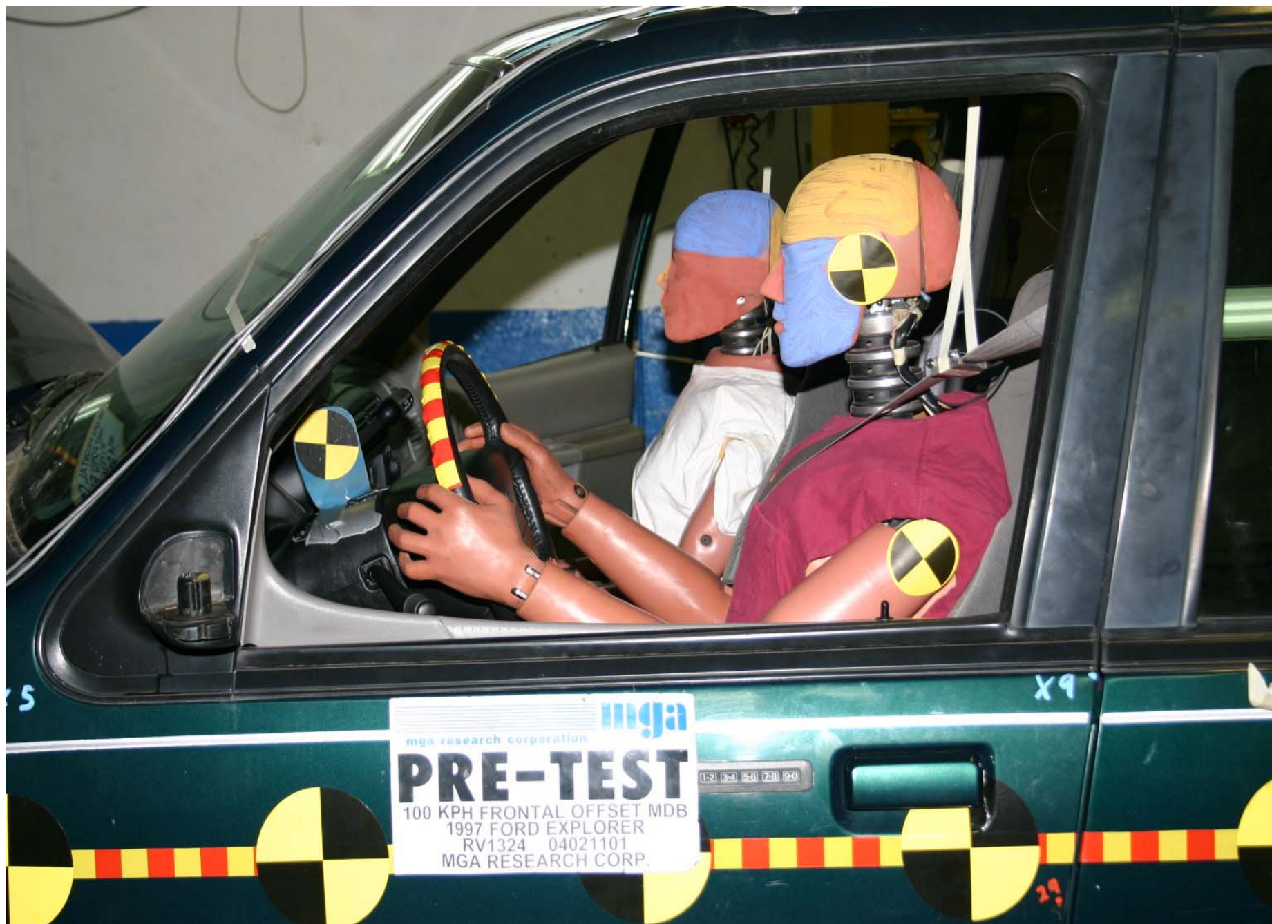
Pre-Test Driver Dummy Position Left Side View
