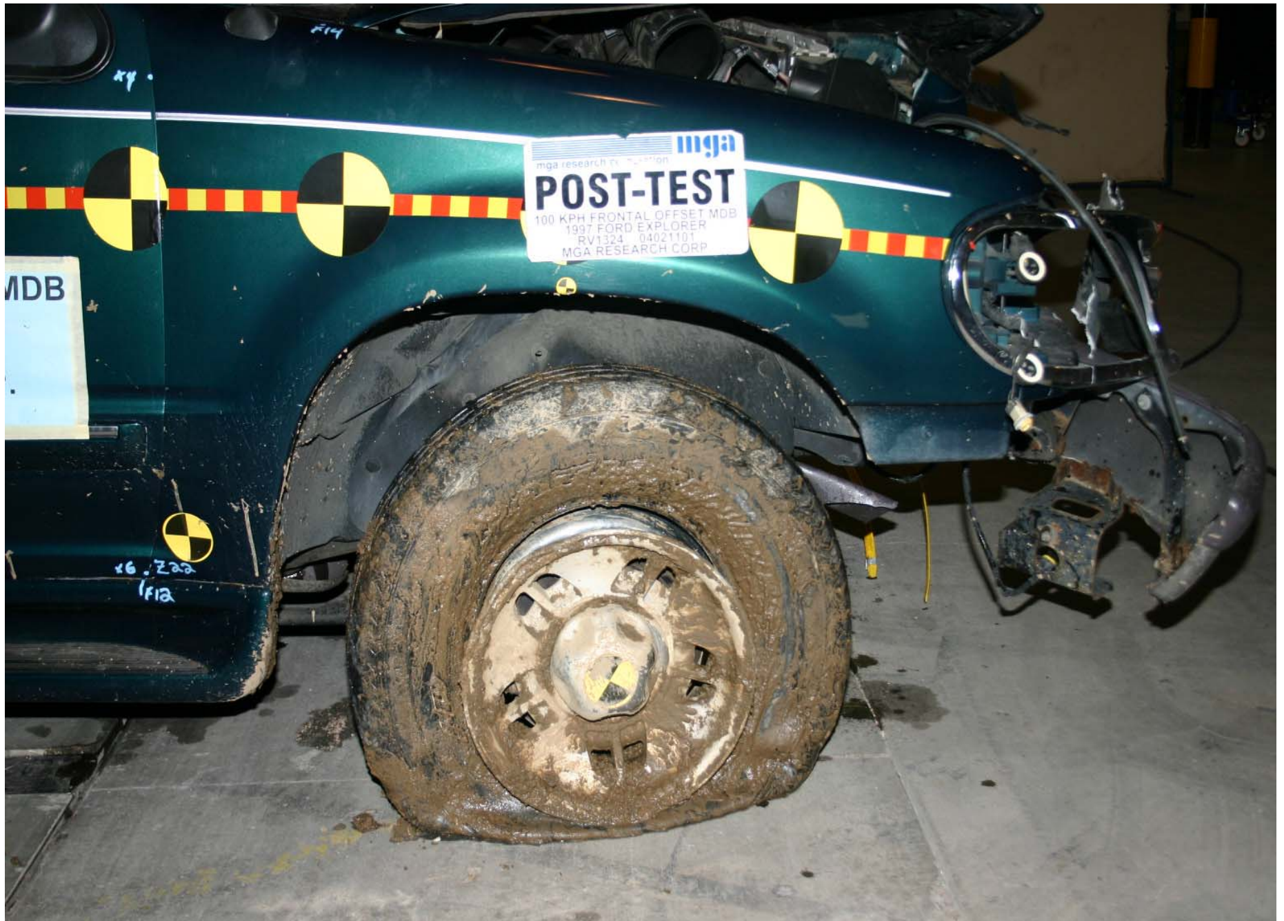
Post-Test Right Front Wheel Well
