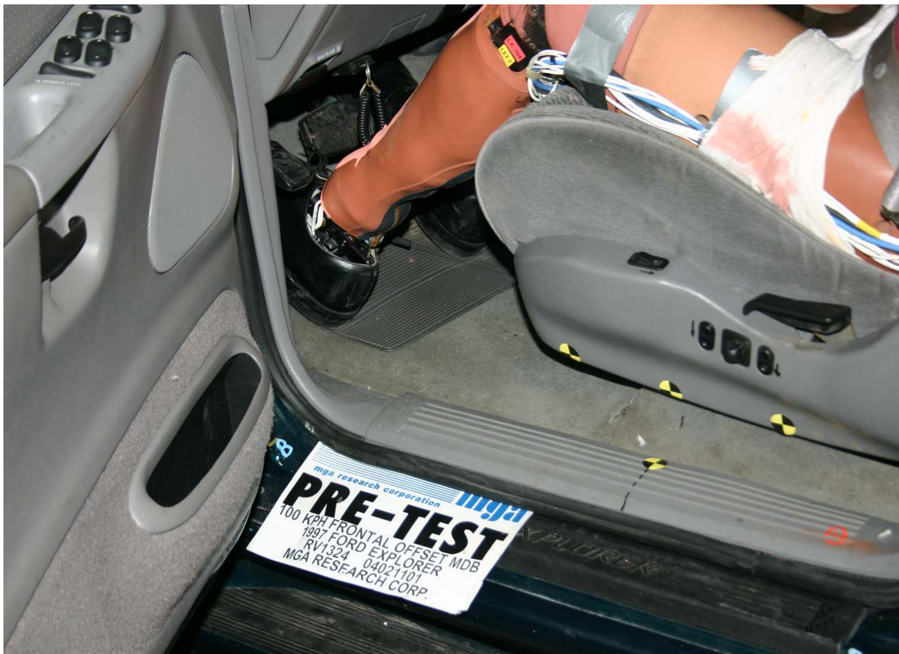
Pre-Test Driver Dummy Feet Position
