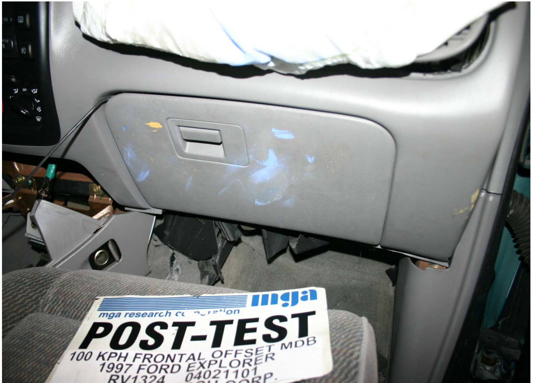
Post-Test Passenger Dummy Knee Contact
