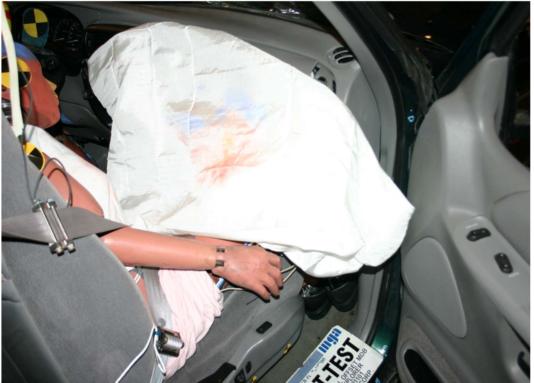
Post-Test Passenger Dummy Airbag Contact
