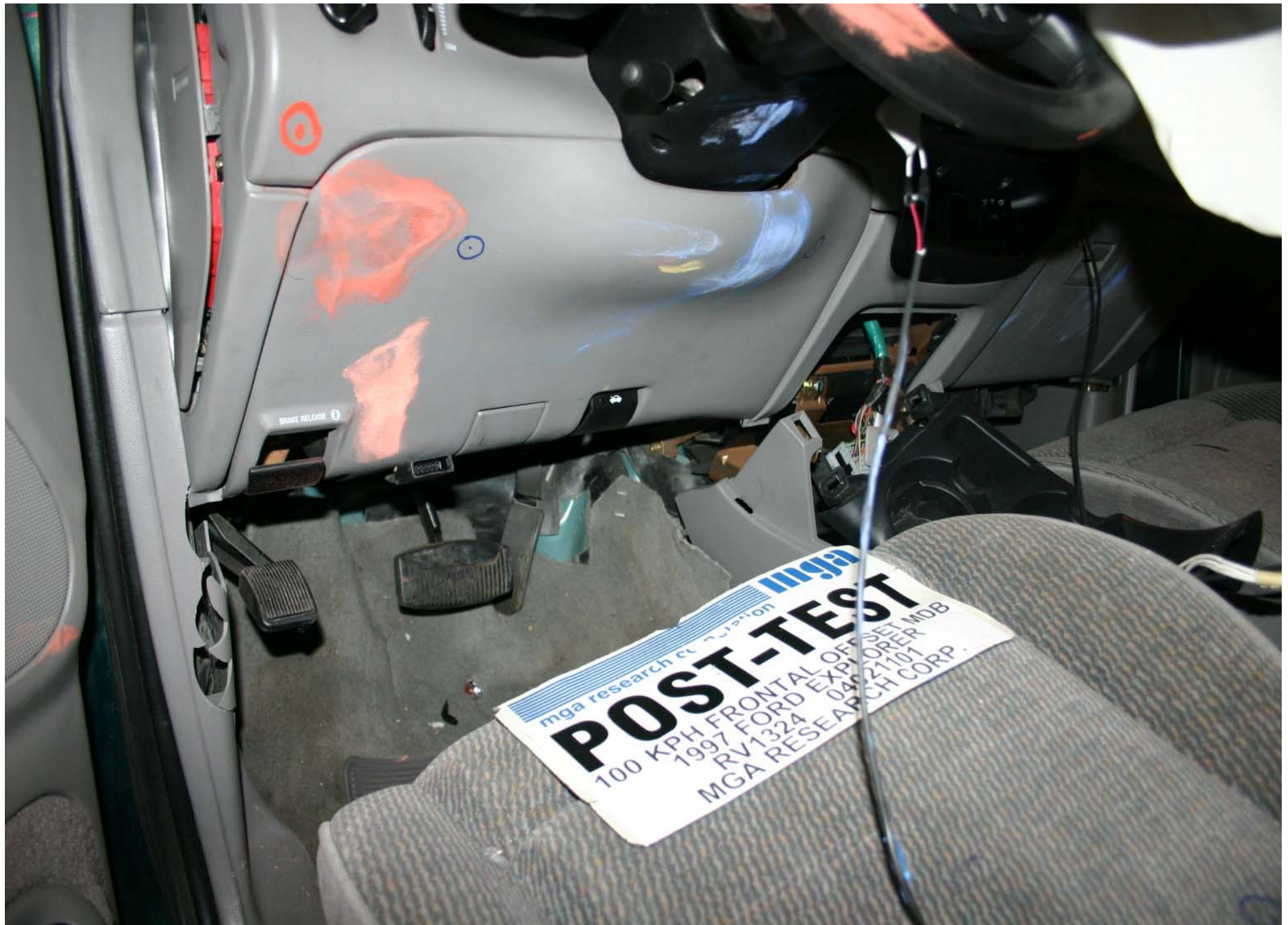
Post-Test Driver Dummy Knee Contact
