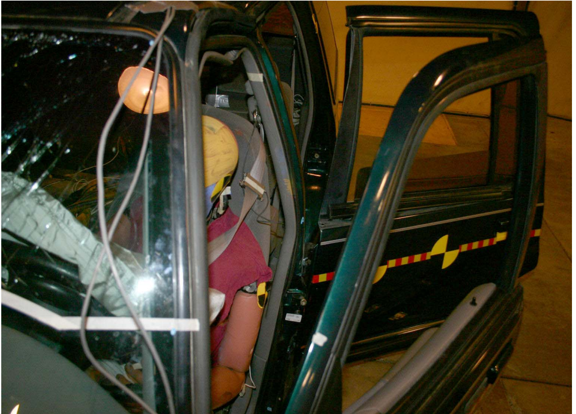
Post-Test Driver Dummy B Pillar Contact
