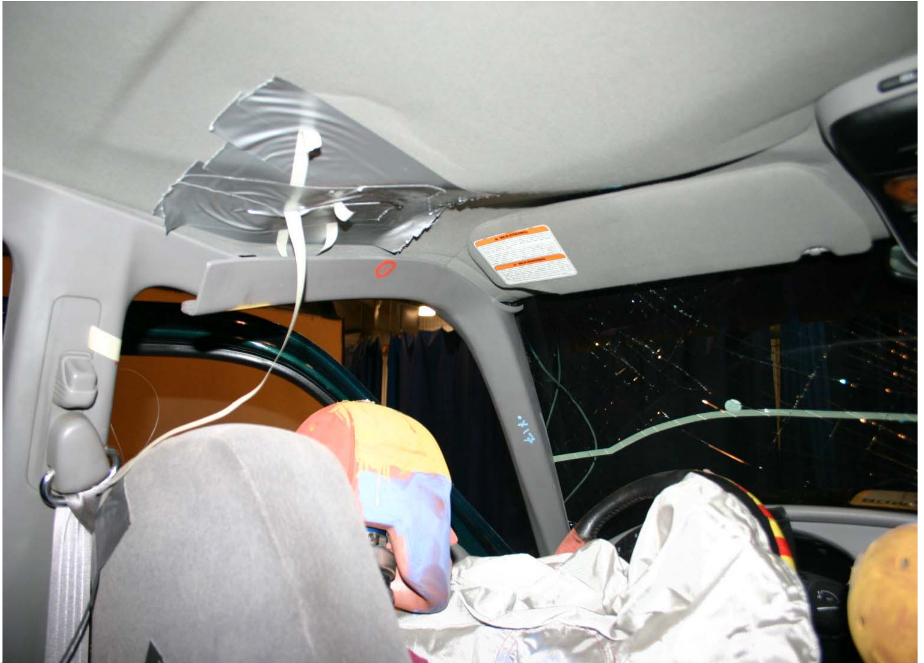
Post-Test Driver Dummy Head Contact
