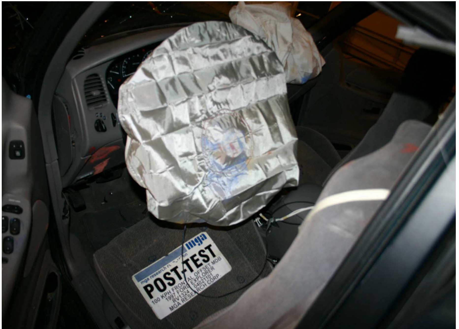
Post-Test Driver Dummy Airbag Contact
