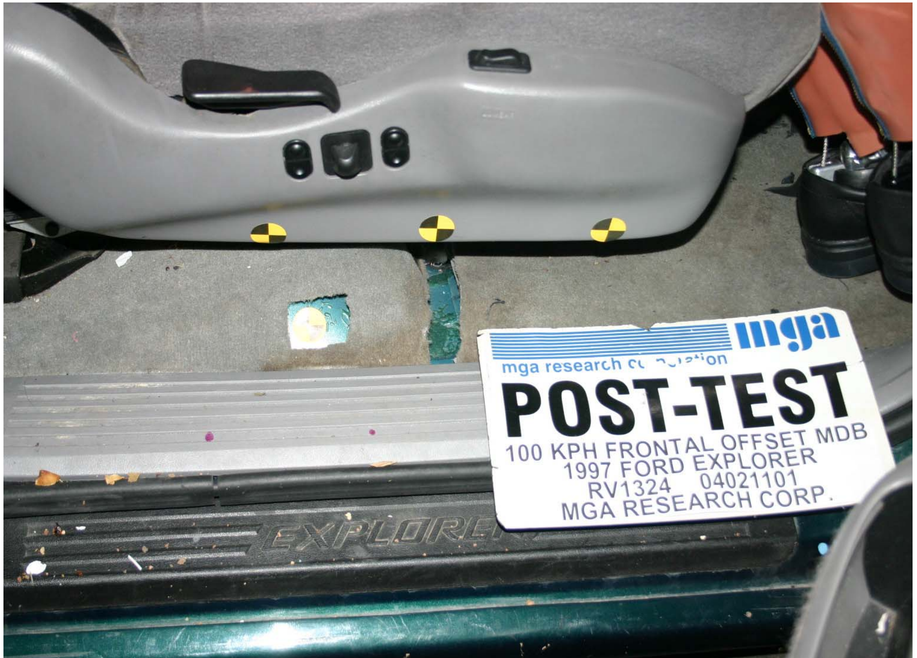
Post-Test Passenger Dummy Seat Position
