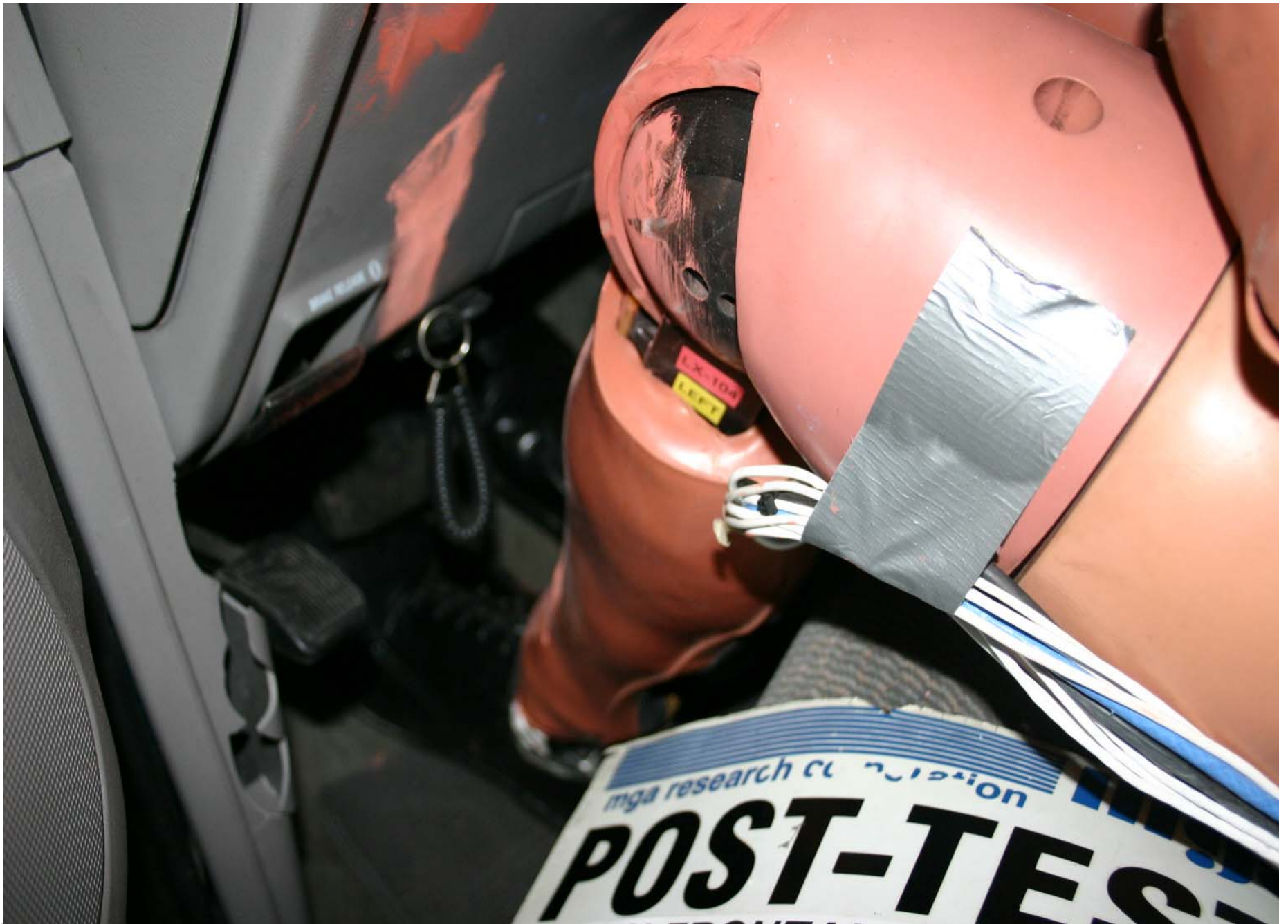
Post-Test Driver Dummy Feet Position
