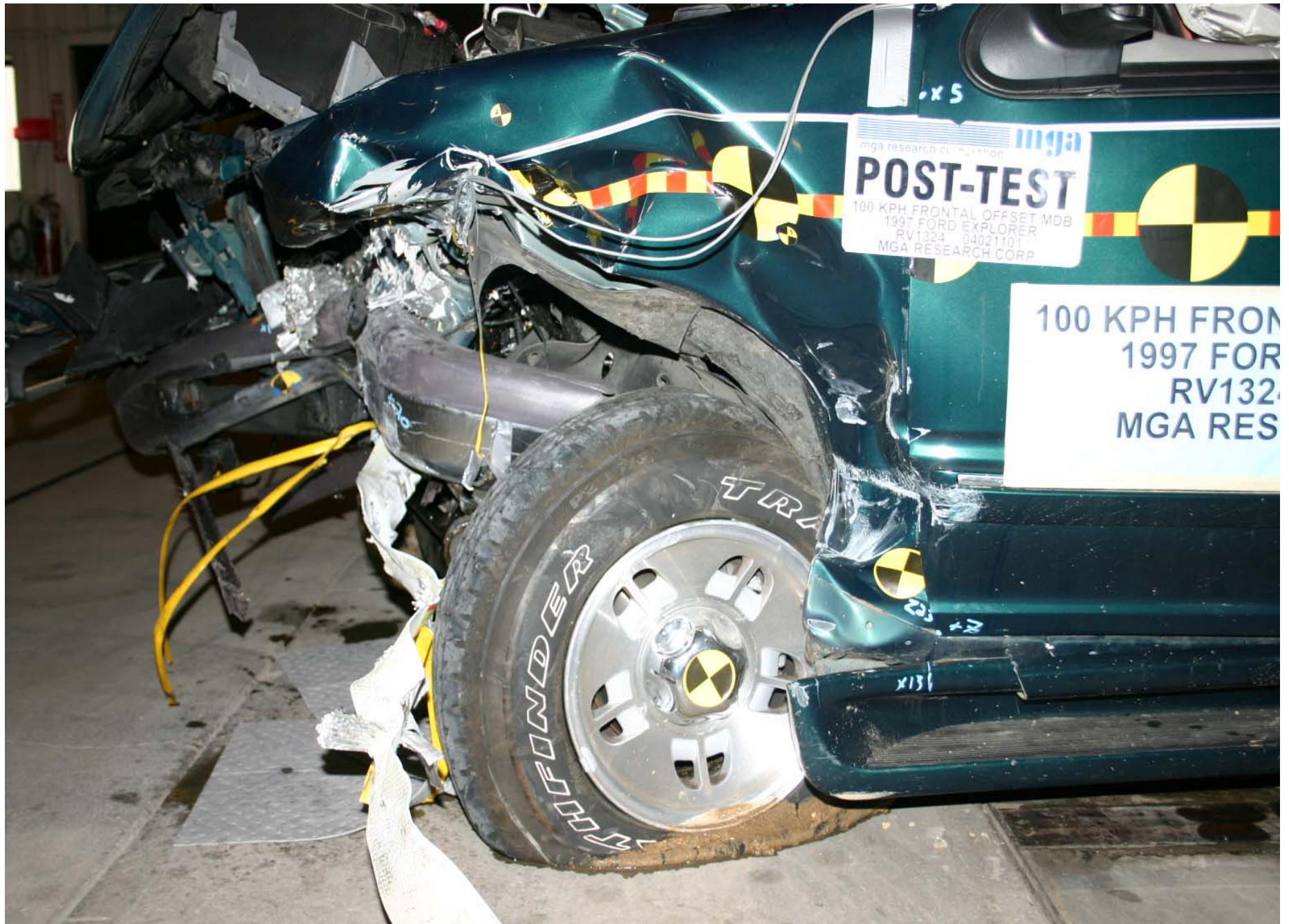
Post-Test Left Front Wheel Well
