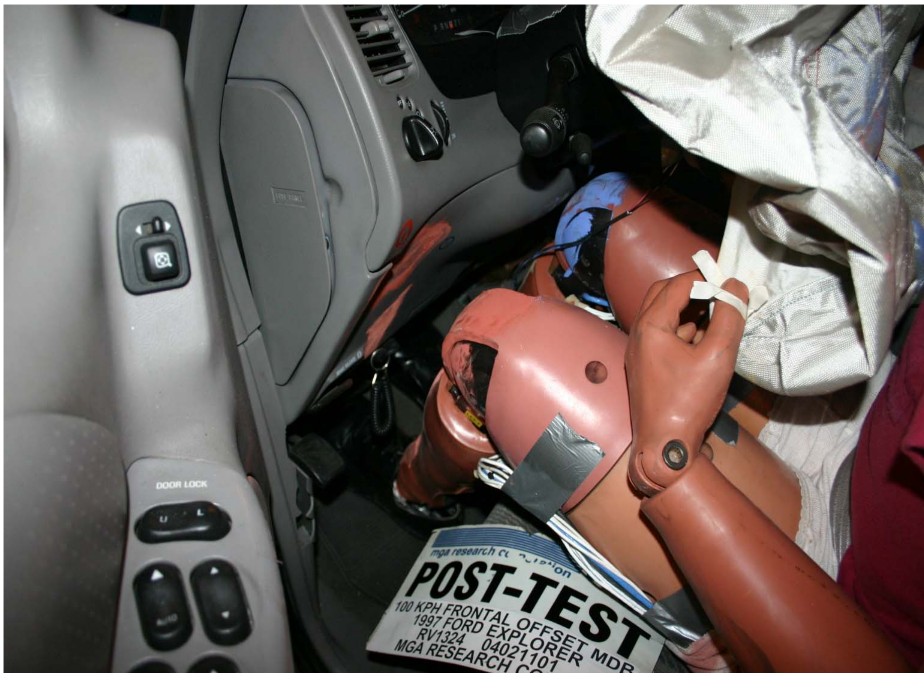
Post-Test Driver Side Knee Bolster View
