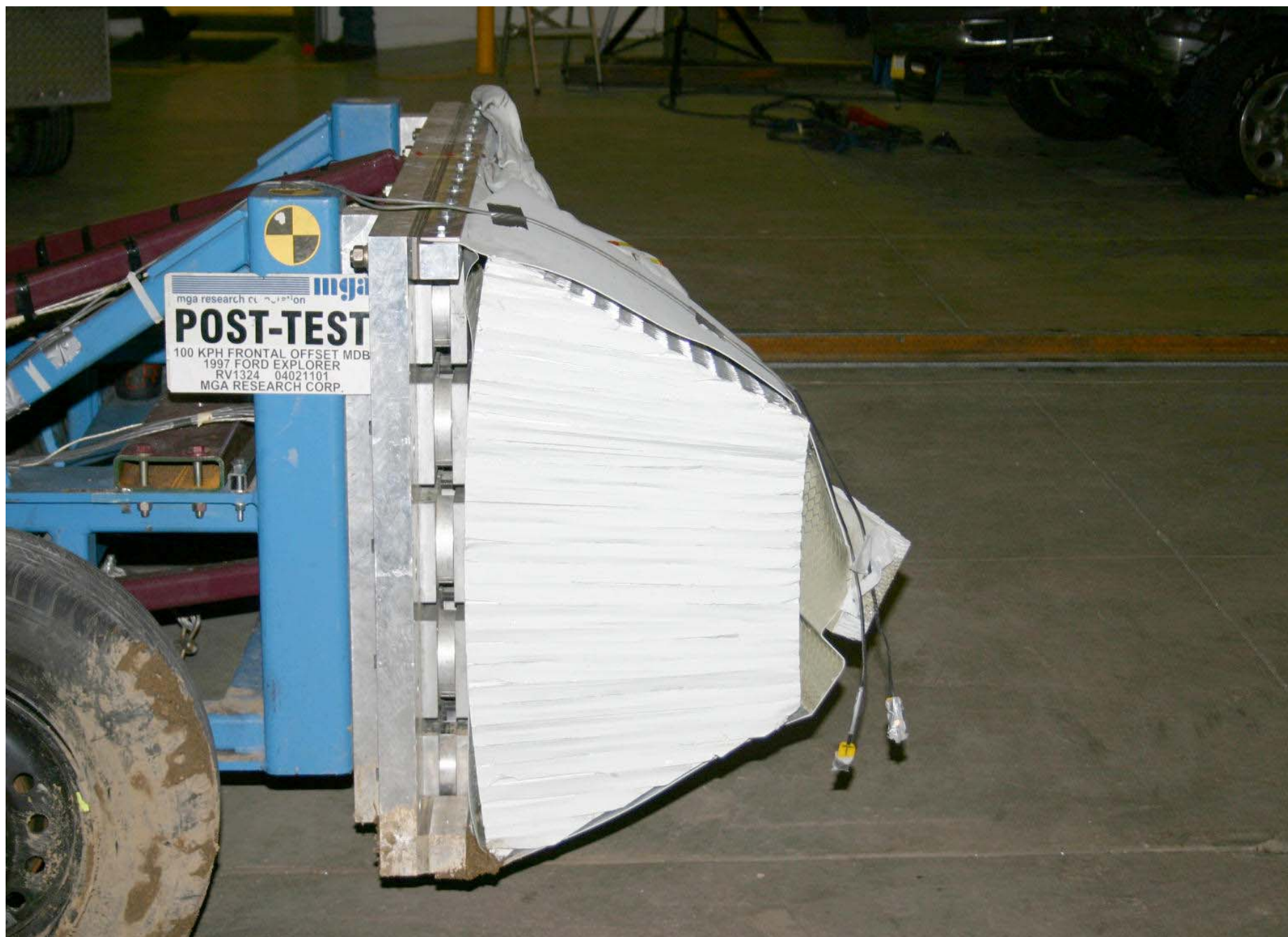
Post-Test MDB Right Side View
