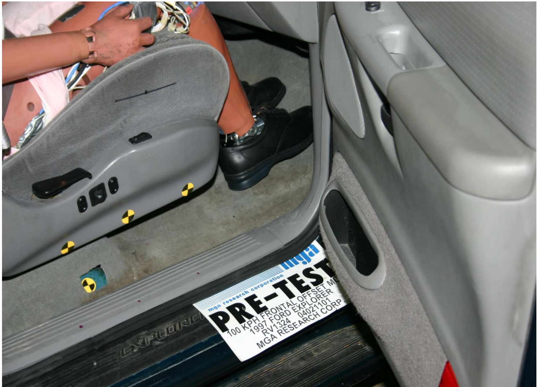
Pre-Test Passenger Dummy Feet Position
