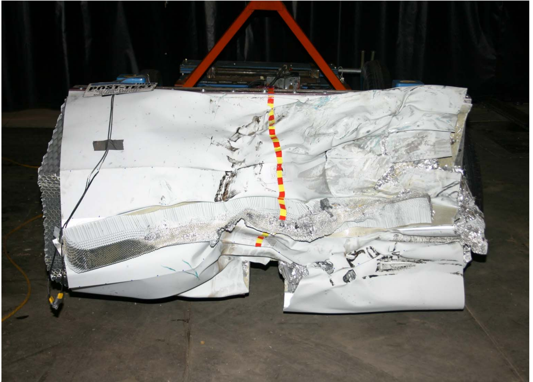
Post-Test MDB Front View
