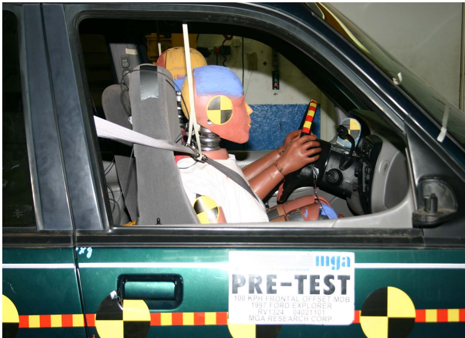
Pre-Test Passenger Dummy Position Right Side View
