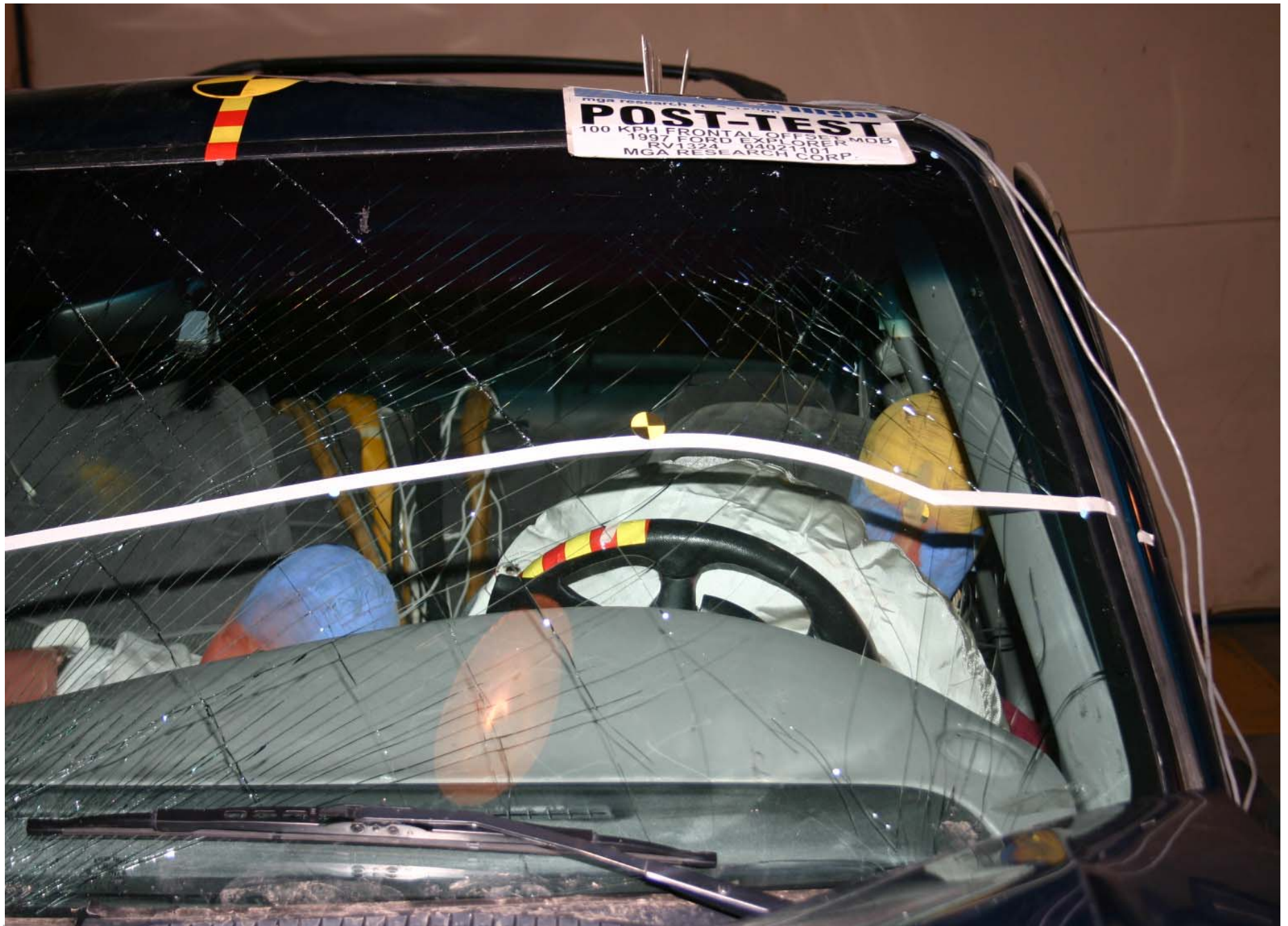
Post-Test Driver Dummy Front View (head position)
