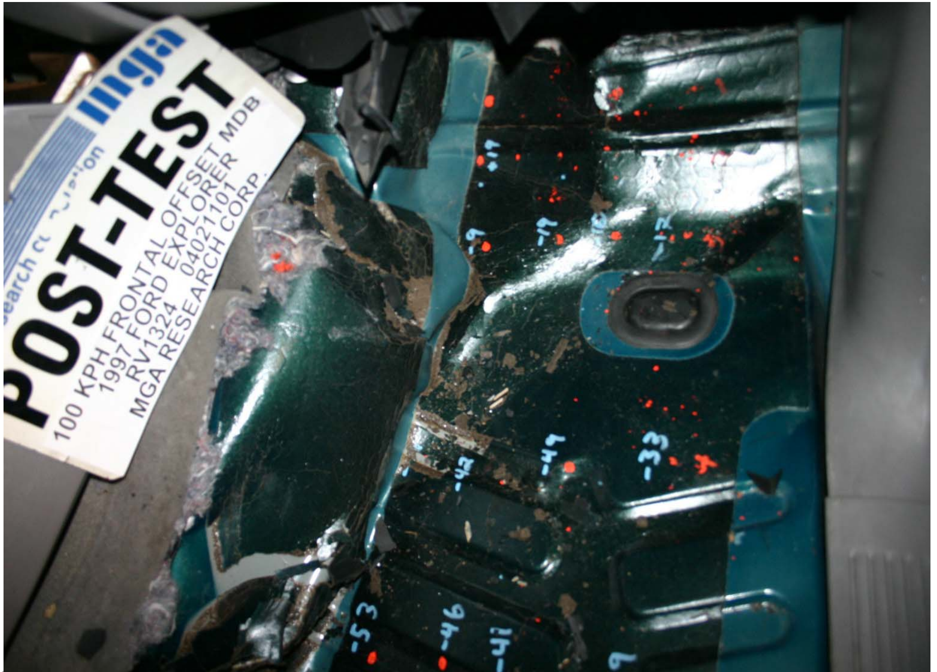
Post-Test Passenger Side Floor Pan View
