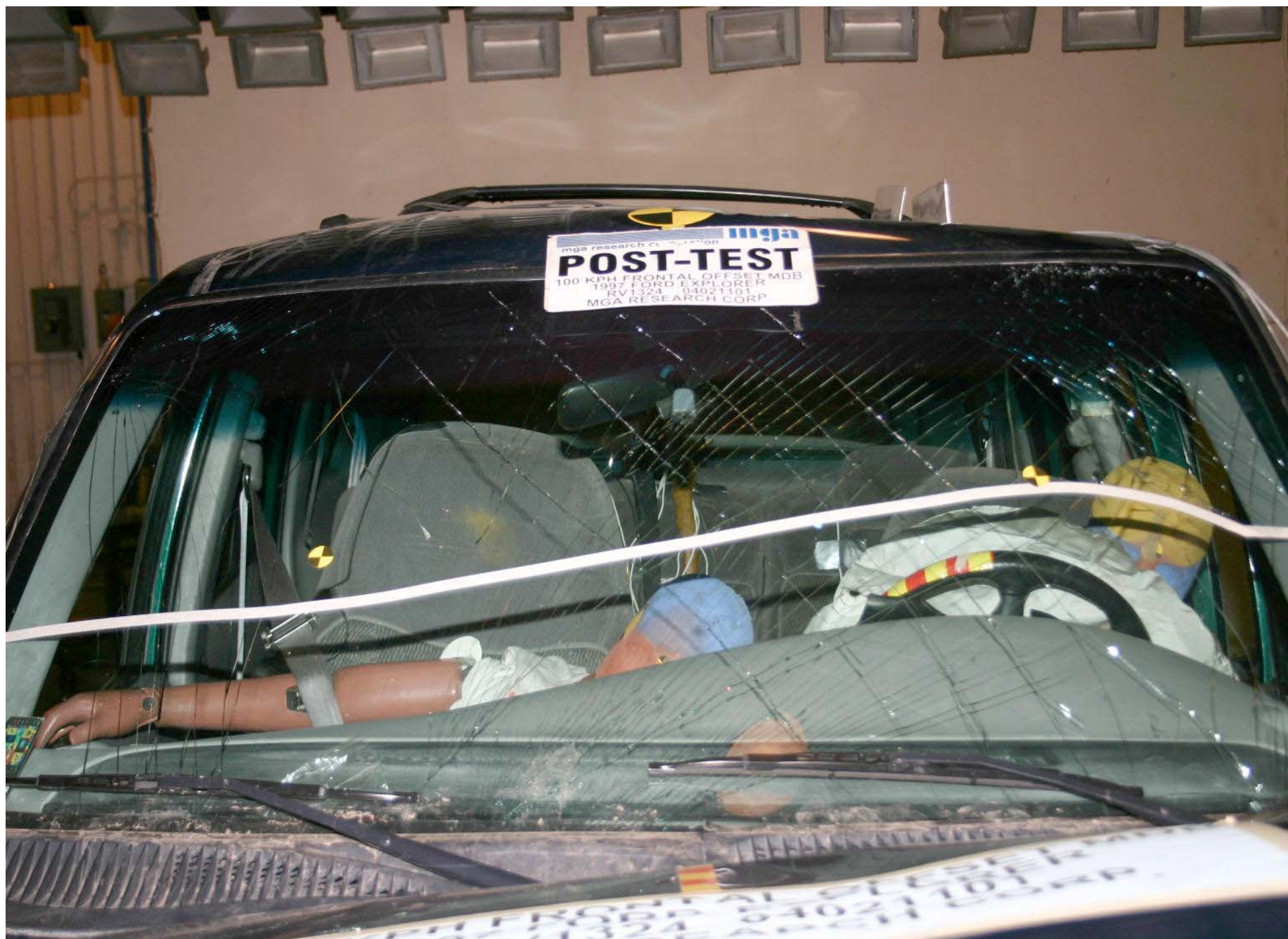
Post-Test Windshield View
