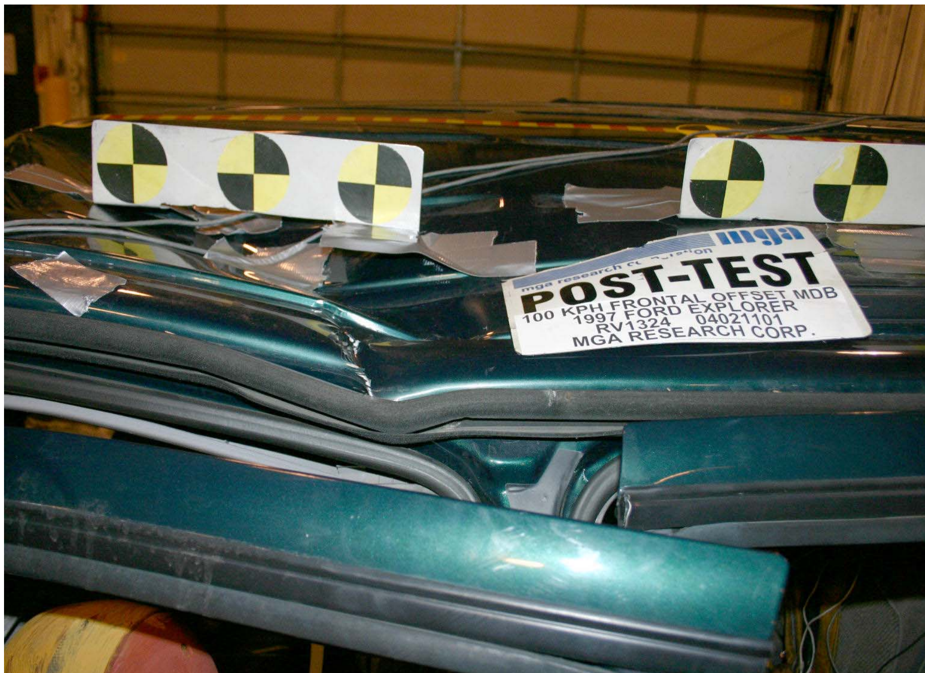
Post-Test Roof Buckle View
