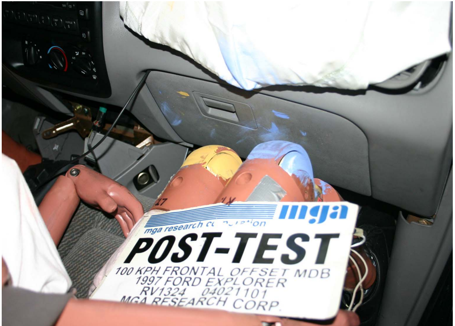
Post-Test Passenger Side Knee Bolster View
