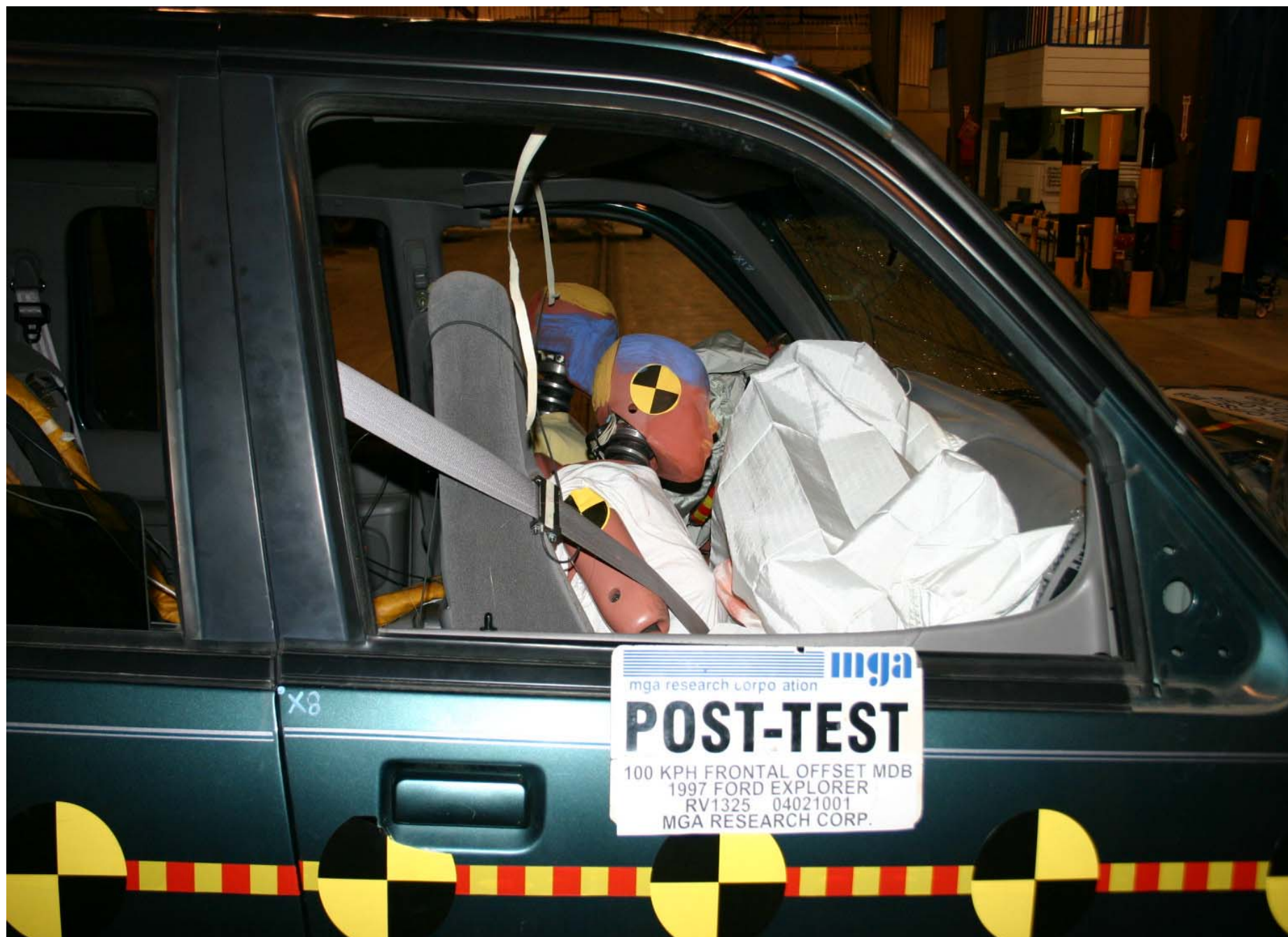
Post-Test Passenger Dummy Position Right Side View
