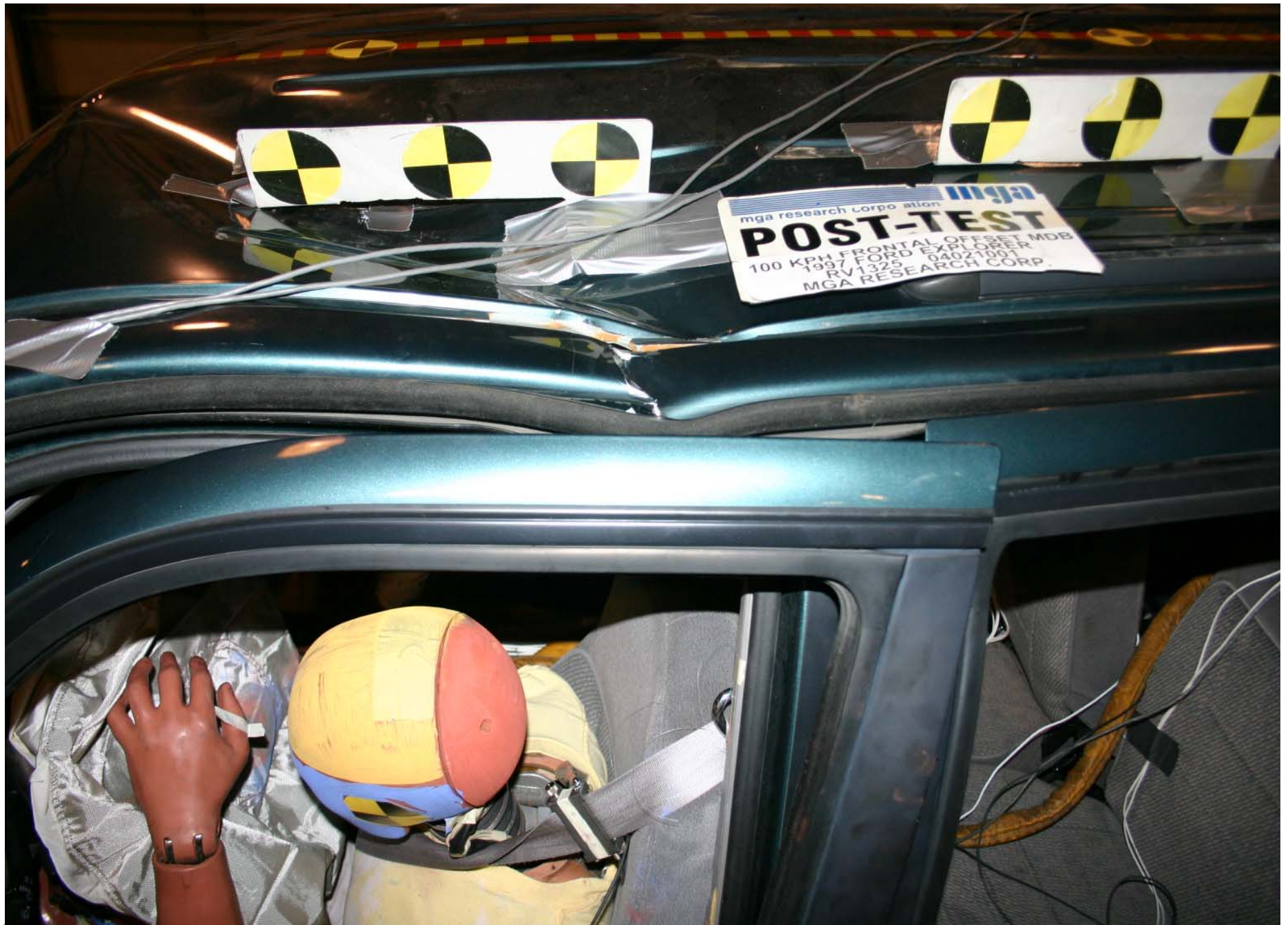
Post-Test Roof Buckle View
