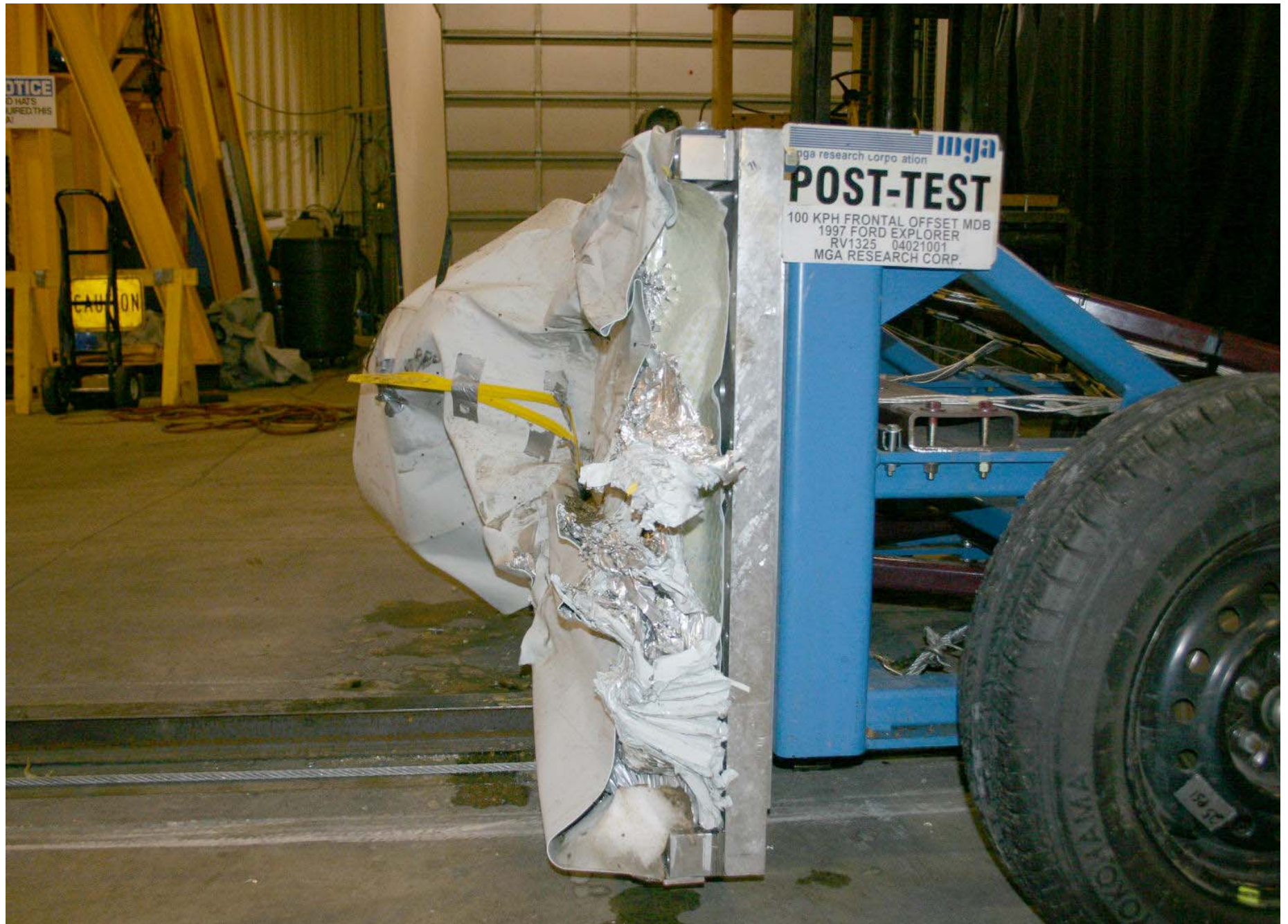
Post-Test MDB Left Side View
