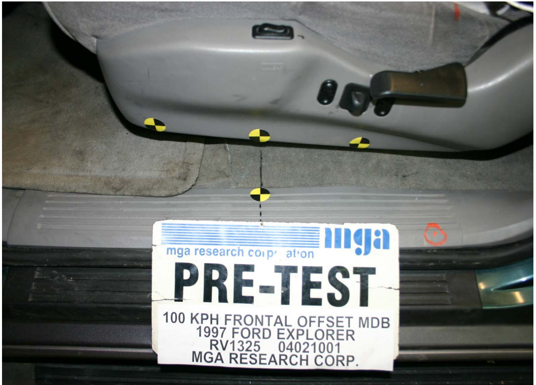
Pre-Test Driver Dummy Seat Position
