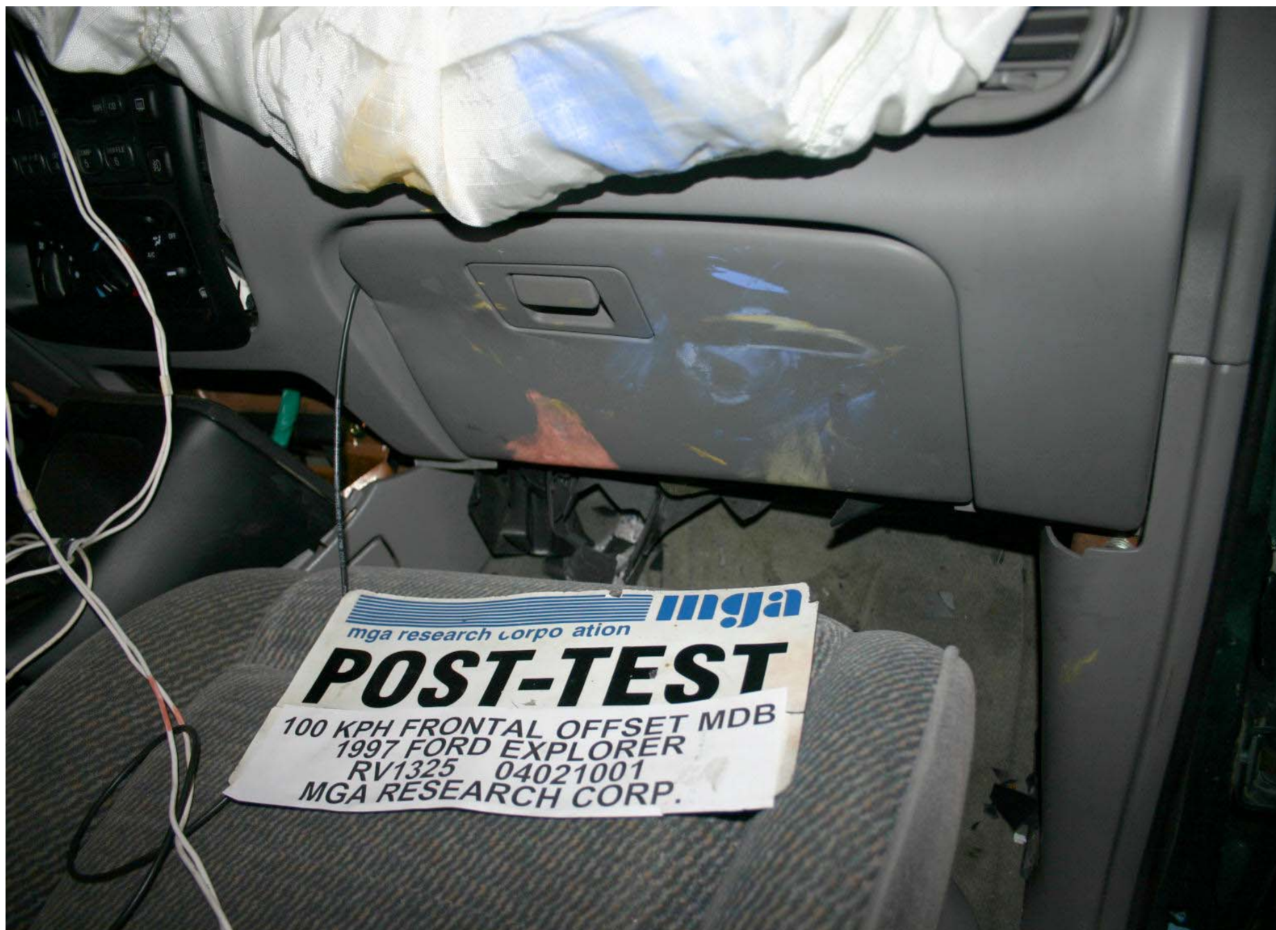
Post-Test Passenger Dummy Knee Contact
