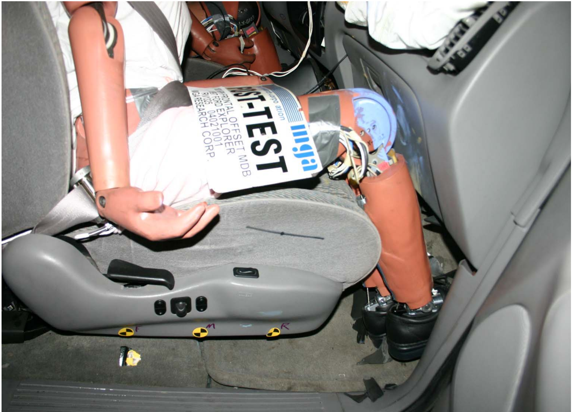
Post-Test Passenger Side Knee Bolster View
