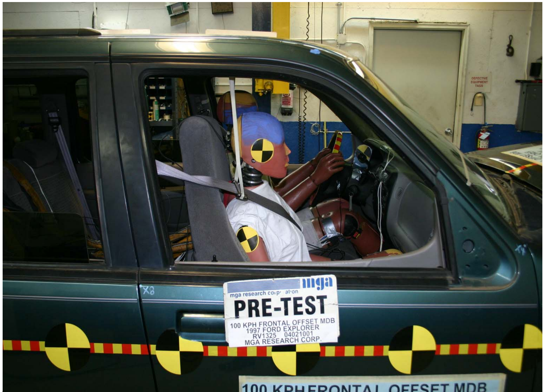
Pre-Test Passenger Dummy Position Right Side View
