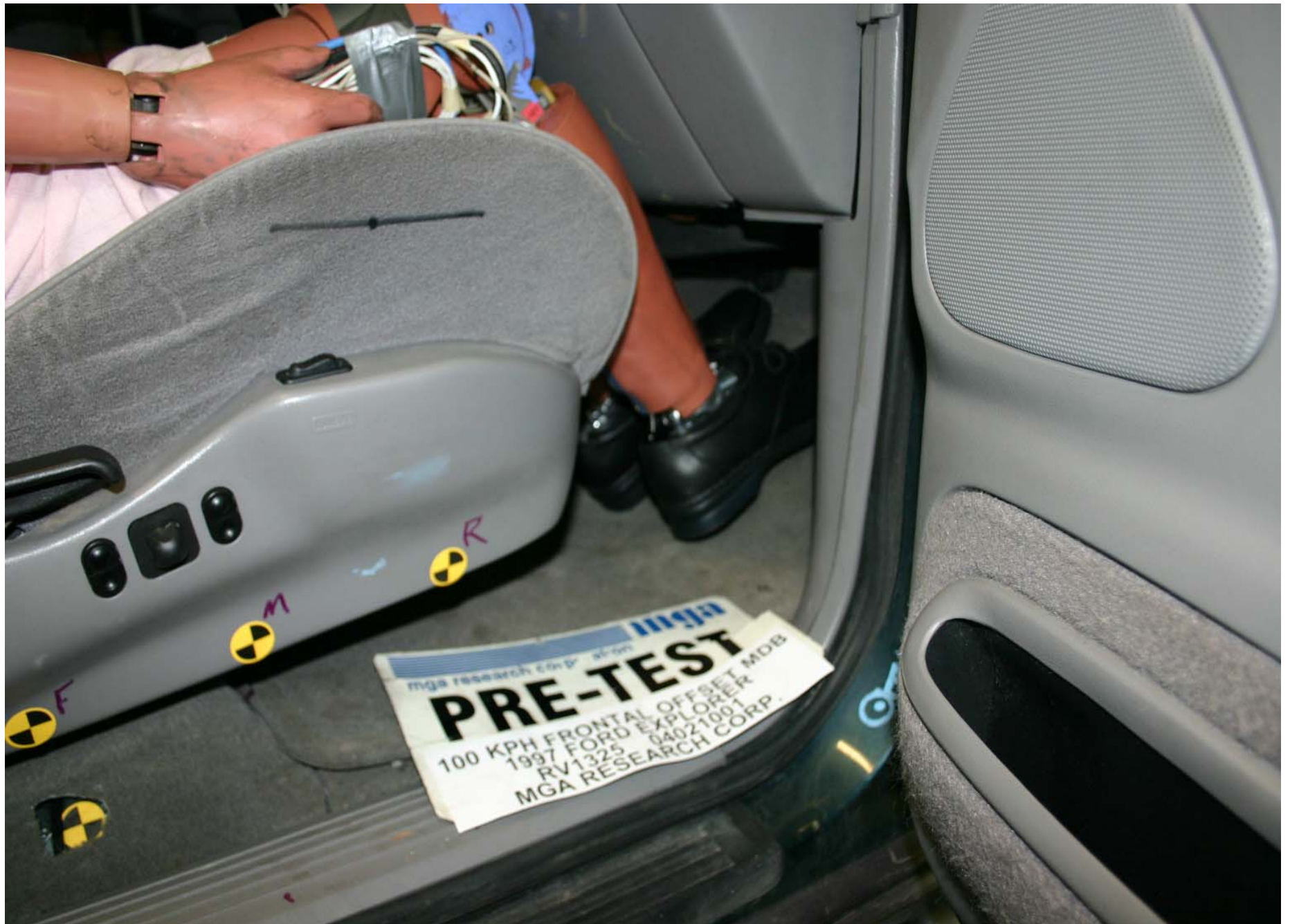
Pre-Test Passenger Dummy Feet Position
