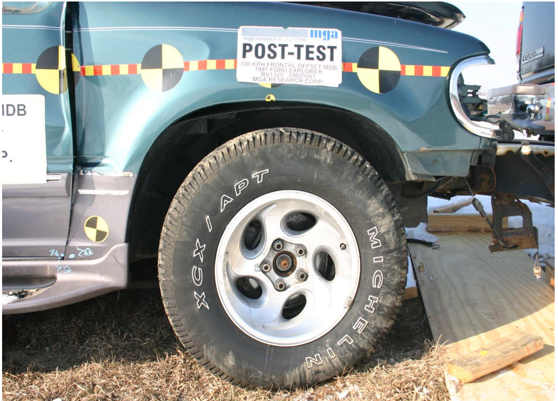
Post-Test Right Front Wheel Well
