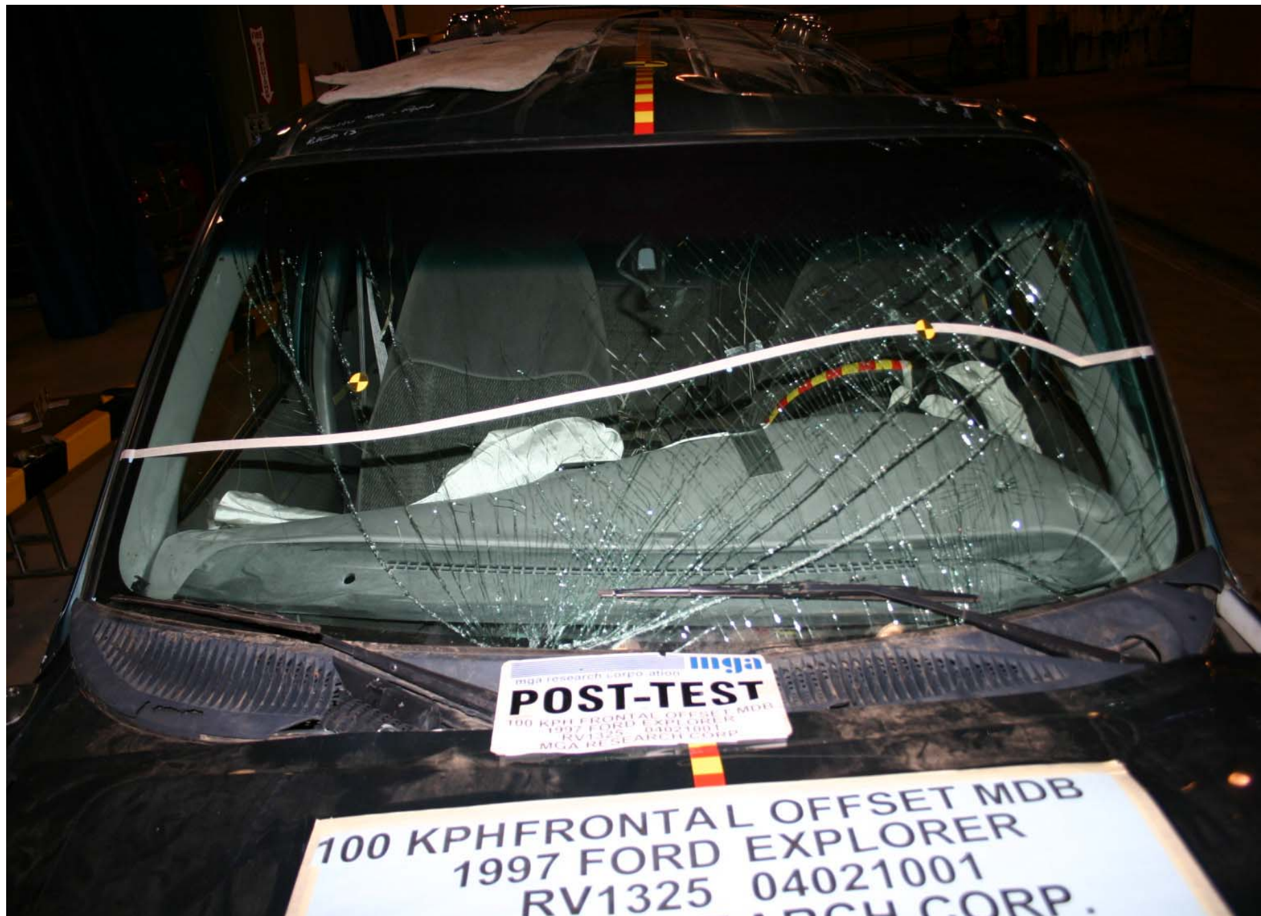
Post-Test Windshield View
