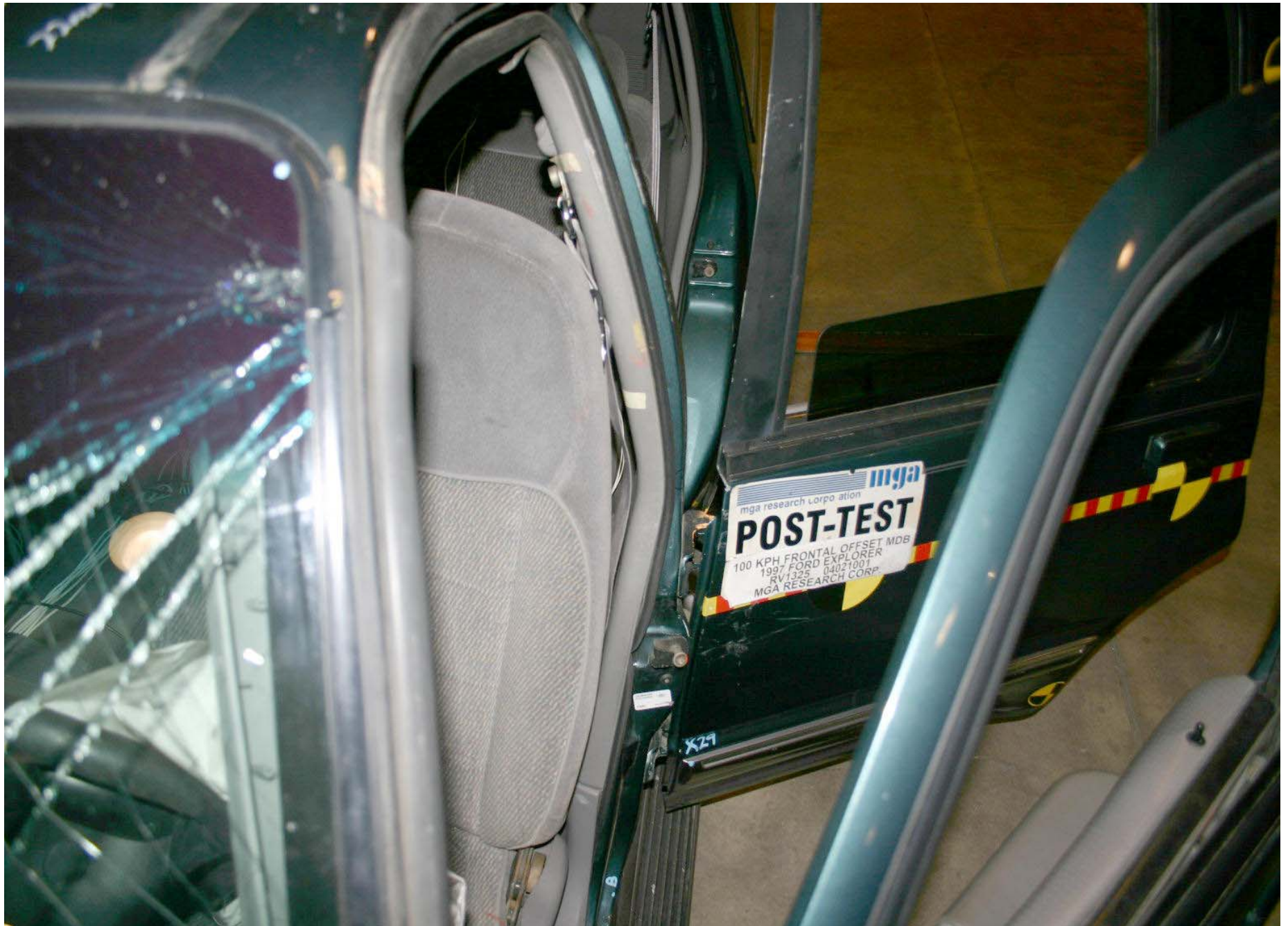
Post-Test Driver Dummy B Pillar Contact
