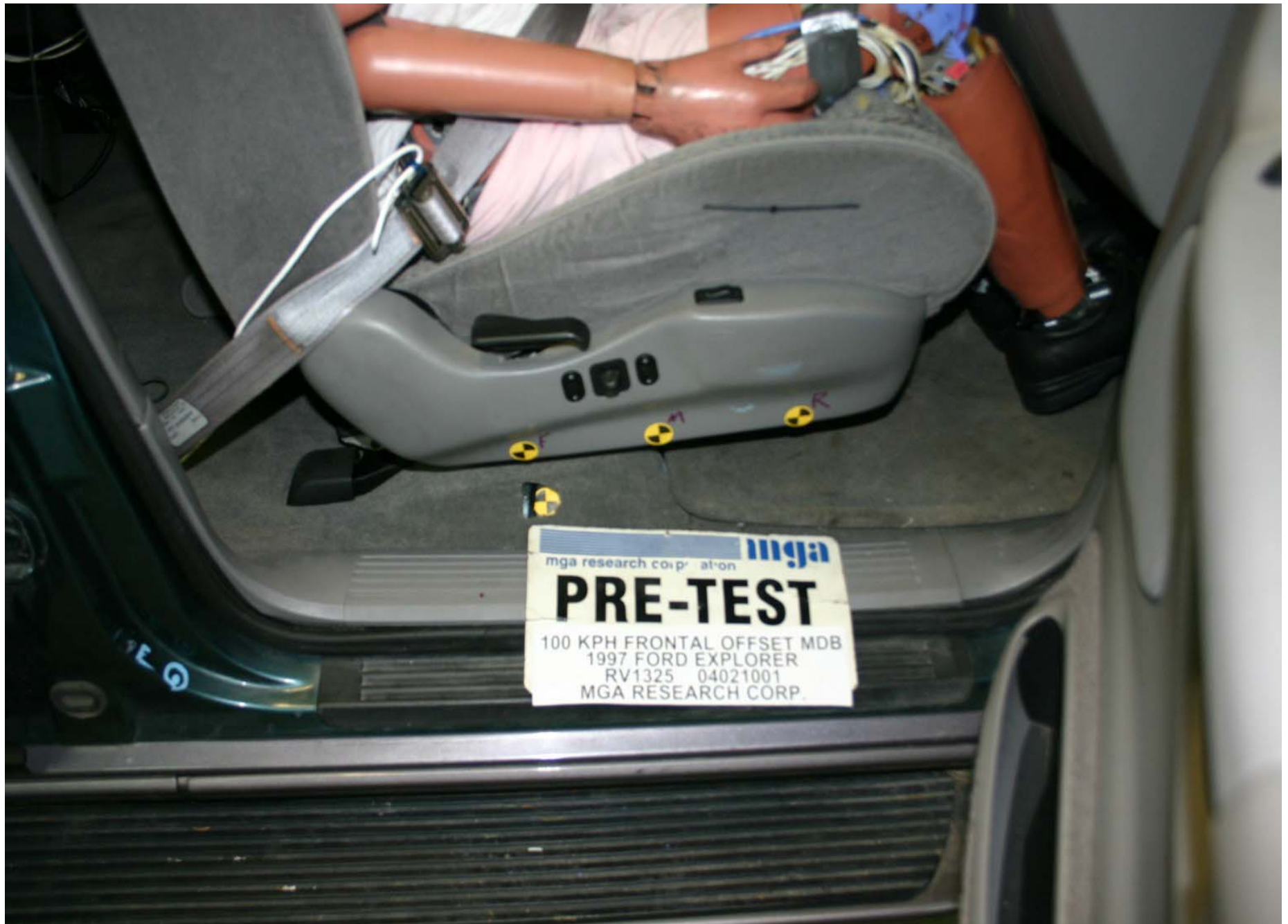
Pre-Test Passenger Dummy Seat Position
