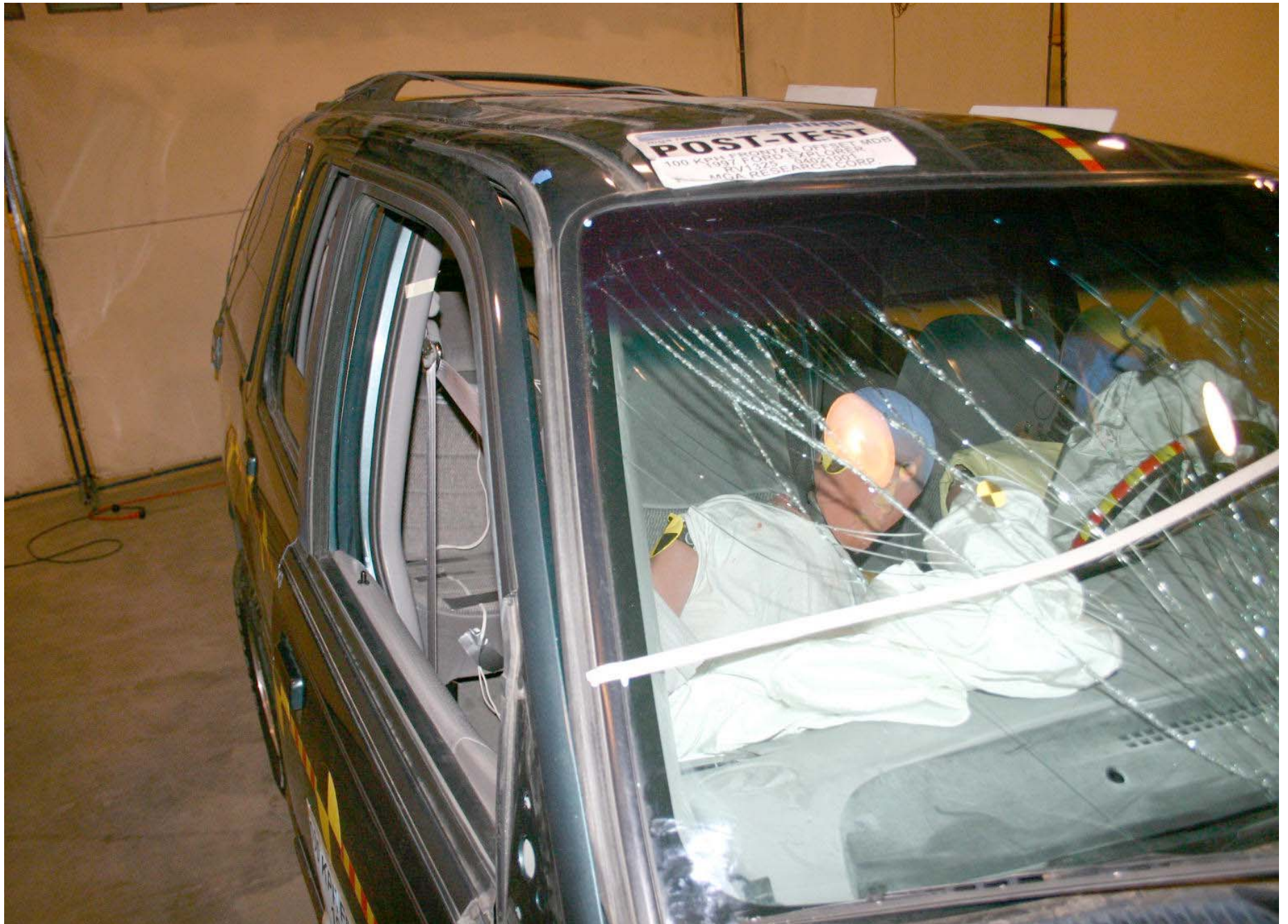
Post-Test Passenger Dummy Front View (head position)
