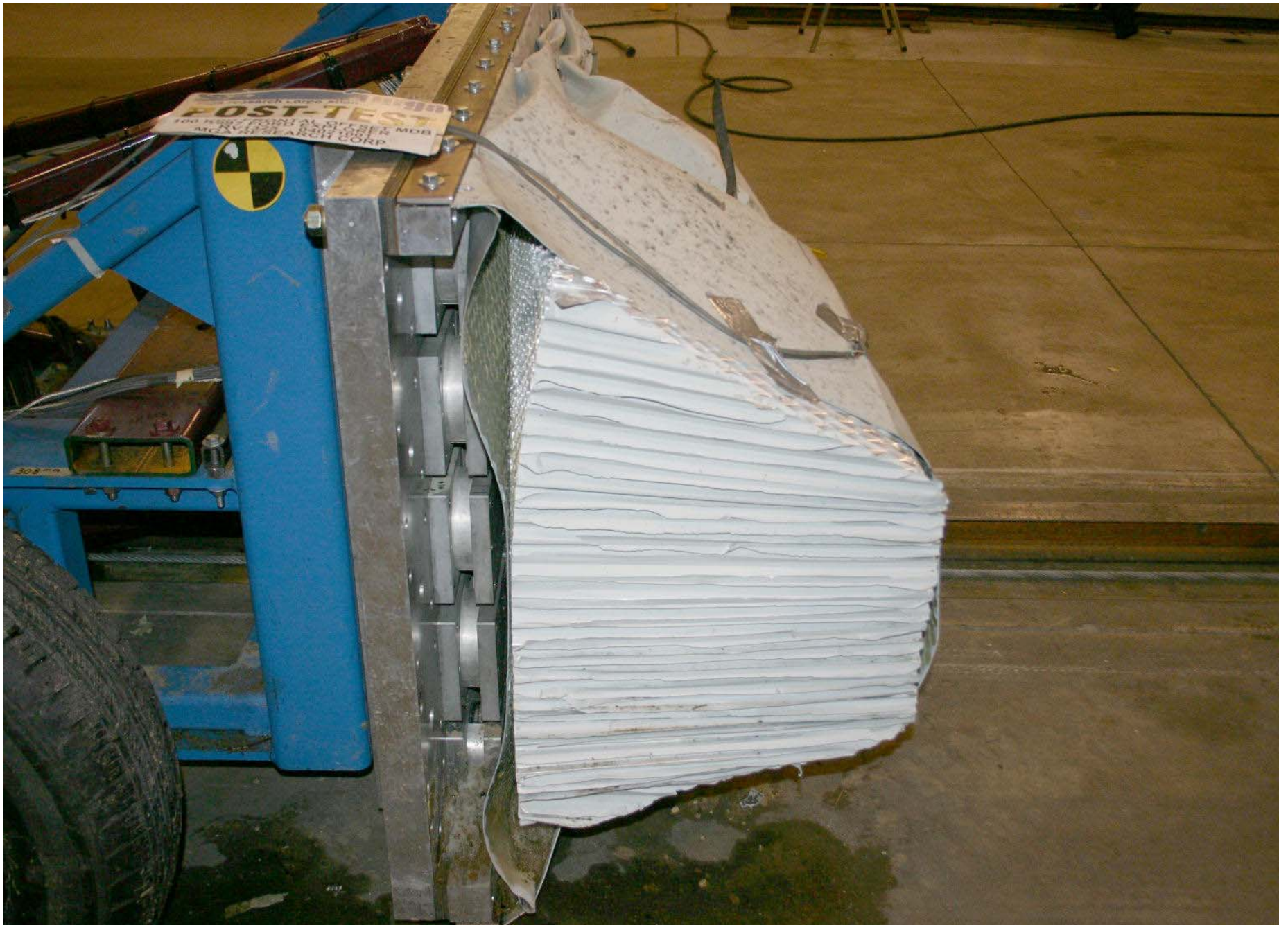
Post-Test MDB Right Side View
