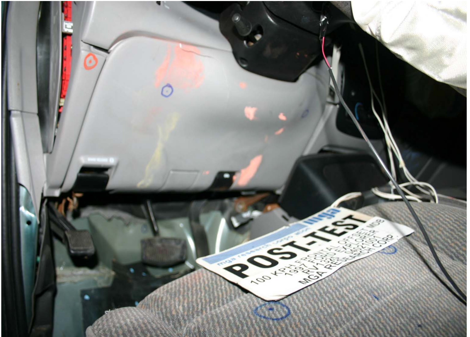
Post-Test Driver Dummy Knee Contact
