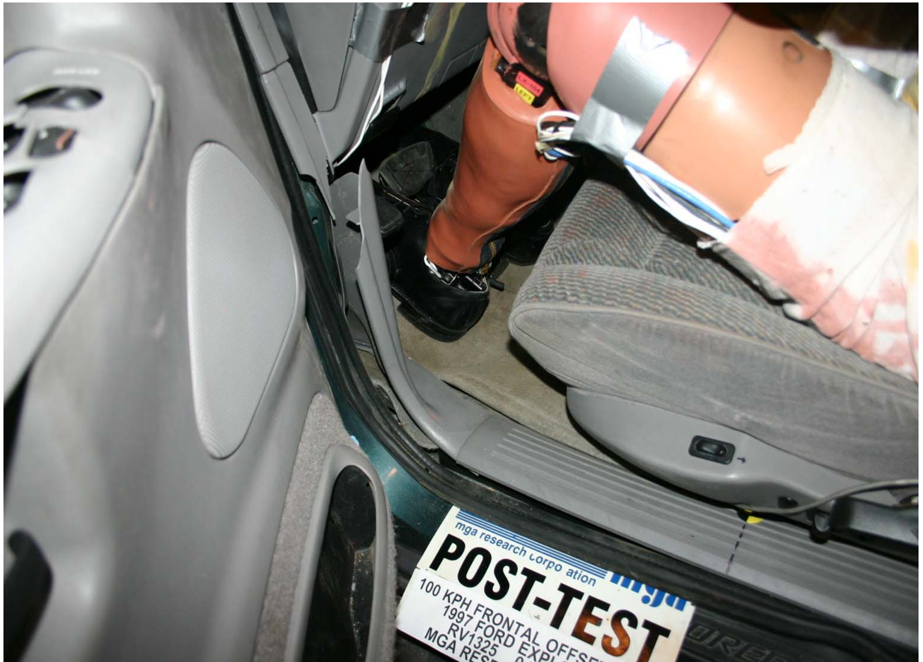
Post-Test Driver Dummy Feet Position
