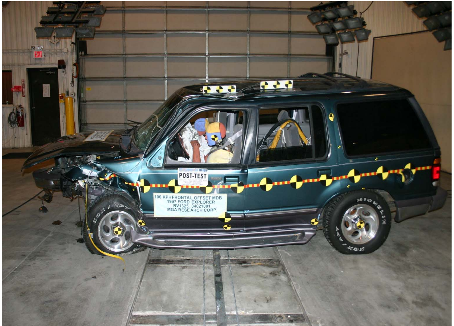
Post-Test Left Side View of Test Vehicle
