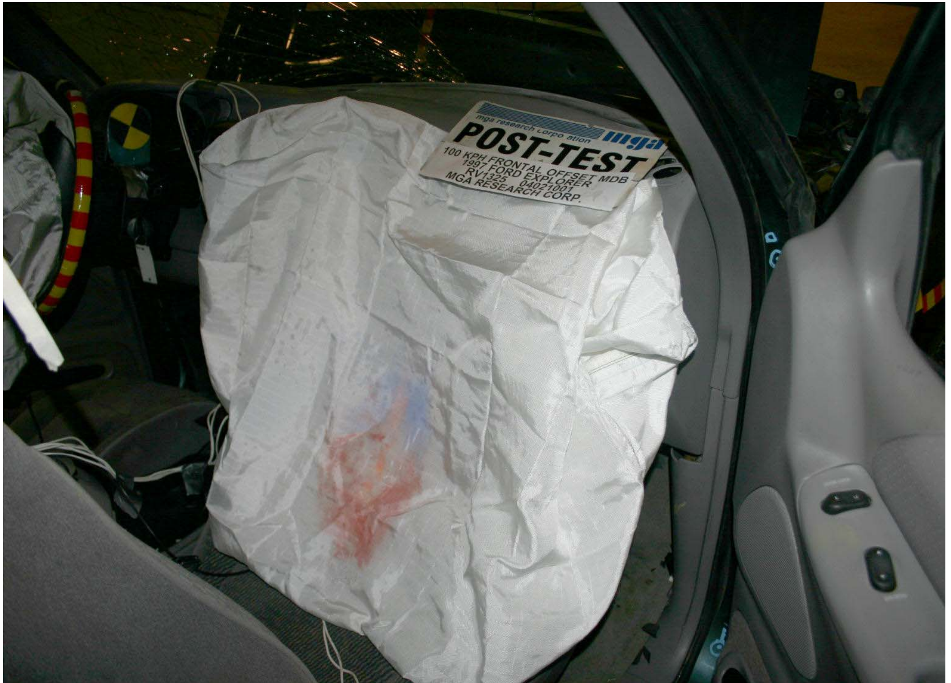
Post-Test Passenger Dummy Airbag Contact
