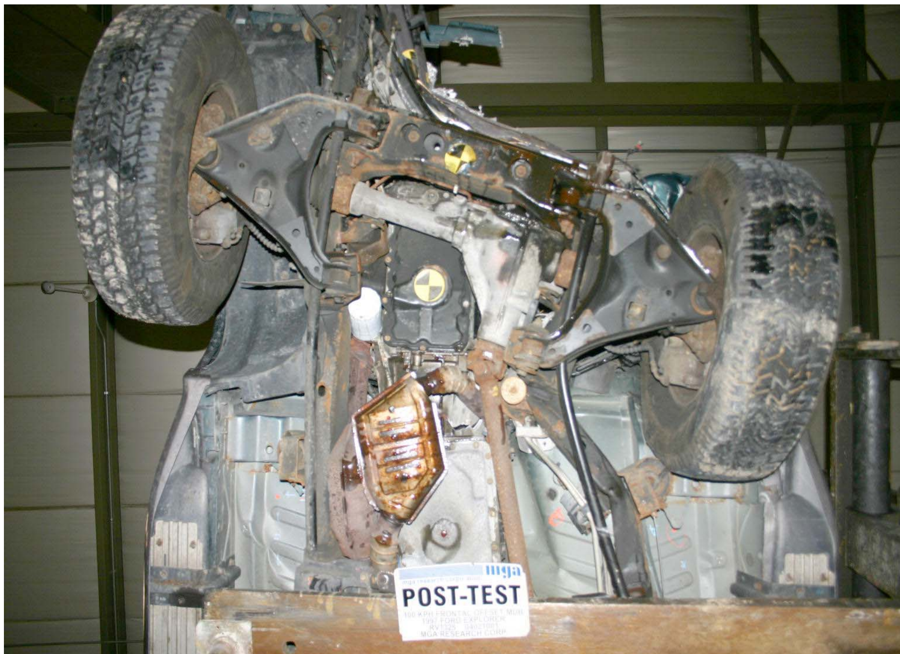
Post-Test Front Underbody View
