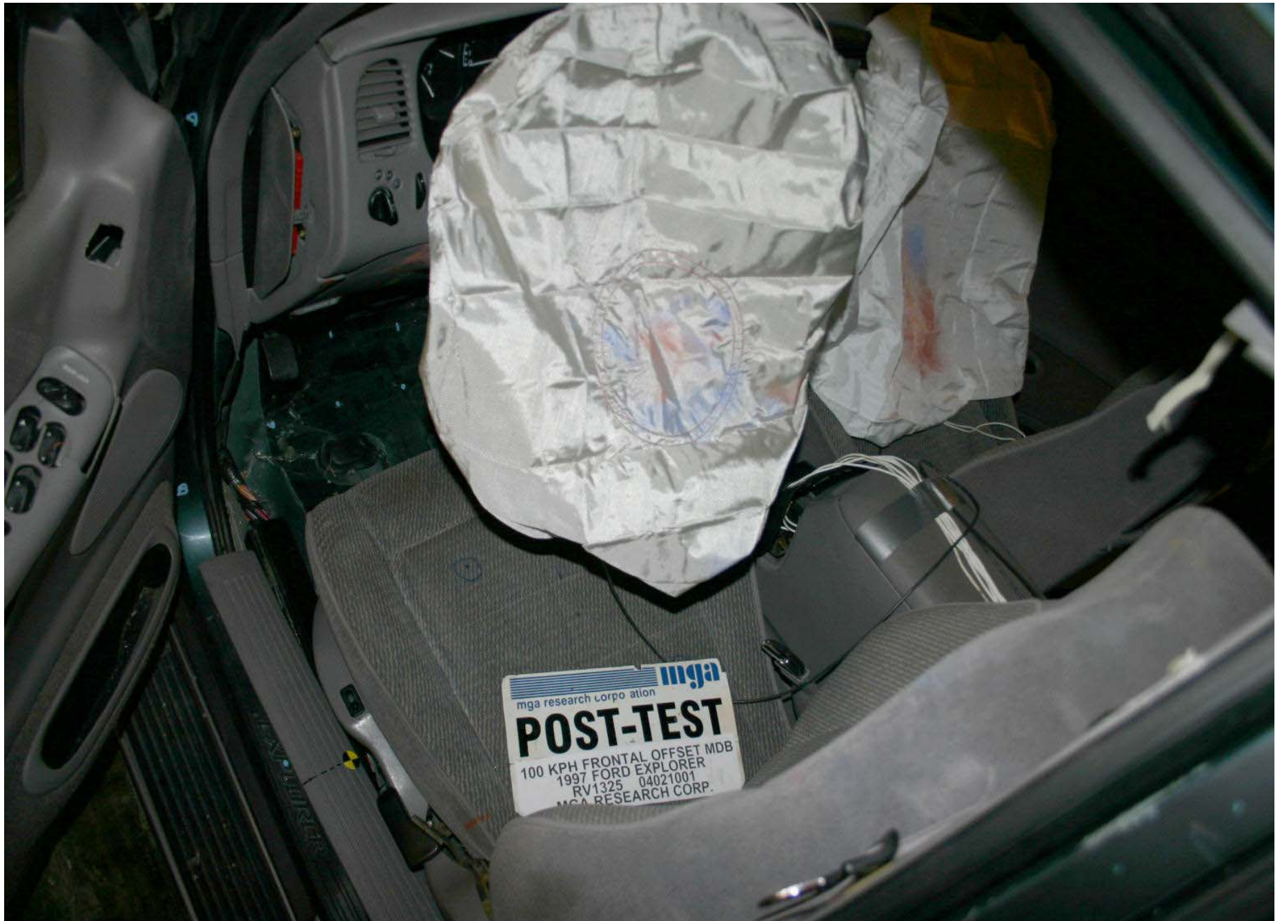
Post-Test Driver Dummy Airbag Contact
