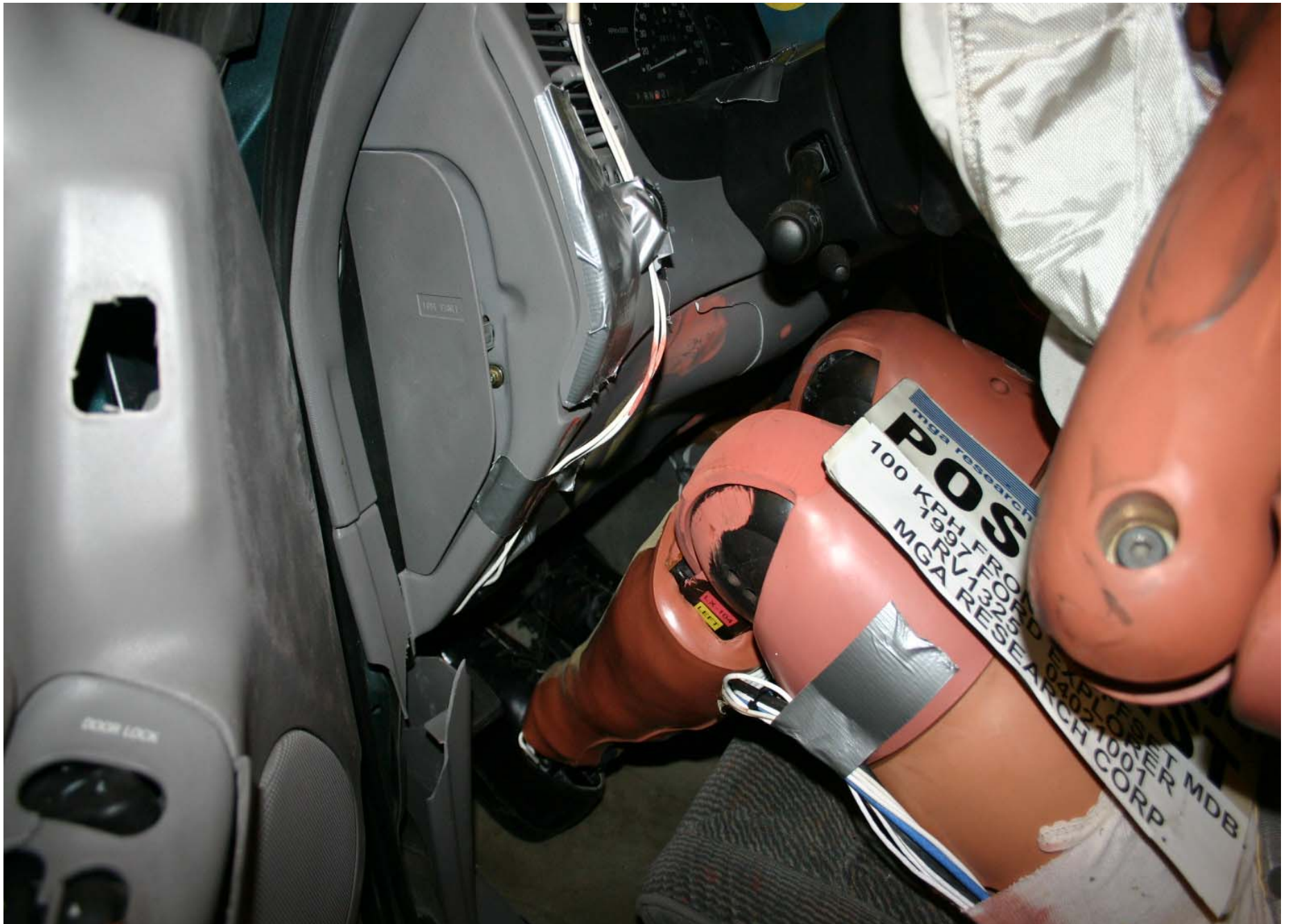
Post-Test Driver Side Knee Bolster View
