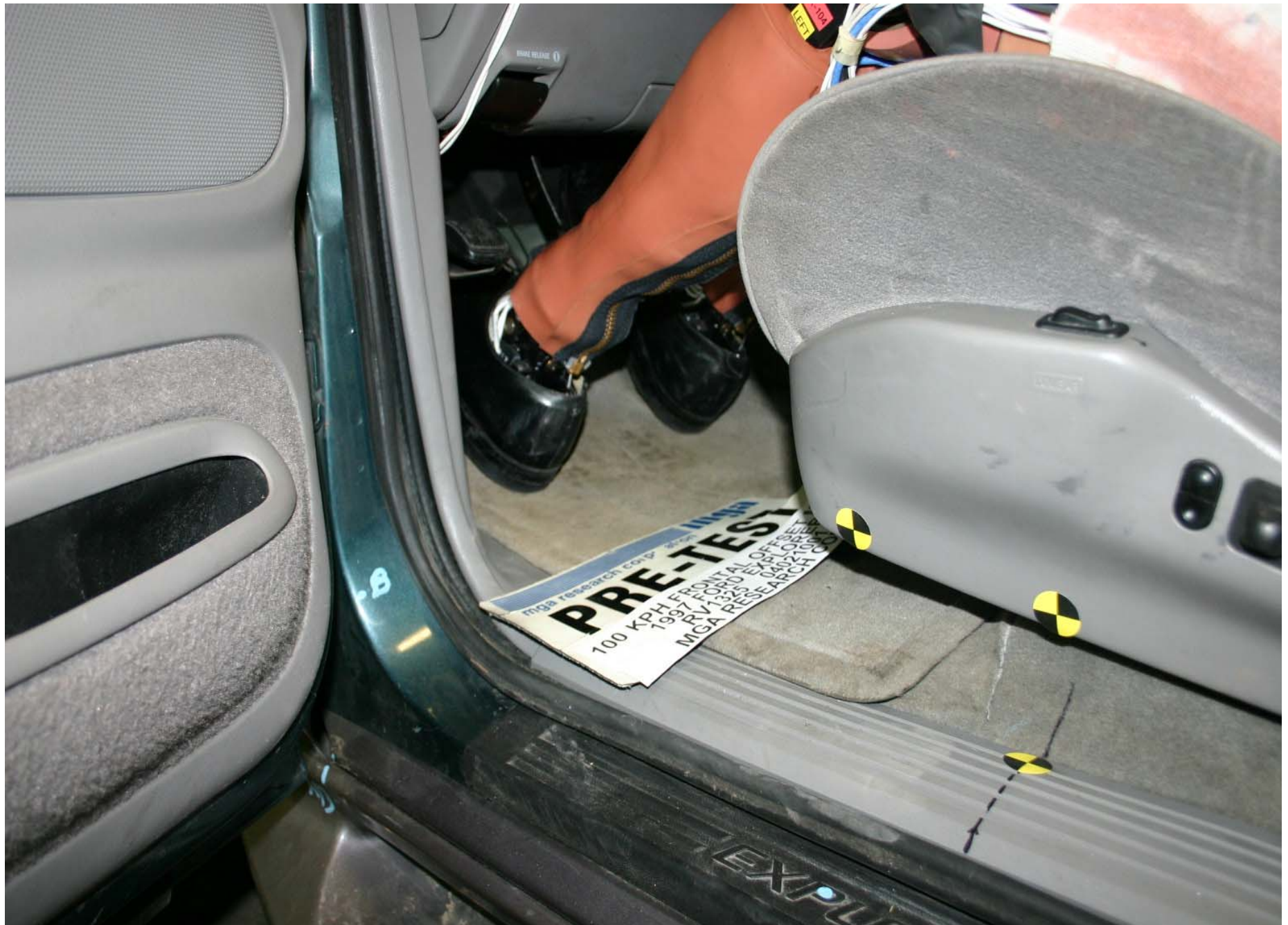
Pre-Test Driver Dummy Feet Position
