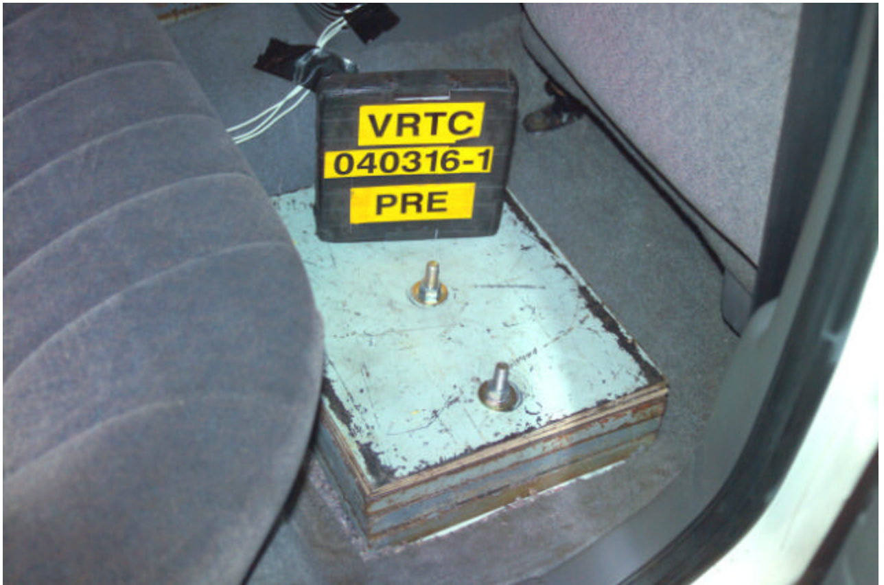
Figure A-13 Pre-Test Vehicle Ballast - View 1
