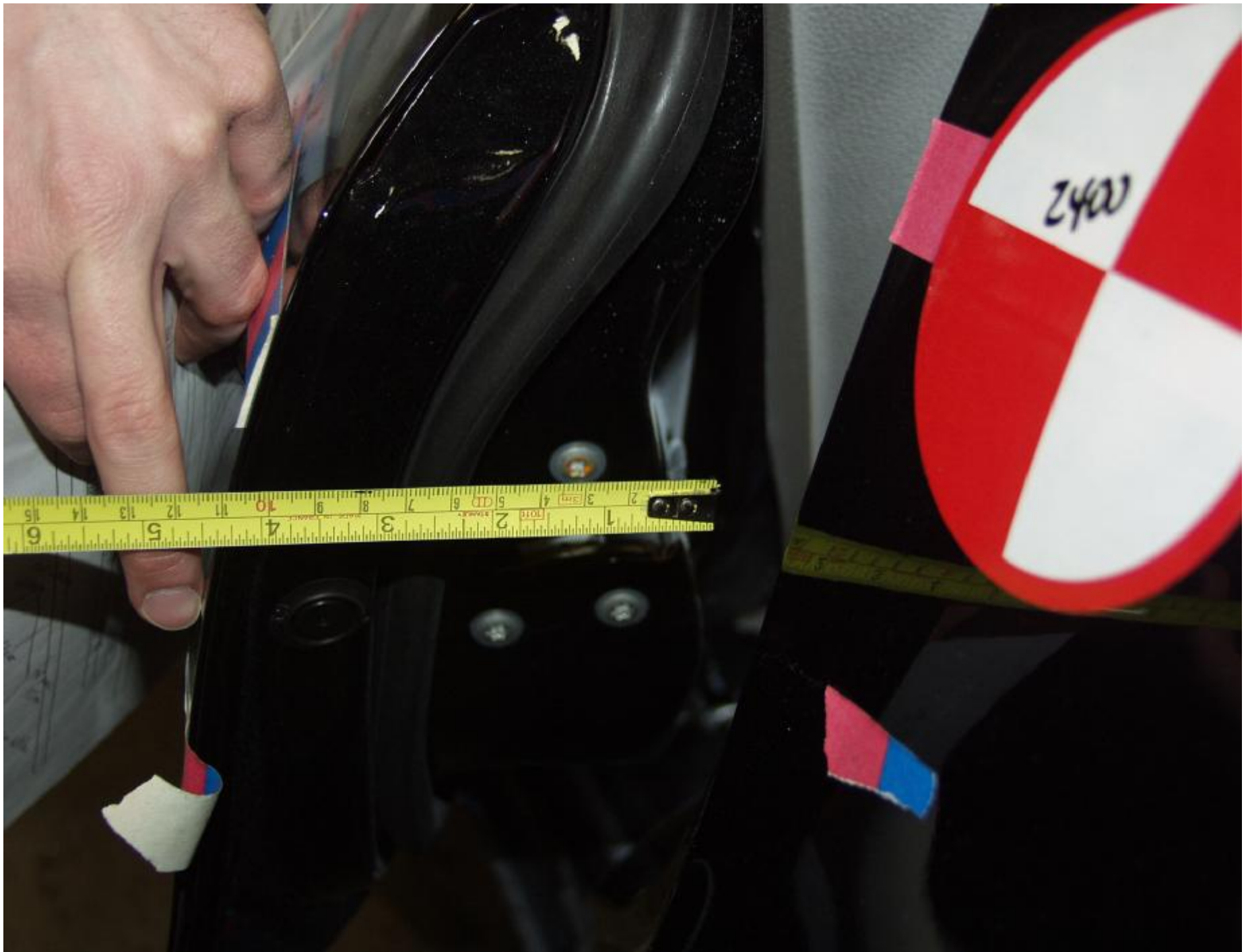
Figure A-47 POST-TEST DOOR OPENING
