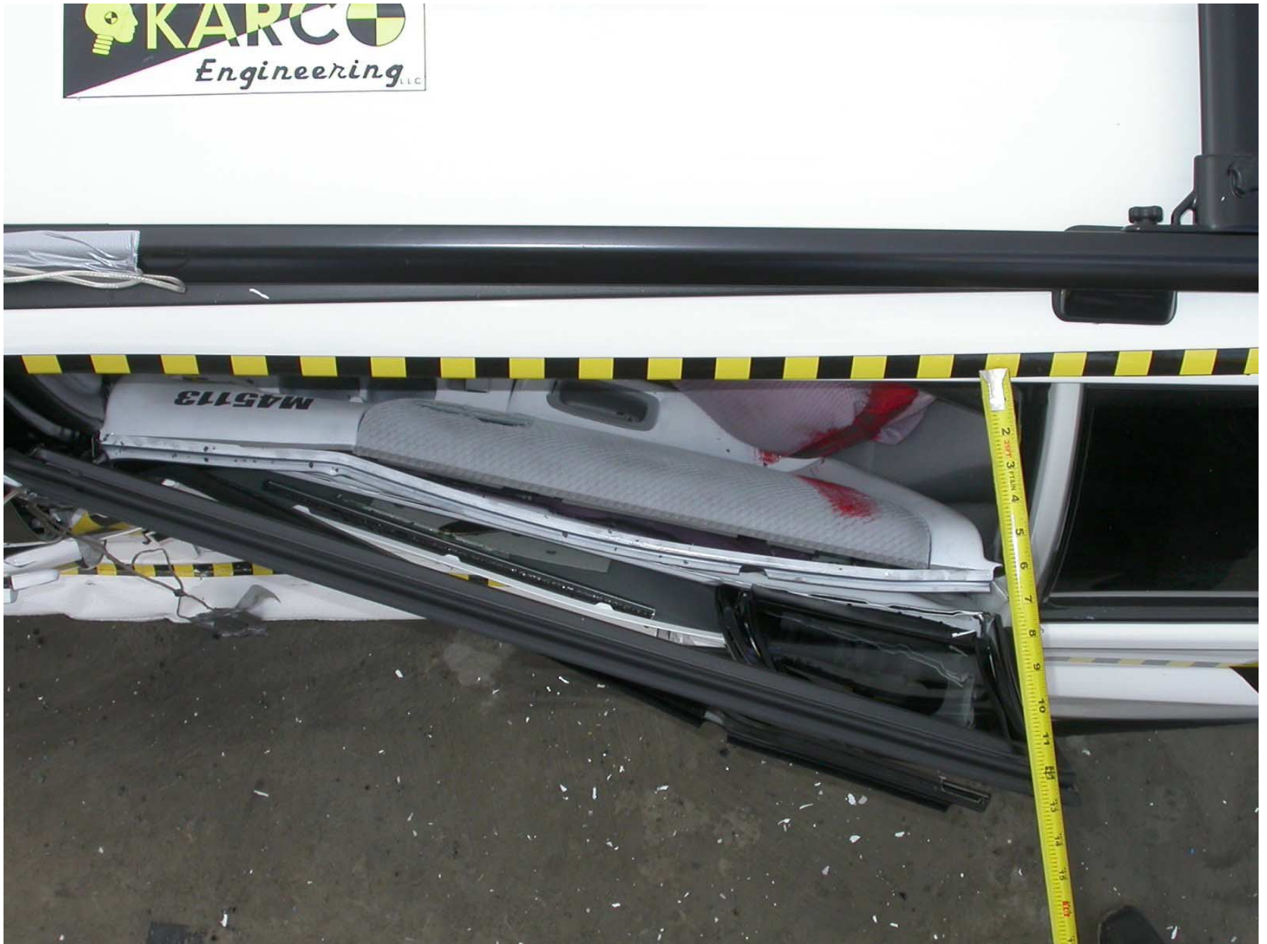
Figure A-66: Left Rear Door Window Separation, Post-Test
