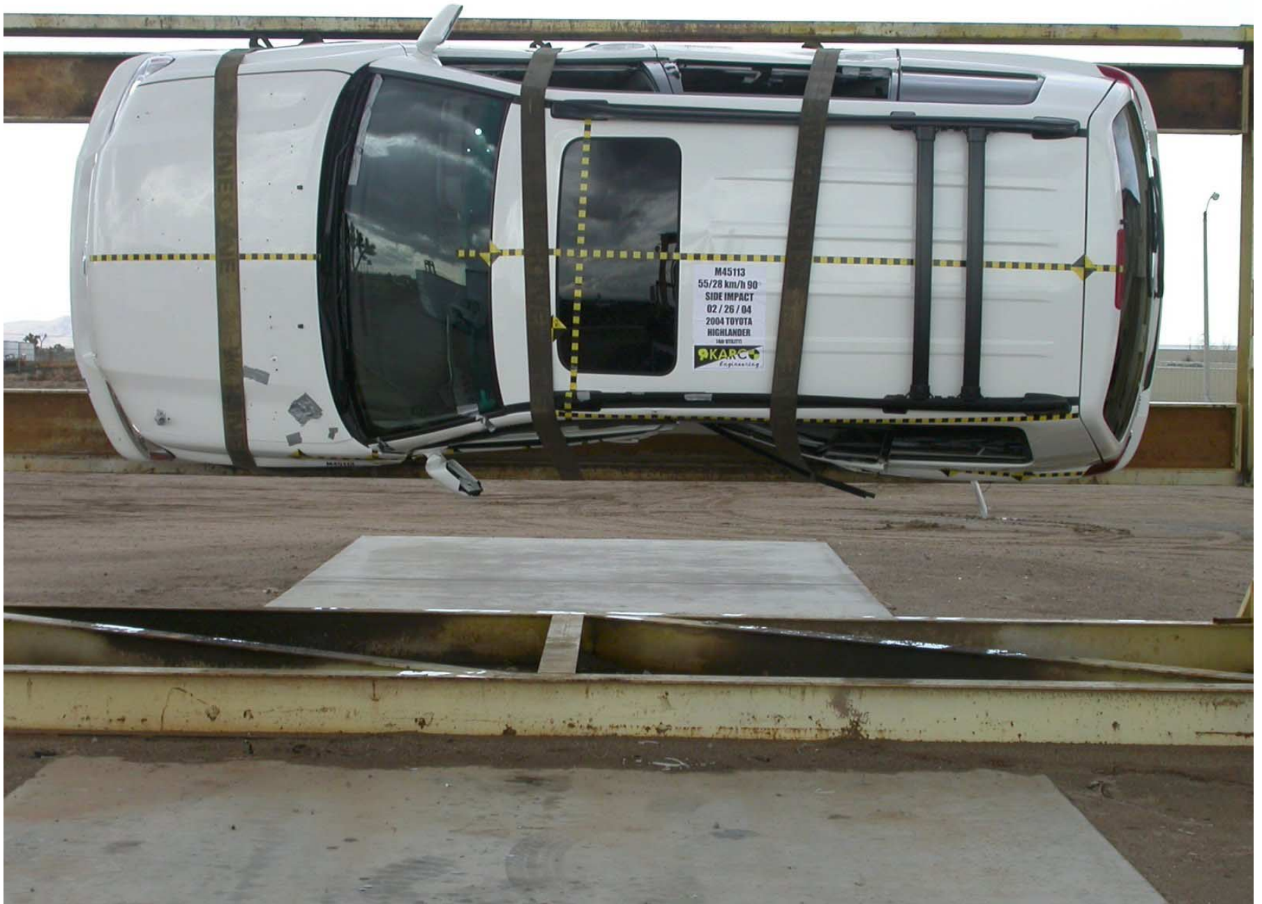
Figure A-62: Vehicle on Rollover Device, 90° View
