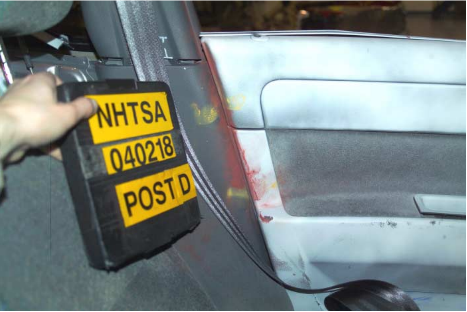
Figure A-33 Post-Test Front SID HIII Contact - View 3 A-36
