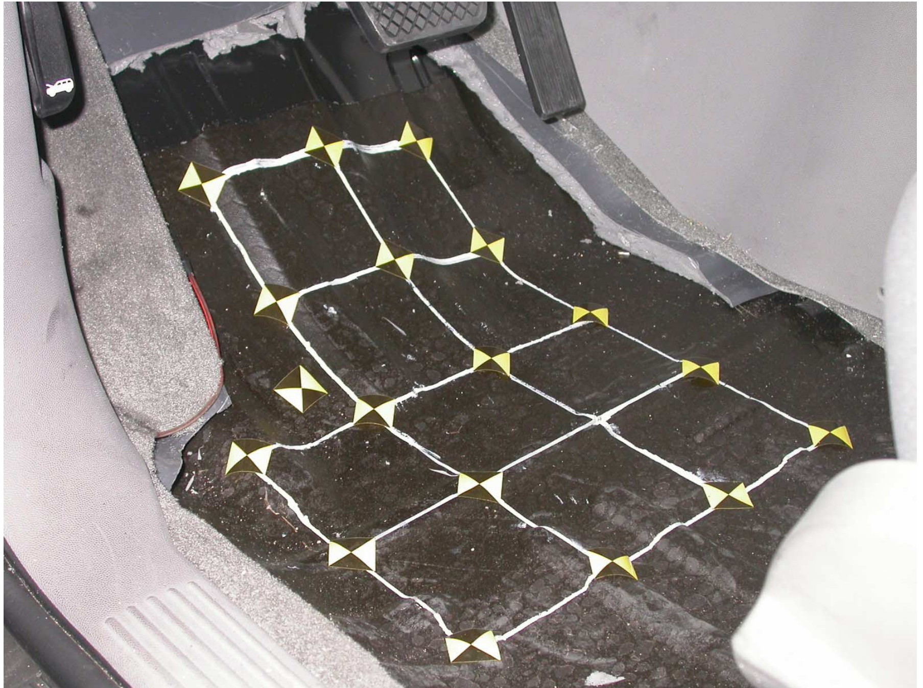
Figure A-40: Pre-Test Driver Side Floor Pan
