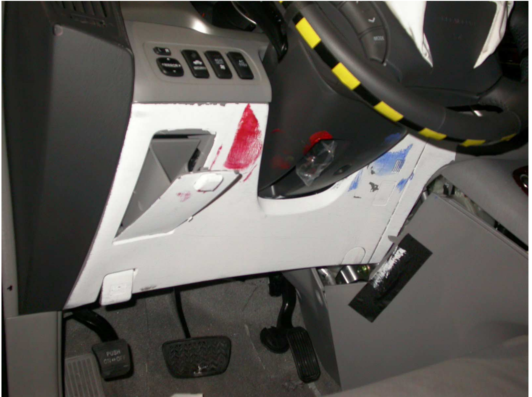
Figure A-39: Post-Test Driver Side Knee Bolster
