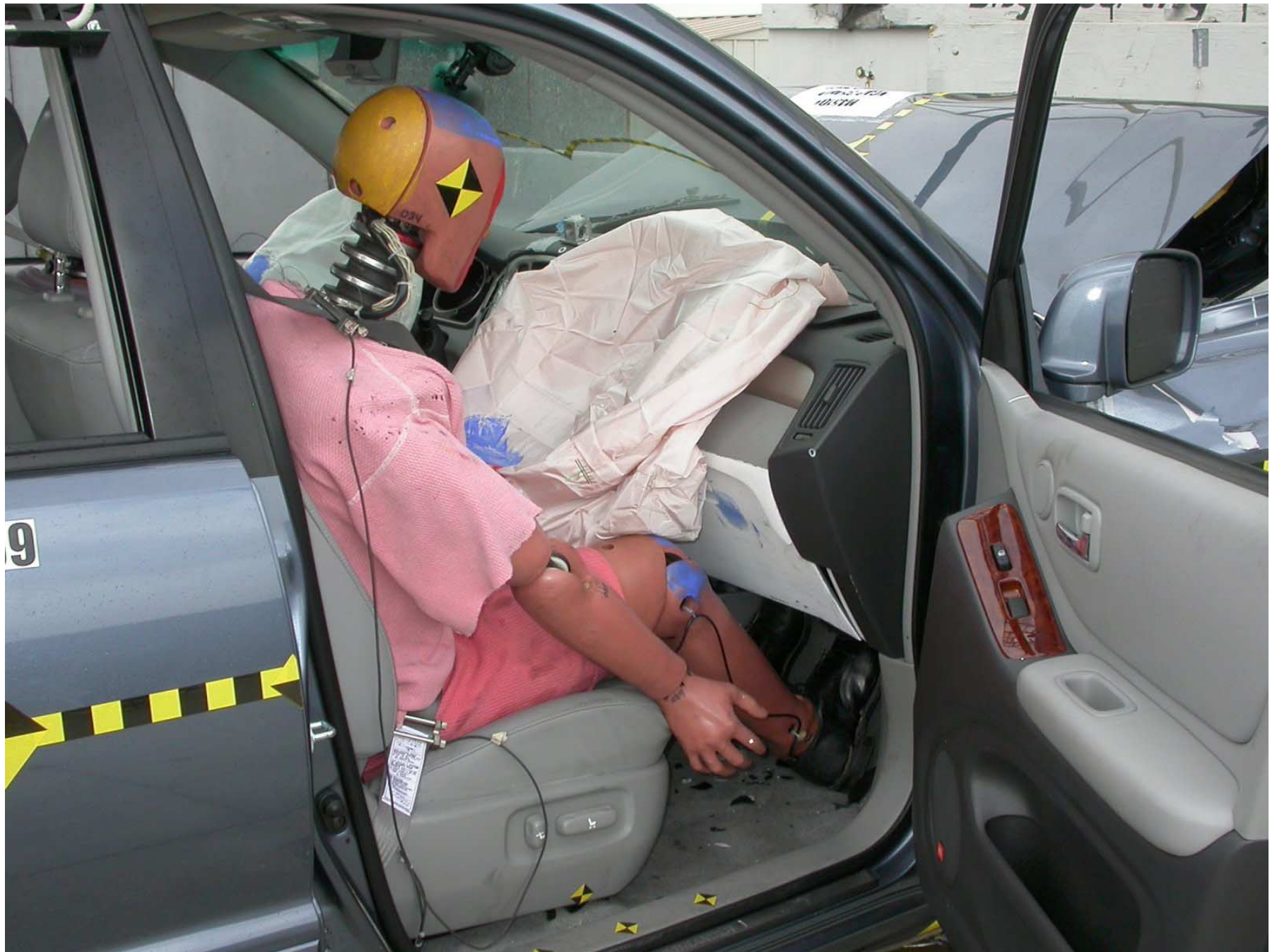
Figure A-49: Post-Test Passenger Dummy Door Open
