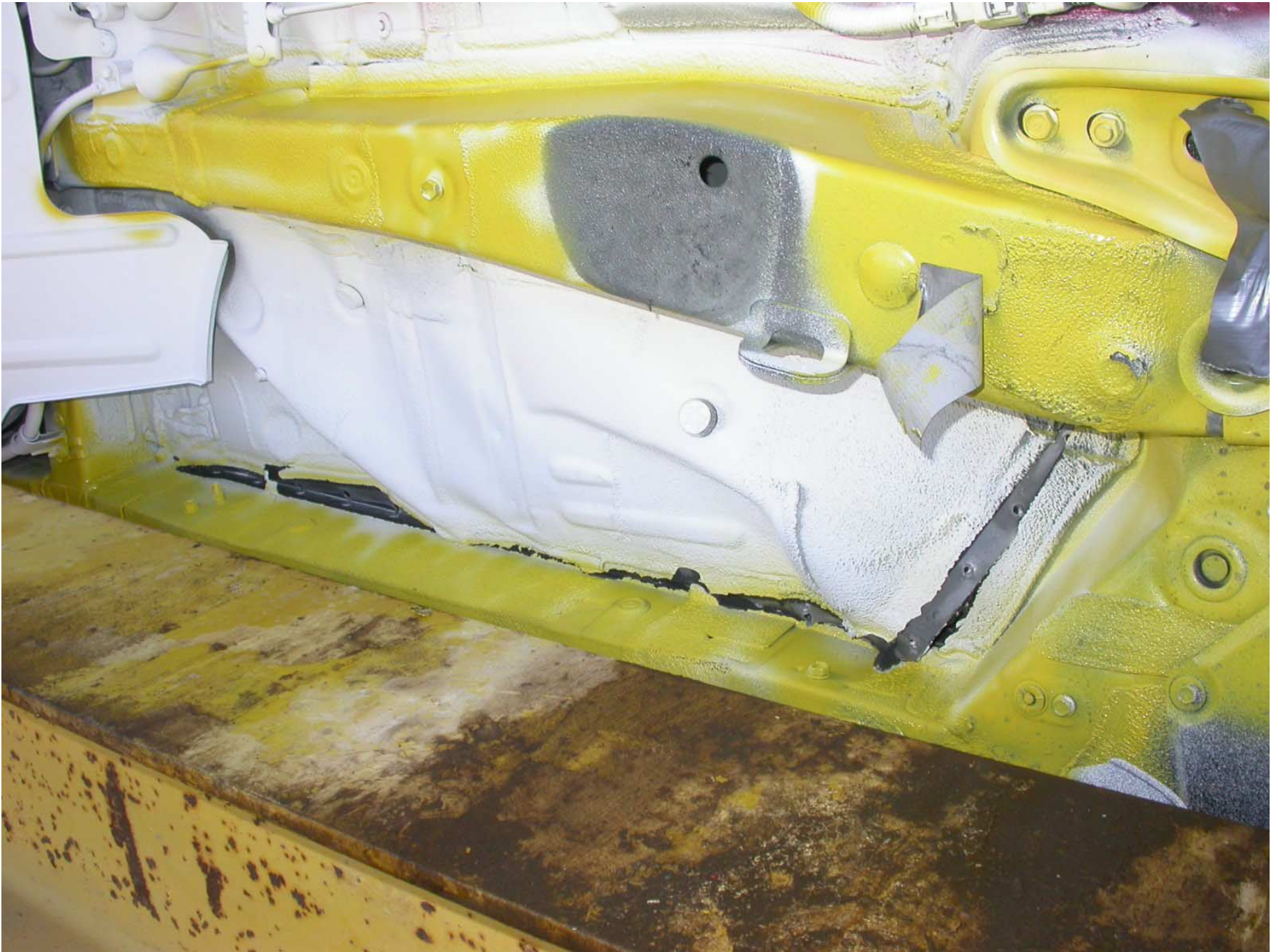
Figure A-65: Driver Side Floor Pan Separation (Underside View)
