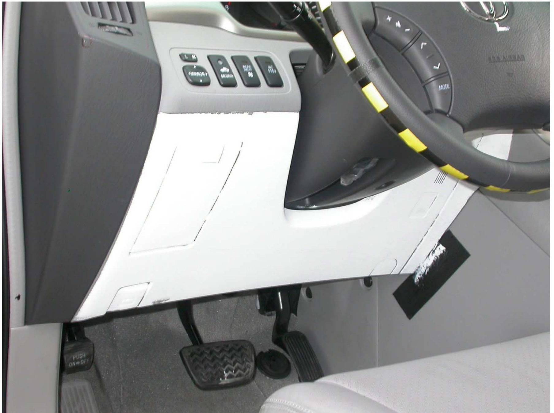
Figure A-38: Pre-Test Driver Side Knee Bolster
