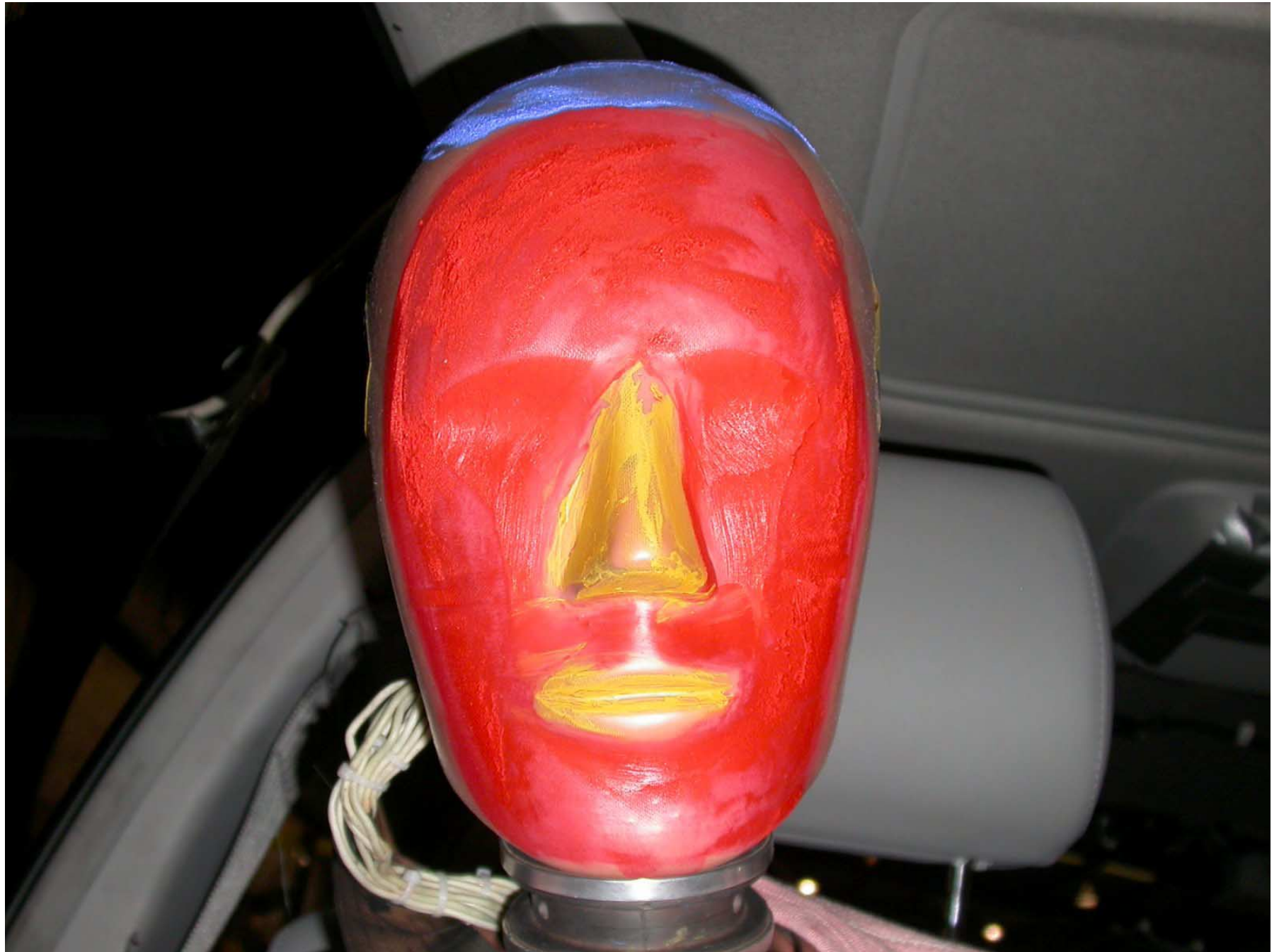
Figure A-56: Post-Test Passenger Dummy Head
