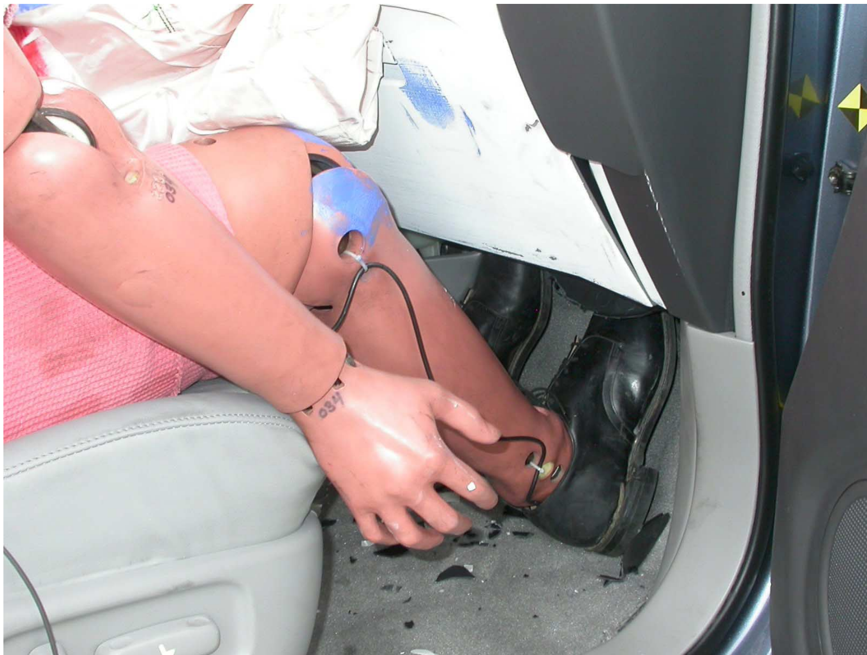
Figure A-51: Post-Test Passenger Dummy Feet
