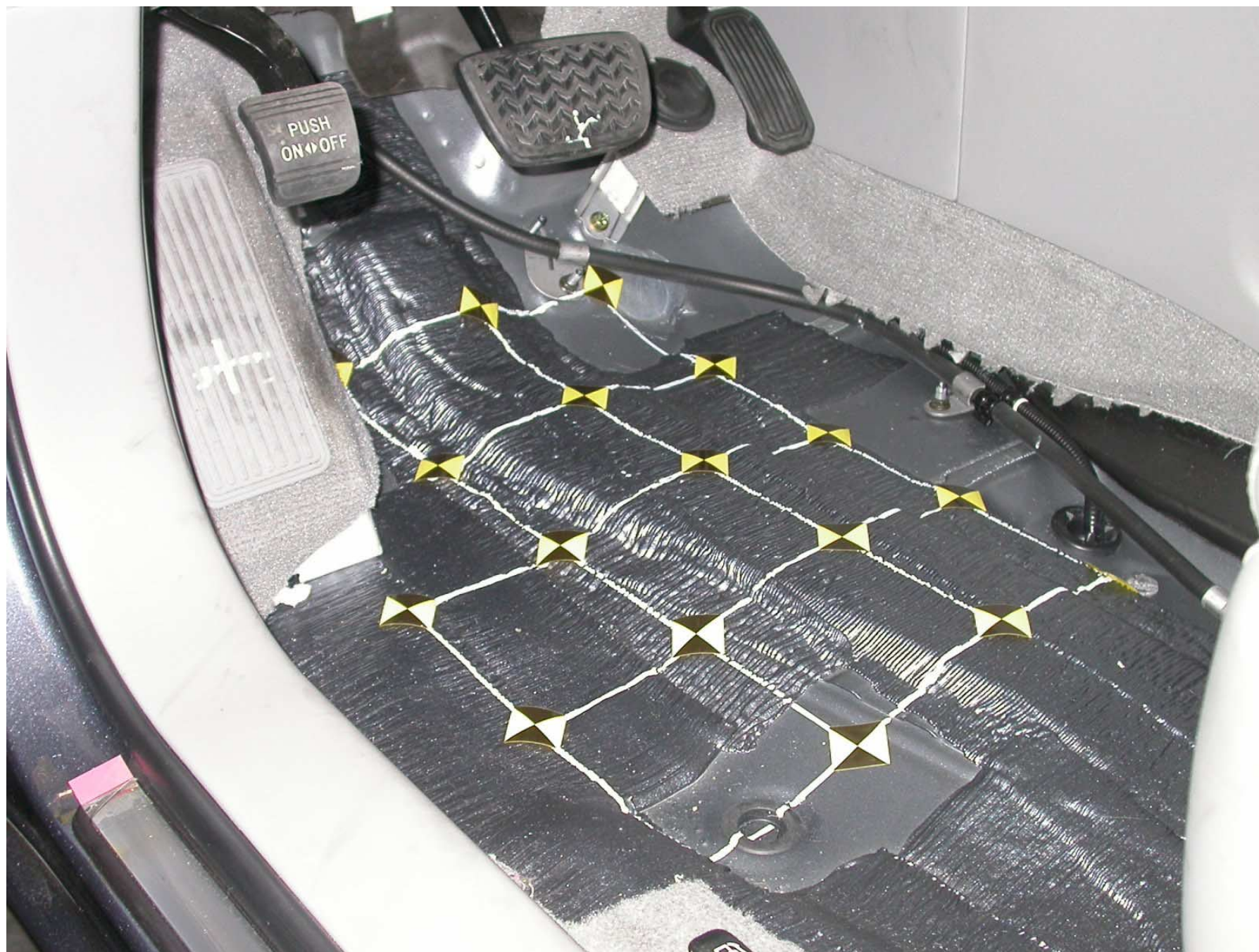
Figure A-40: Pre-Test Driver Side Floor Pan
