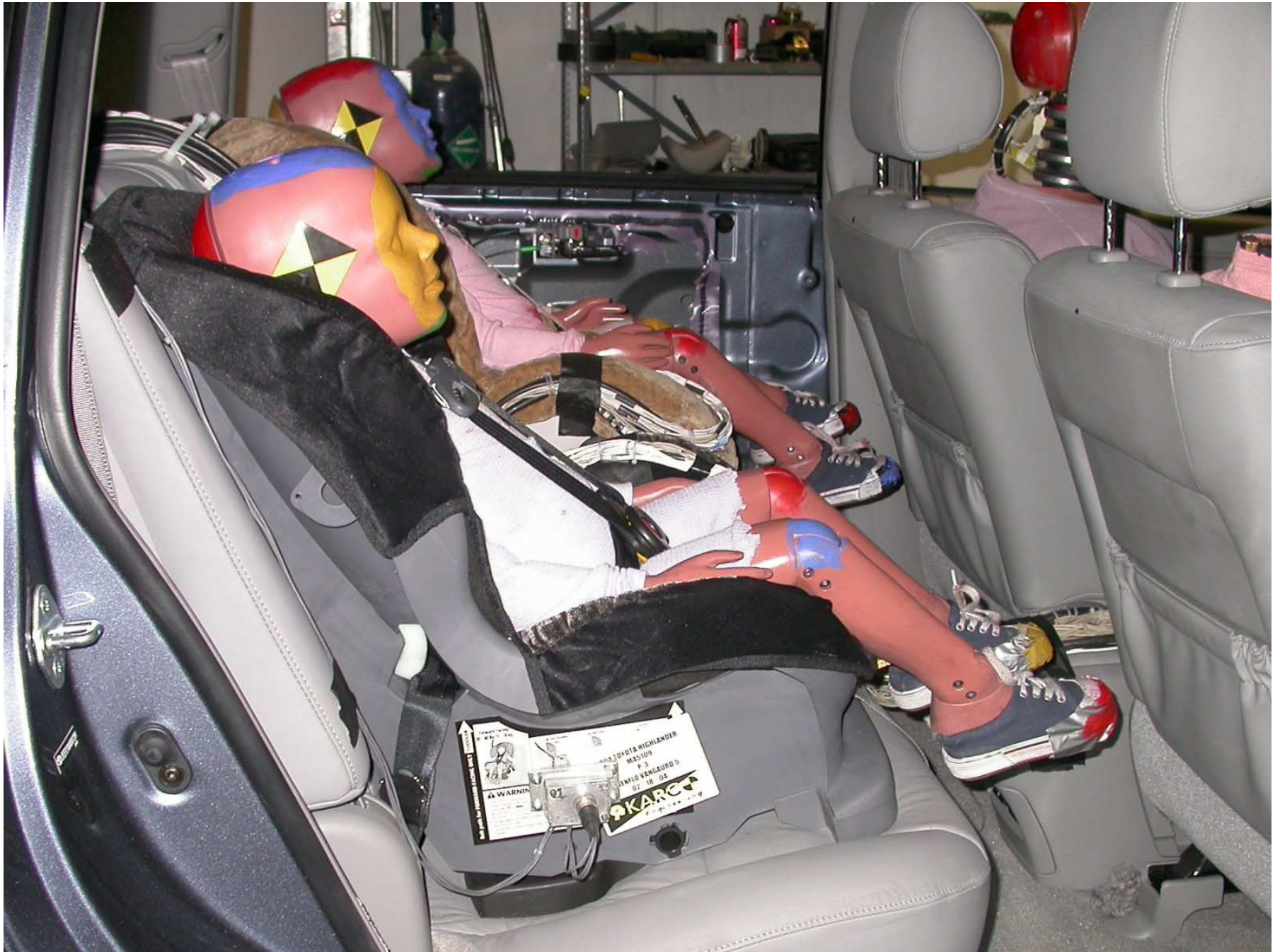
Figure F2-14: Pre-Test Position 3 Right Side View
