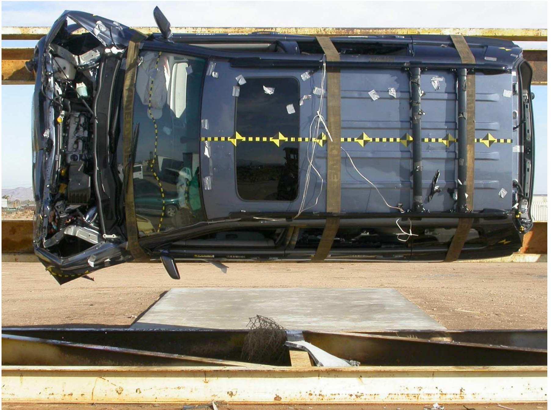
Figure A-59: Vehicle on Rollover Device
