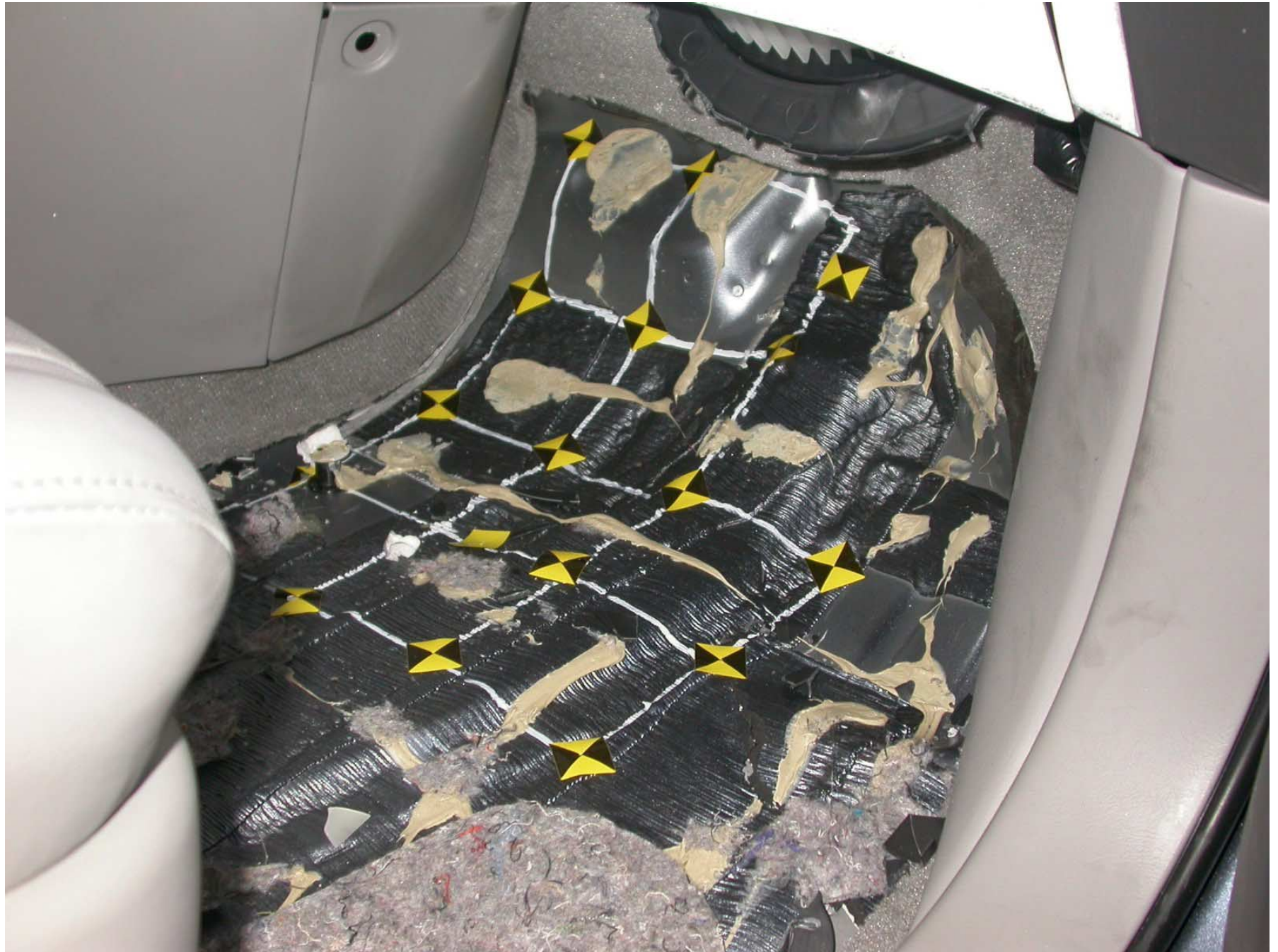
Figure A-55: Post-Test Passenger Side Floor Pan
