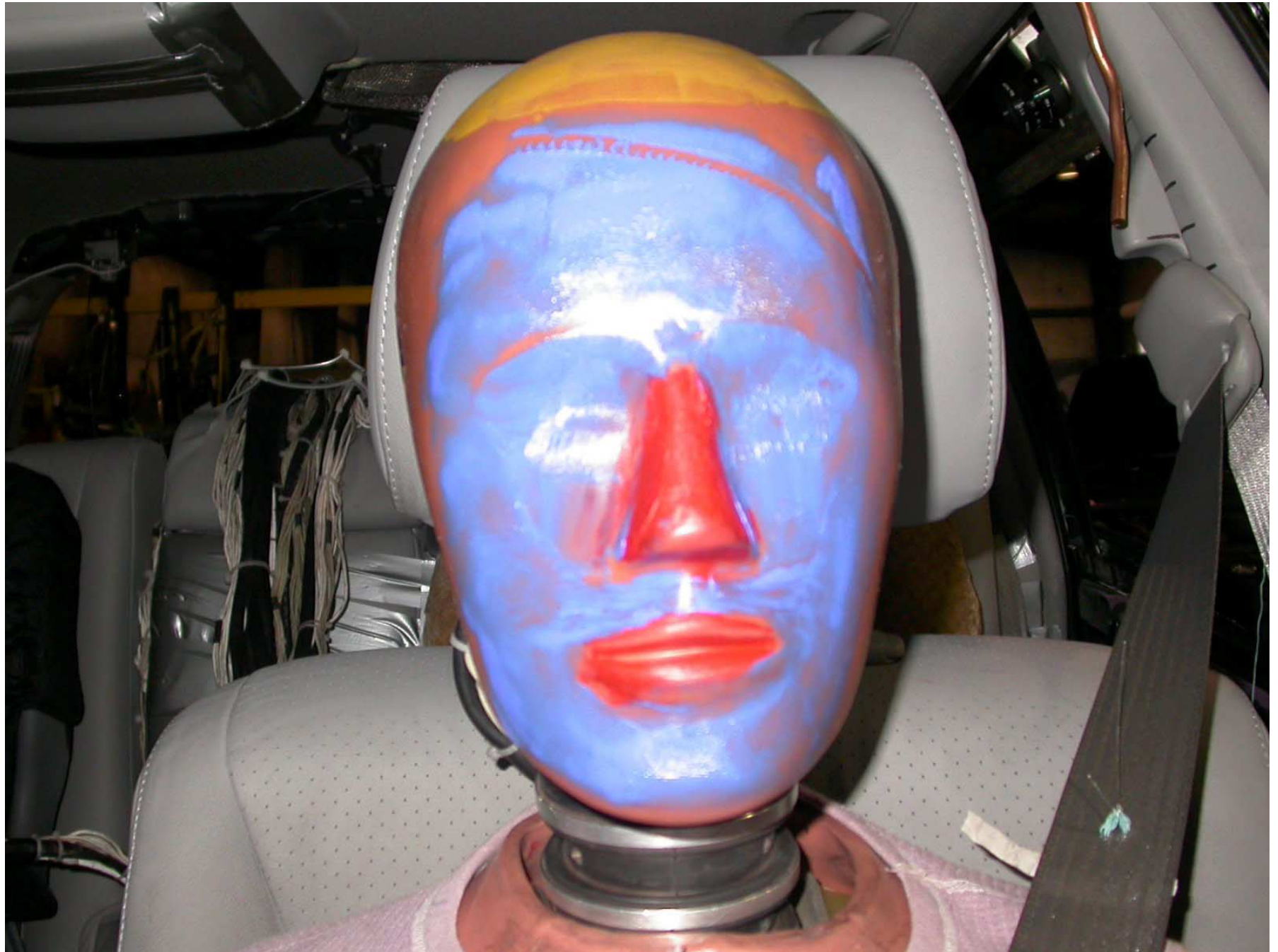
Figure A-42: Post-Test Driver Dummy Head
