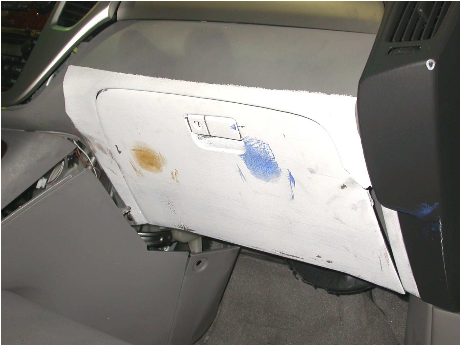
Figure A-53: Post-Test Passenger Side Knee Bolster
