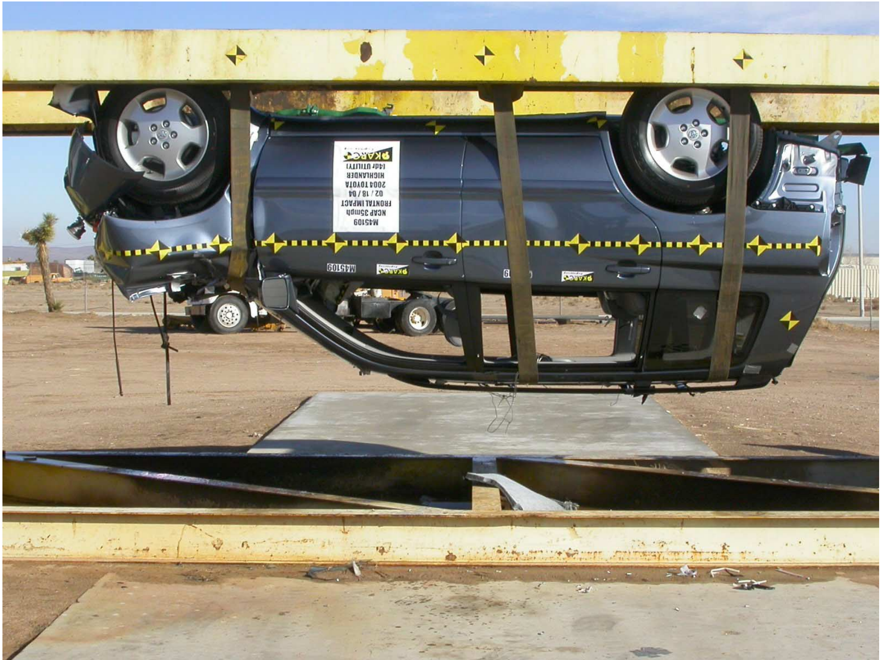
Figure A-60: Vehicle on Rollover Device
