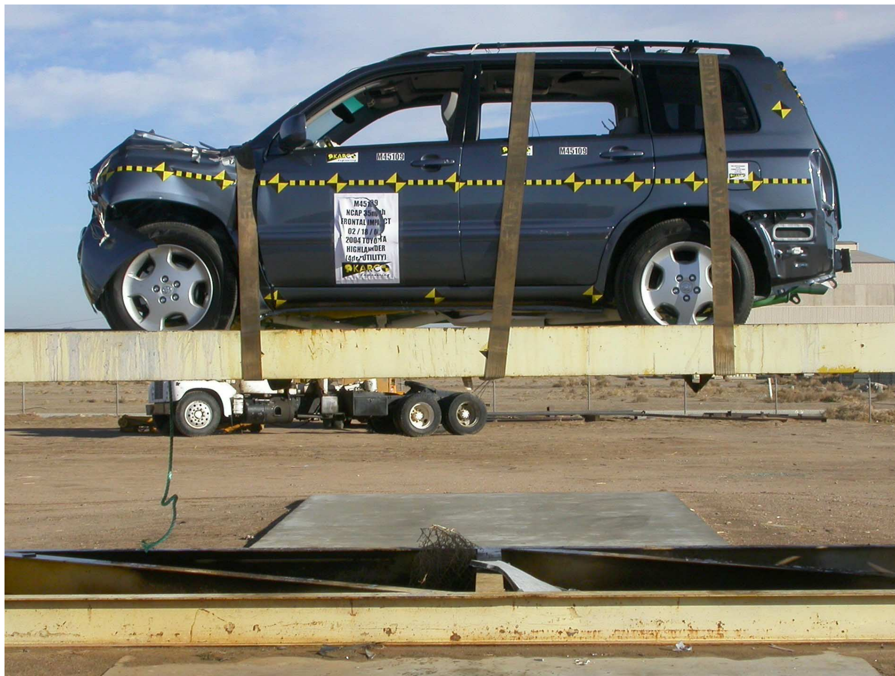
Figure A-58: Vehicle on Rollover Device
