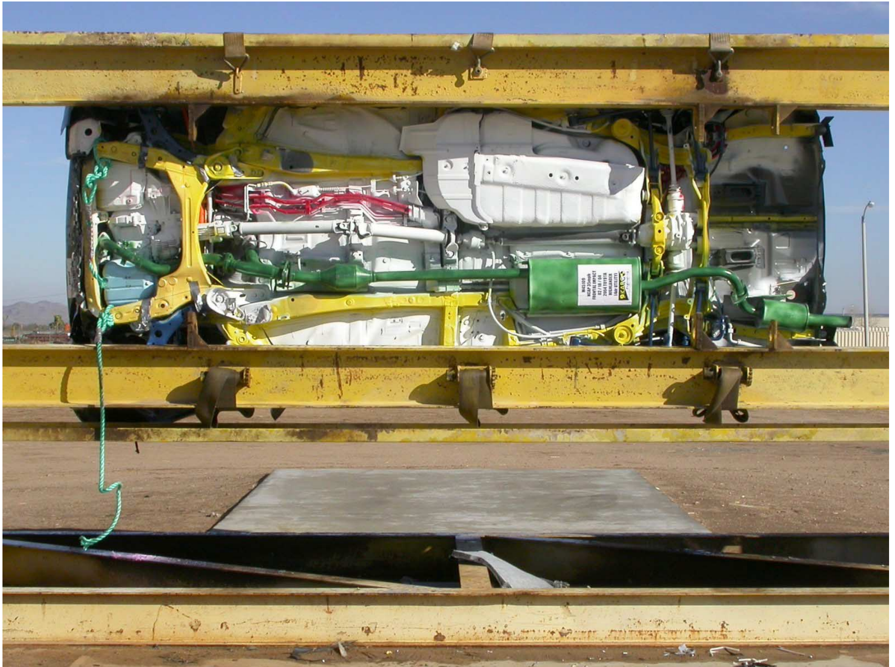
Figure A-61: Vehicle on Rollover Device
