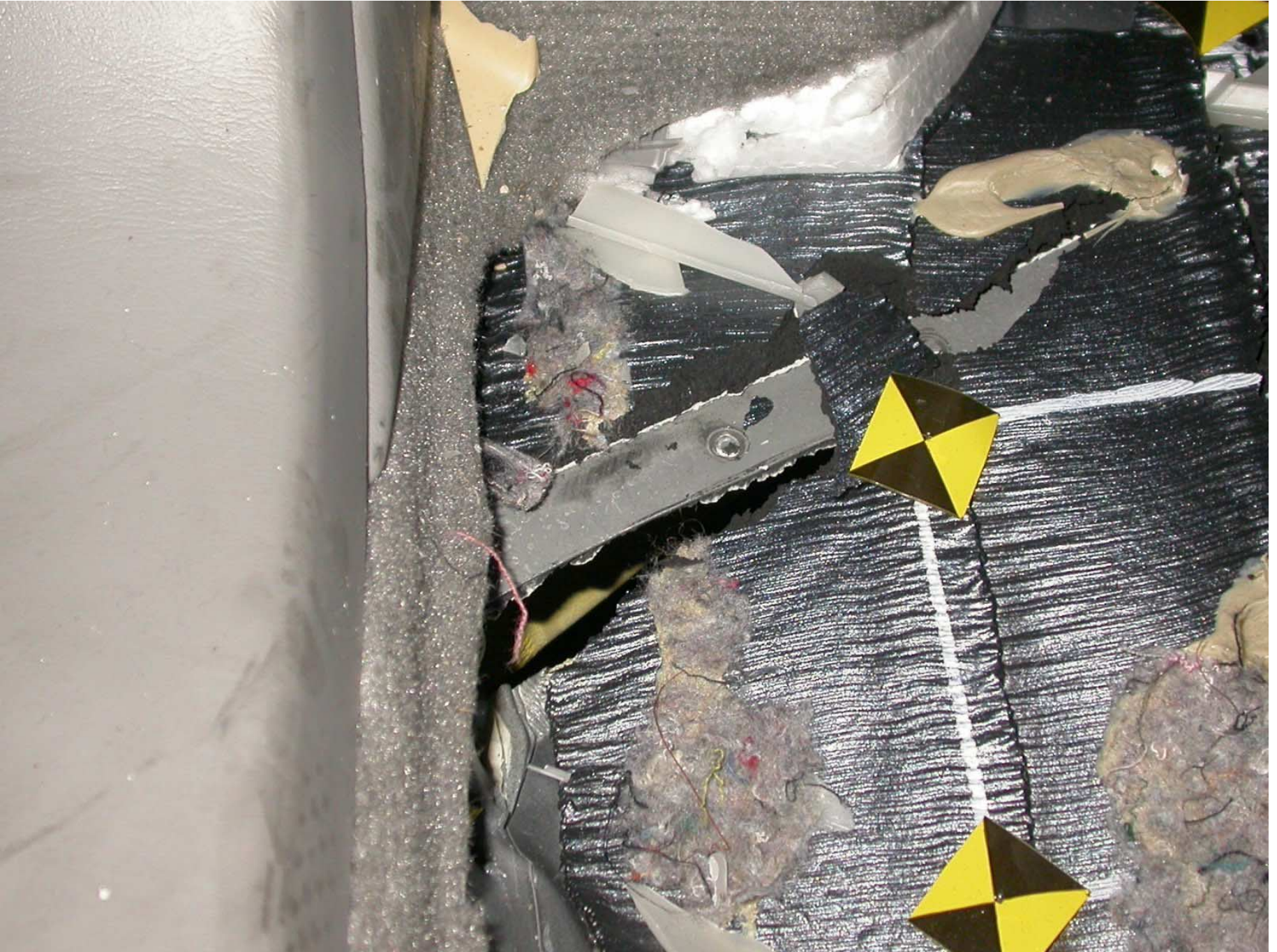
Figure A-64: Driver Side Floor Pan Separation (Inside View)
